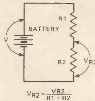
Fig. 8. The potential divider.
