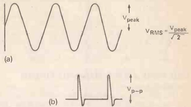
Fig. 6. (a) Peak and RMS. For a sinewave only, RMS voltage = peak voltage /  $\sqrt{2}$ . Using RMS values in power calculations will give true power (wrongly called RMS power) (b) Peak-to-peak measurement, often used in electronics.
