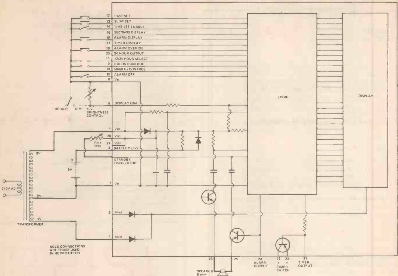
Above is the schematic for the clock module, the slightly thicker lines are the options we used on the prototype — other facilities can be used also if wired up on your version. On the left is the rear end of the HE prototype, as can be seen we did not have much room to spare for extra switch functions.
