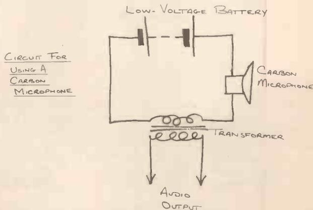
To make the microphone work usefully, the varying resistance must be converted to a varying electrical signal. This can be done quite simply by putting the microphone in series with a low voltage DC power source (could be a battery) and a transformer. As the resistance of the microphone varies, so too (from ohm's law) will the current through it. The current through the
