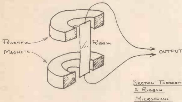
The signal generated by the ribbon is very small. Any length of wire to which it is connected would have a resistance large enough to reduce the signal quite considerably. For this reason a transformer is always mounted inside the microphone. The transformer increases the impedance and voltage of the ribbon's output so that any connecting wire has less attenuating effect. For obvious reasons this type of microphone is called a ribbon mike.
