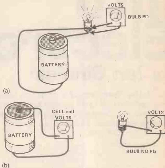
**Fig. 2. EMF and PD** (a) When a cell and a bulb are connected, we measure a PD across the bulb (b) When the cell and bulb are disconnected, we measure an EMF across the cell, but no PD across the bulb.
