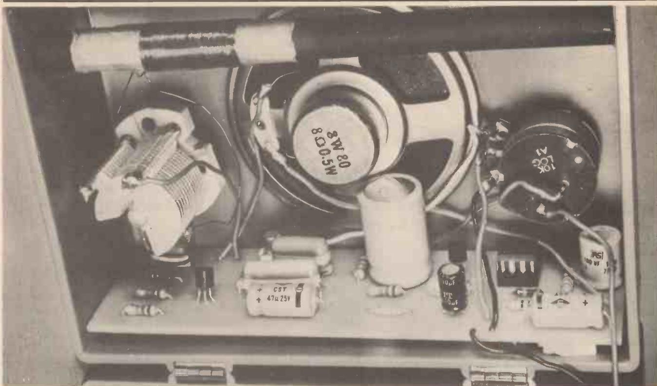
Close up view of our prototype, the aerial can be seen, near the top, we fixed it in place with 'sticky pads' which you can probably get from the same shop you get the board from — the
