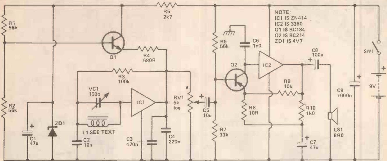
Circuit diagram of the complete Bedside Radio, winding details for L1 (the aerial) are given in the main text, although an
