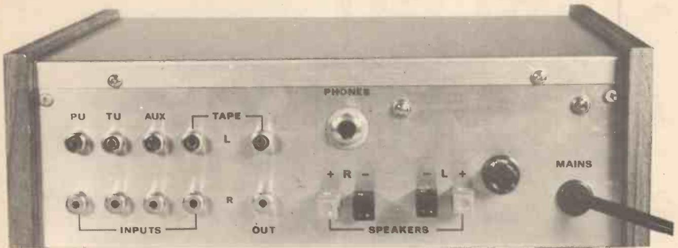
coping with up to four inputs, tuner, tape, radio and a magnetic pick-up. The amplifier also has a tape output socket. All inputs and outputs are brought to a group of phono sockets at the back of the Hobit.
