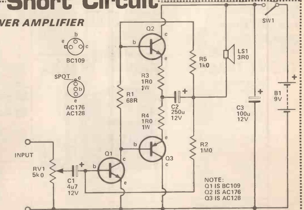
The signals are combined at the common emitter junction of Q2 and Q3, and passed to the loudspeaker through the large electrolytic capacitor C2. Small values of C2 result in a poor low frequency response. Negative feedback is provided by R5 and R2, these
