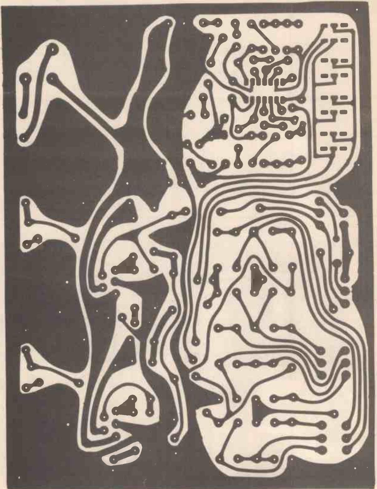
*The printed circuit board pattern shown here is the correct size. This can be copied either photographically or manually. However this and other PCBs should be available from advertisers in Hobby Electronics and next month we shall be giving details of Hobbiprints, a simple dry transfer method of making your own PCBs'.*
