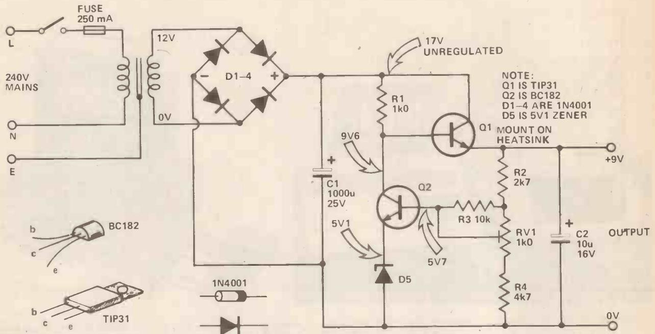
Two transistors and a voltage reference can be used to make a regulated power supply. Transistor Q1 is used as the power control element and so must be mounted on a heat sink. Q2 provides negative feedback and so helps to iron out any changes at the output
