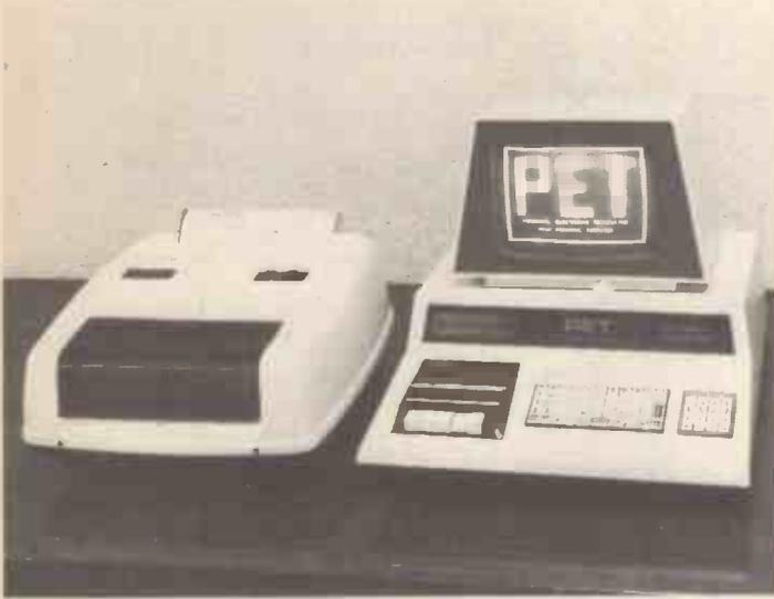
Commodore PET is a display, cassette, keyboard and computer all in a single cabinet. Based on a 6502 computer, the system has a built-in BASIC — stored in ROM. Standard memory is 8K plus 4K monitor system. PET is only supplied prebuilt.
