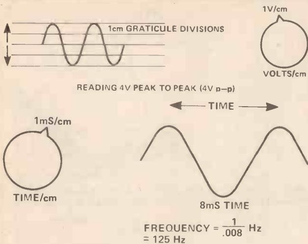
Fig. 13. Measuring the voltage and frequency of waveforms using the CRO.
