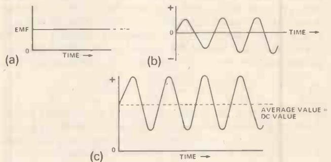
Fig. 5. AC and DC (a) The EMF from a cell is steady — a graph of EMF plotted against time is a horizontal straight line. (b) An alternating EMF has alternate + and - values which repeat at definite intervals. (c) When AC and DC exist together we may find that there are no negative (or no positive) values of EMF.
