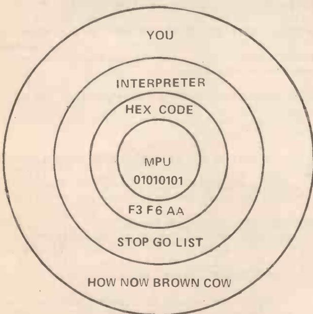
***The various levels between you (the real world) and the binary intelligence of a computer system. Most computers for use in the home have an interpreter level, although some are only useable with lower level 'machine code.'***
