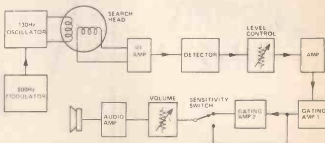
**Fig. 2. Block diagram of an IB metal locator. Techniques vary from machine to machine but the principle is the same. This diagram is of the IB Metal Locator Mk 1 from our sister magazine Electronics Today International.**
