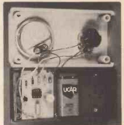
Using just a single 555 IC, this project can be built on either a PCB or Veroboard — we give you details for both. The beat rate can be varied from 30 to 120 beats a minute.
