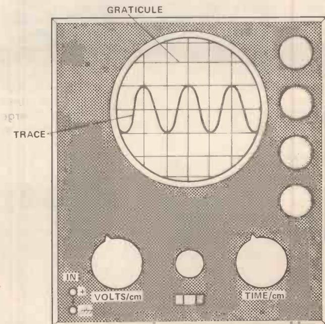
Fig. 12. The front panel of the CRO with the important operating controls labelled. The other controls are used for setting up.
