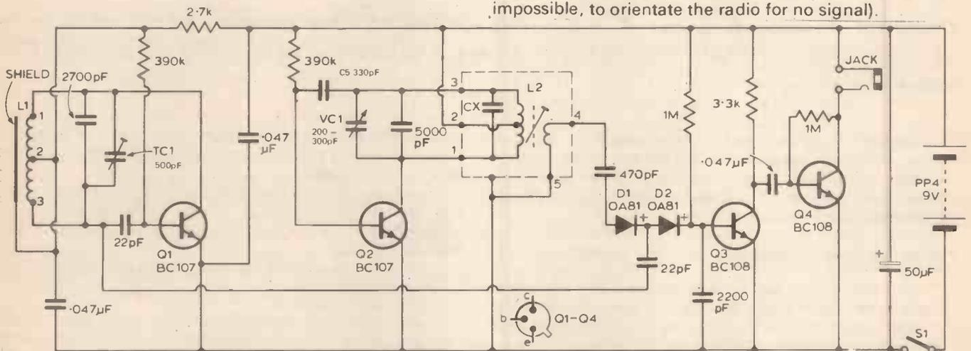
Fig. 3. Complete circuit of a BFO metal locator. A complete description of this appears in ETI Top Projects 1&2. Q1 and the surrounding components form the search oscillator. L1 is made from 50 turns of 26 s.w.g. on a 130 mm former, centre tapped.
