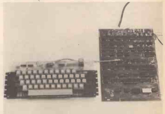
A photo of the Lynx 'NASCOM 1' system. This uses the 8080 processor's 'big brother': the Z-80. The Z-80 will handle programs written for itself (naturally enough) and for the 8080. This makes it a very useful device.
