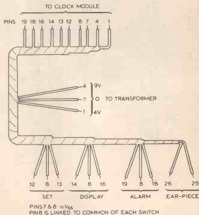
*How we wired up the prototype, if you want you can wire individually and then wrap a wire around the bundle to form a loom.*
