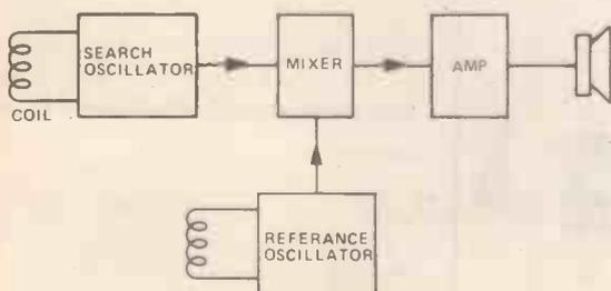
**Fig. 1. Block diagram of a typical BFO metal locator. It is the coil in the search oscillator that is panned over the ground. The second coil, associated with the reference oscillator, is in with the majority of the components.**
