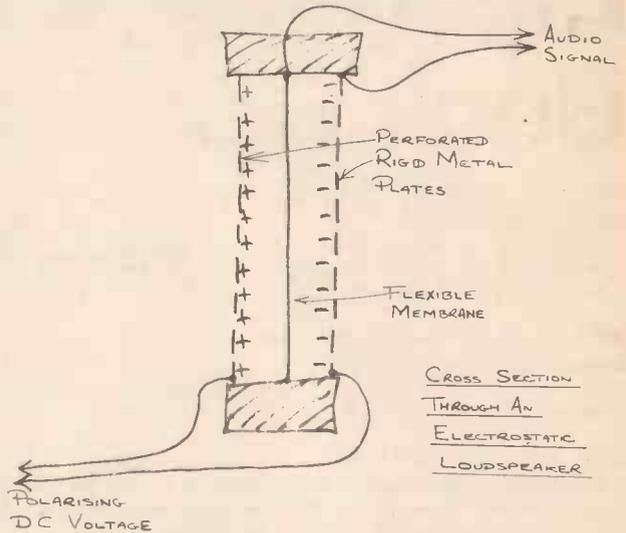
The charge on this plate will be changing with the audio signal. When there is a positive charge on the centre plate it will be attracted to the rigid negative plate, and repelled from the positively charged plate. The centre plate will vibrate, producing a sound output for the electrical input. A company in England (Quad) has been producing electrostatic speakers based on this principle for the last 20 years.
