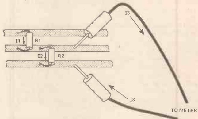
Fig. 11. Errors caused by a voltmeter. The current flowing through R1 must split, some going through R2, some through the meter. More current is being drawn through R1 now than when the meter was not present.
