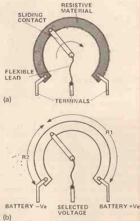
Fig. 9. A volume control is a variable potential divider. (a) construction, (b), use in setting a steady voltage level.
