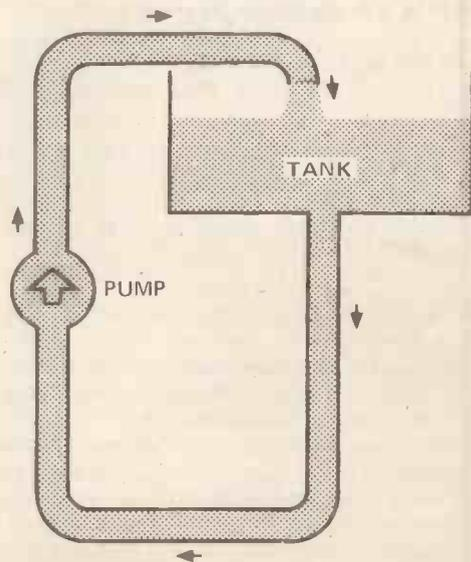
*Fig. 1. Currents. A water current, moved by a pump, can be kept moving if the same water is constantly re-cycled.*
