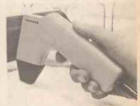
Optical character recognition (OCR) is the term for computer recognition of printed matter. This hand-held OCR scanner by Siemens, when passed along the line of text, enables the attached minicomputer to 'read'.
