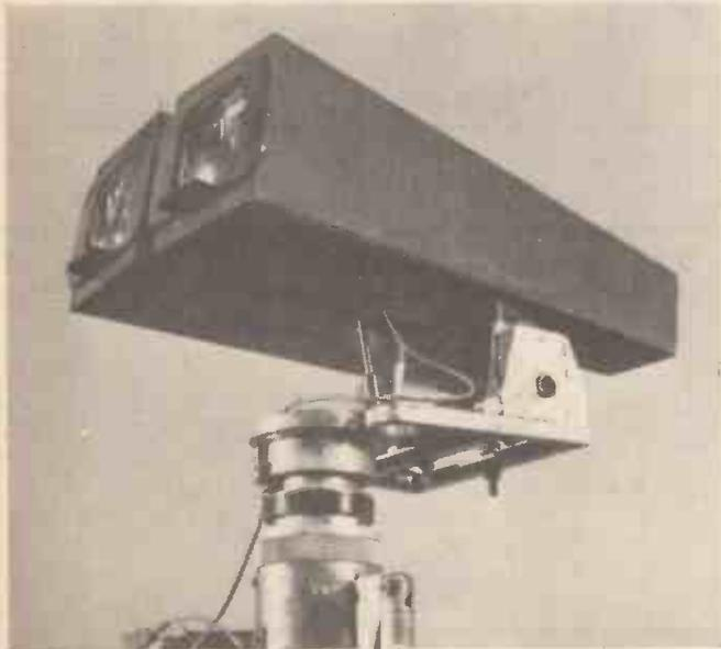
*This closeup of a Star Wars robot gives an idea of the probable visual aids robots will use. Even though the twin TV cameras in this robot were dummies, real robots will have to use some form of image recognition. The main holdup is in the computer techniques needed to interpret the signals from the 'eyes' of the machine.*
