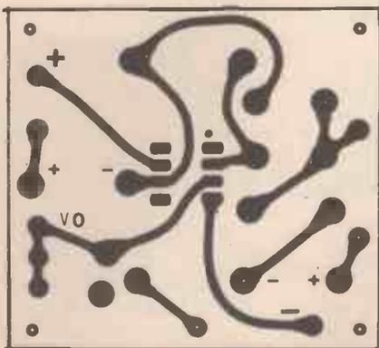
The printed circuit foil pattern (looking at the copper side of the board). This can be used to make your own PC board or ready-made ones can be bought (see adverts in this and later issues).
