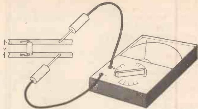
Fig. 10. A voltage measurement. The leads of the voltmeter are connected between the points where voltage is to be measured.
