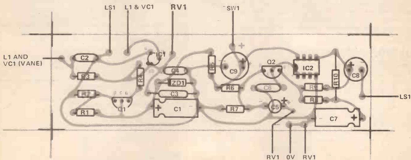
How to position the components on the PCB, make sure the transistors, integrated circuits, diode and electrolytic capacitors are the correct way round before soldering in place.
