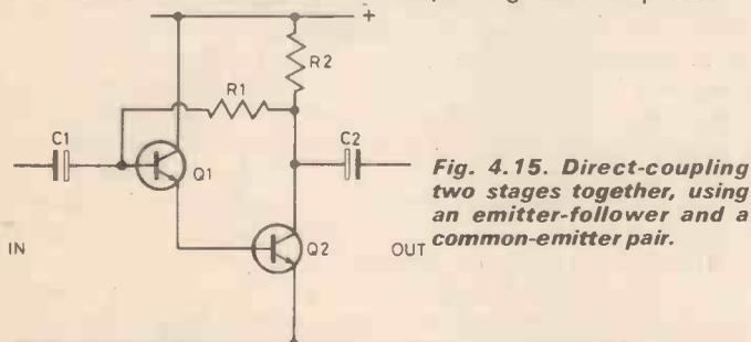
Fig. 4.15. Direct-coupling two stages together, using an emitter-follower and a common-emitter pair.
