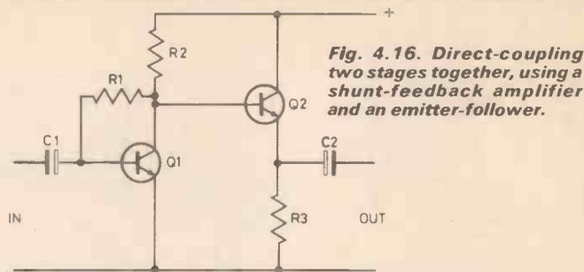
Fig. 4.16. Direct-coupling two stages together, using a shunt-feedback amplifier and an emitter-follower.
