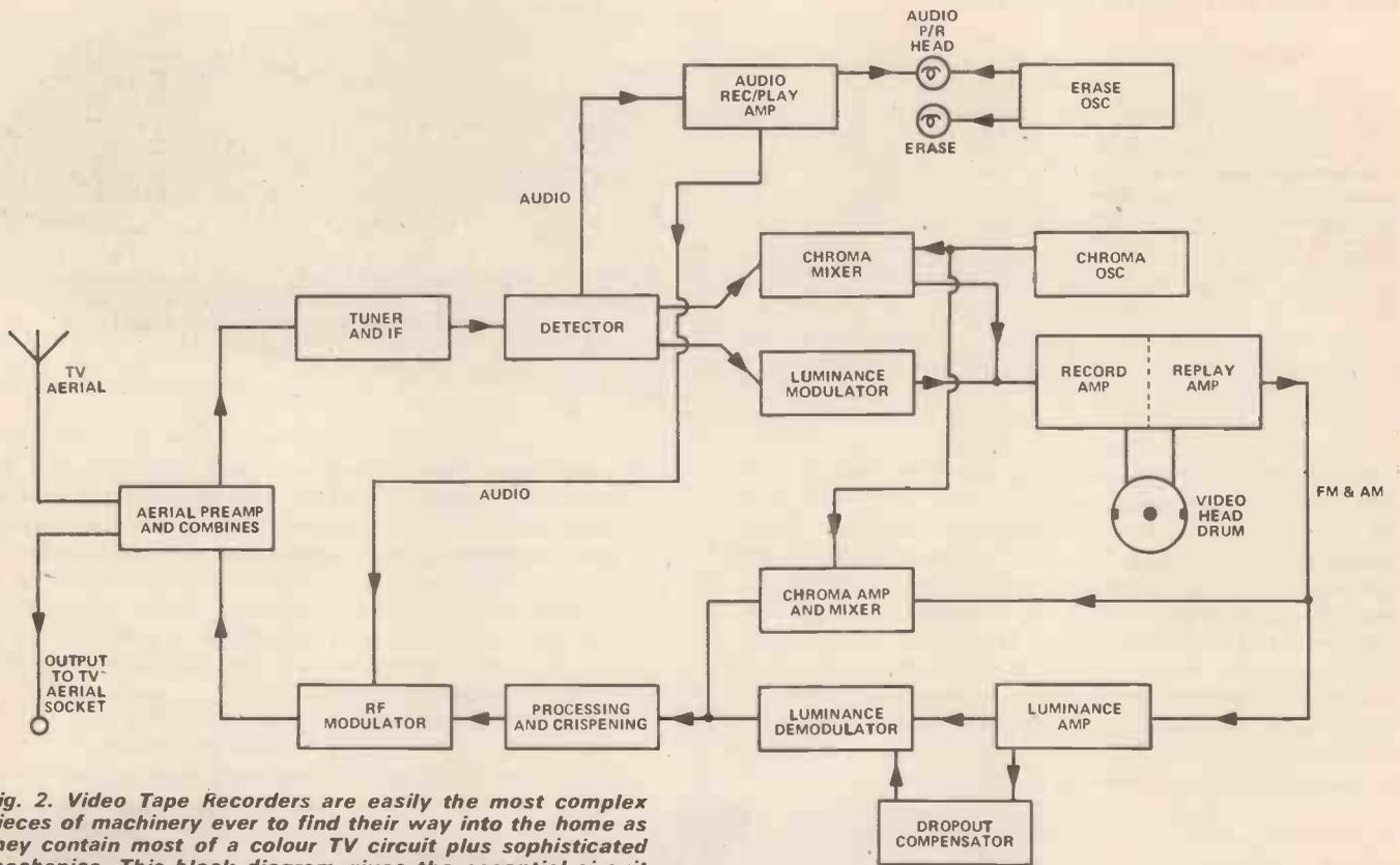
**Fig. 2. Video Tape Recorders are easily the most complex pieces of machinery ever to find their way into the home as they contain most of a colour TV circuit plus sophisticated mechanics. This block diagram gives the essential circuit elements; see the text for a more detailed explanation.**
