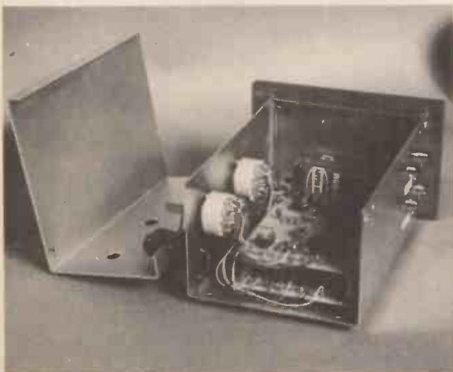
*Inside the stereo version of the filter — two identical PCBs are used, but only a single battery and power switch are needed.*
