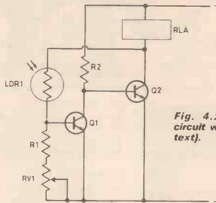
**Fig. 4.20. A light-relay circuit with hysteresis (see text).**
