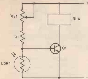
**Fig. 4.18. Circuit for operating a relay when the light level drops.**
