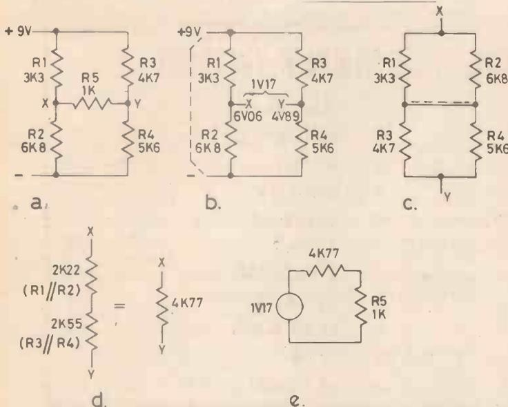
Fig. 6. The bridge circuit (a) is unbalanced. The open circuit voltage across R5 is easily found (b); finding the resistance (c) needs a little bit of re-drawing (d). The final equivalent is shown in (e).
