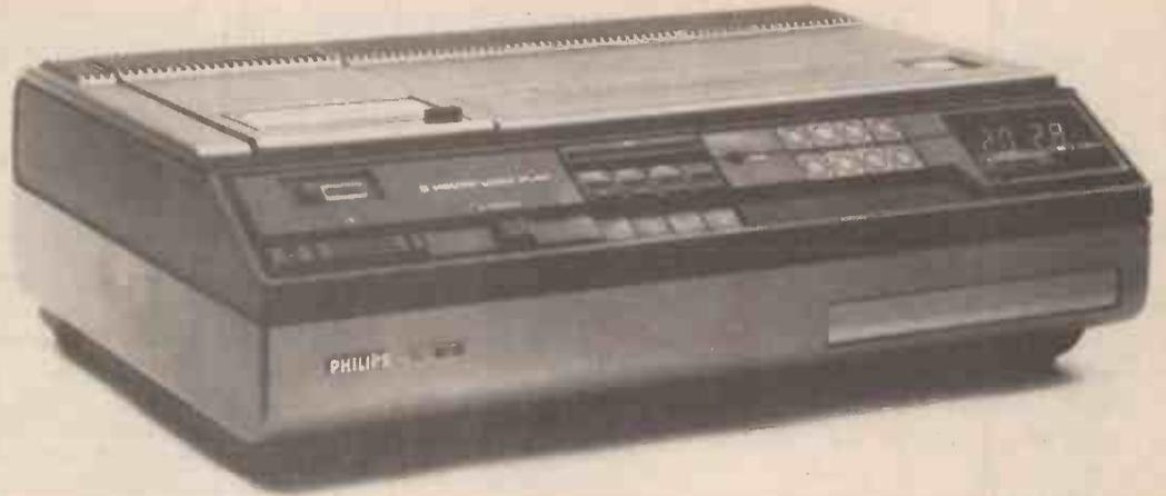
conveniently cover the audio spectrum between 50 Hz and 20 kHz but is obviously insufficient to cover the 50 Hz to the 5 MHz of video frequencies. However, by frequency modulating this wide bandwidth video signal onto a carrier, all these frequencies can be effectively shifted up the spectrum where they can be very conveniently handled, within this octave limitation.
