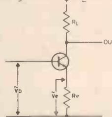
**Fig. 4.7. Series negative feedback using the emitter resistance  $R_e$ .**
