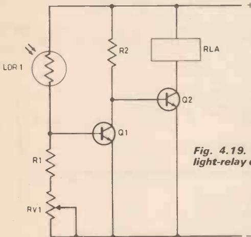
**Fig. 4.19. more sensitive light-relay circuit.**
