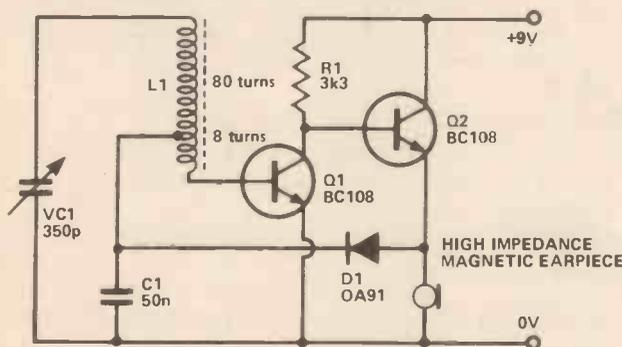
Although transistors are cheap, this was certainly not true some years ago and transistors were made to work at maximum efficiency. A common technique in simple radio circuits was to use a reflex circuit, that is one transistor amplified both at RF and AF.
