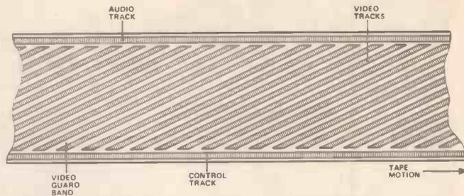
**Fig. 1.** The high tape head to tape speed is achieved by rotating the heads to give diagonal strips of recorded material. The audio is recorded on a narrow track on one edge.
