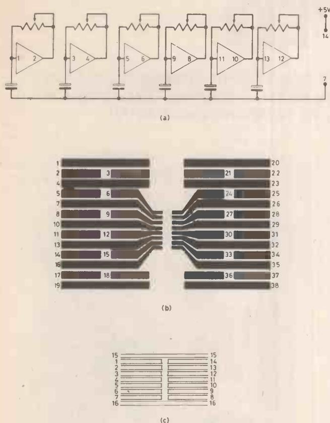
Fig. 4. Sample IC circuit (A), with 1-IC Blob layout (B) and 0.1in Vero cut-out diagram (C).
