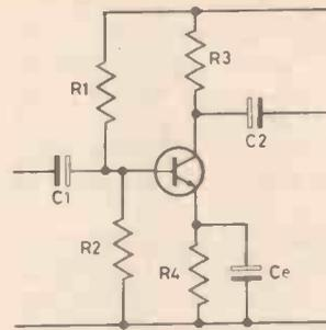
Fig. 4.9. Using a decoupling capacitor ( $C_e$ ) so that there is no series feedback caused by the emitter resistor  $R_4$ .
