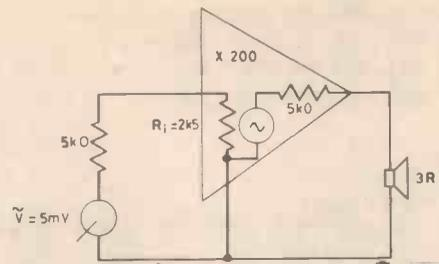
**Fig. 4.4. Single-transistor amplifier, input from a pick-up cartridge, output to a loudspeaker.**
