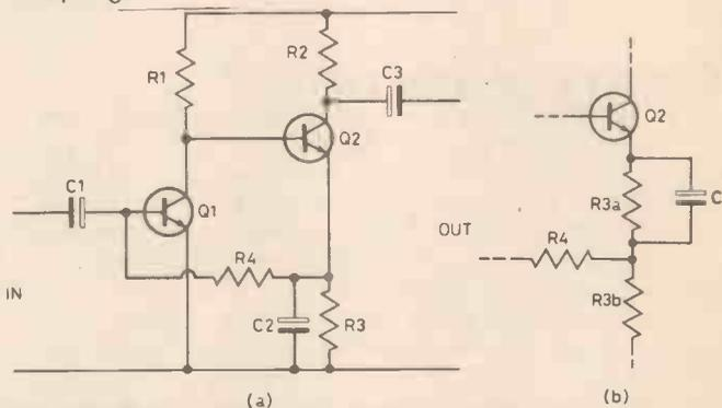
Fig. 4.17. A high gain two transistor circuit (a) with direct coupling negative feedback of signal can be achieved by removing C2, or by using the circuit in (b) where only part of R3 is bypassed.
