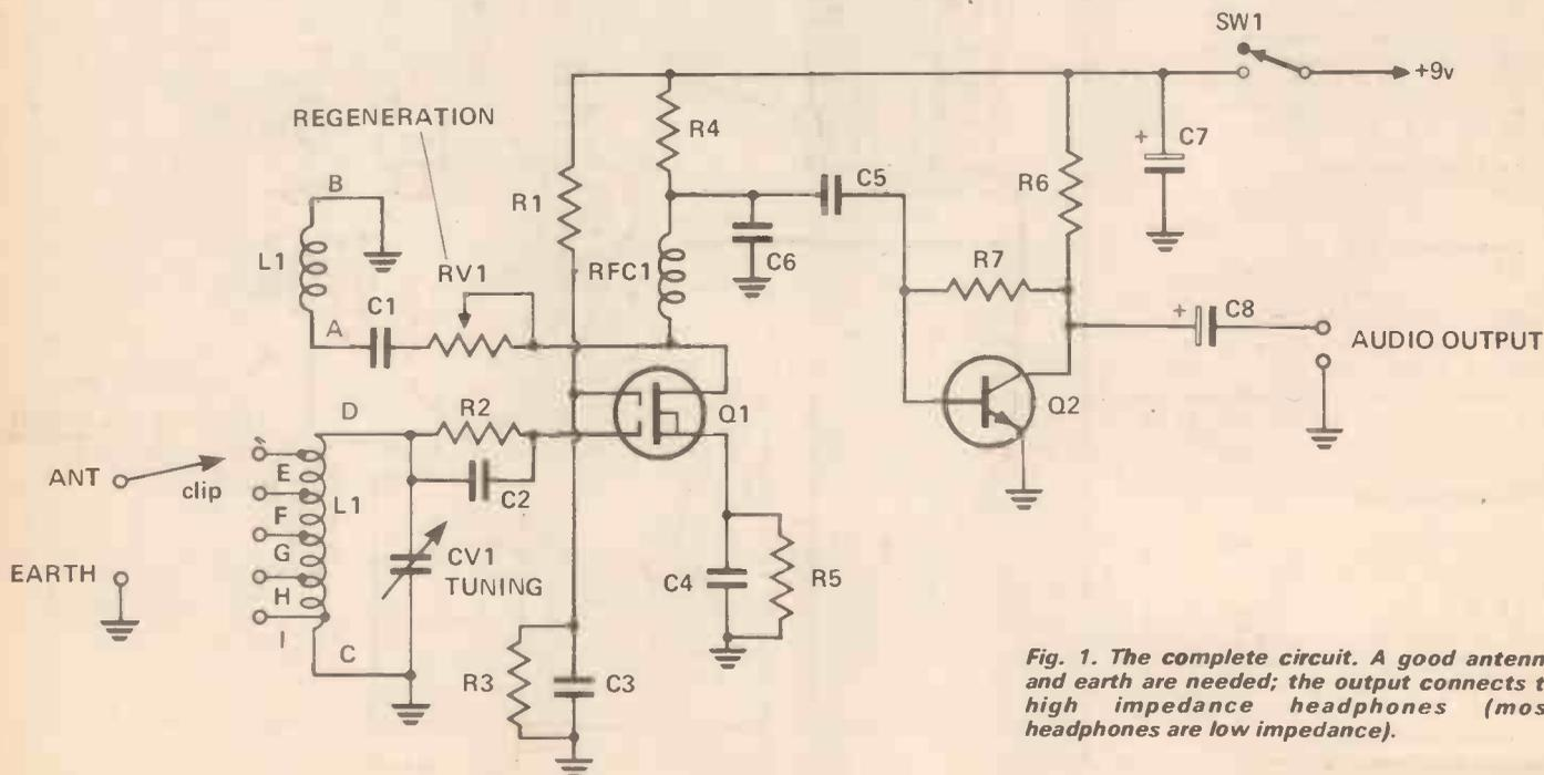
*Fig. 1. The complete circuit. A good antenna and earth are needed; the output connects to high impedance headphones (most headphones are low impedance).*
