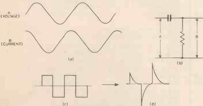
**Fig. 4.13. The effect of capacitor coupling on low-frequency signals. (a) Phase shift of voltage relative to current, (b) in the coupling circuit, the output voltage (A) is not in phase with the input voltage (B) to the next stage. A low frequency square wave (c) becomes distorted to the spiked shape (d) unless very large capacitance values are used.**
