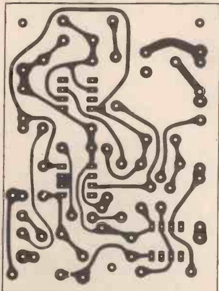
The PCB pattern for the car alarm, shown here full size.
