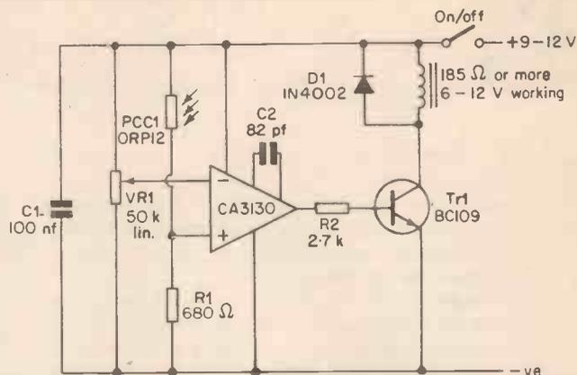
**Fig. 3. If the light falling on PCC1 falls below a certain level, the output of IC1 goes high, turning on Tr1 which operates the relay.**
