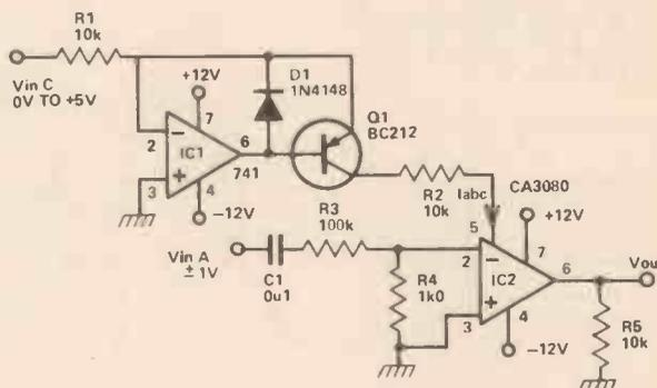
A simple voltage controlled amplifier (VCA) can be made using a CA3080 which is an Operational Transconductance Amplifier made by RCA. This is basically an op-amp with an extra input at pin 5. A current  $I_{abc}$  is injected into this input and this controls the gain of the device linearly. Thus by inserting an audio signal ( $\pm 10$  mV) between pin 2 and 3 and by controlling the current on pin 5, the level of the signal output (pin 6) is controlled.
