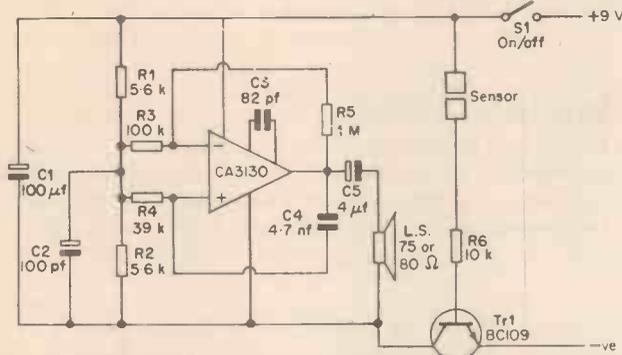
**Fig. 2. Rain alarm circuit.** Basically an audio oscillator with the negative supply controlled by Tr1. When a drop of rain bridges the sensor, Tr1 acts as a low value resistor allowing current to reach the rest of the circuit.
