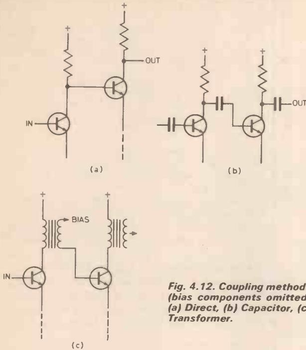
**Fig. 4.12. Coupling methods (bias components omitted) (a) Direct, (b) Capacitor, (c) Transformer.**
