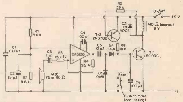
Fig. 8. A self-latching version of Fig. 7. In this arrangement Tr1 and Tr2 act in much the same way as a thyristor (SCR).
