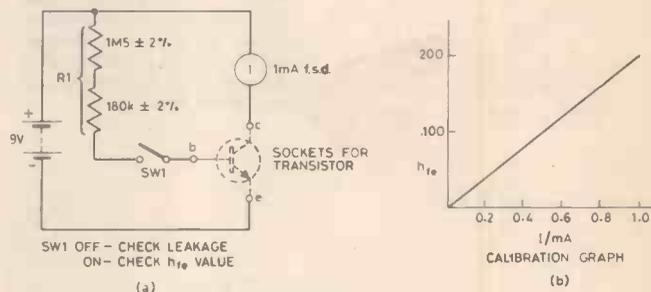
Fig. 4.1. Simple transistor tester circuit (a), with calibration graph (b). If any reading appears on the meter before SW1 is pressed, the transistor is leaky and should be rejected.
