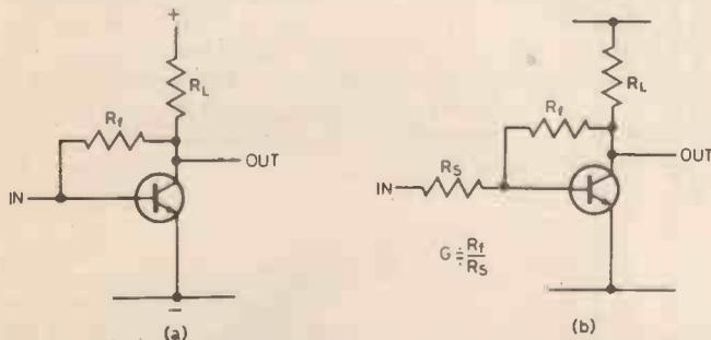
**Fig. 4.6. Shunt negative feedback (a) simple circuit, ignoring bias. (b) Rule-of-thumb formula for finding gain.  $R_s$  is the "source" resistance, either wired in circuit or part of the previous stage resistance.**
