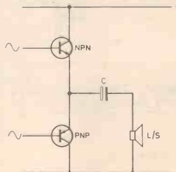
Fig. 4.11. The 'totem-pole' circuit, with two emitter followers, which is used as an output stage to drive loudspeakers. One transistor is NPN, the other PNP.
