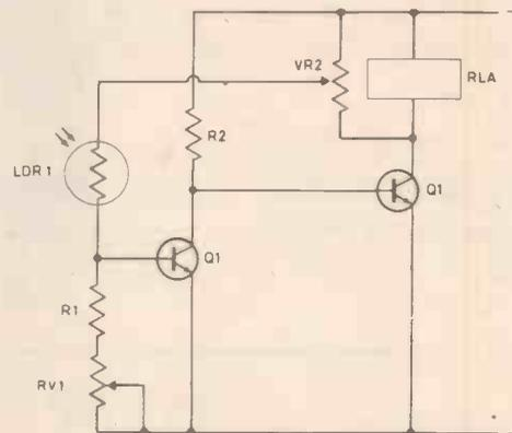
**Fig. 4.21. A more controllable circuit with variable hysteresis.**
