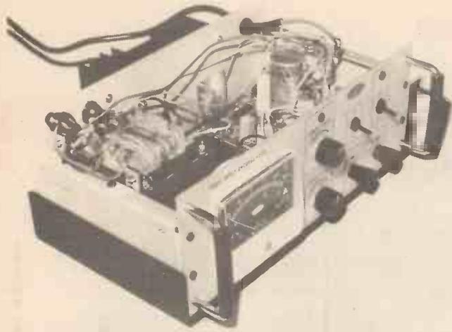
With the lid off the exposed transformer tags can be seen at the left of the box.
