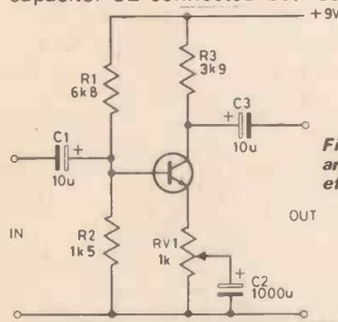
Fig. 4.8. A practical arrangement for testing the effect of series feedback.
