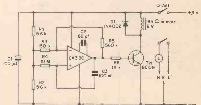
Fig. 9. C3 and R4 make the IC oscillate slowly and in turn the relay switches on and off in sympathy.
