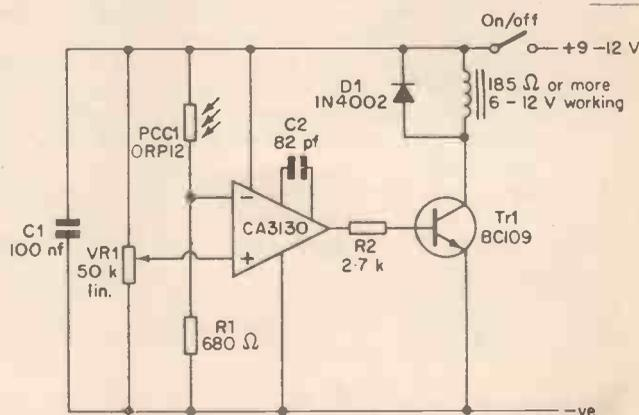
**Fig. 4 Connecting Fig. 3. differently, the same components can be used to switch when the light level increases.**
