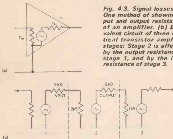
**Fig. 4.3. Signal losses. (a) One method of showing input and output resistances of an amplifier. (b) Equivalent circuit of three identical transistor amplifier stages; Stage 2 is affected by the output resistance of stage 1, and by the input resistance of stage 3.**
