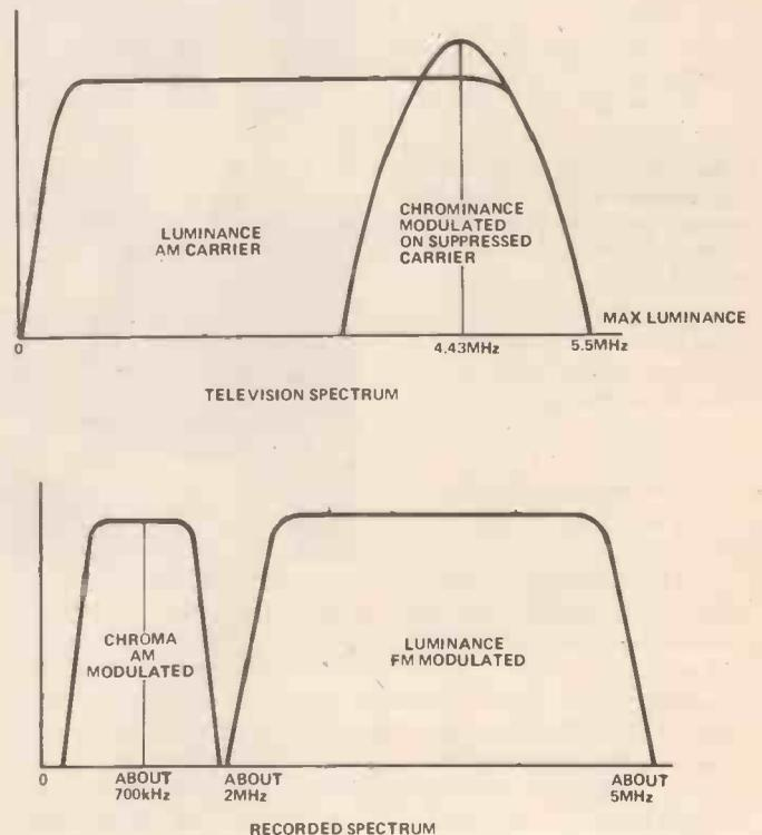
**Fig. 3. To get the most out of a tape recorder, the original TV spectrum is considerably rearranged when put on the tape. The whole luminance section (the monochrome picture) is shifted up the spectrum and is frequency modulated. The colour information is slotted onto lower frequencies and amplitude modulated.**
