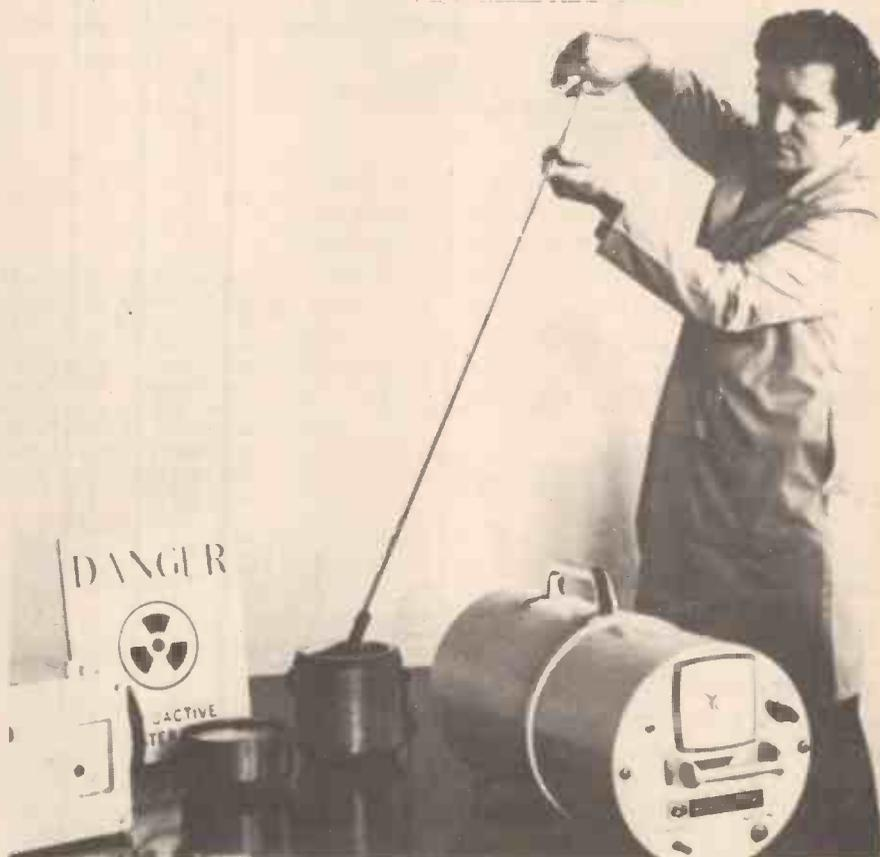
*The operator uses long tongs to keep his body away from the radioactive material in the container, whilst the monitor continuously checks the radiation level. (Courtesy Nuclear Enterprises Ltd.)*
