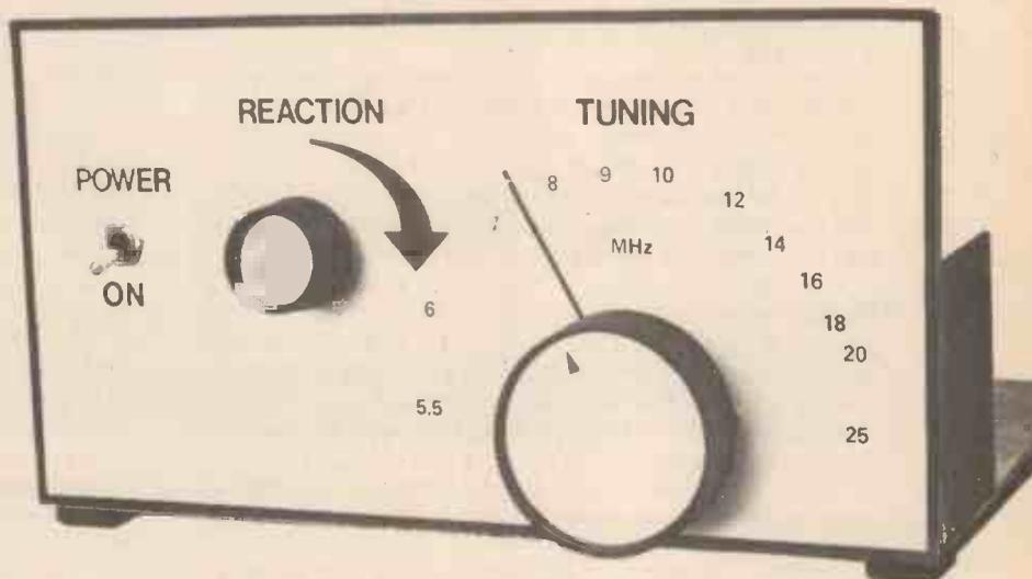
APART FROM THE very early sets, which were based upon coherers and other devices you rarely hear of today, the first radios were very straightforward designs totally unlike today's sophisticated superhets. The early Tuned Radio Frequency (TRF) sets were simply a tuning circuit with some gain and a detector circuit. Later designs used positive feedback, in the form of reaction, to increase the performance and it is still possible to get a lot of fun from sets of this type.
