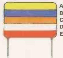
A = 4, B = 7, C = -- n, so value is 47 n; D = accuracy = 10%; E = voltage = 250 V
