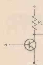
(1)  $G = \frac{h_{fe} R_L}{r_{ie}}$  where  $h_{fe}$  is current gain,  $R_L$  is value of load resistor, and  $r_{ie}$  is input resistance.
