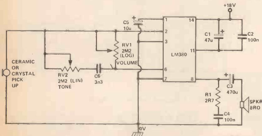
Fig. 7. A practical 2-watt phono amplifier with 'common mode' volume and tone controls.
