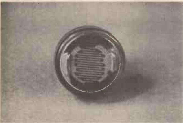
Close up of an LDR, note the track (silver) is cut across the face of the device to expose the maximum amount of resistive element to light.
