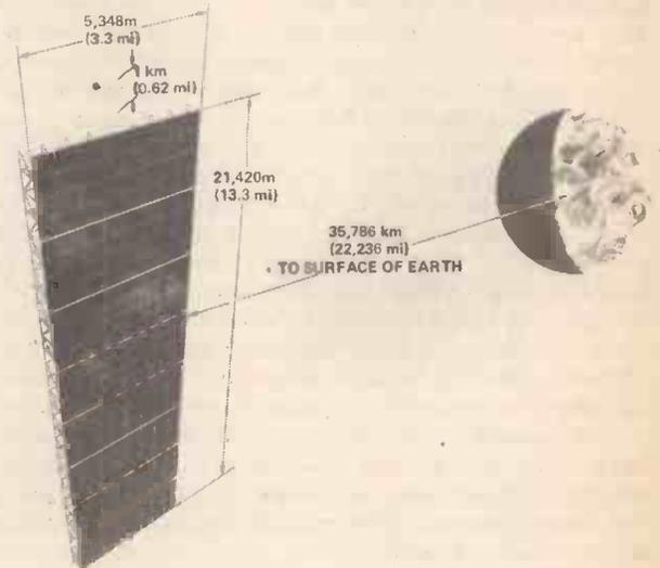
radiator for dispersion into space. The space radiator could employ a liquid metal loop with a helium/liquid metal heat exchanger. A liquid alkali metal such as potassium, would suffer little contamination in space. The gas turbines would drive a dynamo. As there would be no gravitational force in the region, the turbo-generators could be entirely supported by gas bearings.
