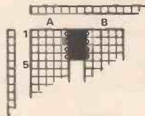
**Fig. 2.** How the small 8-pin IC fits on to the Eurobreadboard. This is the position which will be used in all the circuits in this series using these ICs.
