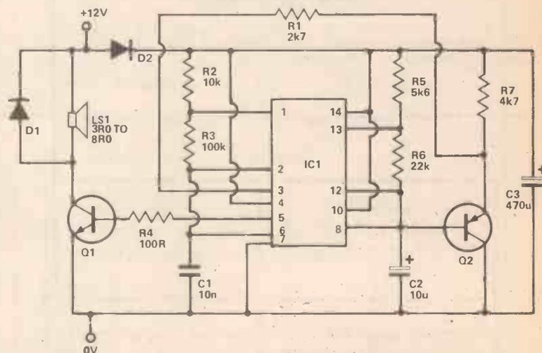
Fig. 4. Circuit diagram for the optional electronic siren.
