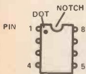
Figure 3. Showing an integrated circuit, viewed from above (with pins pointing away).
