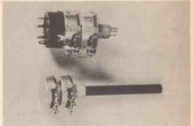
*Ganged pots, the two separate pots are joined together by a single shaft, most often seen in stereo systems.*
