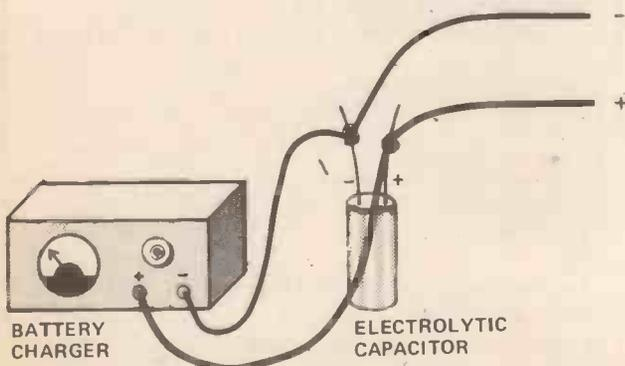
Fig. 9. Adding smoothing to a battery charger — a cheap way to get a single voltage supply suitable for many circuits.
