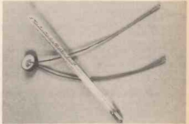
A thermistor, this style will be mostly found in circuits where a degree of thermal protection is required, note the size next to a medical thermometer.
