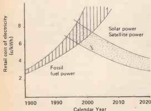
**Fig. 1.** The graph at left shows how the cost of electricity generated from the burning of fossil fuels (coal, oil) will increase over the next two decades. The cost of solar power derived from the proposed satellites is likely to become an economic alternative within 15 years.
