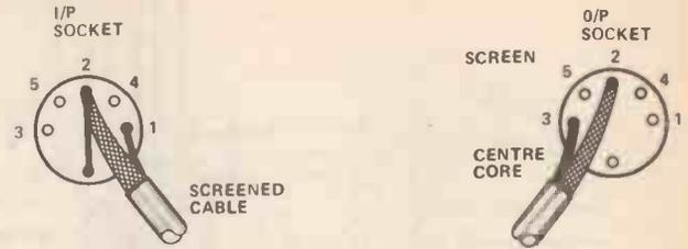
Figure 4. The connections to the input and output sockets.
