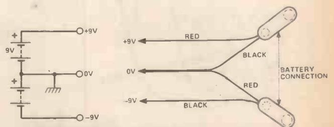
Fig. 8. Using two batteries for a power supply.
