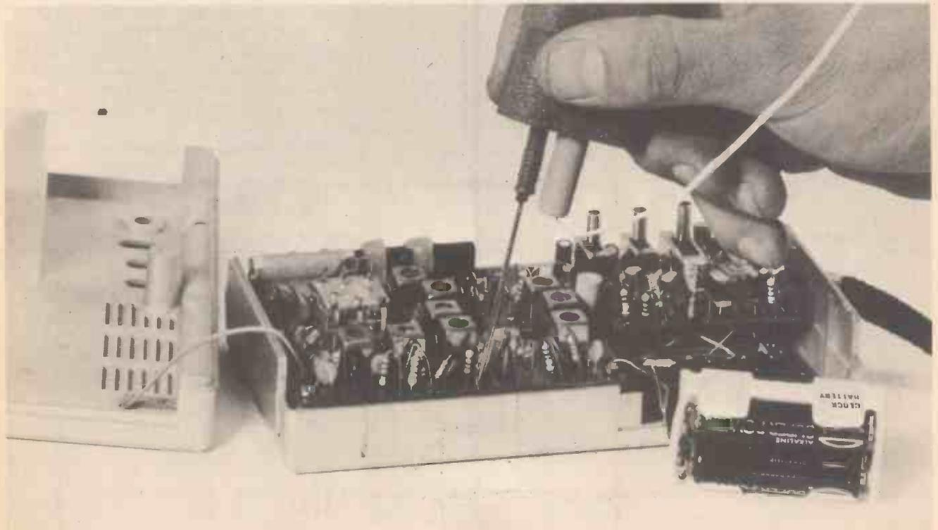
start fault-finding by injecting a signal at the slider of the volume control. If the resulting 1 kHz signal is heard in the set's speaker you'll know that the audio amplifier is OK, and the fault therefore lays further back, in the IF or RF sections of the receiver. If the signal is not heard, you'll know that the audio amplifier is defective. By systematically working either forwards or backwards through the circuit, injecting or tracing as appropriate, the fault area can be easily located.
