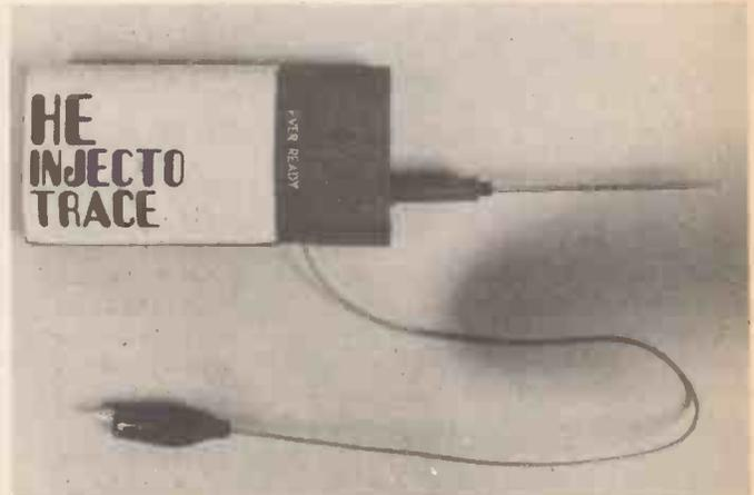
*The HE Injecto Trace in its torch case, note the flying lead and crocodile clip.*
