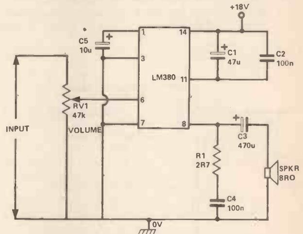
Fig. 4. A the LM380 connected as an inverting 2-watt audio amplifier with volume control and ripple rejection.
