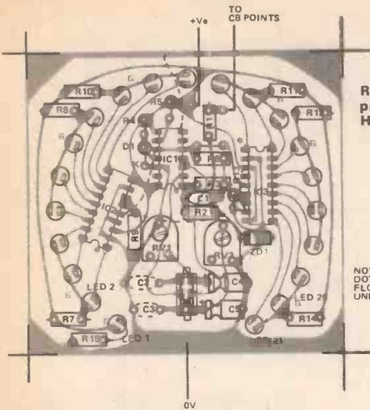
Right, PCB foil pattern for the HE tachometer.
