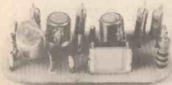
Close up of the circuit board, you can see how important it is to keep the component leads short.
