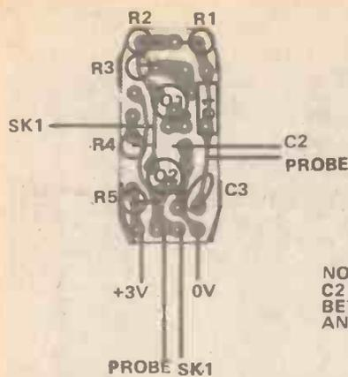
Fig. 2. Component overlay for the Injecto-Trace, keep the leads as short as possible to ensure everything fits in.
