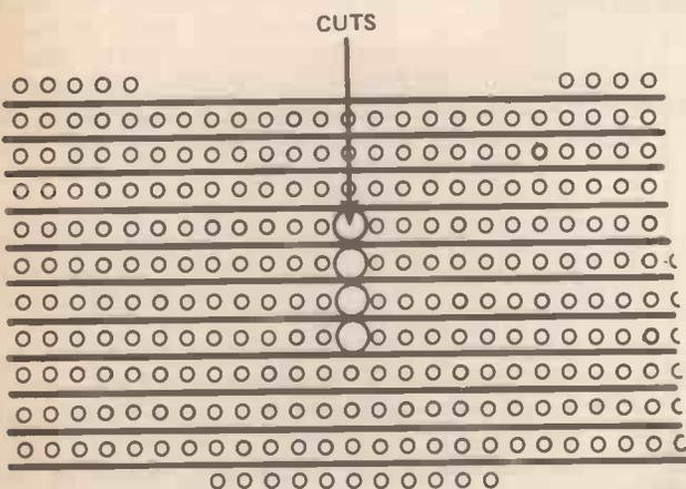
Fig. 6. Cutting 2.5 mm Veroboard to take an 8-pin IC.
