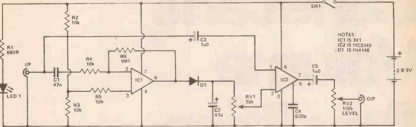
Figure 2. Circuit diagram of the HE Constant Volume Amplifier.
