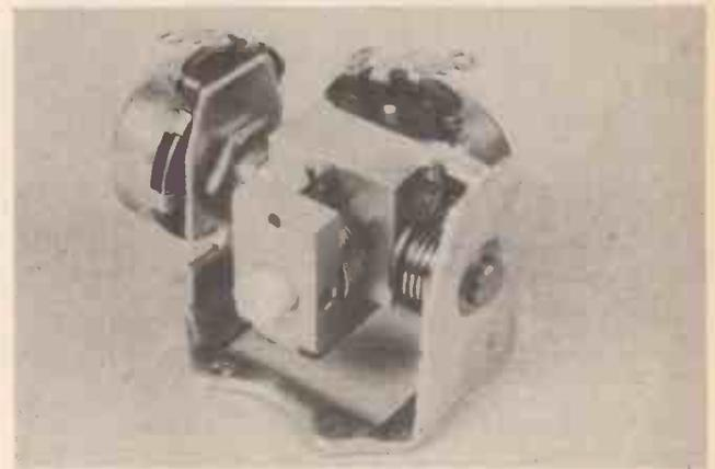
*An unusual application for pots, this is a joystick (found in radio control systems, synthesisers etc) the mechanical linkage will allow both pots to move in an X Y axis.*
