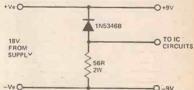
Fig. 10. Obtaining dual supplies from a single 18 V supply. The 1N5346B is a 9.1 V zener diode rated at 5 W and obtainable from RS Components stockists.
