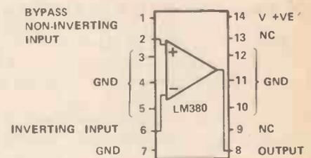
Fig. 2. Outline and pin connections of the standard 14 pin Dual-in-line (DIL) version of the LM380.
