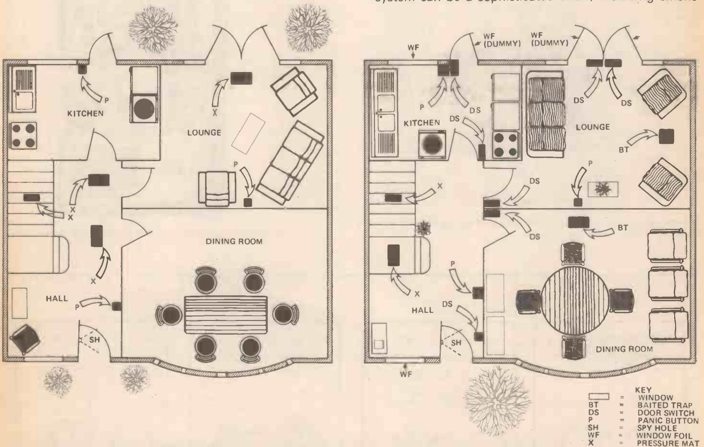
Fig 1. Ground-floor plans of a medium-sized mid-terrace house with two alternative security defence systems.
