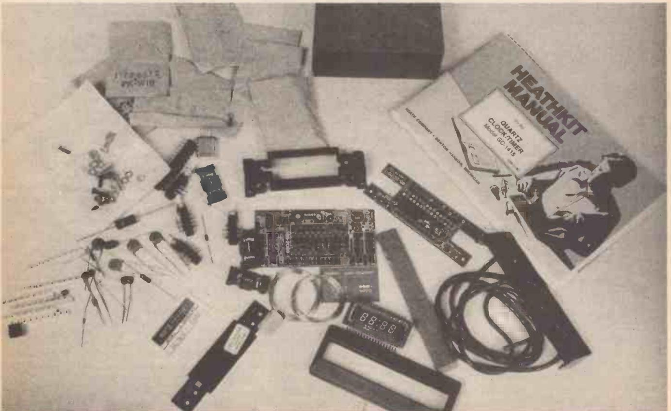
care should be taken when inserting the ICs. The rest of the parts consisted of a handful of resistors, a couple of capacitors, one transistor, six diodes, a crystal and four push button switches. On the display board two spring metal switches need to be soldered to the board, the contact plates were so small they nearly disappeared down one of the holes without trace.
