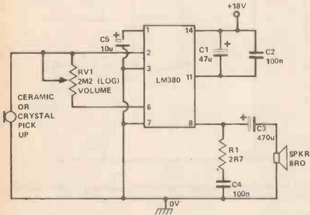
Fig. 6. A 2-watt audio amplifier with 'common mode' volume control.
