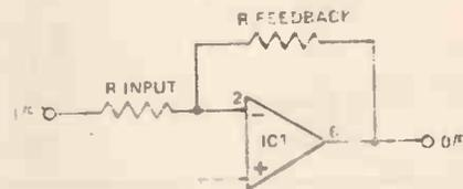
Figure 6. A straightforward operational amplifier circuit.
