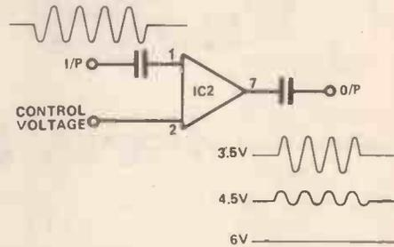
Figure 5. Showing the outputs obtained with various control voltages.
