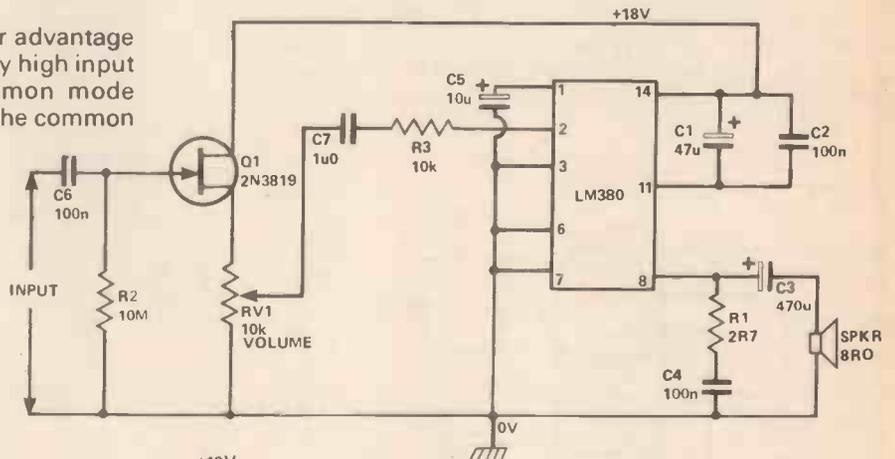
Fig 9. Above: A general purpose 2-watt audio amplifier with an input impedance of 10 Meg ohms.
