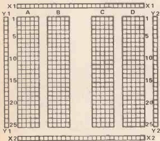
**Fig. 1.** The Eurobreadboard layout. Columns AB or CD are used for small ICs, the larger spacings between B and C can be used for the bigger ICs with 15 mm between lines.
