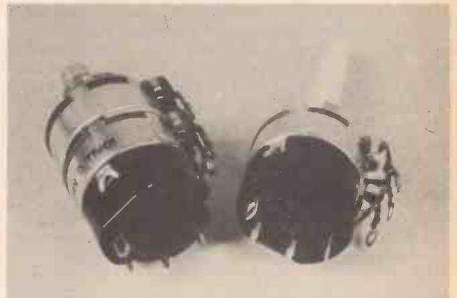
*Pots with switches, the switch mechanism is connected to the shaft assembly.*
