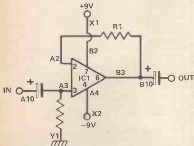
Fig. 3. Instant circuit! When the Eurobreadboard numbers are put on to the circuit, the few extra components that are needed go between these lines and earth or supply lines, or can be accommodated on spare lines.
