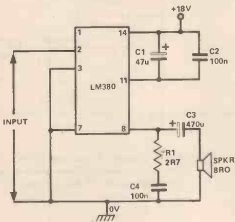
Fig. 3. A simple Non-Inverting 2 watt audio amplifier.
