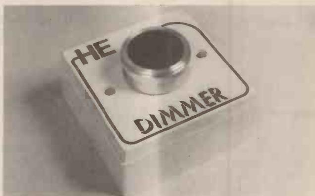
*The HE Dimmer in its wall mounting box. For safety we recommend using a plastic, flush mounting box.*
