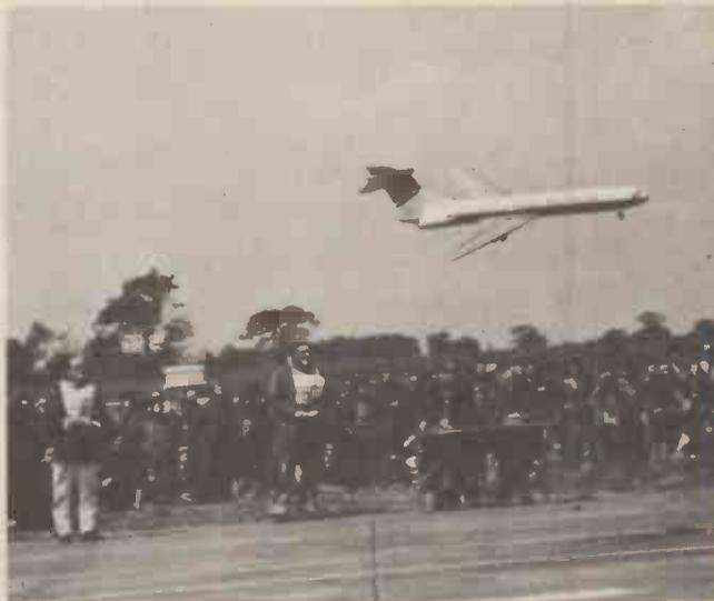
*A semi-scale VC10 being demonstrated during a model airshow at Woodvale, Lancs. This model is powered by two internal combustion engines in place of the four gas turbines of the original.*
