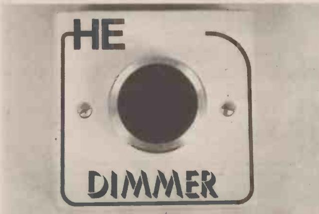
Front panel of the dimmer, experience has shown that a large knob is easier to adjust.
