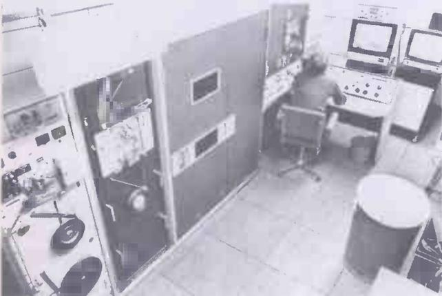
*Telecine equipment used to convert movie film into an electronic image, it is nothing more than a conventional movie projector coupled up to a colour camera.*
