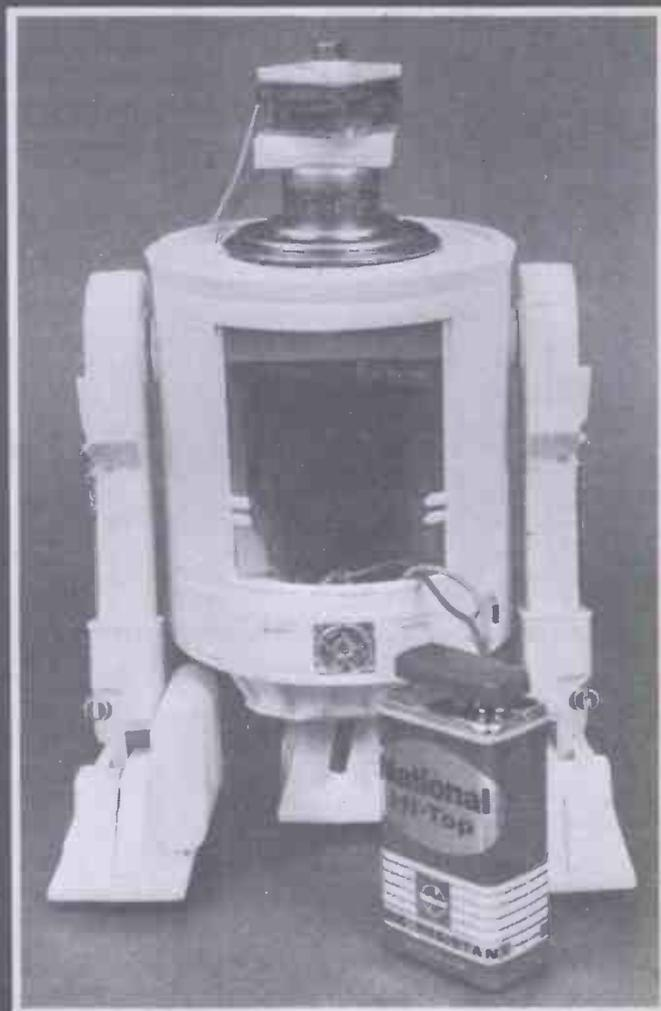
Open for inspection. Note the tuning capacitor mounted above the loudspeaker and the power switch mounted on the base.
