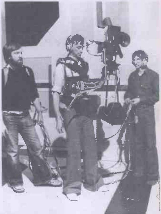
*This rather unwieldy looking piece of apparatus is called a 'Steadicam' camera steadying device with a lightweight electronic camera attached.*
