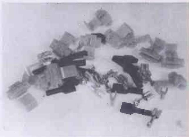
*The mass of connectors supplied with the kit. The connectors at the top of the photograph are the type that can 'patch' into a wire without actually breaking the inner conductor, very useful in this kind of installation.*
