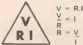
Fig. 6.1 The ancient and extremely useful method of remembering Ohm's law.
