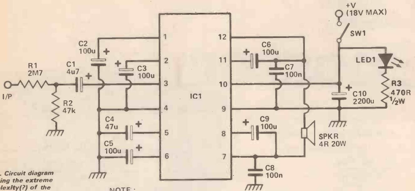
Fig. 1. Circuit diagram showing the extreme complexity(?) of the HE Car Booster — one channel.
