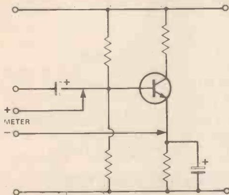
**Fig. 6.6** Measuring the voltage between base and emitter. A meter with a good "figure of merit" is needed for this measurement.
