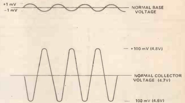
Fig. 6.8 The action of the amplifier. The wave at the output of the amplifier is an enlarged copy of the wave at the input.
