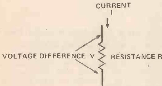
Fig. 6.2 A voltage difference caused by a current flowing through a resistor.
