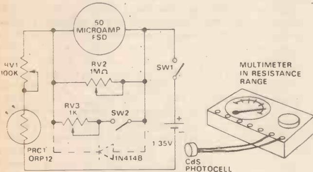
Fig. 4. Circuit diagram of a basic hand-held CdS lightmeter. This version has two ranges which are individually calibrated by RV2 and RV3.
