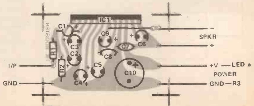
Fig. 2. PCB overlay.
