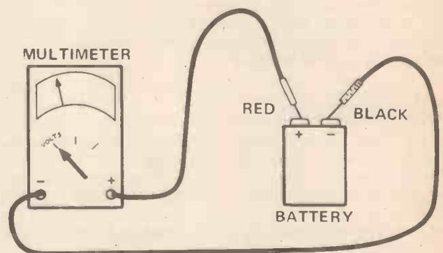
Fig. 6.3 Measuring a battery voltage. The meter must be set to a VOLTAGE range high enough to cope with the battery voltage.
