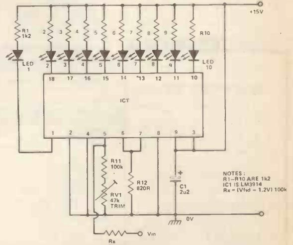
Fig. 4. Circuit diagram of the LED bargraph indicator
