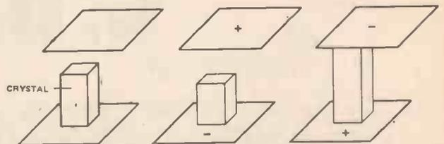
Fig. 2. The drawing's an exaggeration, of course, but it shows the idea. Piezo-electric crystals become shorter in one direction of electric field and longer when the field is reversed.
