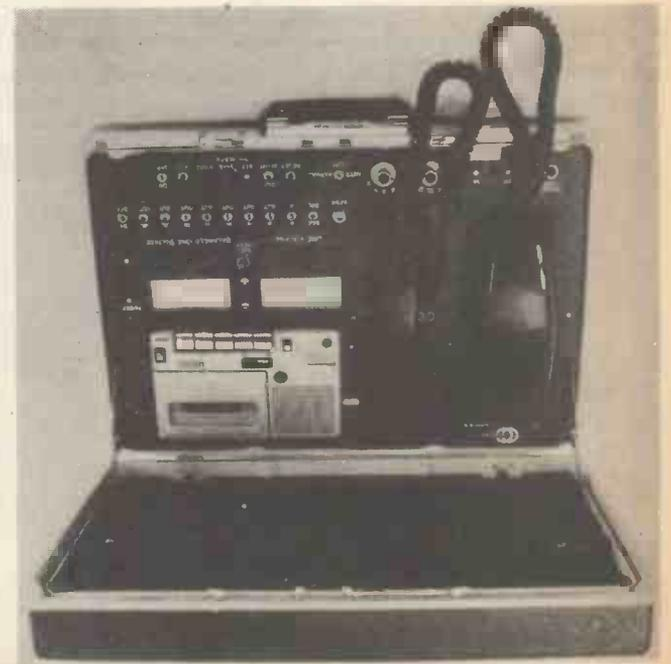
*A complete anti bug system. The suitcase contains a tap detector, a tap defater, telephone monitor and scrambler.*
