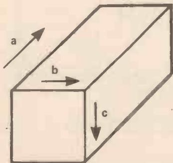
1. An isotropic crystal gives the same readings for quantities like expansivity, resistivity, etc., in any direction along the crystal, a, b, or c.
