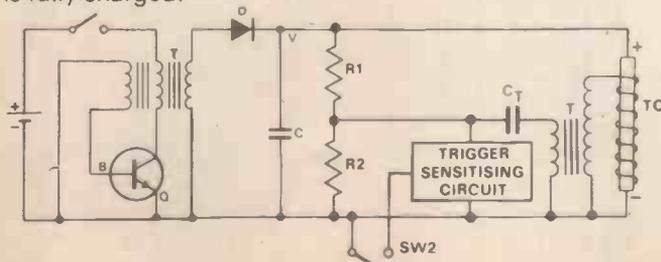
Fig 10. Basic diagram of a manual flashgun.
