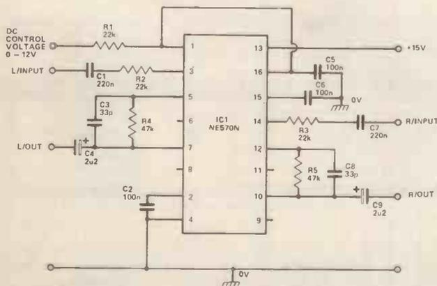
Fig. 3. Circuit diagram of the voltage-controlled stereo pot
