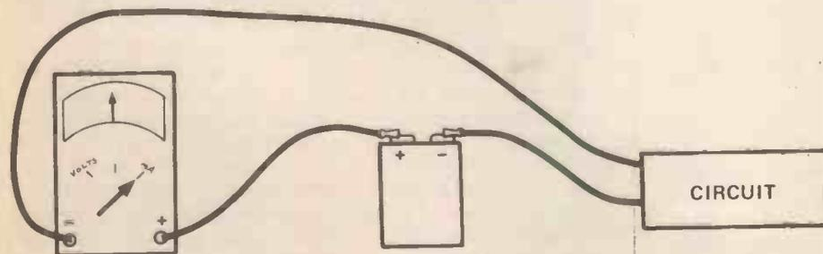
Fig. 6.5 Where to measure the collector voltage of a transistor. The meter must be switched to a voltage range as high as that used for measuring battery voltage.
