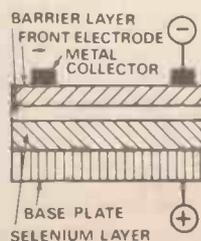
**Fig. 1. Structure of the selenium cell. This was used in the first commercial exposure meter and is still popular today.**
