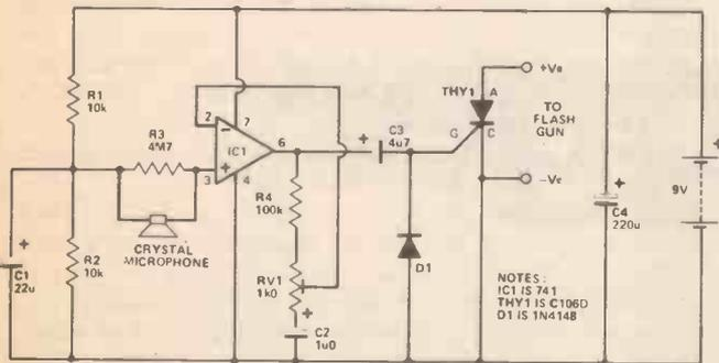
Fig. 1. The circuit diagram of the Flash Trigger.
