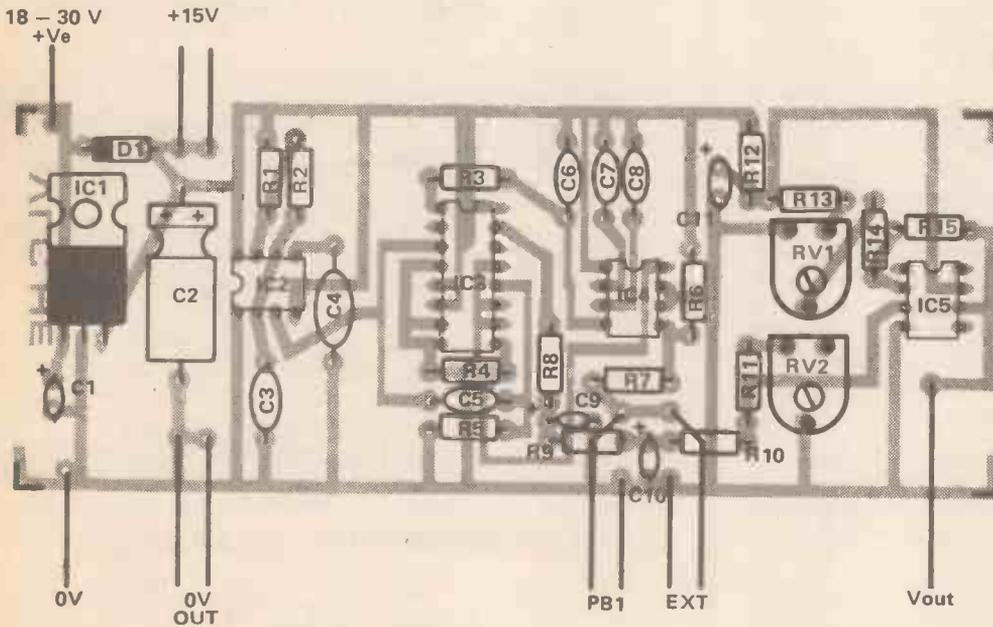
Above Component overlay for the voltage level controller board. Below: PCB design
