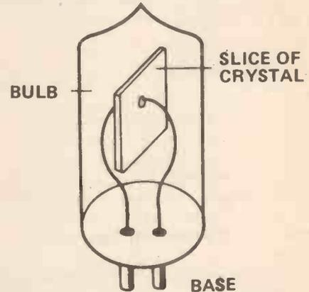
*Fig. 4. A quartz crystal inside an evacuated bulb. This is a type of mounting used for crystals that control radio transmitter frequencies.*
