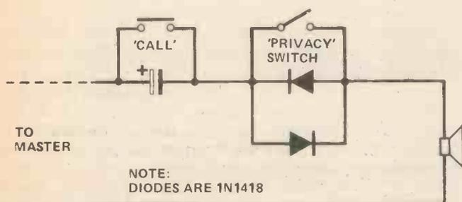
The diodes (1N1418) allow the call tone or voices from the main station to be heard but the minute voltages from the sub-station speaker are not enough to turn the diodes on.
