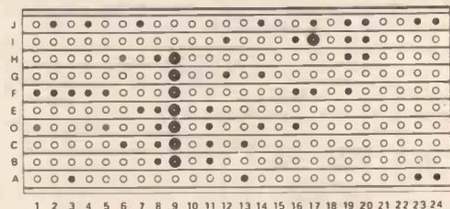
Fig. 3. The underside of the board. The large circles show where to cut the tracks, the dots are soldering points for the component leads.
