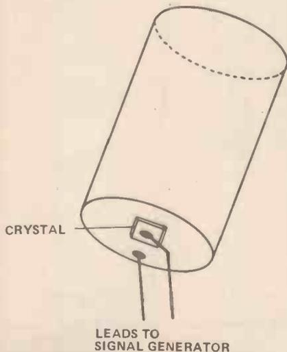
*Fig. 3. An ultrasonic cleaner. The metal beaker has a piezoelectric crystal soldered to the base. Leads to the beaker and to a contact on the face of the crystal are fed with high frequency signals from a generator. The vibrations of the crystal cause the liquid in the beaker to vibrate.*
