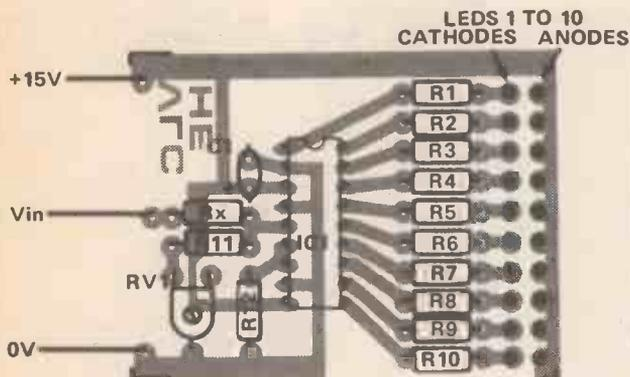
Above: Component overlay for the LED bargraph indicator board. Right: PCB design for the LED bargraph indicator. Below: Photo of the indicator board
