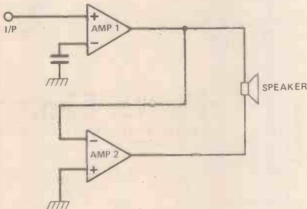
Fig. 3. Simplified internal circuitry of the HA 1388.
