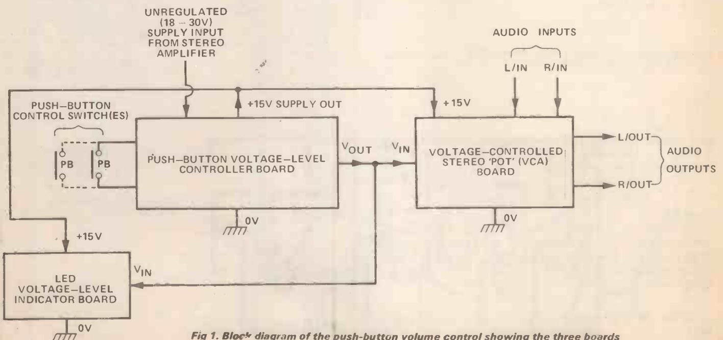
Fig 1. Block diagram of the push-button volume control showing the three boards
