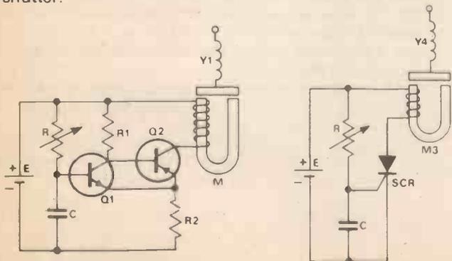
Figs. 8, 9. The Schmitt trigger and SCR timers.
