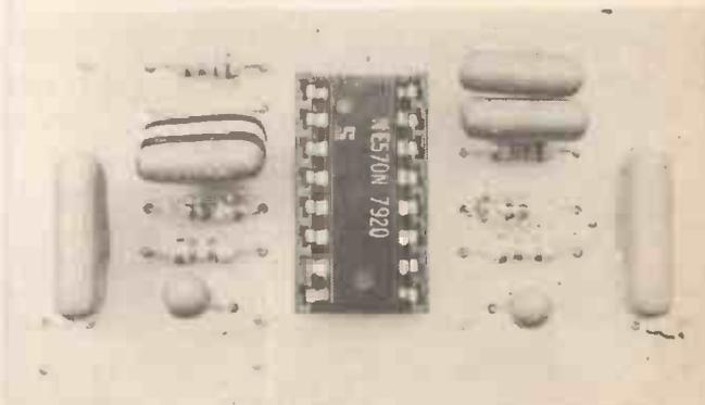
The voltage-controlled stereo pot board
