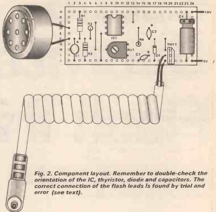
Fig. 2. Component layout. Remember to double-check the orientation of the IC, thyristor, diode and capacitors. The correct connection of the flash leads is found by trial and error (see text).
