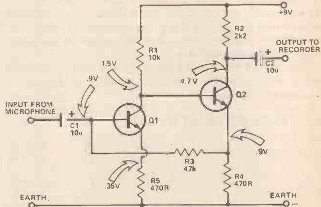
**Fig. 6.7** The amplifier circuit. The figures in circles are the "design voltages" for the circuit; actual readings should not be too greatly different.
