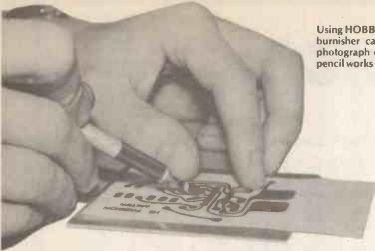
Using HOBBYPRINTS as a resist. A burnisher can be used as in the photograph or alternatively a soft pencil works equally as well.
