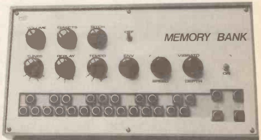
Figure 5. Showing front panel layout and lettering. Note the hole which needs to be cut out for the keyboard push buttons
