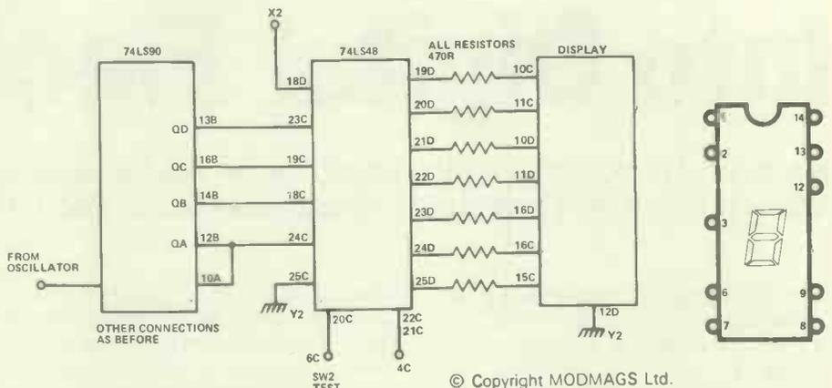
Figure 5.5 Counter-decoder-display circuit. Connections to the 74LS90 counter are the same as they were in Fig. 5.3, but the outputs Qa to Qd are connected to the decoder inputs, and the decoder outputs are connected through 470R resistors to the display
