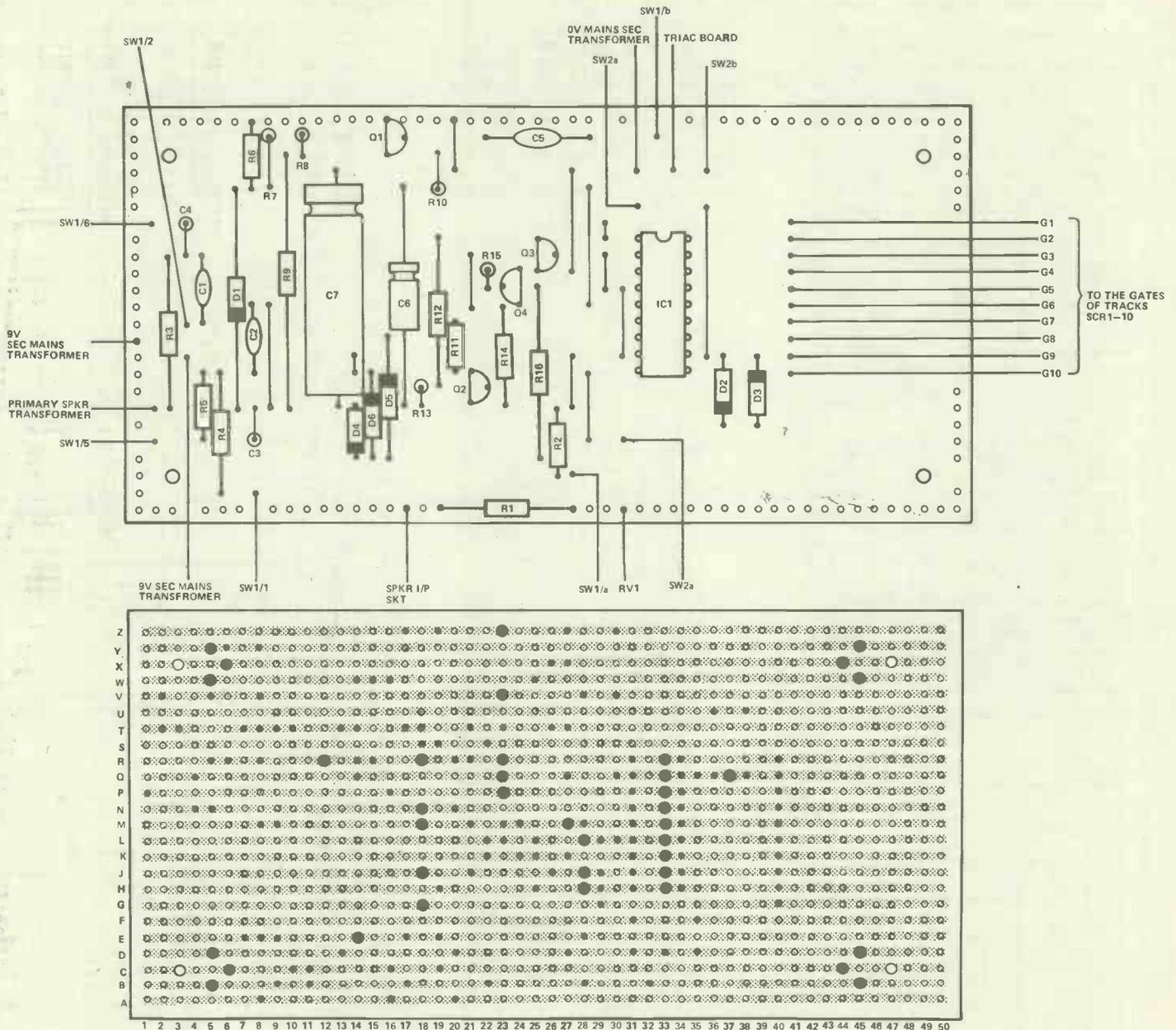
Figure 5. Veroboard layout and underside view showing track breaks
