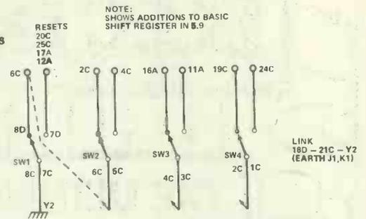
Figure 5.14 The SIPO register connections. Once more, this shows the additions to the circuit in Fig. 5.9, with previous additions removed. This also restores the switches to normal operation for the next set of operations to be described next month
