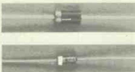
Figure 2. A 1N4001 diode (above) and a 1N4148 diode
