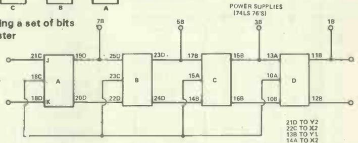
Figure 5.9 Basic shift register layout. The display and the 74LS48 have been removed from the board, and the 74LS76s replaced, wired as shown. The next series of diagrams will consist of additions to this basic scheme
