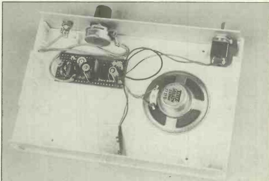
case also helps to avoid stray pick up of mains hum, etc, but a plastic one like we used is satisfactory for most purposes. The input leads and speaker leads should be kept reasonably well separated so that stray feedback is avoided.
