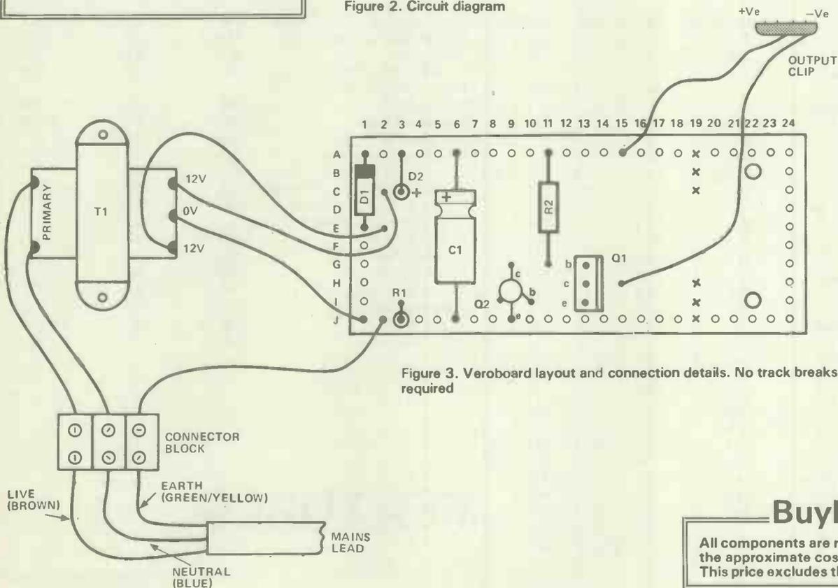
Figure 3. Veroboard layout and connection details. No track breaks are required
