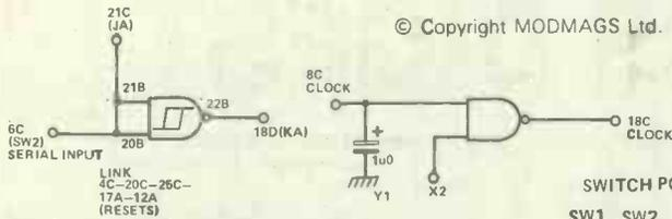
Figure 5.10 The additions to the basic shift register circuit for implementing a SISO register
