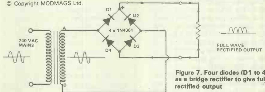
**Figure 7. Four diodes (D1 to 4) used as a bridge rectifier to give full-wave rectified output**
