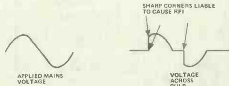
Figure 4. Input and output voltages to an ordinary triac power controller
