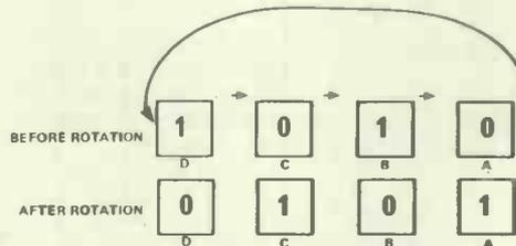
Figure 5.8 Rotating a set of bits with a shift register
