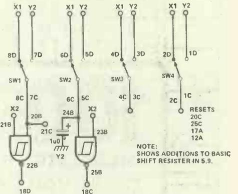
Figure 5.14 The SIPO register connections. Once more, this shows the additions to the circuit in Fig. 5.9, with previous additions removed. This also restores the switches to normal operation for the next set of operations to be described next month
