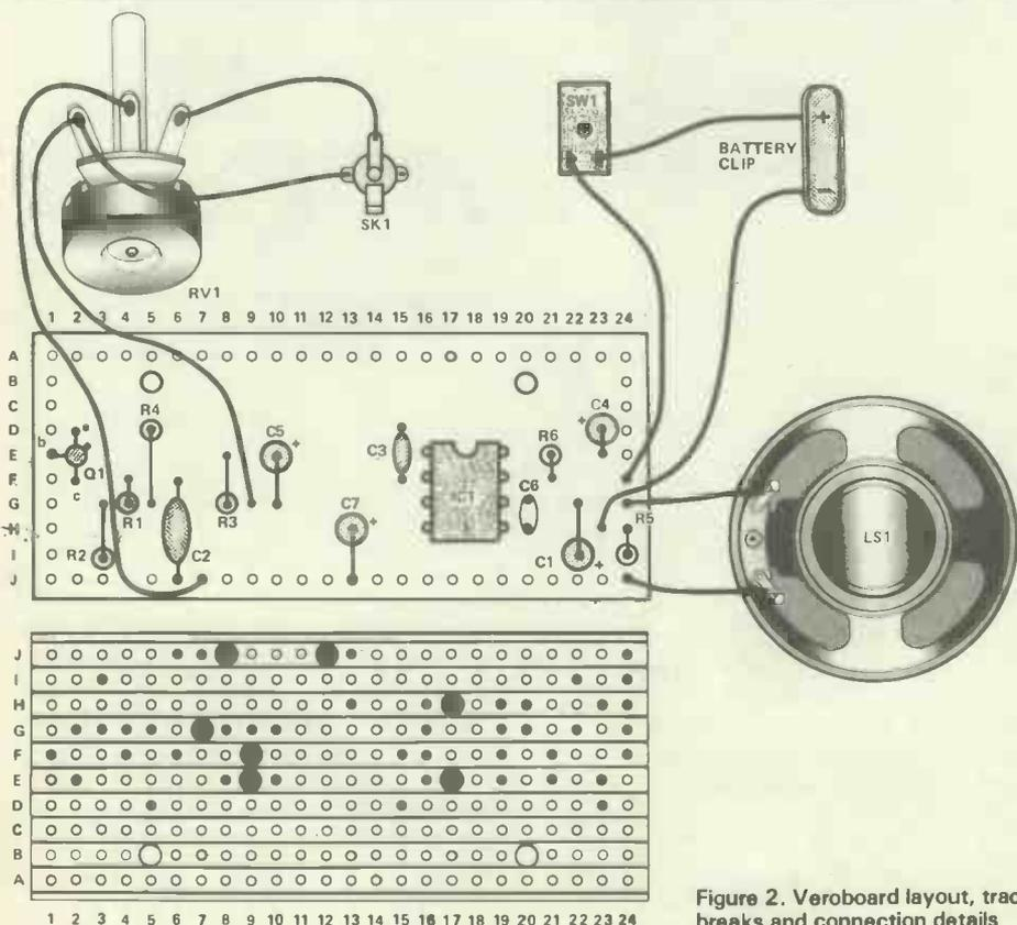
Figure 2. Veroboard layout, track breaks and connection details
