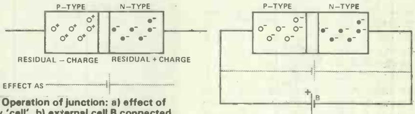
**Figure 4. Operation of junction:** a) effect of imaginary 'cell', b) external cell B connected to p-n junction in 'forward bias'. The imaginary cell appears to be connected to assist current flow
