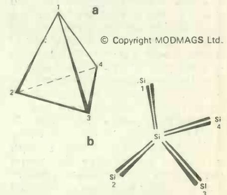
Figure 2. Semiconductor crystal: a) 'diamond' structure (pyramid-like) form in which silicon and germanium crystallise, b) central silicon is bonded to four others, one at each apex of the pyramid
