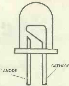
Figure 5. By holding the LED up to a bright light the junction can be seen
