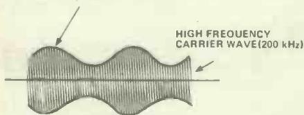
Figure 9. Amplitude modulation of a radio-frequency carrier wave
