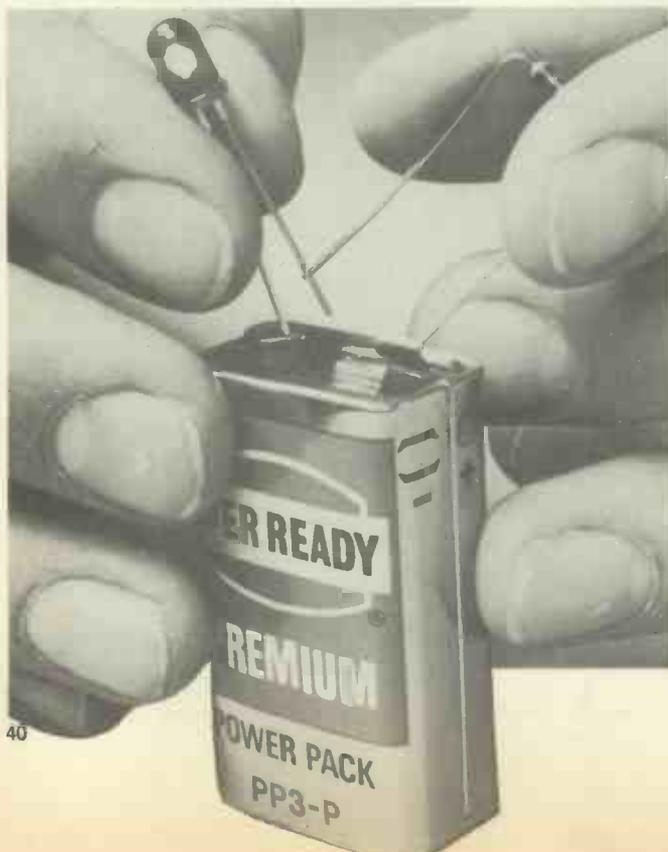
Figure 6. By holding a LED, resistor and battery in series you can find out which lead is which
