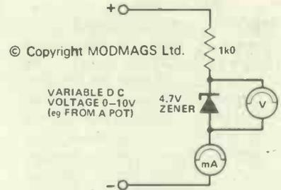
Figure 12. Circuit to demonstrate action of a zener diode
