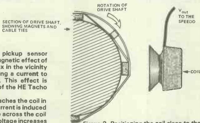
Figure 2. Positioning the coil close to the drive shaft results in the waveforms below
