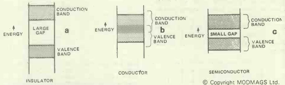
Figure 1. Conduction bands for a) insulators (well separated), b) metal (very close) and c) semiconductors (small gap)
