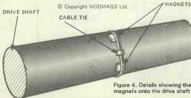
Figure 4. Details showing the positioning of magnets onto the drive shaft
