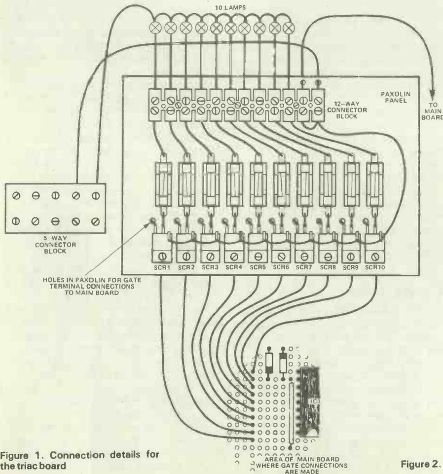
Figure 1. Connection details for the triac board
