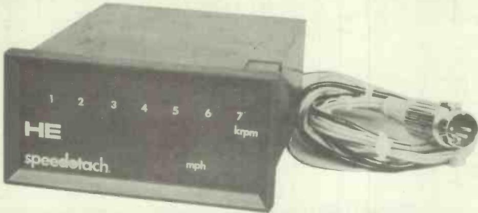
Yet another application of the now famous LM3914 dot/bar voltmeter chip — this tachometer project is designed to complement our Digital Speedo in both style and size — fit them both into the same case or use them individually.
