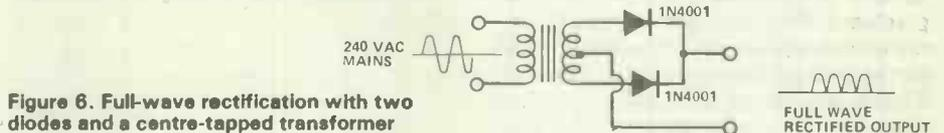
**Figure 6. Full-wave rectification with two diodes and a centre-tapped transformer**
