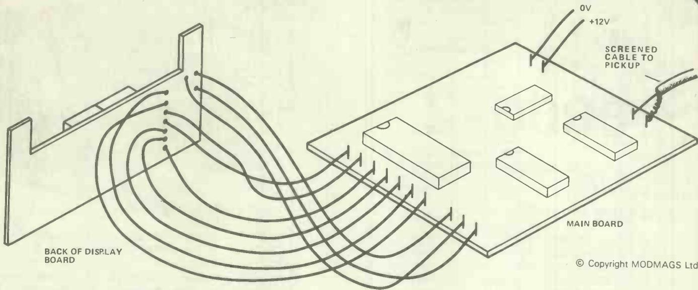
Figure 1. Connection details of the two boards of the Speedo
