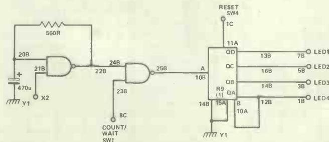
Figure 5.3 A clock-pulse oscillator driving the decade counter through a gate. The outputs of the counter are taken to LEDs
