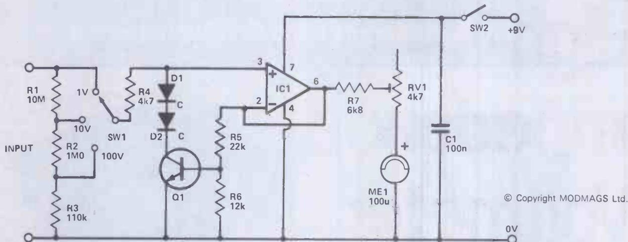
Figure 1. Circuit diagram of the High-Impedance Voltmeter
