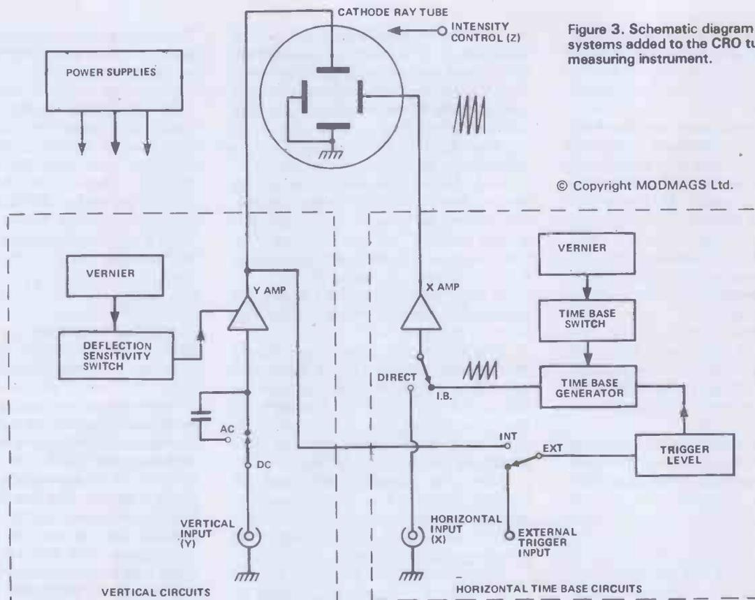
Figure 3. Schematic diagram of essential sub-systems added to the CRO tube to make it a measuring instrument.
