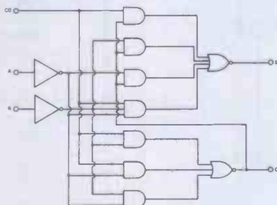
Figure 6.4 Circuitry for a full adder. Inputs are the bits to be added, plus a carry from the previous stage; outputs are the usual sum and carry bits
