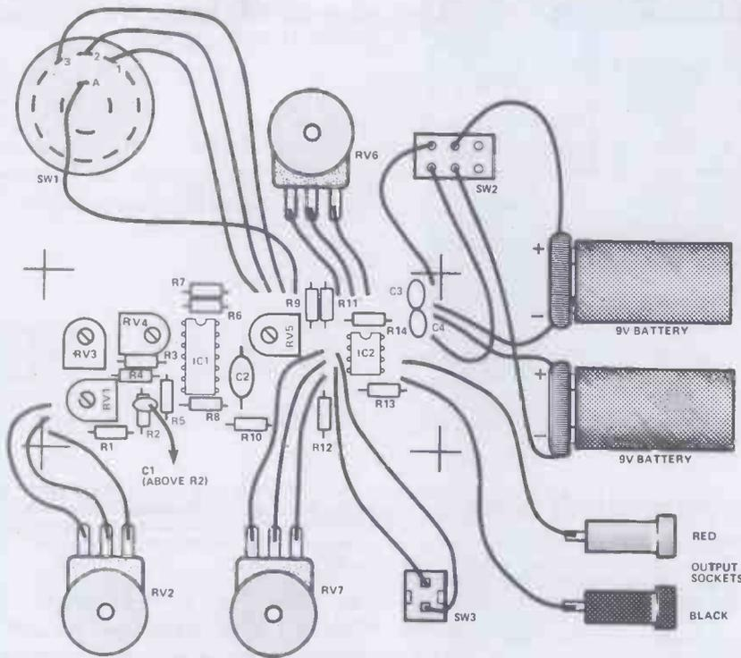
Figure 2. Overlay of the PCB and connection details of the Audio Signal Generator.
