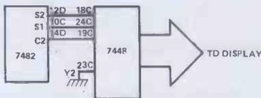
Figure 6.7 Connecting the adder outputs to the 74LS48 decoder so that results can be displayed in denary if wanted. The D input of the decoder must be earthed
