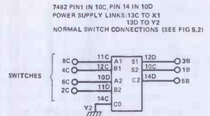
Figure 6.6 Using the 74LS82 full-adder. The switches provide the inputs, and the LEDs provide the outputs. The 74LS132 can be removed if desired
