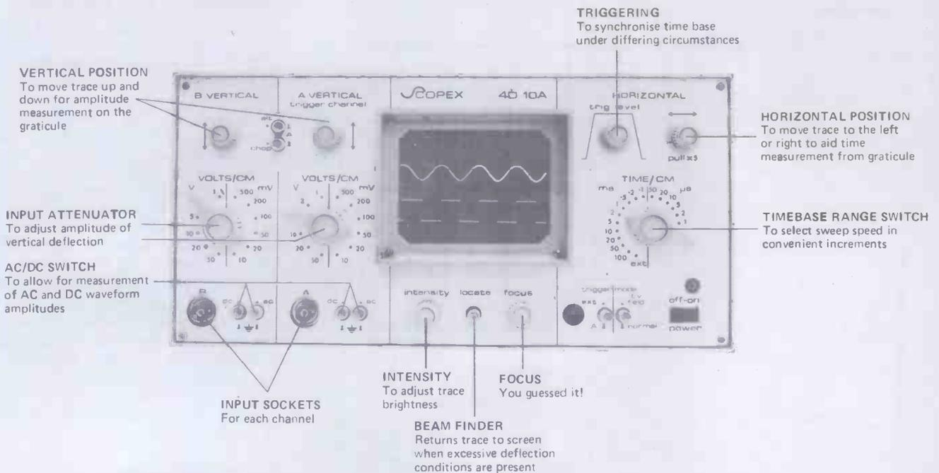
A typical oscilloscope front panel layout, showing the positions of the major controls.
