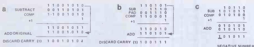
Figure 6.12 Two's complement subtraction. The number to be subtracted is put into two's complement form, equivalent to placing a negative sign in front. The numbers are then added, and the carry is discarded
