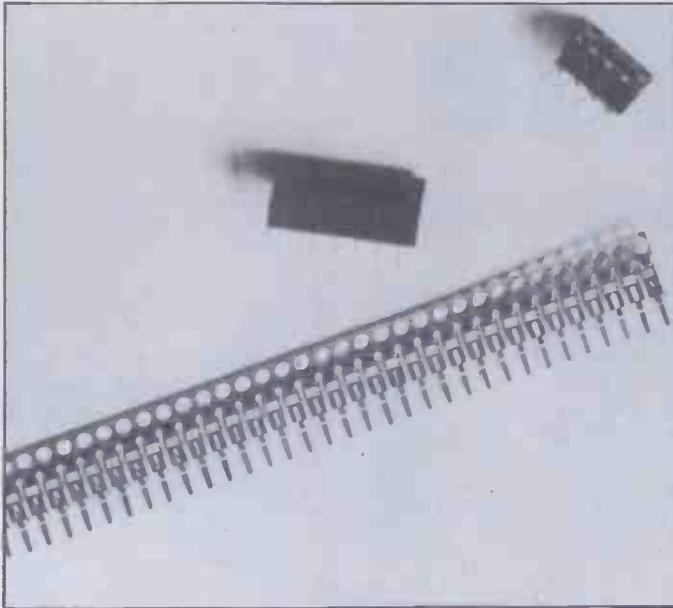
Figure 4. Typical sizes and types of IC sockets including the 'do-it-yourself' kind.
