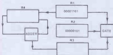
Figure 6.15 An arrangement of registers which could be used to multiply two numbers, provided that the correct sequence of control pulses could be obtained
