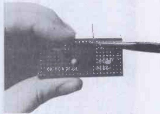
Figure 2. Making a link exactly the right size for the circuit board.
