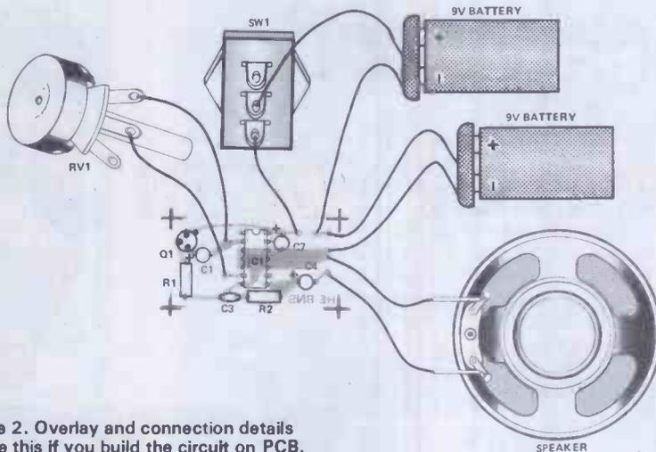
Figure 2. Overlay and connection details — use this if you build the circuit on PCB.
