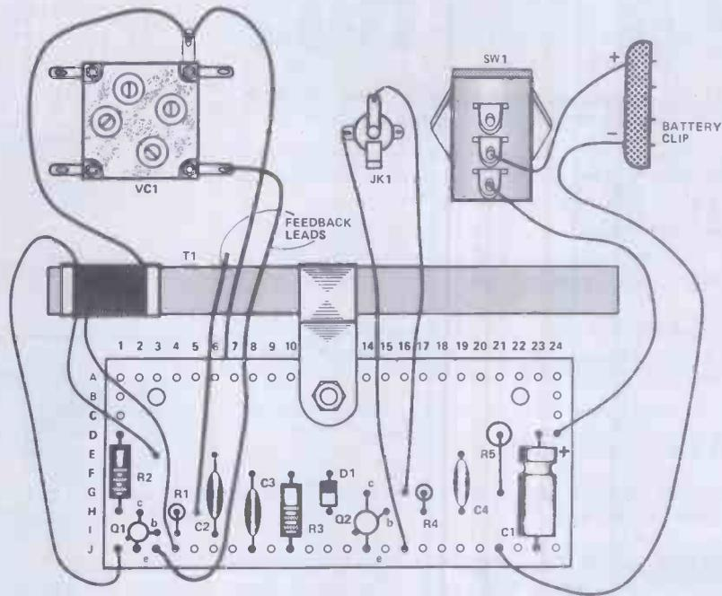
Figure 2. Connection details of the project along with Veroboard overlay and underside track break.
