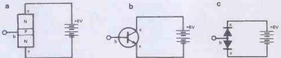
Figure 2. Transistor connected unhelpfully to a 6 V battery: a) the device, b) the circuit symbol, c) showing it to be equivalent to two pn-junction diodes
