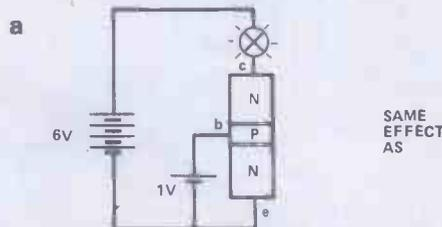
Figure 4. a) how we would theoretically get a transistor to conduct by forward-biasing the emitter-base junction, b) how it is usually achieved in practice (note arrows indicate electron flow)
