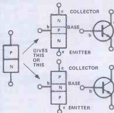
Figure 1. Three-layer device is either a pnp or npn transistor (with corresponding circuit symbol)
