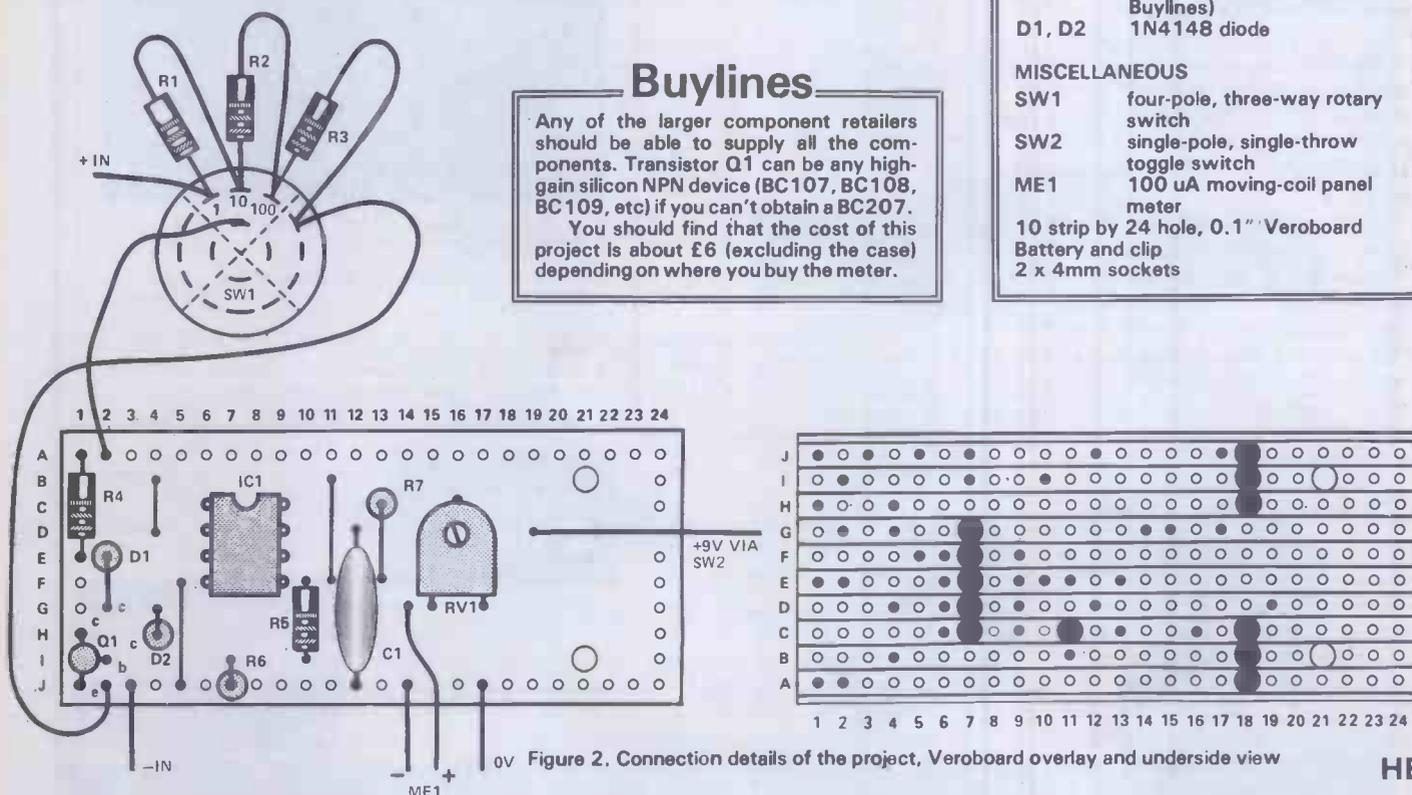
Figure 2. Connection details of the project, Veroboard overlay and underside view
