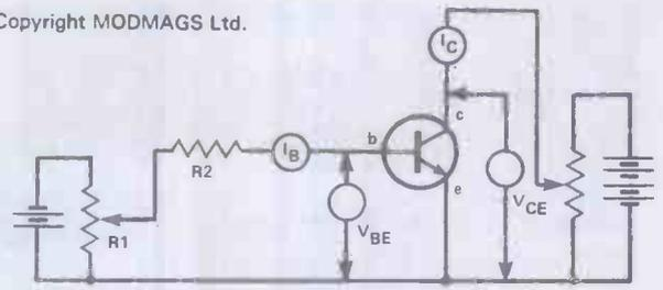
Figure 7. How to measure  $V_{BE}$  and  $V_{CE}$
