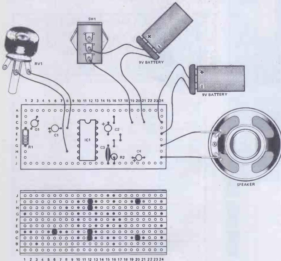
Figure 3. Veroboard layout and connections along with underside view.
