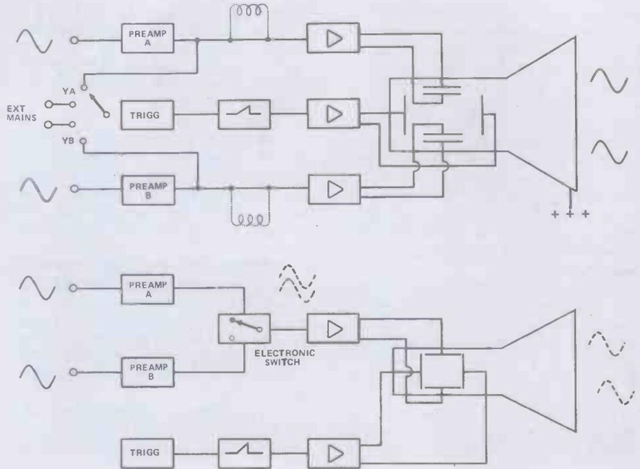
Figure 5. Dual-trace oscilloscopes can be implemented in two ways: using a dual beam cathode ray tube or using a single beam tube and electronic switching of the trace. The block diagram at the top is of a Philips model 3232 and is typical of dual-beam types. The block diagram at the bottom shows the electronic switching technique of obtaining dual-trace operation with a single beam cathode ray tube.
