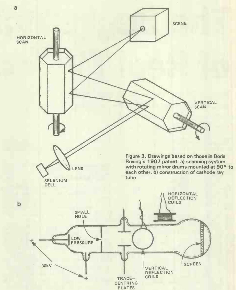
Figure 3. Drawings based on those in Boris Rosing's 1907 patent: a) scanning system with rotating mirror drums mounted at 90° to each other, b) construction of cathode ray tube
