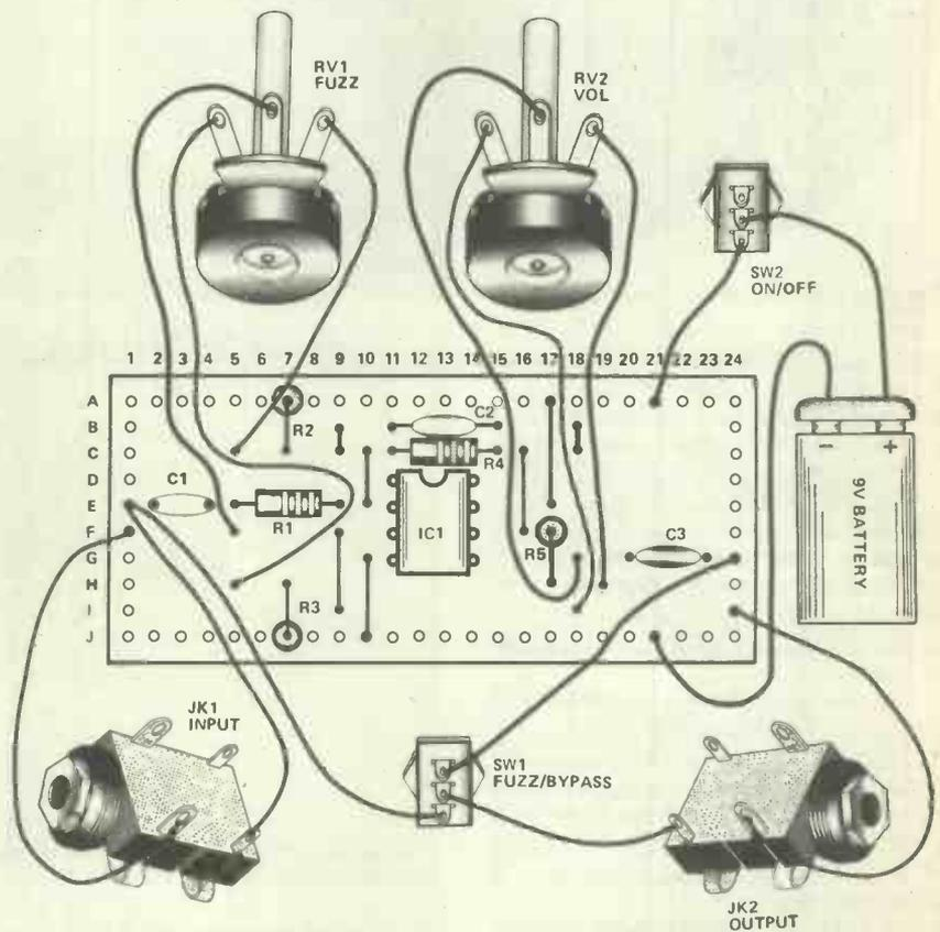
then capacitors and finally the IC as shown in Fig.2. Wiring up should be done as per connection details and then you can test your project. There is little to go wrong so providing your constructional skills are up to scratch the fuzz should work first time.
