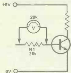
Figure 5. A voltmeter 'loading' the base resistor of a transistor
