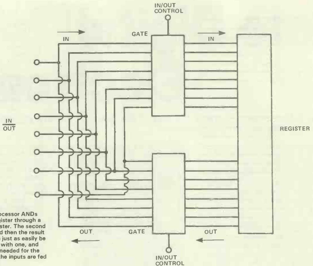
Figure 7.2 How the microprocessor ANDs bits. One bit is fed in to a register through a gate and is stored in the register. The second bit is then fed in, ANDed, and then the result is fed out. The operation can just as easily be performed with eight bits as with one, and only the eight input pins are needed for the inputs and output, because the inputs are fed in at different times
