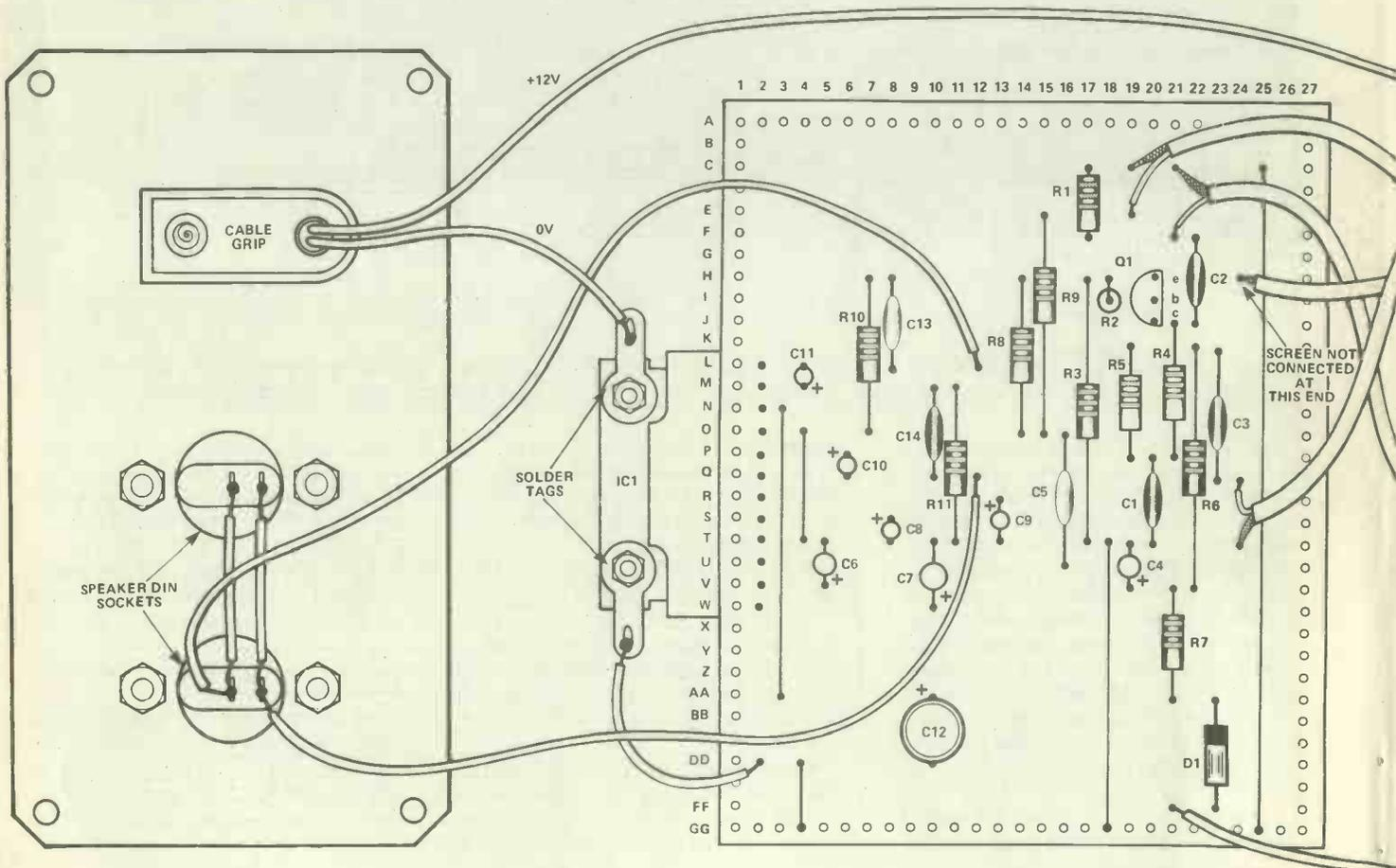
Note also that fairly heavy-gauge cable is necessary for the power and output connection because a lot of current will be flowing through them at times. Use of fine-gauge wire will result in loss of power and possible audible instability. Use sleeving, if you have any, to cover all soldered connections thus helping to prevent short circuits.
