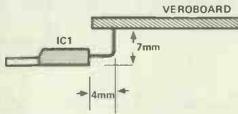
Figure 1. Correct mounting procedure for IC1, below the board.
