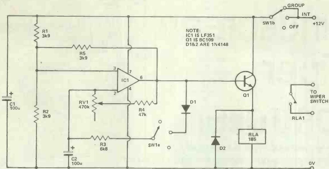
Figure 1. Circuit diagram of the HE Windscreen Wiper Controller
