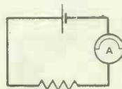
Figure 3. How an ammeter is connected into the circuit
