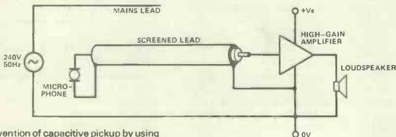
Figure 5. Prevention of capacitive pickup by using screened cable
