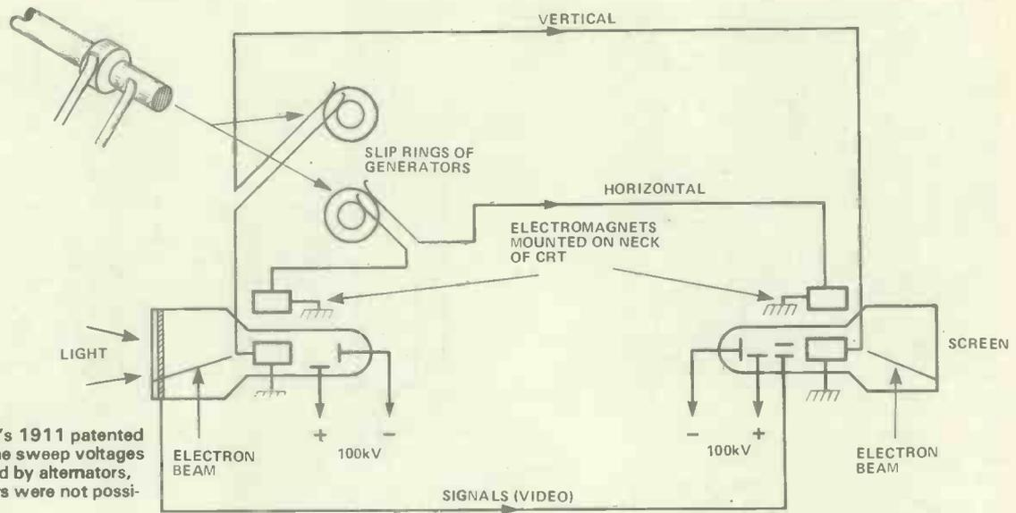
Figure 4. Campbell-Swinton's 1911 patented sketch in simplified form. The sweep voltages were to have been generated by alternators, because electronic oscillators were not possible at that time
