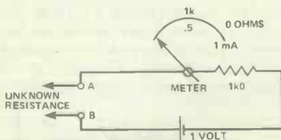
Figure 6. A design for a simple ohmmeter
