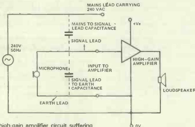
Figure 4. A high-gain amplifier circuit suffering from capacitive pickup
