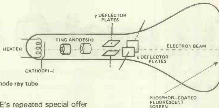
Figure 7. A cathode ray tube
