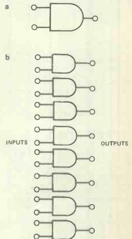
Figure 7.1 One operation — ANDing. A single AND gate (a) can AND two bits. To AND a set of eight bits (b) would need eight AND gates, with sixteen inputs and eight outputs
