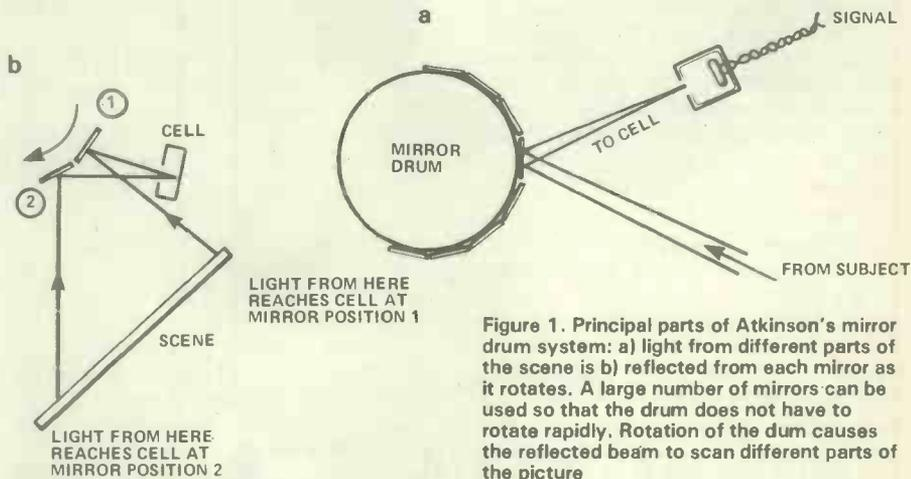
Figure 1. Principal parts of Atkinson's mirror drum system: a) light from different parts of the scene is b) reflected from each mirror as it rotates. A large number of mirrors can be used so that the drum does not have to rotate rapidly. Rotation of the drum causes the reflected beam to scan different parts of the picture
