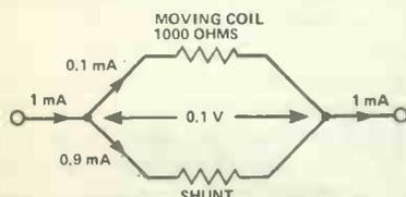
Figure 1. To convert a moving-coil meter into an ammeter, you connect a low-value resistance in parallel with it
