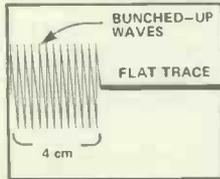
Figure 9. Using an oscilloscope to time how long a hammer was in contact with a metal rod
