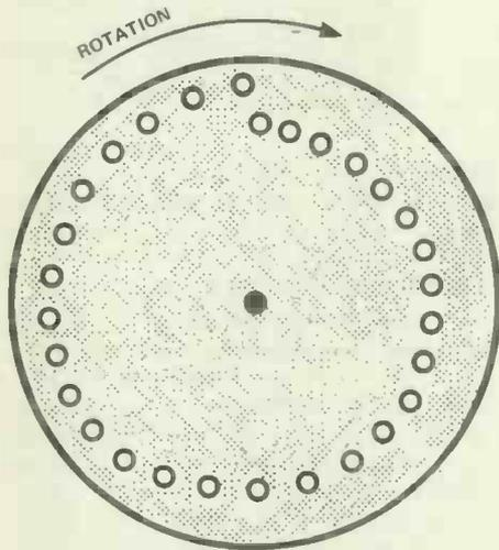
Figure 2. Nipkow disc, the scanning system used by most of the mechanical TV systems
