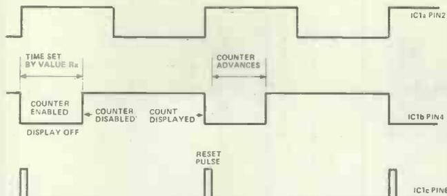
Figure 3. Waveforms within the circuit, not to scale
