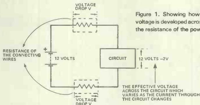
Figure 1. Showing how less than the original voltage is developed across the circuit because of the resistance of the power supply leads
