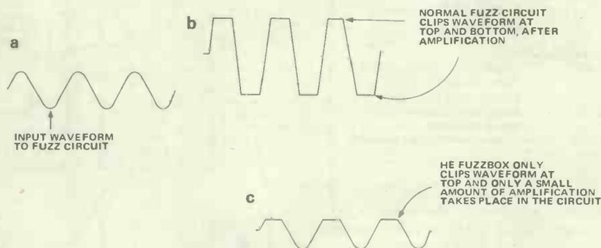
Figure 3. a) A possible input signal b) The output of a conventional fuzz circuit c) The output of the HE Fuzzbox
