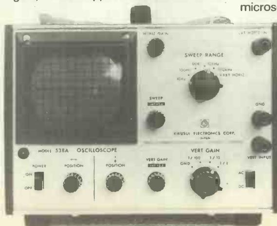
Figure 8. Front panel of an oscilloscope (Kikusui 538A) showing the various controls
