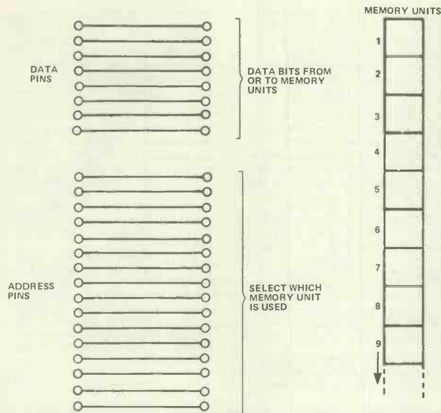
Figure 7.4 Using memory to ensure that instructions and data follow each other in the correct sequence. It is impossible to tell without knowing the sequence, whether a byte is an instruction or data
