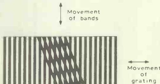
Left. Measurement of movement by optical means. Two gratings placed above one-another will produce interference patterns that can be used to determine movement
