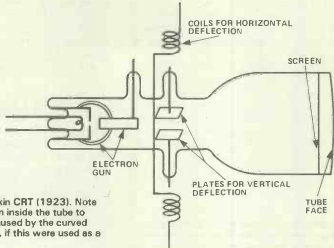
Figure 5. Early Zworykin CRT (1923). Note the use of a flat screen inside the tube to avoid the distortion caused by the curved outer face of the tube, if this were used as a screen
