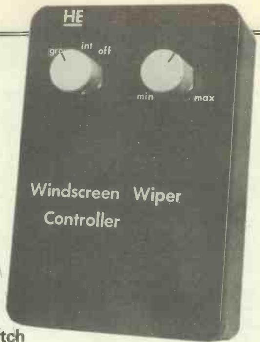
YES, ITS YET another design for a windscreen wiper controller, but in addition to giving single, intermittent wipes, this one can also be used to give several sweeps of the windscreen followed by a pause for a similar length of time. This second mode of operation can be very useful under certain conditions where single strokes of the wipers just tend to smear the screen, possibly even making things worse rather than better.
