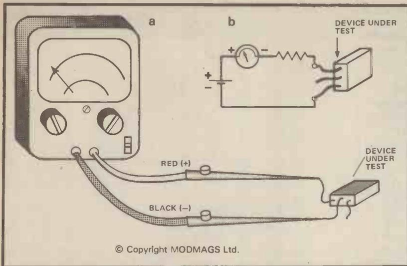
◀ Figure 4. Measuring resistance with a) a multimeter (note polarity of leads), and b) a battery, meter and resistor (see text for details)
