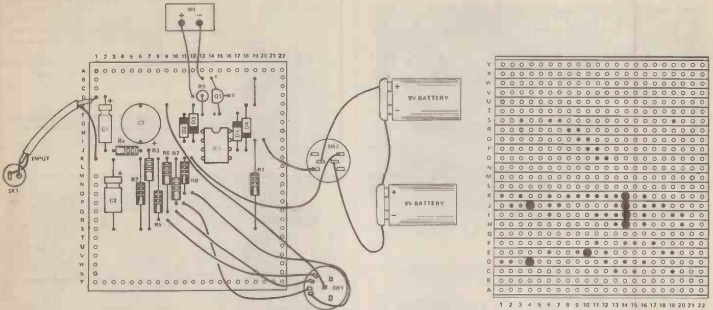
Figure 2. Veroboard layout of the project, showing component positions, track breaks underneath the board and connection details. Make sure you use screened cable for the input lead
