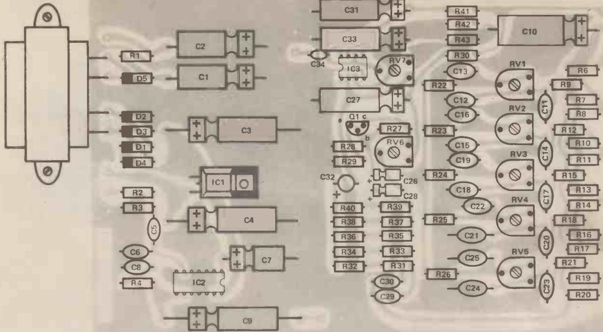
Figure 3. Overlay of Board 1
