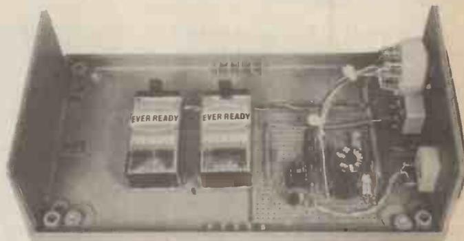
Internal photograph of the Audio Millivoltmeter
