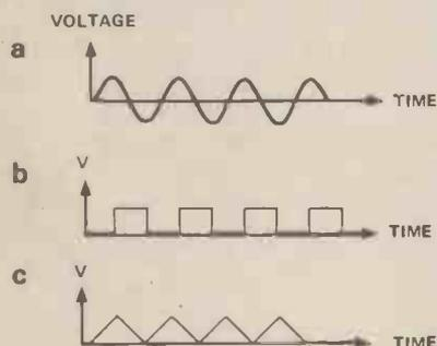
Figure 6. A variety of oscillator waveforms: a) sinewave, b) squarewave, c) sawtooth
