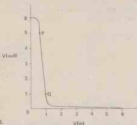
Figure 4. A plot of  $V$  (out) against  $V$  (in). This can be called the transfer characteristic
