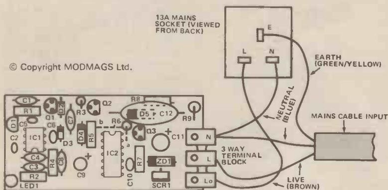
Figure 2. Overlay and connection details
