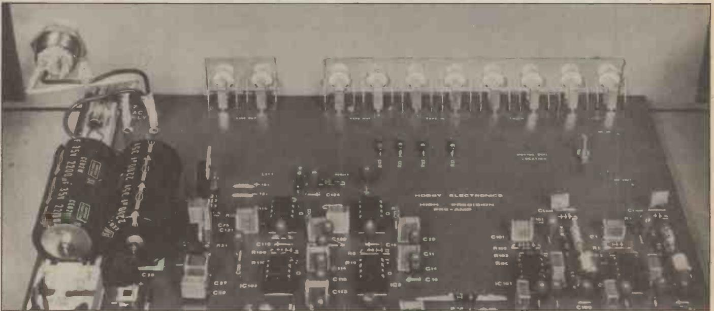
Figure 3. Internal photograph of the Pre-amplifier showing power supply connection details
