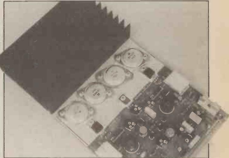
Figure 5. When more than one semiconductor is fastened to a heatsink as above, they must be electrically isolated
