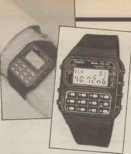
used to after being more familiar with conventional hand-held calculators. The 'clear display' button is sited on one edge while the +, x, - and = buttons are along the opposite edge.
