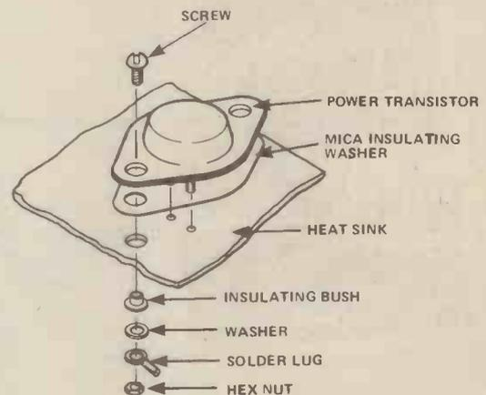
Figure 6. Use a mica washer to electrically insulate the semiconductor from the heatsink
