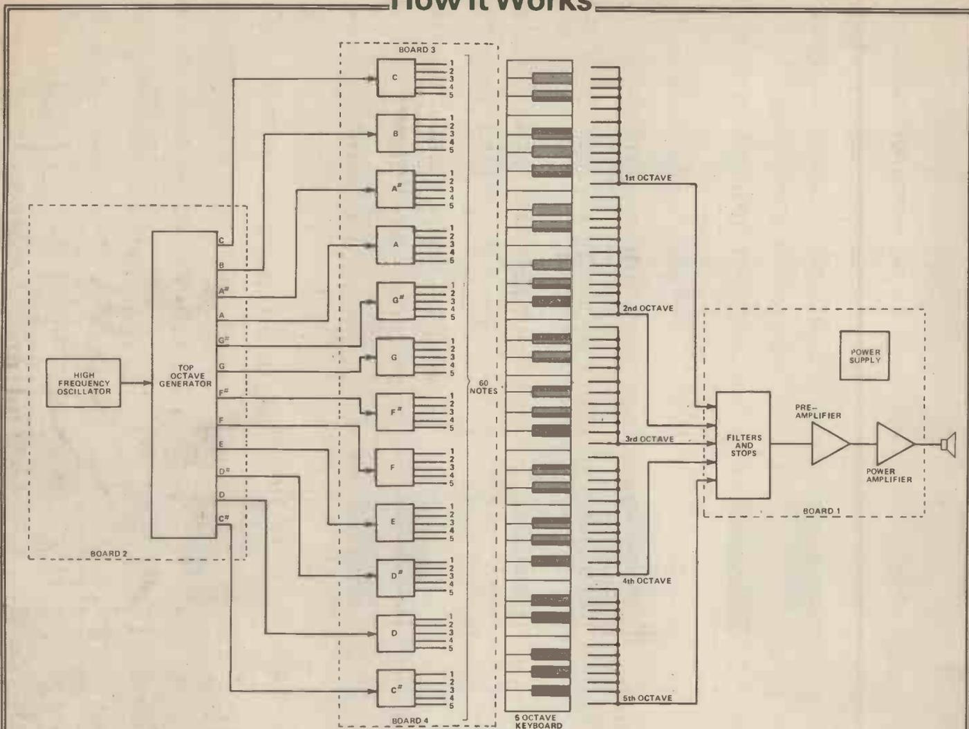
The 60 notes of the organ are all generated from a single high frequency oscillator, running at about 500 kHz. The signal from this oscillator is applied to a top-octave generator which divides the 500 kHz into the 12 different notes making up a top octave.
