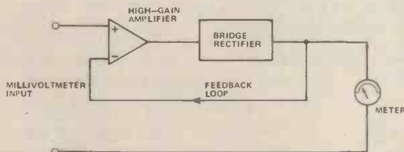
Integrated circuit IC1 forms the high-gain amplifier and is in a non-inverting configuration. This type of circuit allows a very high input resistance to be obtained which does not 'load' the circuit whose voltage is under test. Switch SW1 connects various resistors (R5-8) into circuit, each having a different value, to define the gain of the amplifier.
