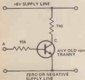
Figure 1. Simple amplifying circuit
