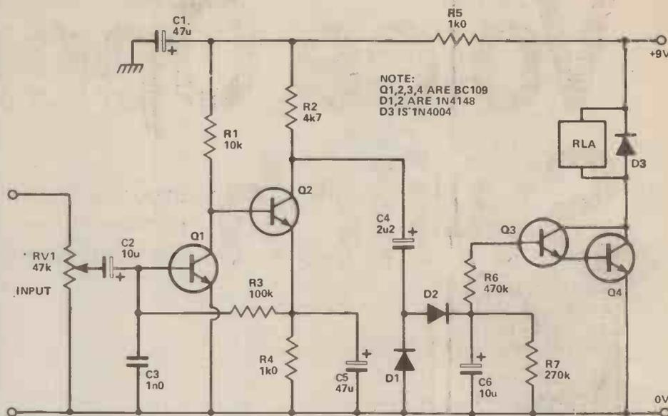
Figure 1 (above). Circuit of HEVOX. Almost any small-signal NPN transistors will work in this project, so don't worry if you can't find any BC109s
