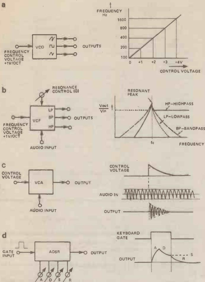
Figure 4. Principal voltage controlled stages found in a synthesiser: a) voltage controlled oscillator, b) voltage controlled filter, c) voltage controlled amplifier, d) attack, decay, sustain and release stage (envelope generator)
