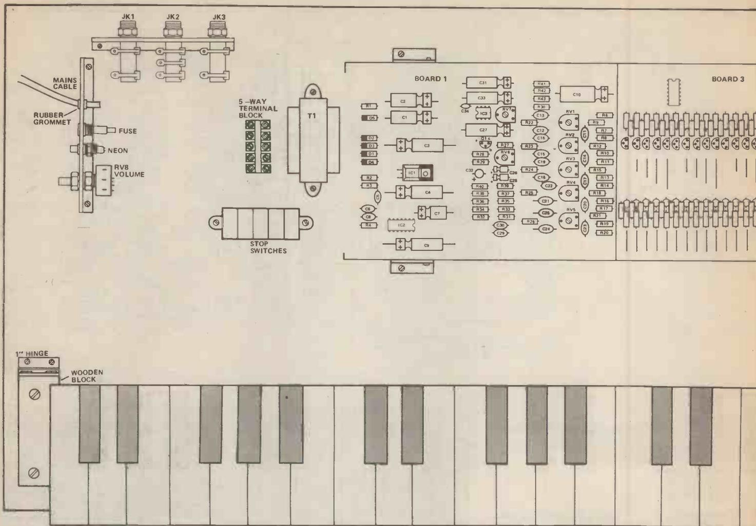
▲ Figure 6. Layout of main parts of HE Electronic Organ (not to scale). These comprise the keyboard, PCBs, transformer T1 and its terminal block, stop switches and brackets holding control potentiometers, sockets, neon indicator, fuse and mains cable grommet
