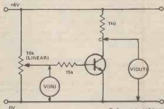
Figure 3. Circuit to investigate operation of simple one-transistor amplifier
