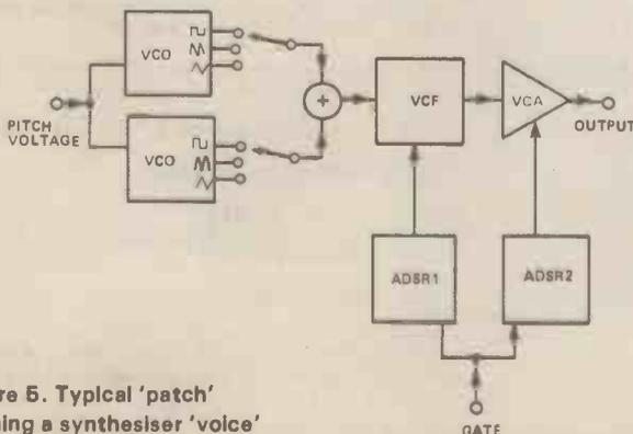
Figure 5. Typical 'patch' forming a synthesiser 'voice'
