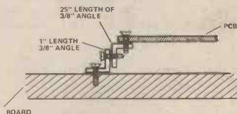
Figure 1. Section view of a PCB guiderail
