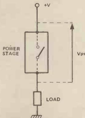
Figure 1. Showing the voltage developed across a semiconductor power stage, when driving a load
