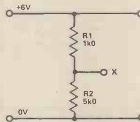
Figure 2. Using two resistors in series to demonstrate how the circuit in Fig. 1 operates. The voltage drop across R1 and R2 is measured from point X
