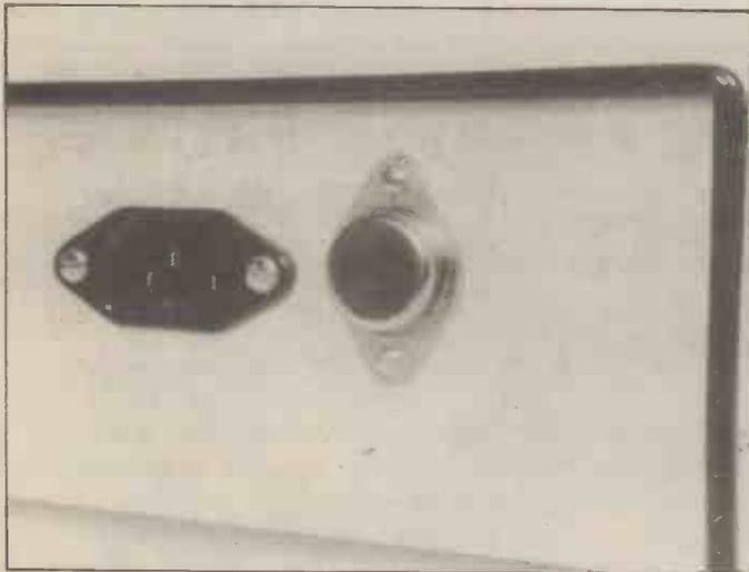
Figure 4. If your project is housed inside a metal case you can use one of the case sides as a heatsink
