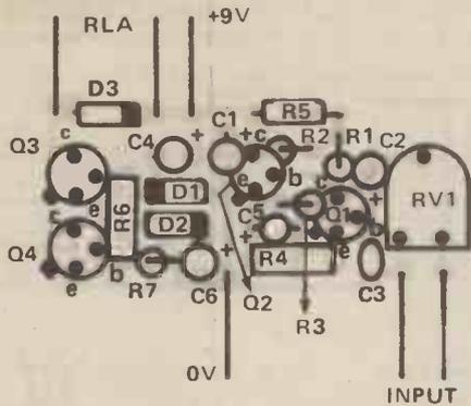
Figure 3. Overlay and connection details of the printed circuit board
