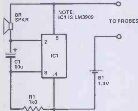
Figure 1. Circuit of the Continuity Checker
