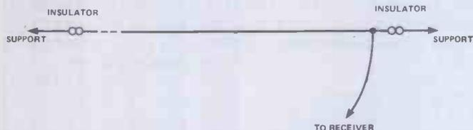
Figure 8. The traditional aerial, a long piece of wire insulated from its supports
