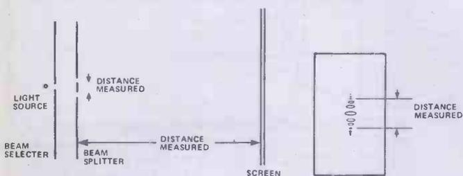
Figure 2. The method Hertz used to measure wavelength of light: (a) a slit in an opaque sheet selects one ray of light, which is then split into two by close-spaced splits in another sheet. The image projected on the screen (b), when examined with a microscope, consists of alternate dark and light bands caused by wave interference. The wavelength can be calculated from the distances indicated
