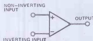
Figure 2. Circuit representation of an op amp
