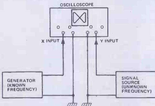
Figure 5. How a signal generator, providing a signal with known frequency and a signal source of unknown frequency, are connected to an oscilloscope to produce Lissajous figures
