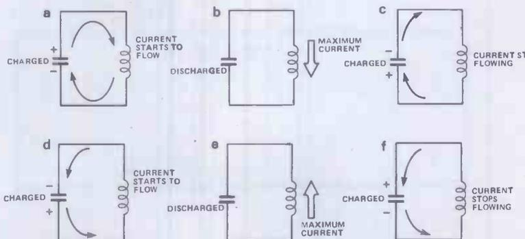
Figure 11. A charged capacitor in a resonant circuit. Figures 11a to 11f show how the charge produces a current which then charges the capacitor in the opposite direction, reversing the current until the charge is almost at its original value
