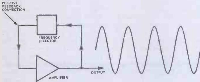
Figure 2. Block diagram of an oscillator
