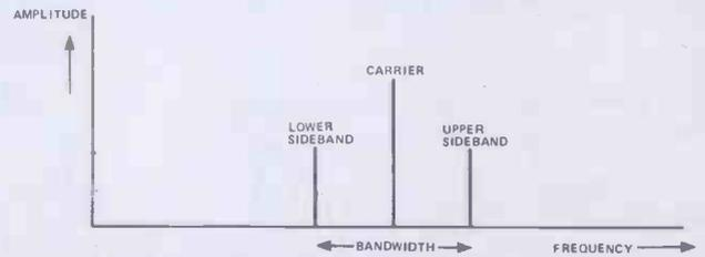
Figure 6. Sidebands. A carrier alone has a single value of frequency. When it is modulated by a low-frequency signal, the result is two new frequencies, the upper and lower sidebands
