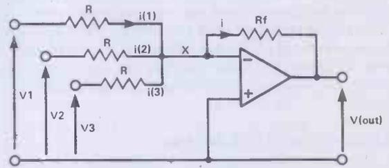
Figure 4. Op amp used as a summing amplifier
