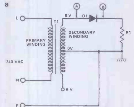
Figure 2. Simple power supplies. Figs. 2c and 2d are shown overleaf a) single-diode, half-wave rectified circuit, with resistive load.
