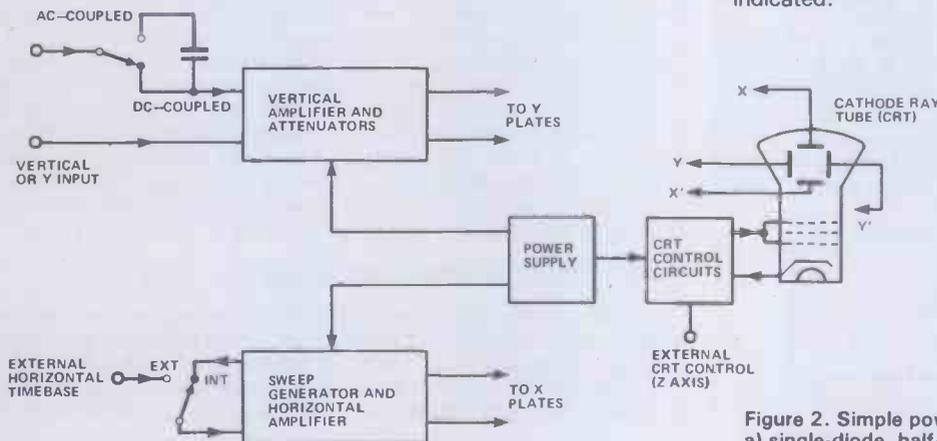
Figure 1. Principal stages of a simple oscilloscope
