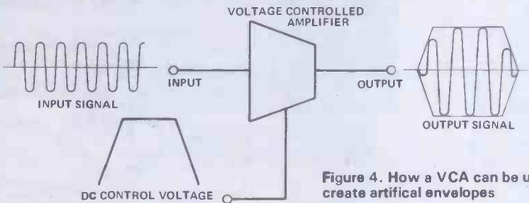
Figure 4. How a VCA can be used to create artificial envelopes
