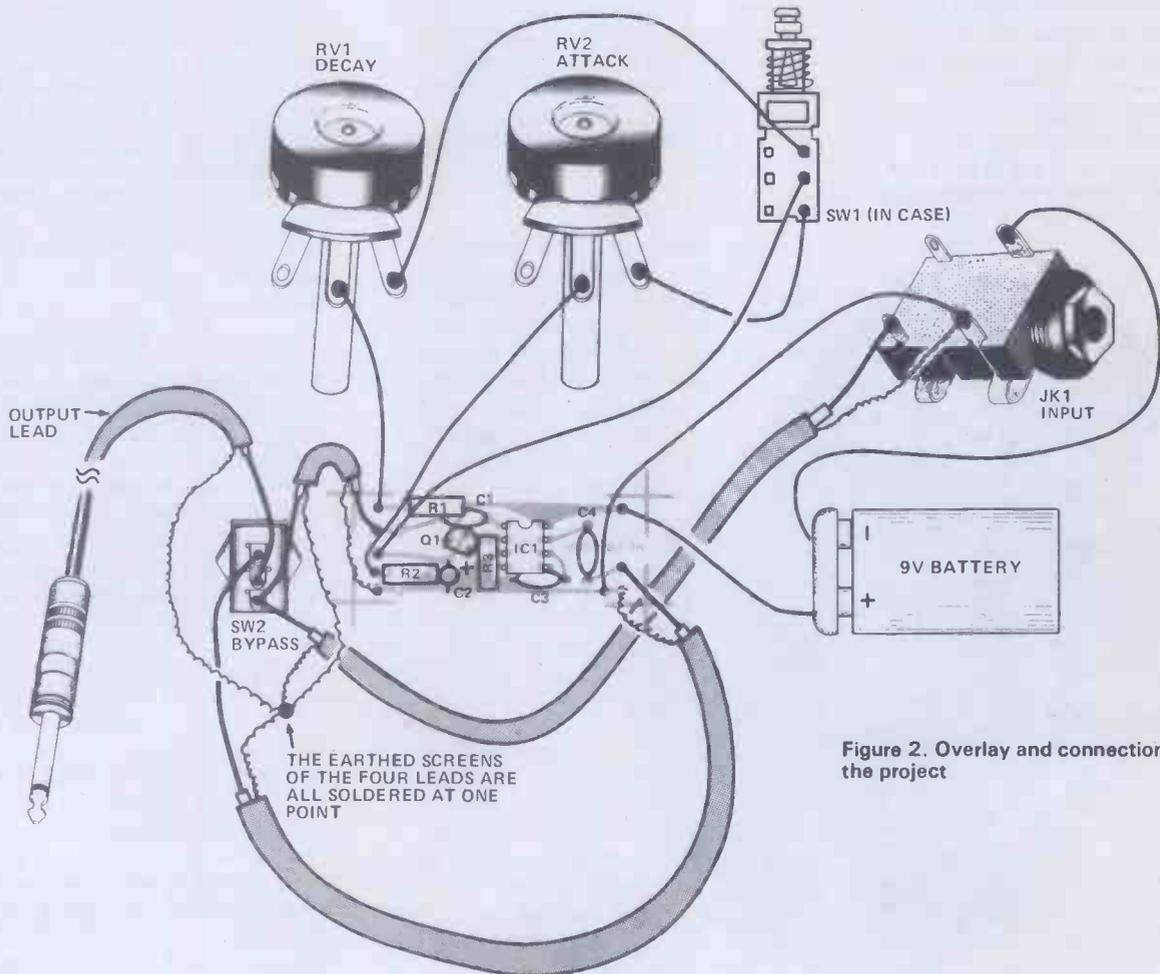
Figure 2. Overlay and connection details of the project
