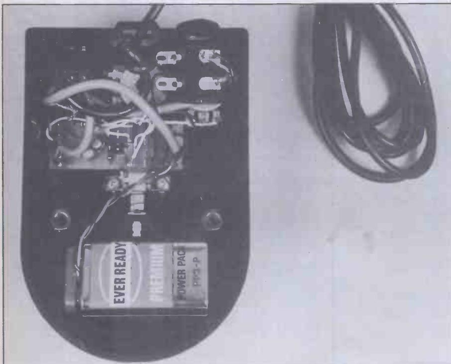
Figure 5. Internal view of the case showing how tight a fit it is. Note the use of screened cable for all audio signal-carrying leads
