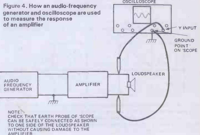
Figure 4. How an audio-frequency generator and oscilloscope are used to measure the response of an amplifier
