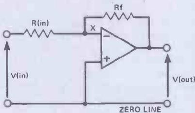
Figure 3. Circuit arrangement to show that voltage  $A_v$  is equivalent to  $R_f/R(\text{in})$
