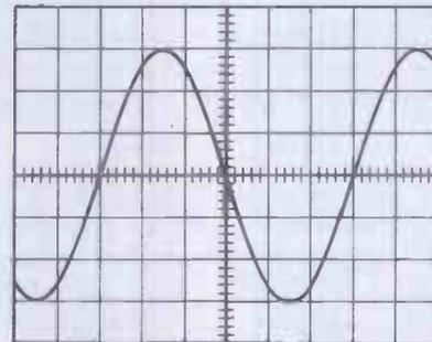
Figure 7. Example of sine wave signal displayed on typical oscilloscope screen. Timebase has been set to 5 ms/cm and vertical attenuator to 1 V/cm
