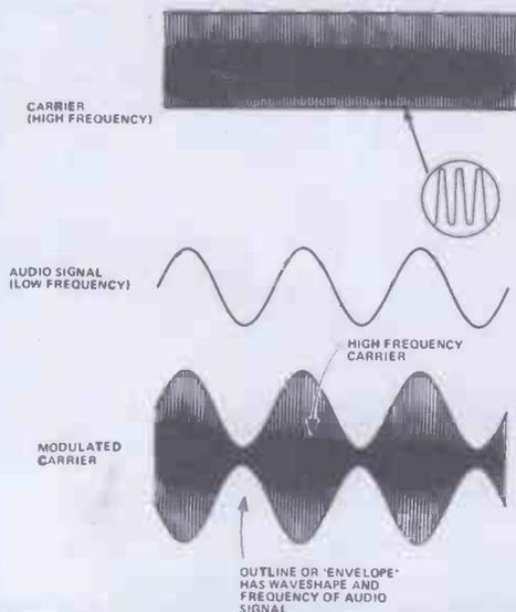
Figure 5. Modulating a radio-frequency carrier so that it carries an audio frequency wave. The frequency of the carrier must be much higher than the frequency of the audio wave
