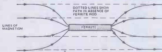
Figure 9. How ferrite concentrates magnetism. The dotted lines show what the tracks of the magnetic lines would be if no ferrite were present
