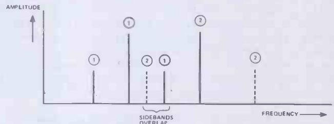
Figure 7. Interference is caused when the sidebands of two transmitters overlap, even though the carriers are separated
