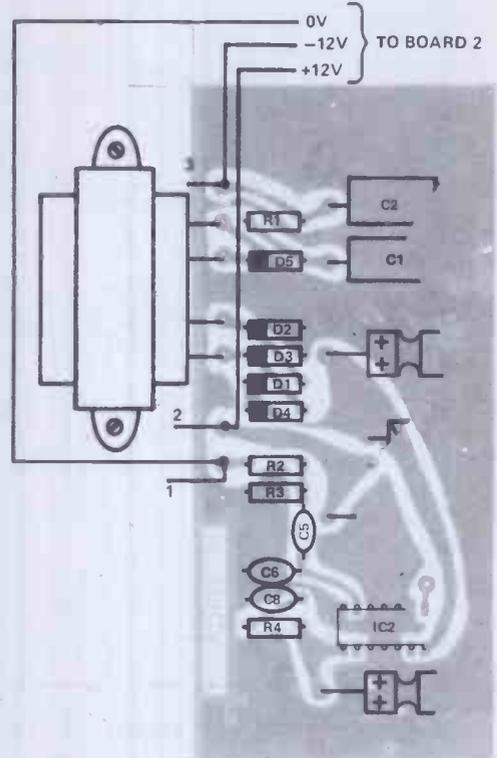
Figure 3. The edge of Board 1 where power connections are taken to Board 2
