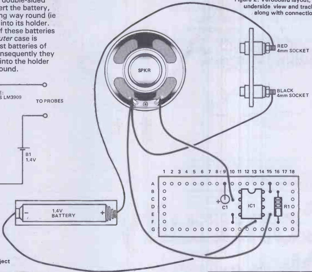
Figure 2. Veroboard layout, showing underside view and track breaks, along with connection details
