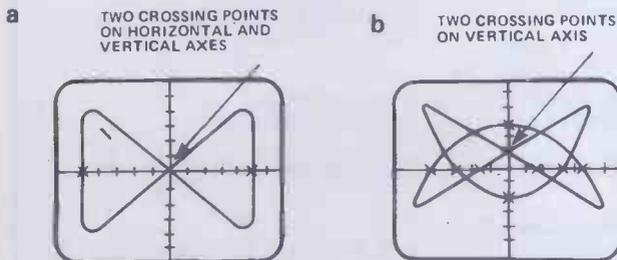
Figure 6. Lissajous figures produced by signals applied to the vertical and horizontal inputs of a 'scope: a) trace crosses horizontal axis at four points (twice at centre of screen) and vertical axis at two points (both at centre of screen), b) six crossing points on horizontal axis and four on vertical axis
