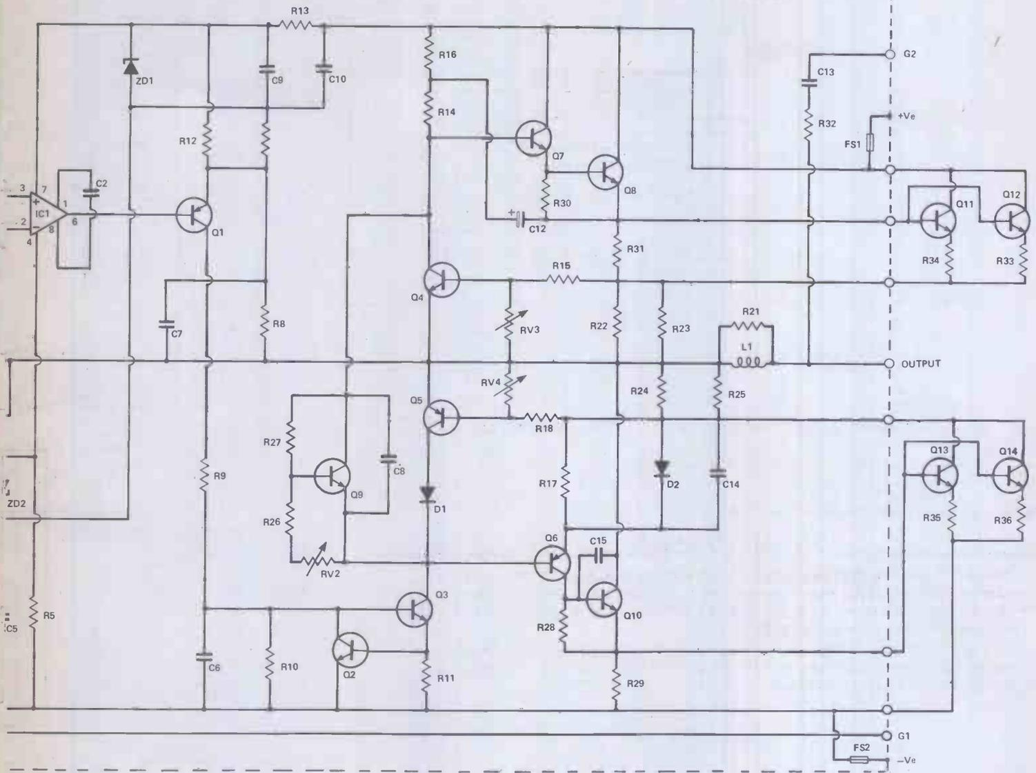
Figure 4 Circuit of the 150 W power amplifier, reproduced by courtesy of Capricorn Electronics. Two identical circuits are used on ready-built PCBs in the HE Power Amplifier
