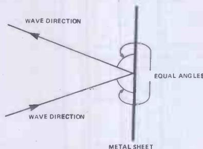
Figure 3. Wave reflection. Radio waves are reflected from a metal sheet in just the same way as light waves are reflected from any mirror
