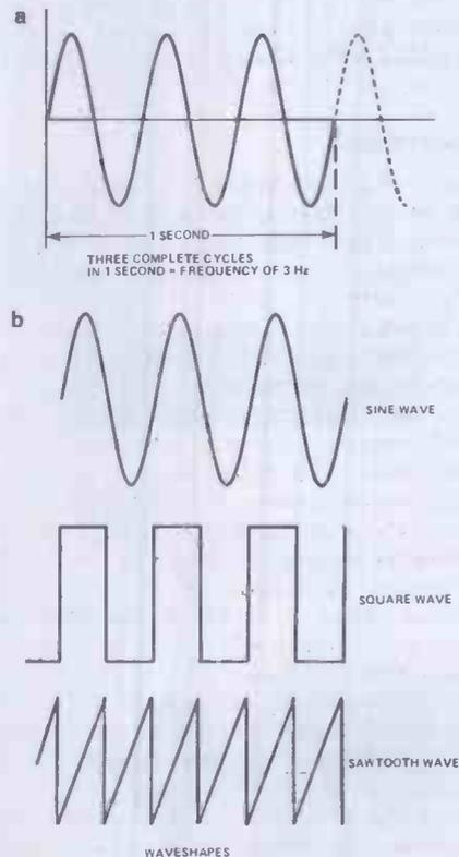
Figure 3. Frequency and waveshape. Frequency (a) is the whole number of complete cycles of a wave which happen each second. The waveshape is the shape of the graph of the wave plotted against time. For a sound wave, the quantity that is plotted is air pressure, and for an electrical wave, voltage is plotted
