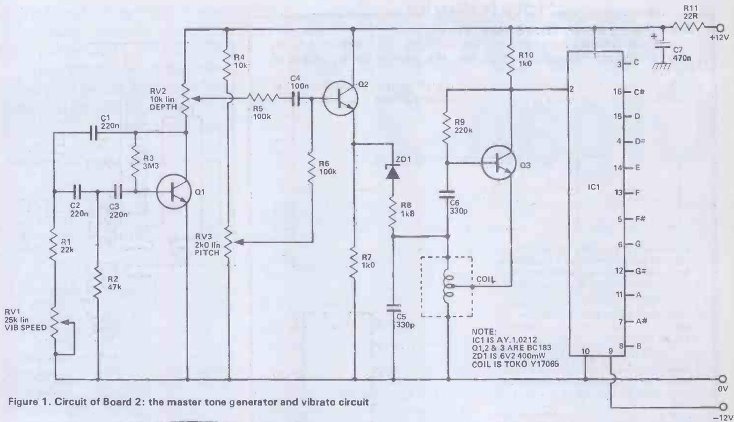
Figure 1. Circuit of Board 2: the master tone generator and vibrato circuit
