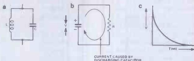
Figure 10. The resonant (tuned) circuit (a). This is a parallel type. If the capacitor were charged and connected to a resistor (b), then the capacitor would rapidly discharge through the resistor (c)
