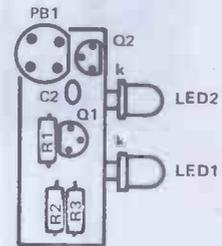
Figure 2. Overlay of the PCB
