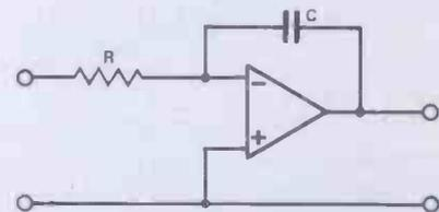
Figure 5. Op amp used as an integrator
