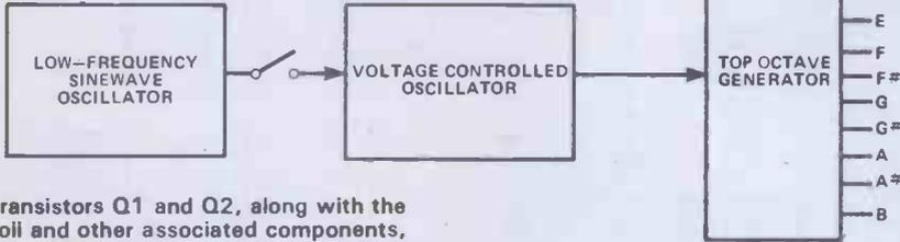
Transistors Q1 and Q2, along with the coil and other associated components, form a high-frequency voltage controlled oscillator, the main frequency of which is adjustable by the position of the ferrite slug in the coil. Other control inputs come from pitch control RV3 and the low-frequency sinewave oscillator output from RV2.
