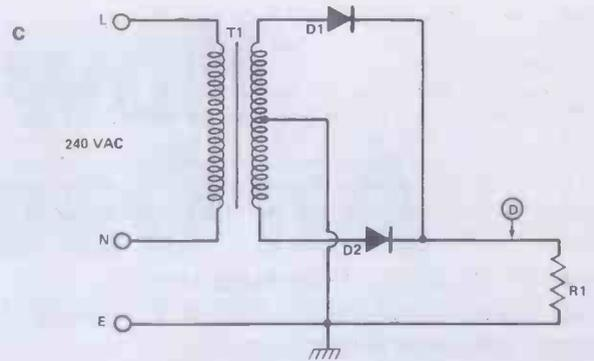
c) two-diode, full-wave rectified circuit, with resistive load.
