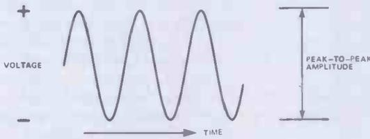
Figure 4. Peak-to-peak amplitude for a wave
