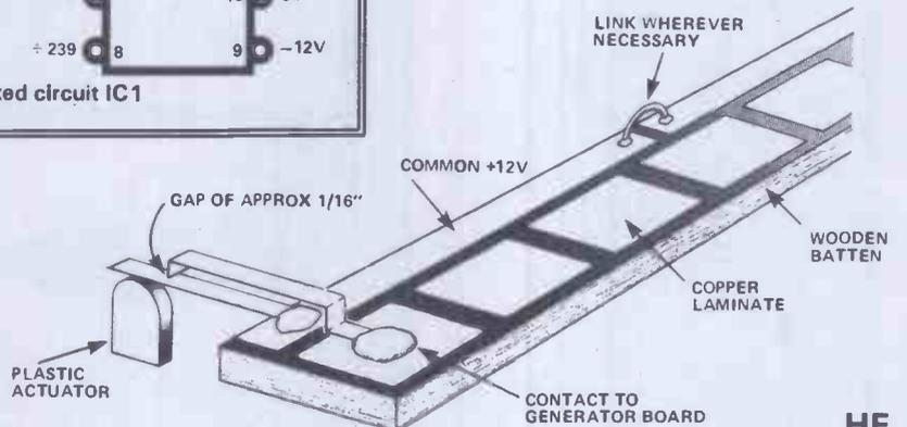
Figure 4 (above). Details of one key contact. This should be repeated along the length of the keyboard, until all 60 notes have a working contact
