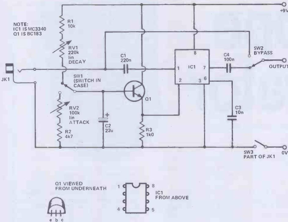
Figure 1. Circuit of HE Envelope Generator
