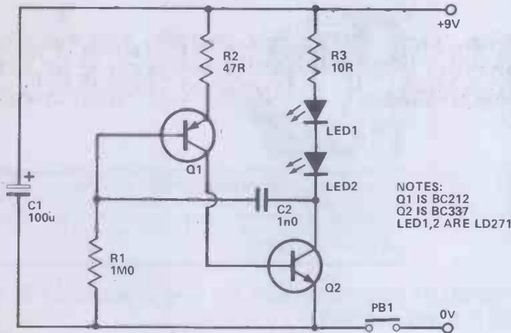
Figure 1. Circuit of the infra-red transmitter
