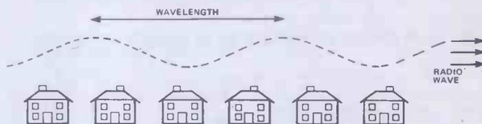
Figure 1. Wavelength. As the radio wave travels through space, there is a measurable distance between wavepeaks. This distance is the wavelength
