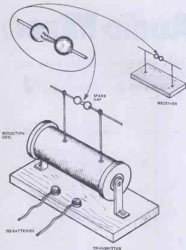
Figure 1. Hertz's transmitter and receiver. The induction coil is a DC to AC converter producing high-voltage pulses (about 40 kV)
