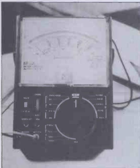
Figure 5. The HE Multitester. If you already have a multimeter (20k/V or better) then you will be able to use it for the measurements described in this series. If you have *no* meter then take advantage of this excellent instrument at an attractive price
