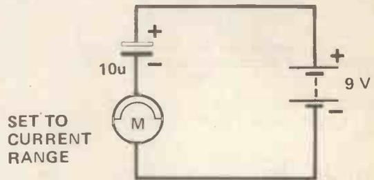
Figure 8. How to measure leakage current through an electrolytic capacitor
