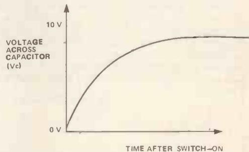
Figure 12. Graph of voltage/time for a capacitor charging in a 10 V circuit
