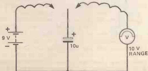
Figure 4. Simple method of charging a capacitor and measuring the charge voltage
