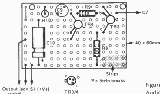
Figure 11.4 Audio amplifier board
