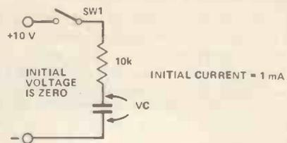
Figure 11. Charging a capacitor — the voltage across the capacitor is zero before the switch contacts are closed
