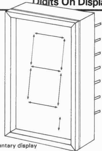
Figure 10. Typical filamentary display
