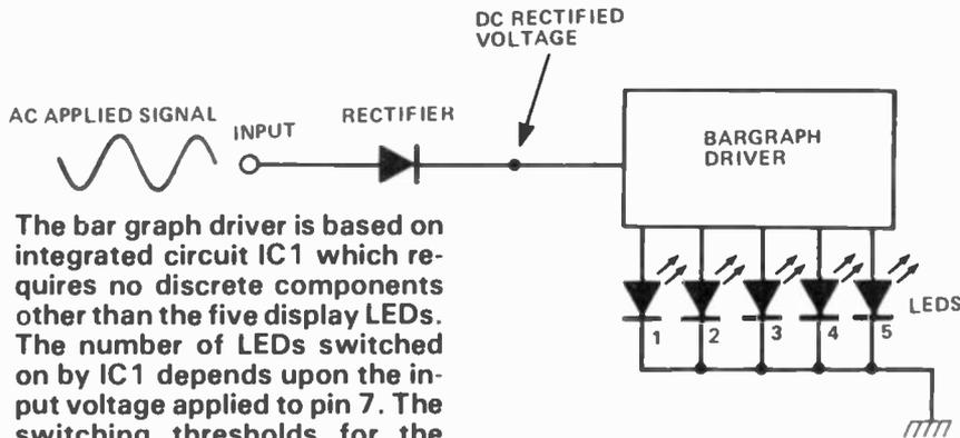
The bar graph driver is based on integrated circuit IC1 which requires no discrete components other than the five display LEDs. The number of LEDs switched on by IC1 depends upon the input voltage applied to pin 7. The switching thresholds for the LEDs are 0.1 V for LED1, 0.32 V for LED2, 0.71 V for LED3, 1 V for LED4 and 1.41 V for LED5. This non-linear sequence is needed to give the five conveniently spaced VU levels, and the U267B is specifically designed for use in this type of equipment.
