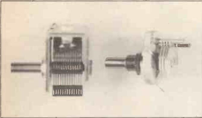
Figure 9. Variable capacitors: (a) miniature air-spaced type, (b) standard size air-spaced, (c) twin-ganged air-spaced capacitor: the two capacitors are on the same shaft so that their values change together, (d) a solid-dielectric variable capacitor — the material between the plates is a solid insulator
