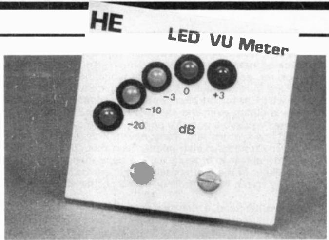
If you require a quality VU meter to use with your tape recorder, or if you simply want a pretty audio display on the front of your hi-fi system, then build this five LED VU meter. Better still, build two for stereo
