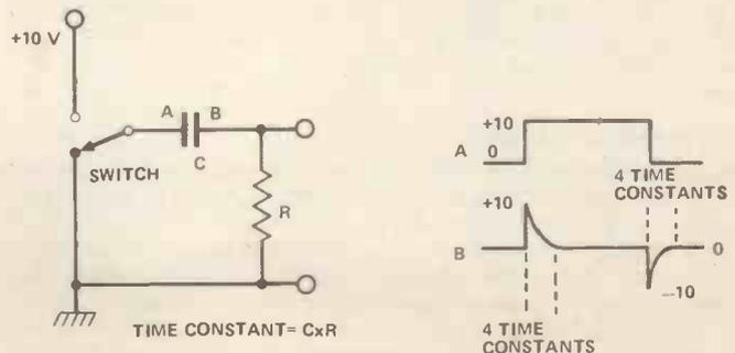
Figure 13. Demonstrating the effects of time-constants
