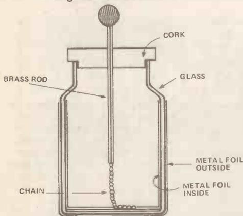
Figure 1. Classic Leyden Jar form of capacitor. Right up to the end of World War II, the Navy still measured capacitance in units called 'Jars'
