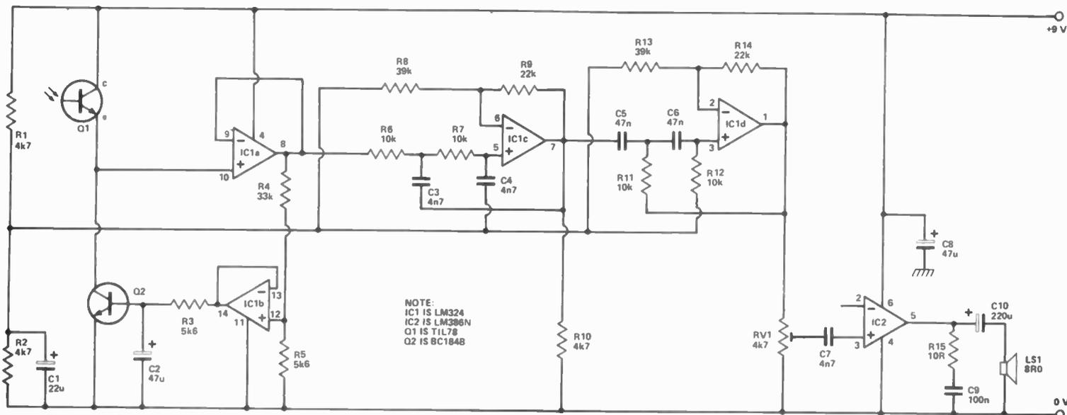
Figure 1. Circuit of the HE Sound Torch Receiver
