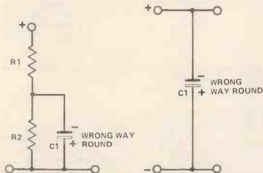
Figure 7. Wrongly-connected electrolytics: (a) probably harmless, because the resistors will prevent excessive current flow flowing, (b) wait for the bang!
