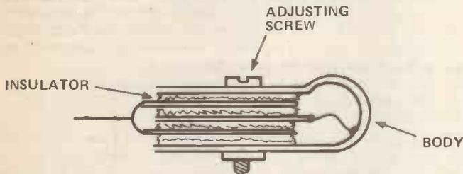
Figure 10. Operating principle of the compression trimmer — tightening the screw forces the plates closer together, so increasing capacitance
