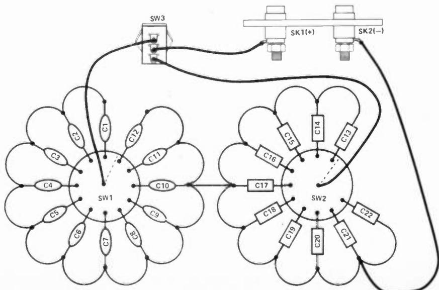
Figure 2. Wiring diagram of the Capacitance Substitution Box
