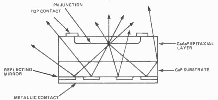
Figure 4. Section through high efficiency gallium arsenide phosphide (GaAsP) or gallium phosphide (GaP) LED
