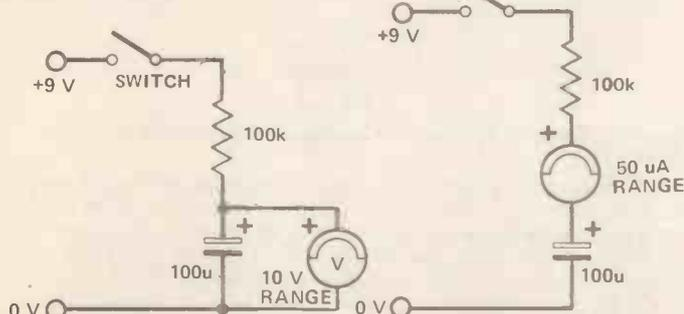
Figure 15. How to measure the voltage across a charging capacitor — this is possible only if the capacitor has a large value, because smaller values will have completed charging before the meter has had time to respond
