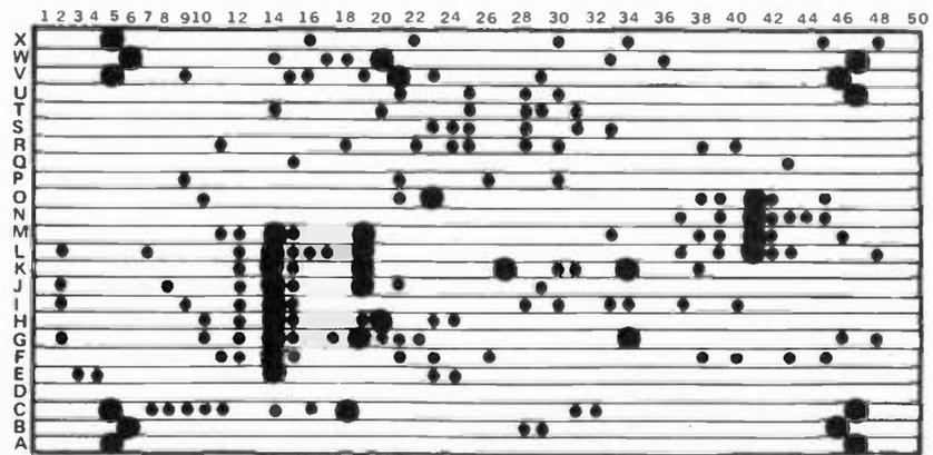
Figure 2. Veroboard layout, and underside view showing component locations and track breaks
