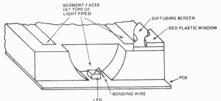
Figure 5. Section through a 7-segment LED display where light is transmitted to the segment faces by means of 'light pipes'
