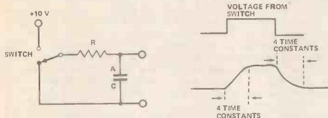
Figure 14. Circuit similar to that in Fig. 13, to demonstrate effects of time-constants. Here the positions of the capacitor and resistor have been swapped
