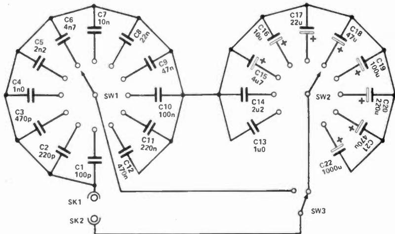
Figure 1. Circuit of an HE Capacitance Substitution Box. By replacing capacitors with resistors (see text) a resistance substitution box can also be made
