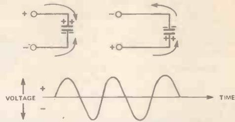
Figure 17. Effect of AC — the capacitor alternately charges and discharges for each direction of voltage, so that current flows continually
