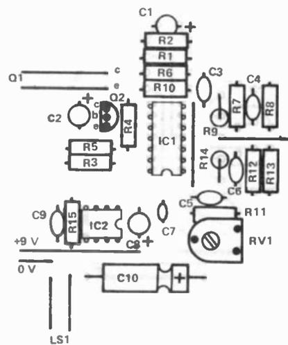
Figure 2. Overlay of the receiver PCB
