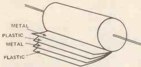
Figure 6. Tubular rolled capacitor construction
