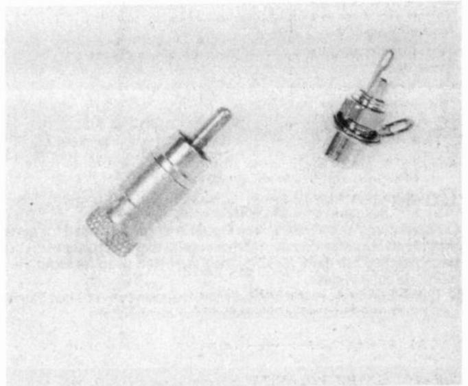
Figure 1. Phono plug (left) and socket. The socket bolts directly onto the case of the circuit.
