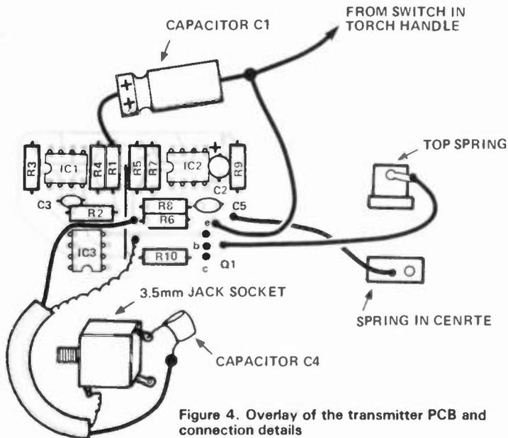
Figure 4. Overlay of the transmitter PCB and connection details
