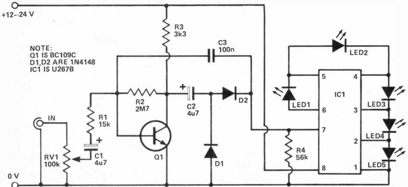
Figure 1. Circuit of the HE LED VU Meter
