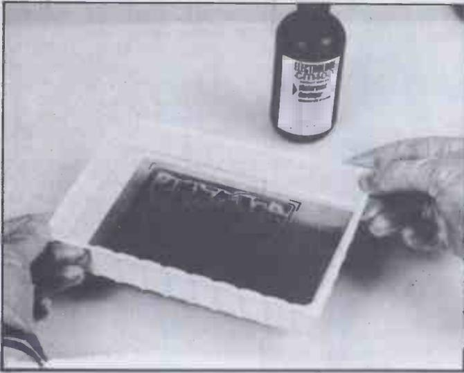
The exposed board is developed to reproduce the circuit layout.
