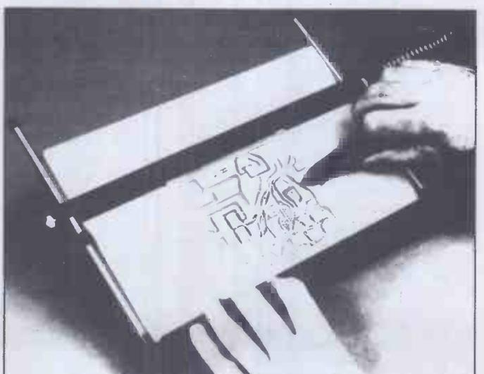
Finally, the component leads are cropped, ready for soldering.
