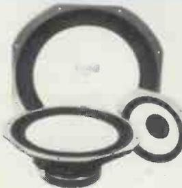
15" 109 watt R.M.S. Impedance 8ohm 59 oz magnet, 2" aluminium voice coil. Resonant Frequency 20Hz. Frequency Response to 2.5KHz Sensitivity 97dB. Price £32 each £3.00 Packing and Carriage each
