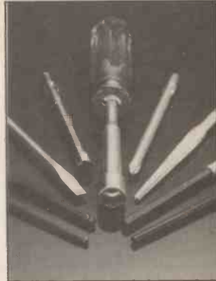
An ideal way to tackle a multitude of fastener problems is to choose a driving kit with universal handle and interchangeable blades and sockets like the kit shown here.
