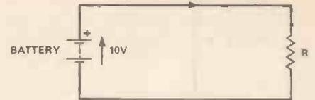
Figure 7. Showing an electric circuit, but using symbols for each component, not drawings.
