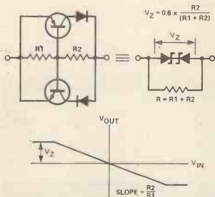
Figure 4. The 'Zener' network and its characteristics.
