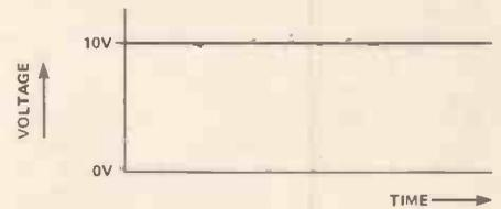
Figure 8. Output voltage of a dry-cell battery is steady with time. We call this a direct current (DC) voltage.
