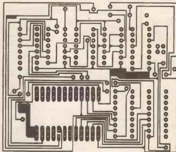
The printed circuit for the ZX81 High Resolution Graphics Project uses a double-sided board; on the left is the foil pattern for the component side and on the right is the bottom foil pattern. The PCB supplied by Cambridge Computing will be a through-hole-plated type, but home constructors will need to solder links to connect the top and bottom tracks. Do this very carefully as faults, especially dry joints, can be extremely difficult to locate!
