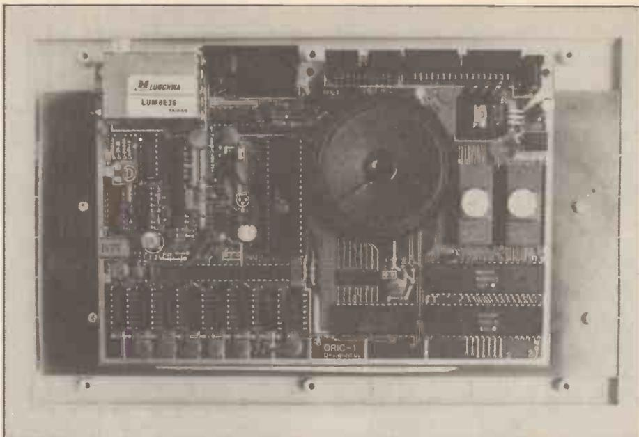
The component side of Oric's PCB, with their custom RAM refresh chip to the left of the loudspeaker.
