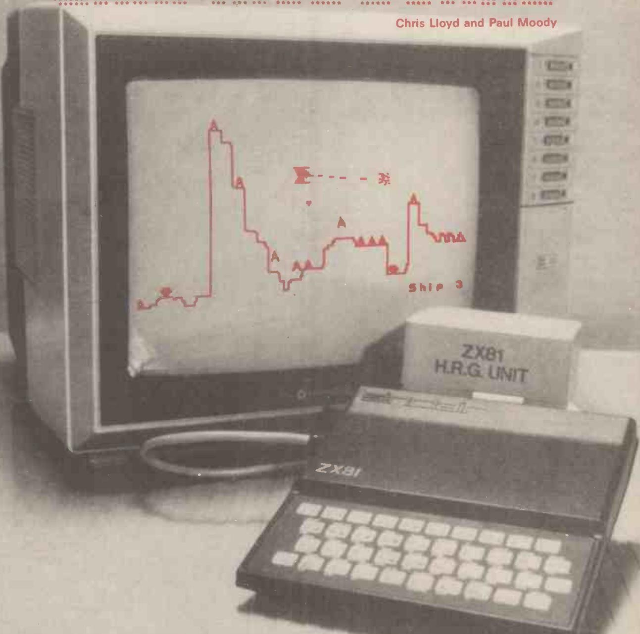
Fed up with chunky, block graphics on your ZX81? Then try our High Resolution Graphics board. It allows you to plot at least 512 points (more, with clever programming) and works with either the standard 1K computer or with a 16K RAM pack plugged in.
