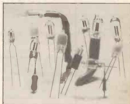
available as individual components or with a butt welded special film resistor suitable for 110-130V or 220-250V operation at temperature up to 130°C.
