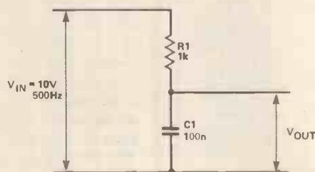
$$\text{The reactance of } C1 \text{ at } 500\text{Hz} = \frac{1}{2\pi \times 500 \times 100 \times 10^{-9}} = 3k2$$
