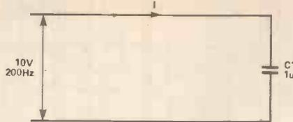
**Figure 17. The simplest AC capacitor circuit. Calculation of the current flowing in the circuit is identical to a resistor circuit as long as we know the reactance of the capacitor ] and that depends on the source voltage frequency.**
