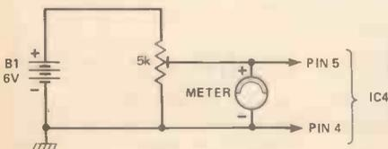
Figure 5. This circuit can be used to calibrate the IC4 circuit.
