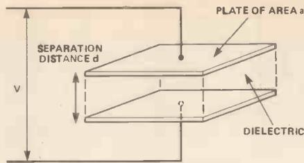
Figure 14. Basic form of a capacitor — two parallel conductive plates separated by a dielectric.
