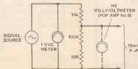
Figure 6. Using a millivoltmeter to calibrate the SPL meter.
