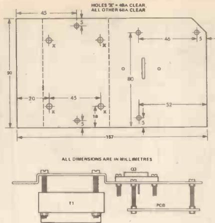
Figure 2. Assembly positions for the power supply's internal mountings: above, where and how to drill; below, the assembly seen from above.
