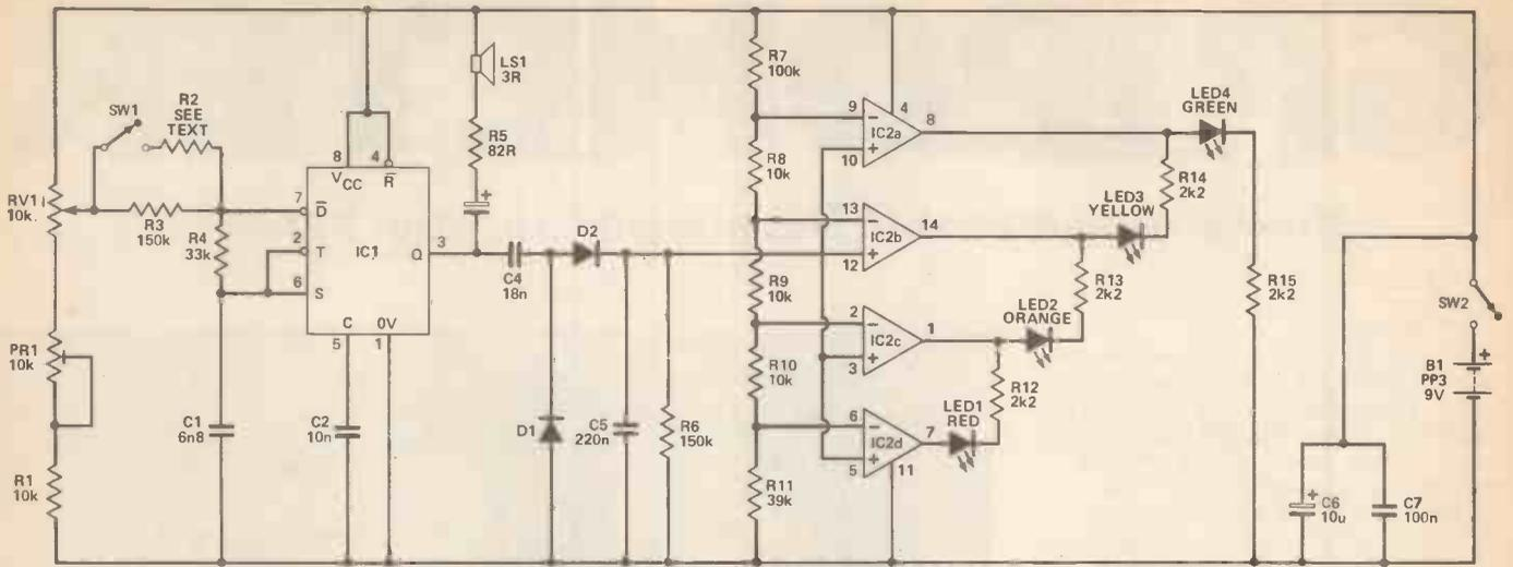
Figure 3. The Gripometer circuit.
