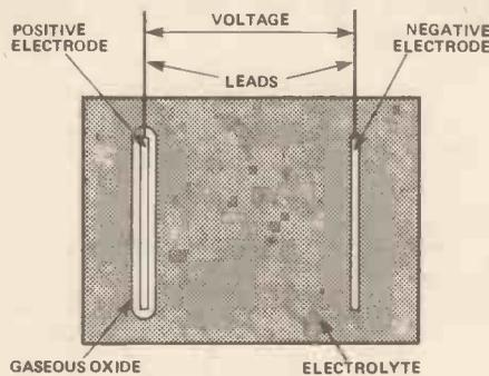
Figure 15. An electrolytic capacitor. The 'plates' are formed by the positive electrode and the surface of the electrolyte. The dielectric is the gaseous oxide layer around the positive electrode.
