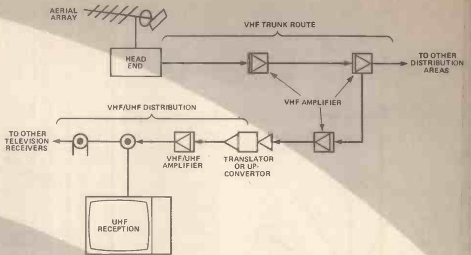
Figure 3. A typical hybrid VHF/UHF cable system.
