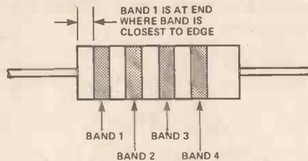
Figure 4. The resistor colour code and a table relating to each band and its colour to a resistor's value. The bulk of the colours (red to violet) are the colours of the spectrum.
