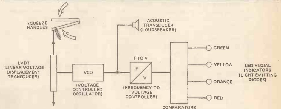
Figure 1. A block diagram of the HE Gripometer.
