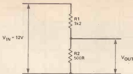
Figure 6. A voltage divider or potential divider is made with two resistors. The output voltage,  $V_{out}$ , is a ratio of the input voltage,  $V_{in}$ .
