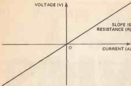
Figure 1. Showing the graphical relationship between voltage across a resistor and current through it.
