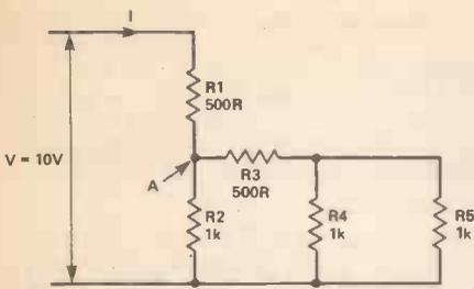
Figure 11. Quite a complex electronic circuit, but we can reduce it in complexity to an equivalent circuit.
