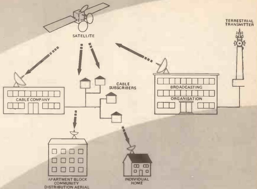
Figure 6. The integration of all modes of transmission.
