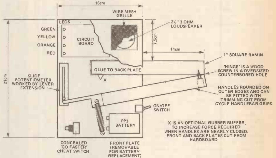
Figure 4. The mechanics of the Gripometer.
