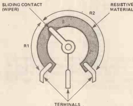
Figure 7. Make-up of a pot — a potentiometer. The wiper can rotate around the resistive material altering the ratio between  $R_1$  and  $R_2$ .
