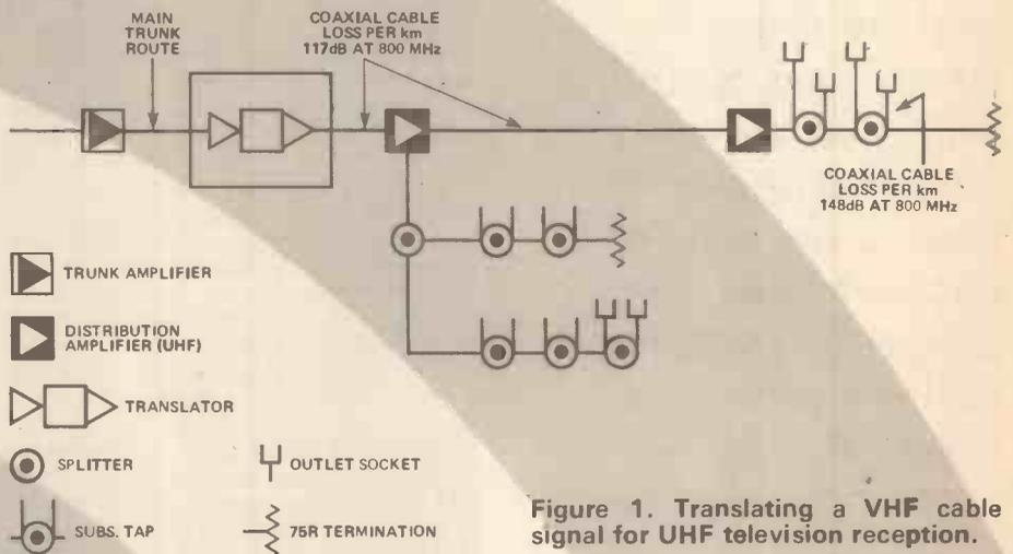
Figure 1. Translating a VHF cable signal for UHF television reception.
