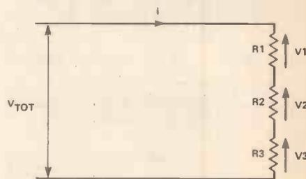
Figure 9. A more complex circuit, consisting of three resistors in series. The total voltage is made up of three voltages across each resistor. The current flows equally through each resistor.
