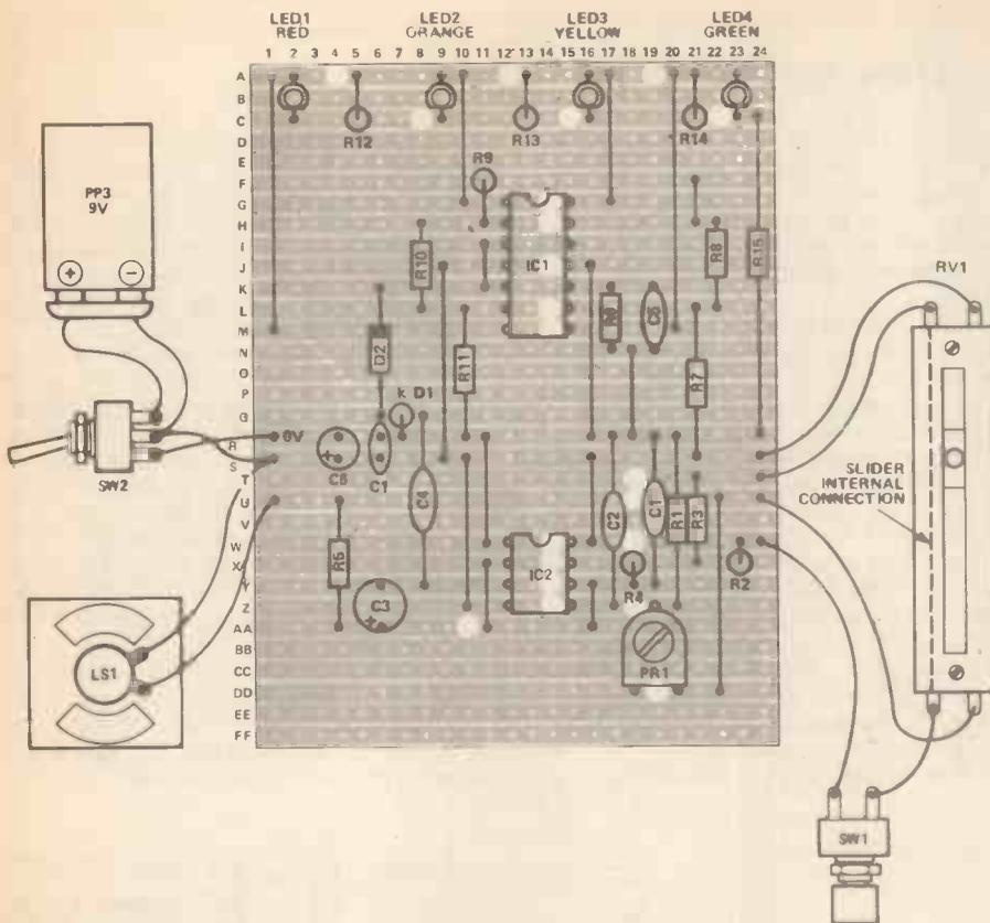
Figure 5. The Veroboard layout.
