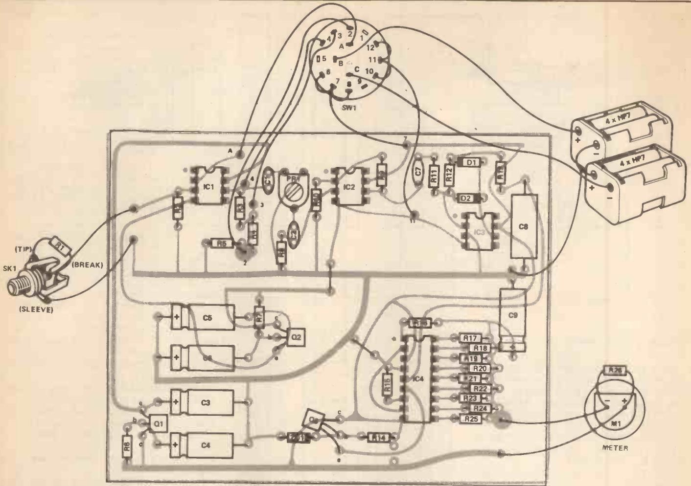
Figure 3. The PCB and components for the Sound Pressure Level Meter.
