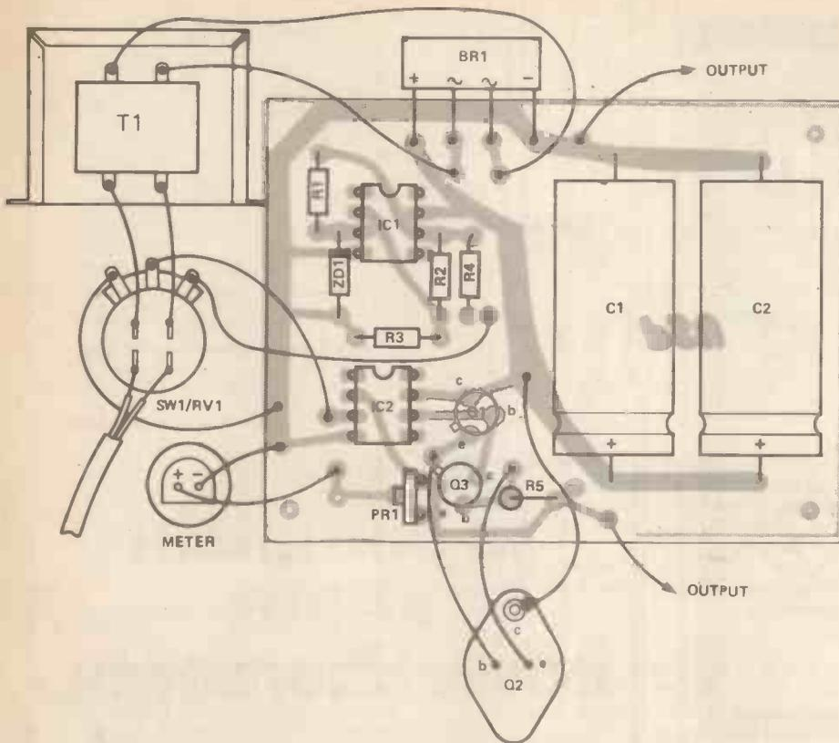
Figure 4. The components. The trick is to get the wire links short enough so that they don't make a 'rat's nest' and long enough so that they don't pull off if any components work loose in transit.
