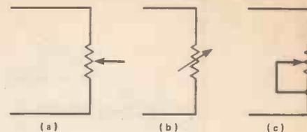
Figure 8. a) Symbol of a pot used as a potential divider. b) Symbols of a pot used as a variable resistor — either symbol is correct, but version c shows correctly how the pot is physically connected in a circuit.
