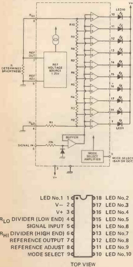
Figure 4. Inside the IC4, the LM3915 (see page 15 above).
