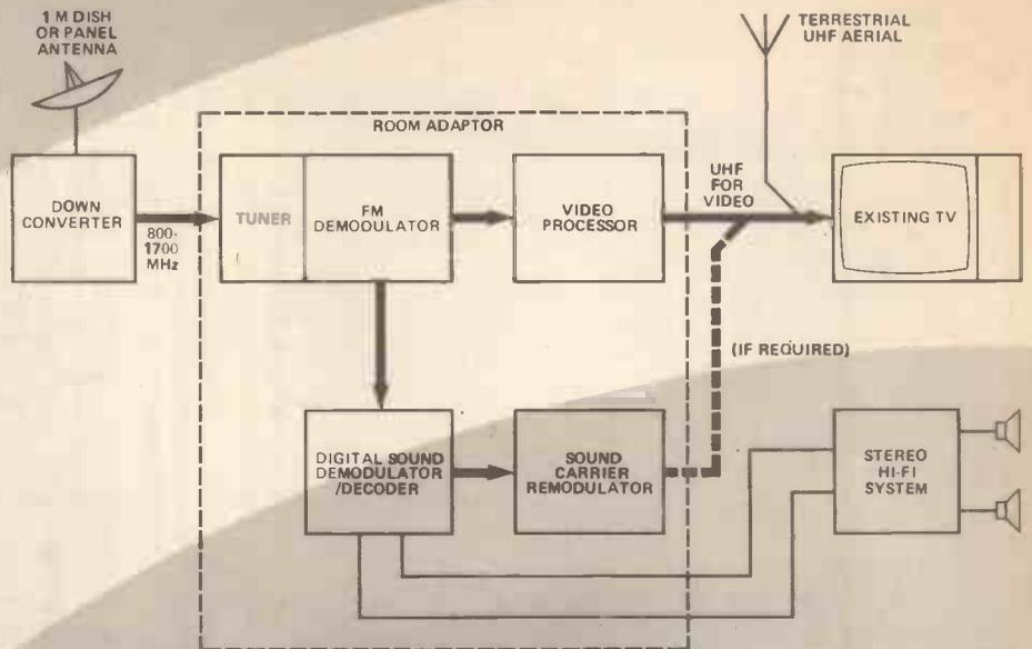
Figure 7. Stages in translating a DBS signal for a UHF receiver.
