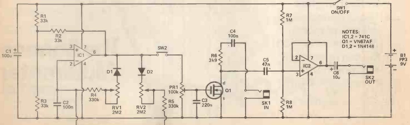
due to the high input impedance of the buffer amplifier formed by IC2 and its associated components, so the signal reaches the output virtually unattenuated, but when Q1 is switched on, most of the input voltage is dropped across R6 and a high level of attenuation (typically about 66dB) is produced.
