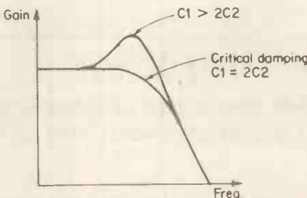
Figure 11. Response curves of the classical filter circuit.
