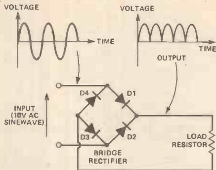
Figure 9. A bridge rectifier, consisting of four diodes, giving a full-wave rectified DC output from an AC sine wave input.
