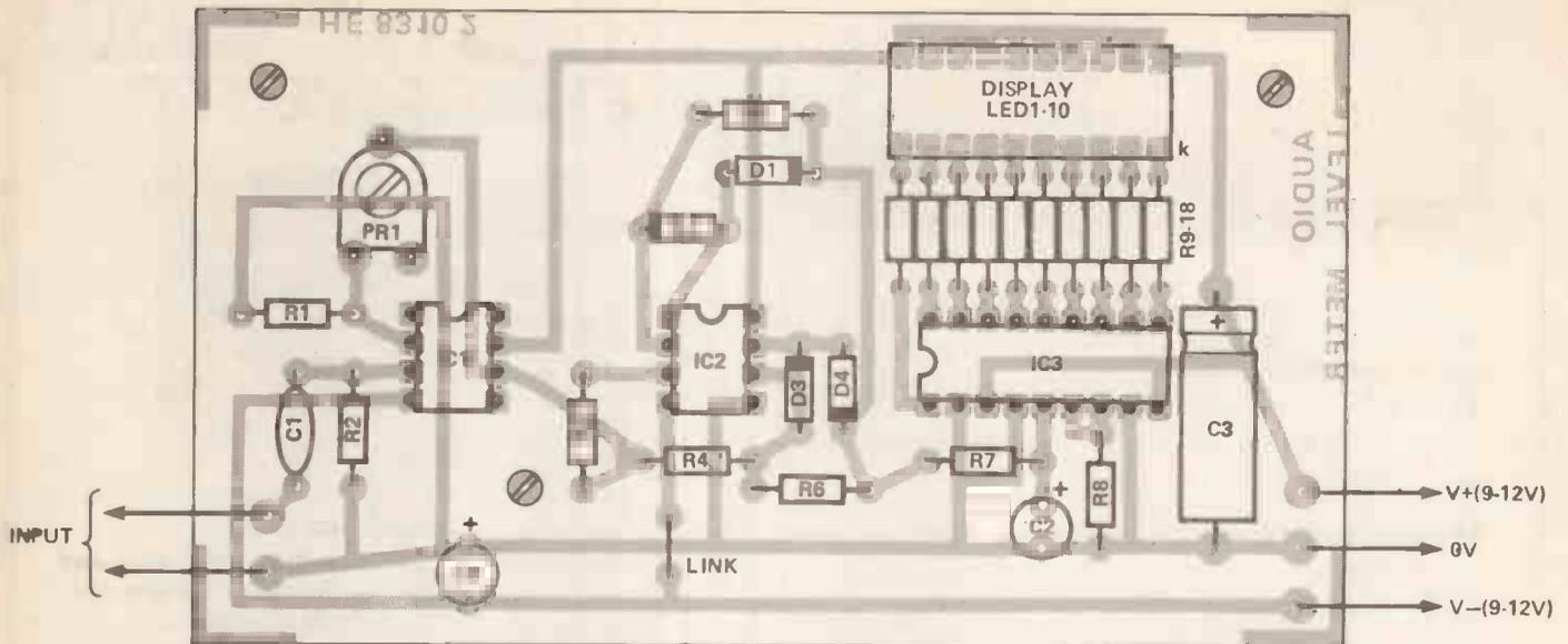
Figure 3. The components, with one wire link.
