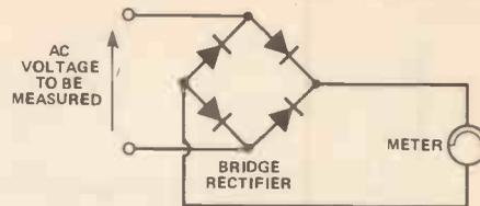
Figure 11. Measuring an AC voltage with a DC meter.
