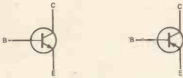
Figure 14. Circuit symbols for NPN and PNP transistors.
