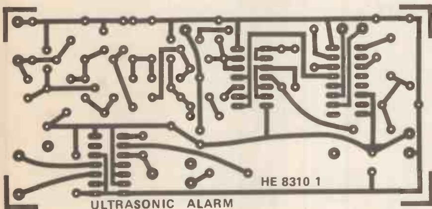
Left: The Ultrasonic Intruder Alarm PCB layout.
