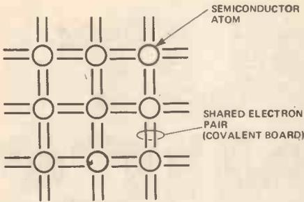
Figure 2. A minute section of semiconductor material showing atoms and covalent bonds.
