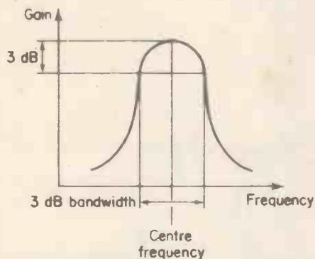
Figure 18. The response obtained by a bandpass filter.
