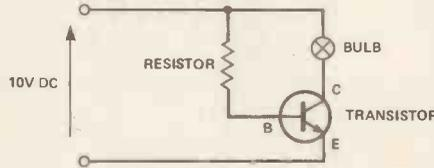
Figure 18. The circuit of Figure 17 — using a transistor.
