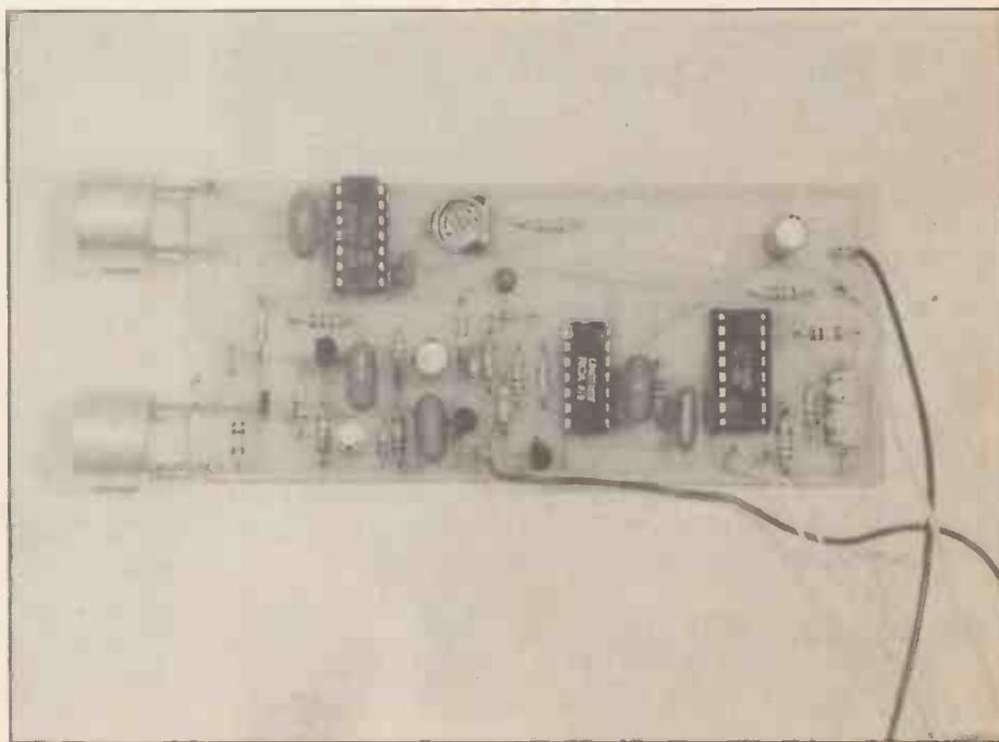
In the prototype, the transducers are mounted directly on the board.
