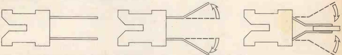
Figure 1. How to bend the pins on the edge-connector socket for soldering to the PCB.
