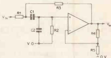
Figure 15. A single-amplifier band pass filter.
