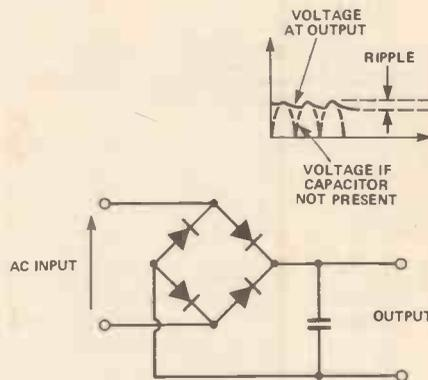
Figure 12. A reservoir capacitor used to smooth the full-wave rectified DC output of the bridge rectifier to an acceptable ripple.
