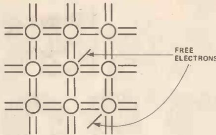
Figure 3. N-type semiconductor. Pure semiconductor material is doped with atoms which have five electrons in outer orbit. Four electrons pair with electrons of adjacent atoms leaving one free electron.
