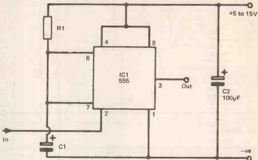
Figure 4. Basic 555 monostable. It is triggered by briefly taking pin 2 below  $\frac{1}{3} V+$ .
