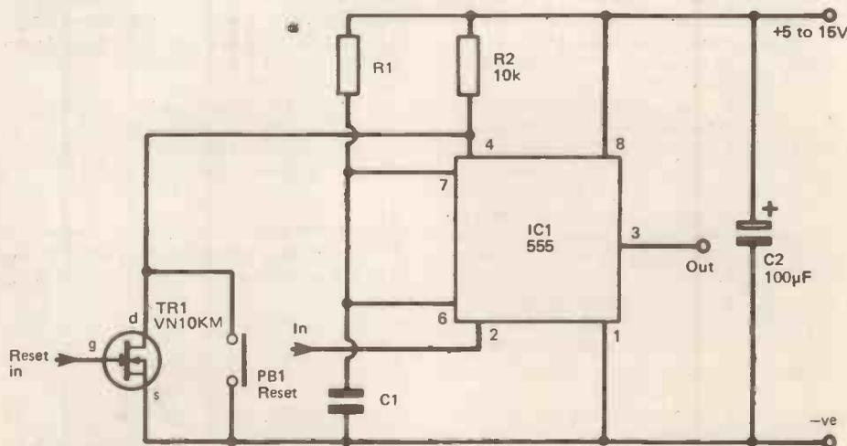
Figure 6. The monostable can be reset by taking pin 4 low, either manually with a switch or by taking the gate of TR1 a few volts positive.
