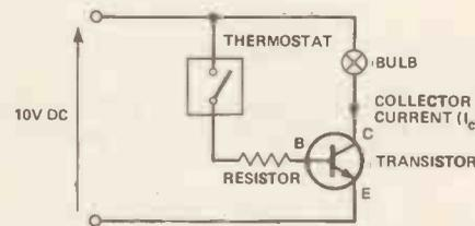
Figure 19. Automatically switching a transistor using a thermostat.
