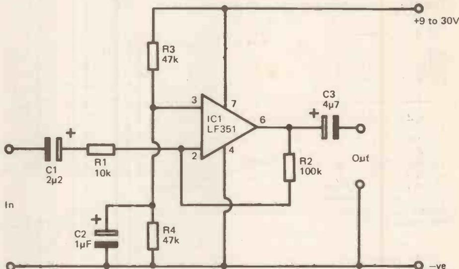
Figure 22. The circuit for an inverting amplifier using the LF351 op-amp, biased from a single supply rail.
