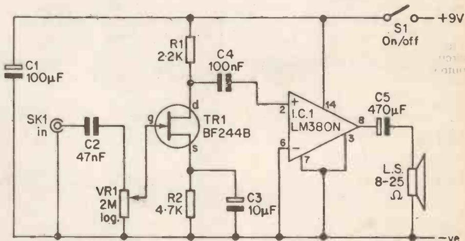
Figure 8. The LM380N has built-in thermal and short circuit protection, making it the ideal device for test and breadboard situations.
