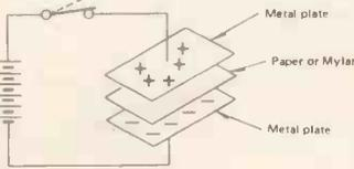
The amount of electricity stored (the electrostatic capacity) depends upon the size of the metal plates. Larger plates — more capacity (F).
