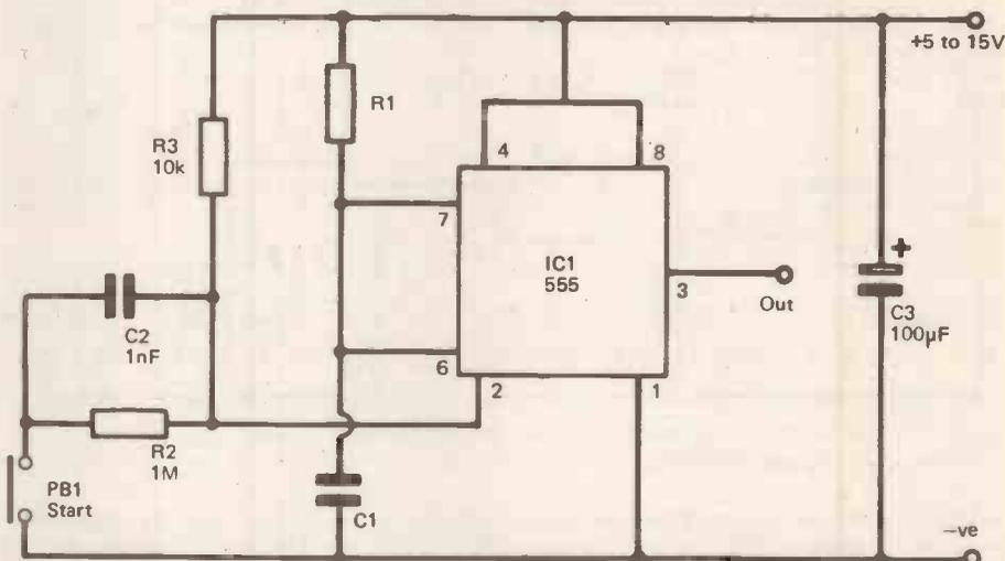
Figure 5. The length of the trigger pulse can be controlled by an RC network around the trigger switch.
