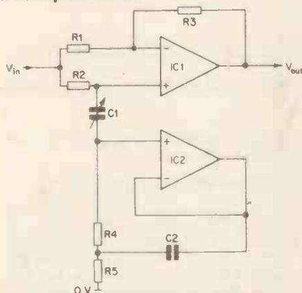
Figure 19. A turnable notch filter.
