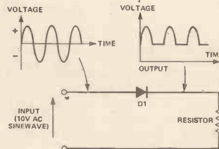
Figure 7. Application of an AC voltage to a diode gives a halfwave rectified output.
