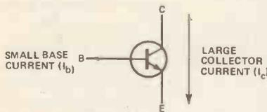
Figure 16. Summarised action of an NPN transistor.
