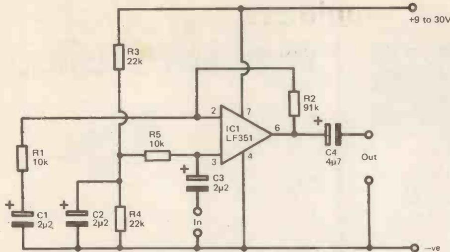
Figure 23. The LF351 in non-inverting mode.
