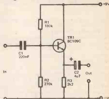
Figure 7. A simple emitter follower circuit is often used to reduce loading effects.
