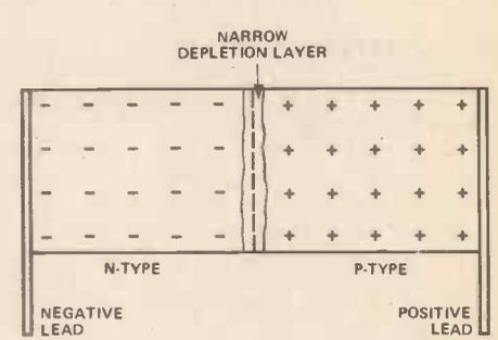
Figure 6. A diode with a positive potential applied to the P-type semiconductor layer. Above 0V7 (for a silicon diode) current flows.
