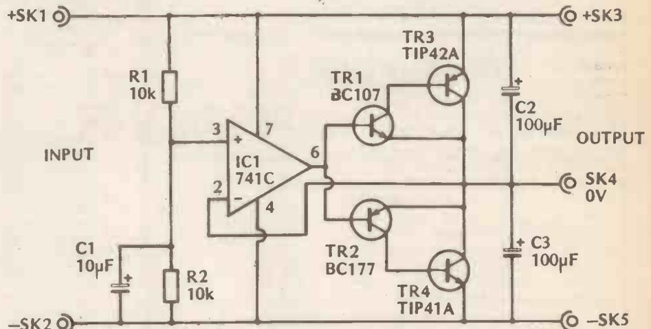
Figure 24. This supply splitter will prove its usefulness to the experimenter.
