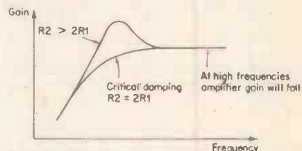
Figure 13. High pass filter response curves.
