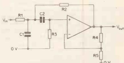
Figure 16. An alternative band pass circuit.
