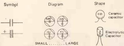
A capacitor stores direct current (charges up) by way of two metal plates positioned face-to-face.
