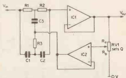
Figure 20. This notch filter has adjustable Q.
