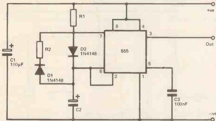
Figure 3. The mark-space ratio can be varied continuously if R1, R2 are replaced by variable resistors.
