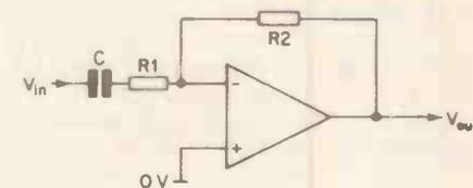
Figure 14. The simplest high pass filter circuit.
