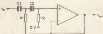
Figure 12. The classical high pass filter.
