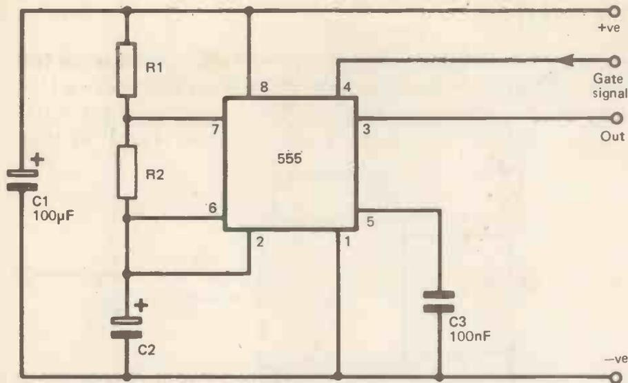
Figure 2. The gated astable can be used for producing tone-bursts or a gated clock signal.
