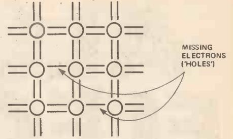
Figure 4. P-type semiconductor formed by doping pure semiconductor material with atoms having only three electrons in outer orbit. This leaves a hole for a missing electron.
