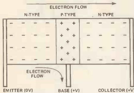
Figure 15. Basic format and applied potentials to an NPN transistor.
