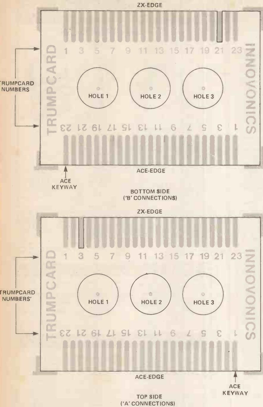
Figure 2. Wires are routed either via the HOLES in the PCB, DIRECT from edge to edge, or between the pins of the EDGE connector as seen in the photograph.
