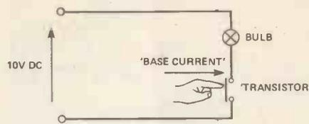
Figure 17. Likening the action of a transistor to that of a mechanical push-button switch.
