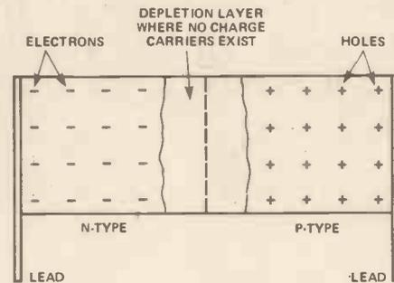
Figure 5. A diode, formed by a combination of P-type and N-type semiconductor material. No voltage is yet applied across the diode.
