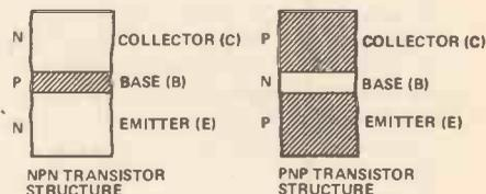
Figure 13. NPN and PNP transistor constructions.
