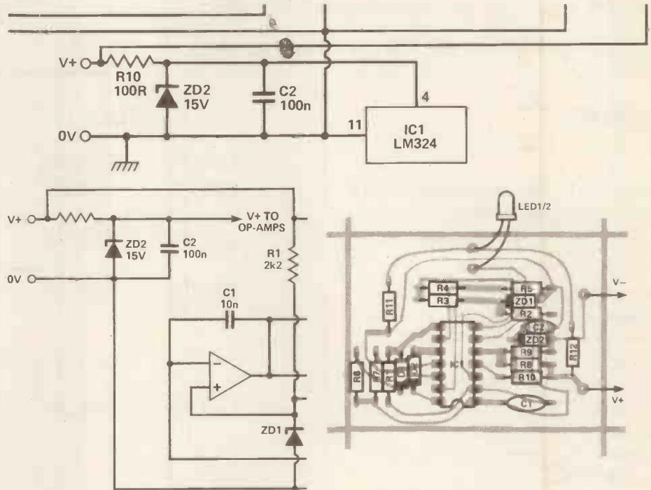
The diagrams show the correct details from Figure 1 (above) and Figure 2 (below left), and the whole of Figure 3, the component overlay, with R12 added.
