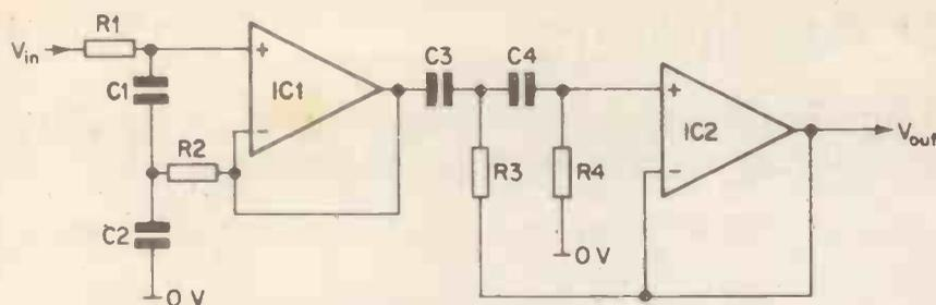
Figure 17. A two stage bandpass filter.
