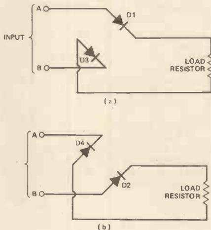
Figure 10: a) what occurs during the positive half cycle of input sine wave b) what occurs during the negative half cycle.
