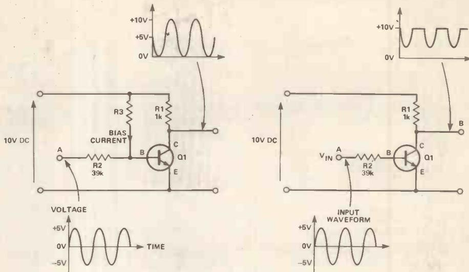
Figure 21. Attempting to use the circuit of Figure 20 to amplify a AC sinewave.
