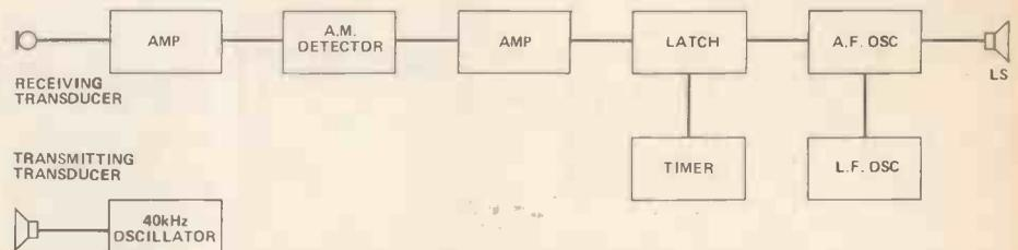
Figure 1. The block diagram, showing the transmitting and receiving stages.
