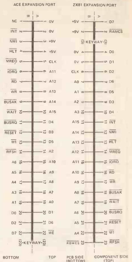
Figure 3. The ACE pins have been re-numbered according to the convention used for the ZX81.
