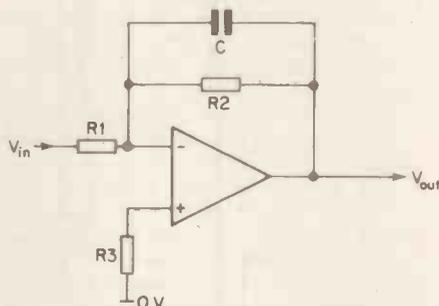
Figure 9. Simple op-amp low pass filter.
