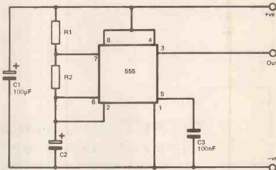
Figure 1. The trusty 555 geared up as an astable oscillator.
