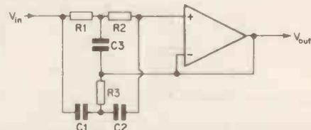
Figure 21. The high Q notch filter.
