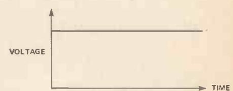
Figure 8. Output voltage of a cell is a very smooth DC.
