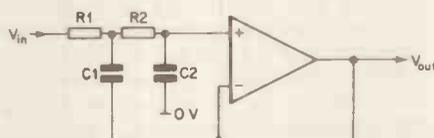
Figure 10. The classical filter gives a sharper cutoff.
