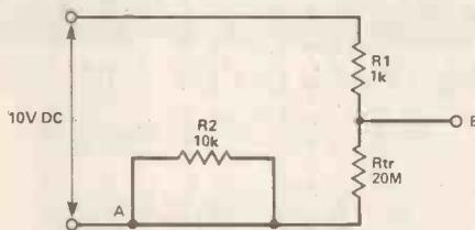
Figure 2. Equivalent diagram of a single transistor inverter with logic 0 at point A.
