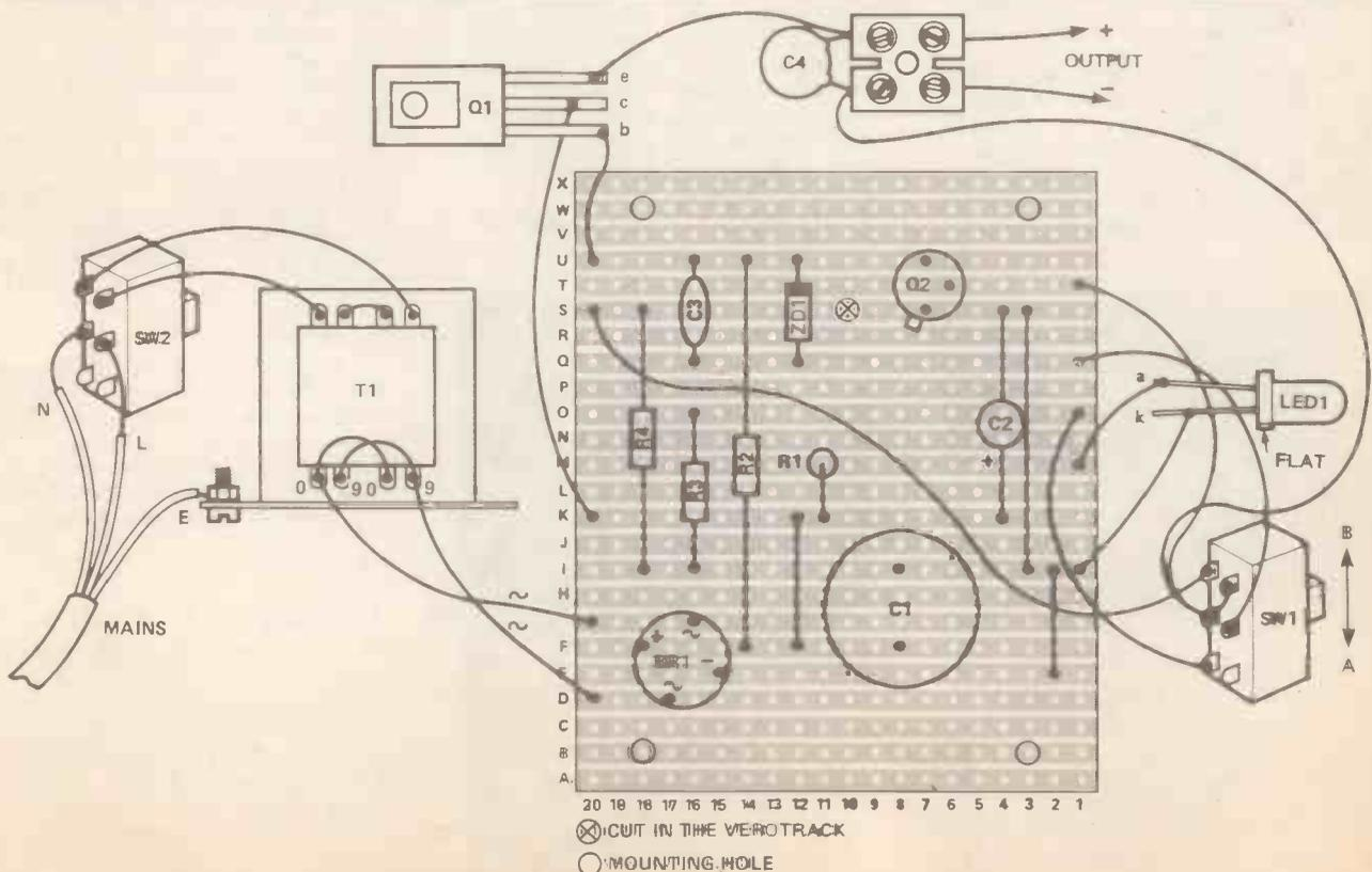
Figure 2. A small piece of Veroboard mounts most of the components, but there is a lot of off-board wiring.
