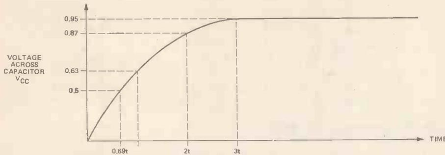
Figure 15. Important points on the exponential curve of a charging capacitor.
