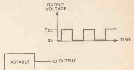
Figure 17. Block diagram of an astable.
