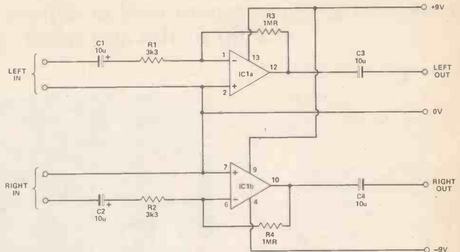
Figure 1. The circuit: a simple stereo preamp used for boosting a magnetic cartridge.
