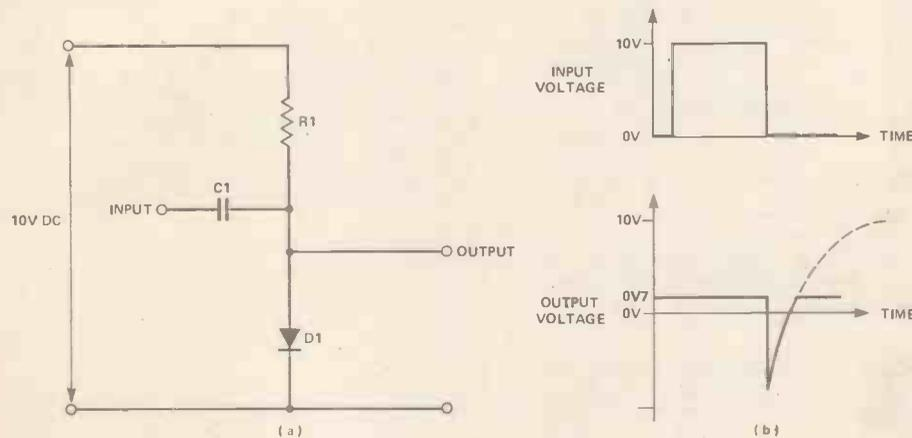
Figure 16a) Resistor/capacitor/diode (RCD) circuit b) Operating voltages of the RCD circuit.
