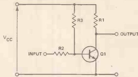
Figure 19. AC current amplifier formed by a single transistor.
