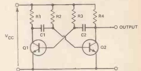
Figure 18. Astable formed by two transistors and two RCD circuits. The diodes of each RCD circuit are formed by the base-emitter junction of the transistors.
