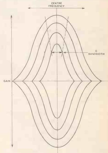
Figure 3. This graph shows a few of the infinite variety of response curves that the Para-Q can generate. There are three variables: the centre frequency can be positioned anywhere between 50Hz and 11kHz; the gain at that frequency can be varied by  $\pm 20dB$ ; and the Q or bandwidth of frequencies effected can range from 1 to 25, giving boost or cut over a very narrow range or over a wide band of frequencies.
