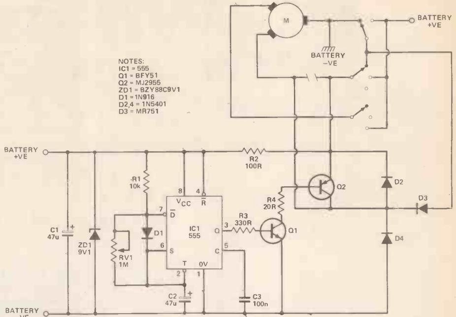
Figure 2. The circuit uses a 555 timer in the astable mode to provide the delay function. The unit is connected into the slow speed wiper circuit at the points indicated by the breaks.
