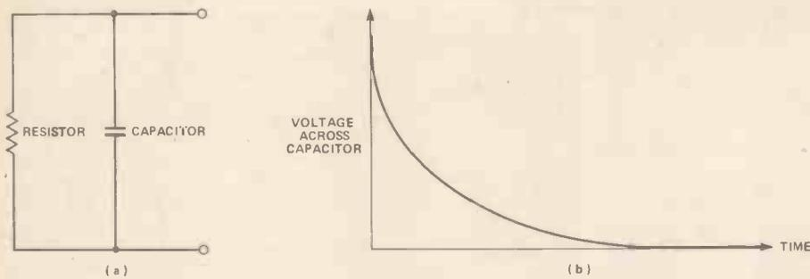
Figure 14. Discharging a charged capacitor through a parallel resistor.
