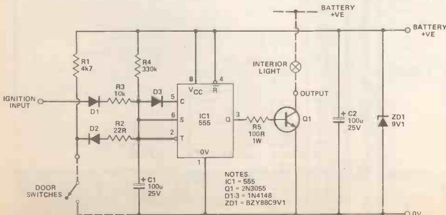
Figure 1. The circuit is based on a 555 used as a comparator.
