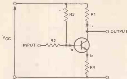
Figure 20. Common emitter amplifier with feedback.
