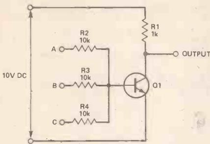
Figure 6. A single transistor, three-input NOR gate.
