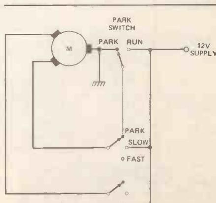
Figure 1. The wiper control circuit shown is conventional on most makes. The Delay unit is installed in the 'slow speed' circuit, but slow wipe is still possible by turning the delay to zero.
