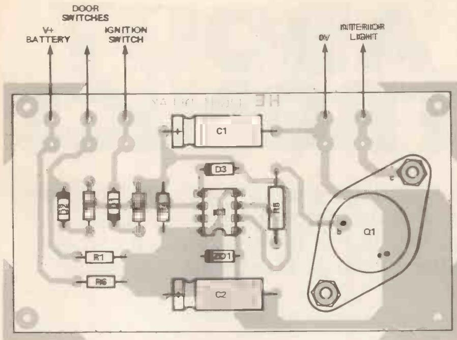
Figure 2. The PCB is compact, for easy installation.
