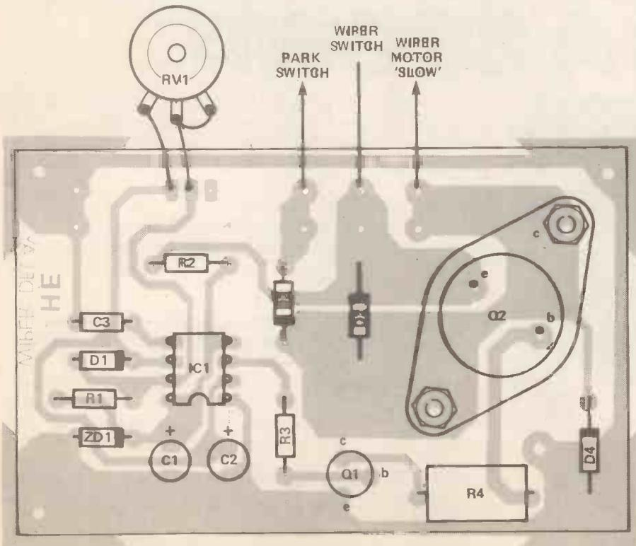
Figure 3. All components are mounted on the PCB except the control potentiometer, which can be mounted on the dashboard or steering column.
