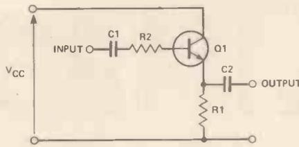
Figure 22. Common collector amplifier (emitter follower) formed by a single transistor.
