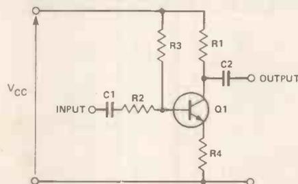
Figure 21. Common emitter amplifier with feedback and DC blocking capacitors.
