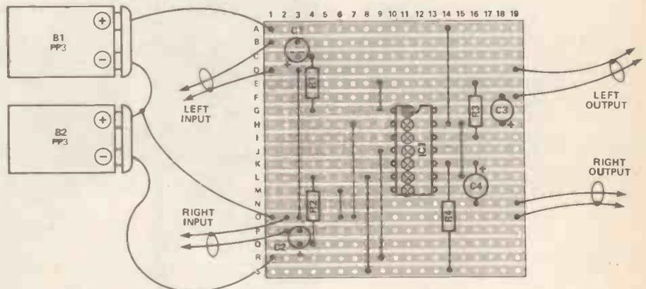
Figure 2. Careful use of screened cables for all inputs and outputs when constructing the Veroboard will keep undue noise out of the system.
