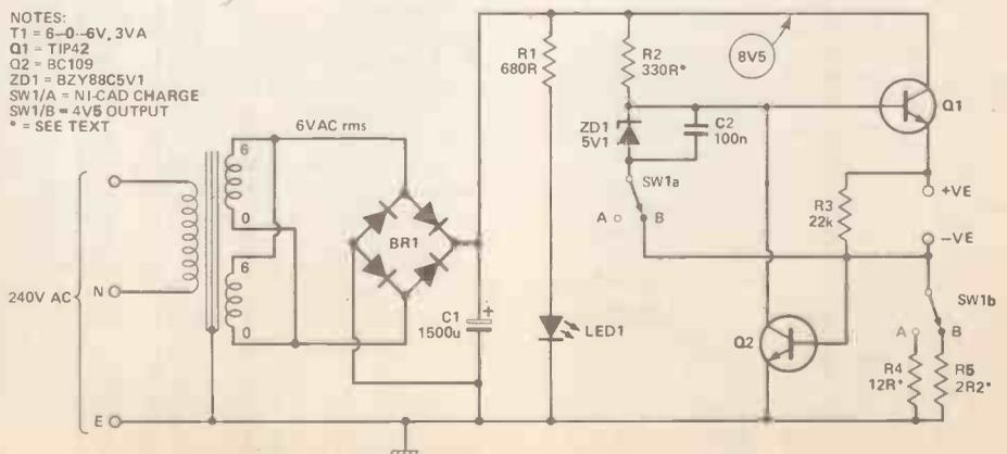
Figure 1. The values for current limiting resistors R4 and R5, must be calculated from the formula given in the text.
