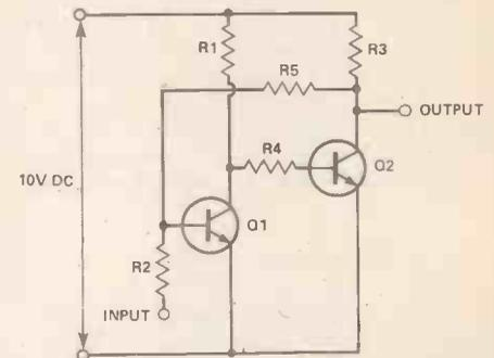
Figure 9. A two-transistor bistable formed by connecting the output of the first to the input of the second.
