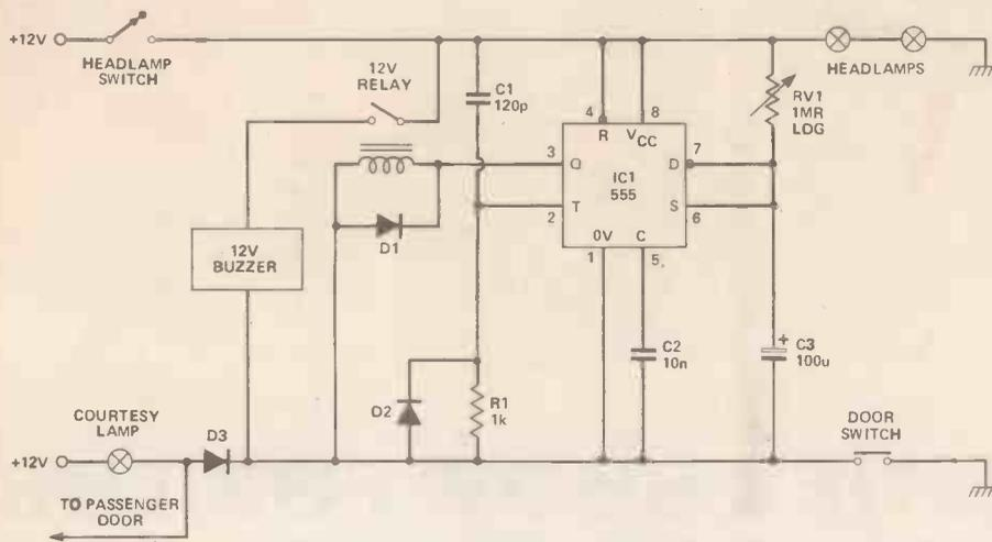
THIS little circuit switches on a 12V buzzer when a car's lights are accidentally left on and the door opened, but then switches it off after a predetermined time (to avoid embarrassing incidents when the Highway Patrol opens your door as you are saying Goodnight to your girlfriend!).
