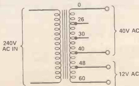
Another solution is to use two transformers: one 0-12V @ 100mA and one 20-0-20V @ 1A or 2A as required.
