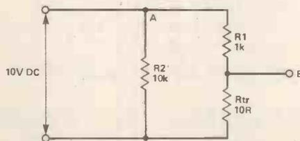
Figure 3. Equivalent diagram of a single transistor inverter, this time with logic 1 at point A.
