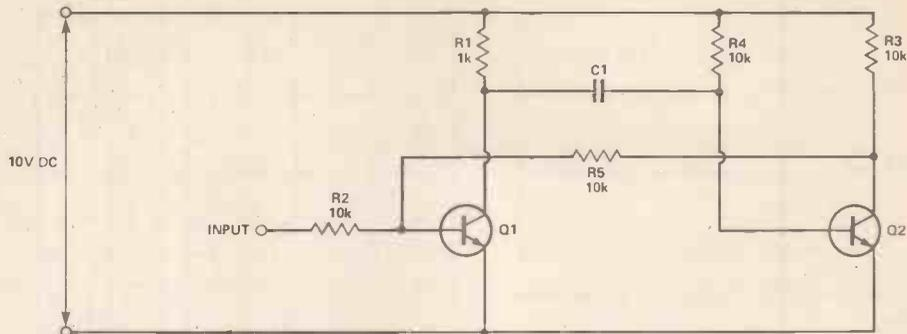
Figure 11. Monostable formed by two transistors connected by a capacitor.
