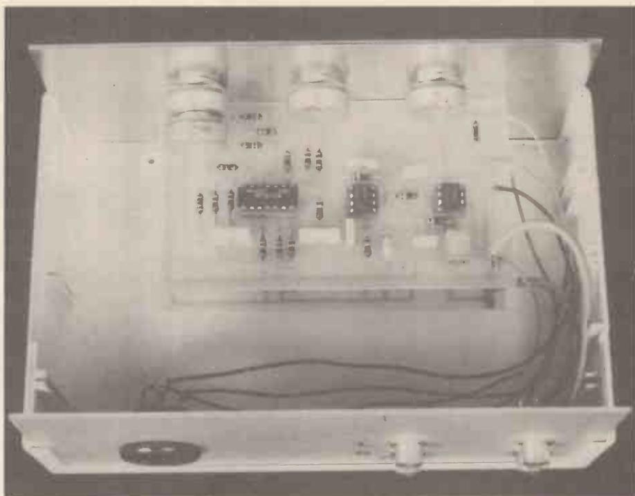
be screened within the housing of the equaliser, ie from the point marked 'output' on the overlay to the output socket.
