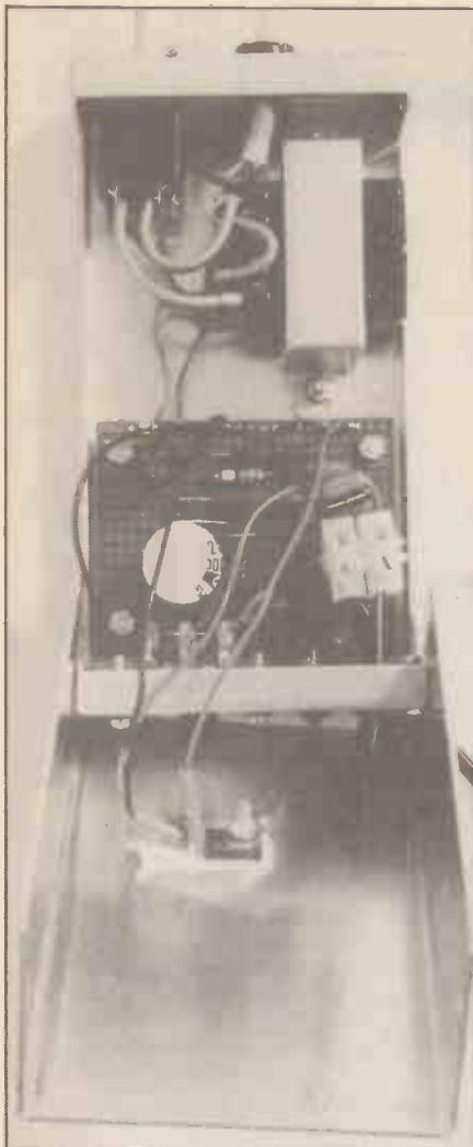
Careful construction is required when working with mains voltages, as usual. The output transistor, Q1, is mounted on the lid of the plain aluminium case, but isolated from it by a TO126 mounting kit; note the use of sleeves on the leads to this transistor.
