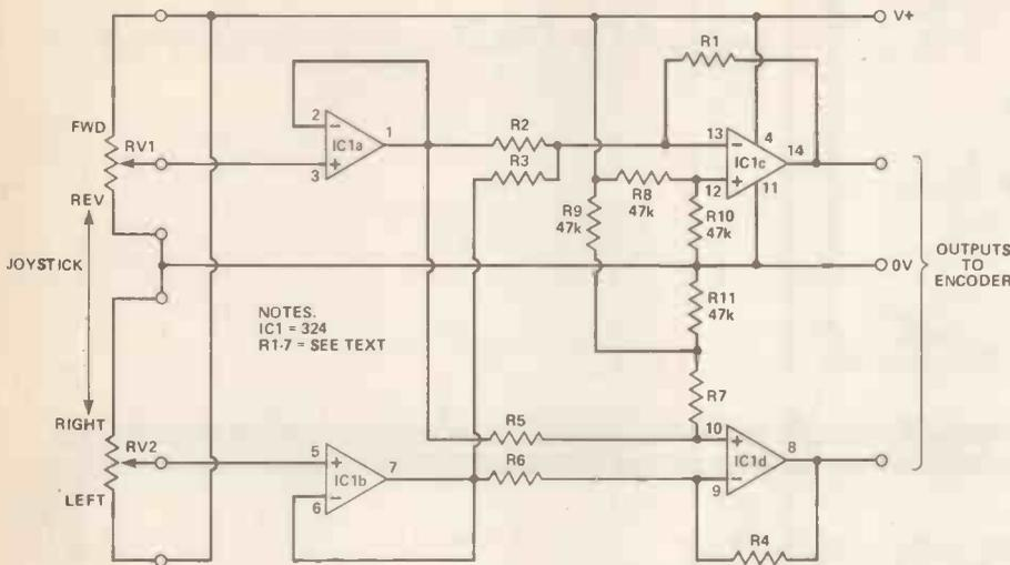
THIS mixer was designed to be fitted to a radio control transmitter to allow a tracked vehicle (eg a tank) to be controlled from a resistive joystick controller.
