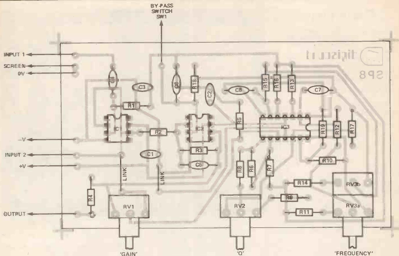
Figure 2. The printed circuit board accommodates the components for a single channel of equalisation. Two boards are required for the full stereo facility (see internal picture, next page) or any number can be connected in series using the series input (labelled input 2 in the diagram above).
