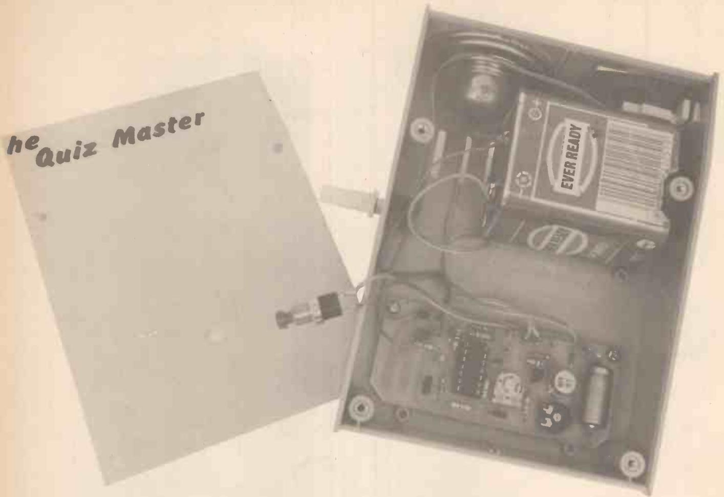
Figure 6. Internal wiring of the Quizmaster.
