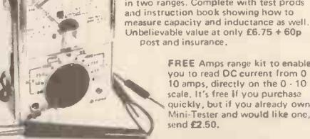
Continuity and resistance 0 - 1 meg ohms in two ranges. Complete with test prods and instruction book showing how to measure capacity and inductance as well. Unbelievable value at only £6.75 + 60p post and insurance.
