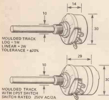
**Moulded Carbon Track:** The usual potentiometer chosen for panel mounting in non-critical applications. Also available with DPST switch rated for mains voltage (bottom).
