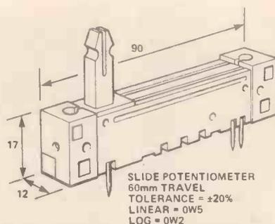
**Slide Potentiometers: Favoured for application where controls are being operated continuously.**
