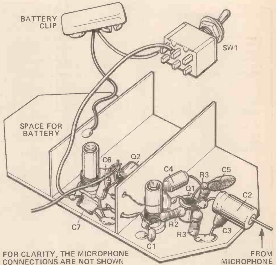
Figure 5. The construction diagram. The "up in the air" construction needs care to ensure that leads are not cut too short and that short circuits do not occur. It is not as hair-raising as it looks, however — and it is a technique worth practising.
