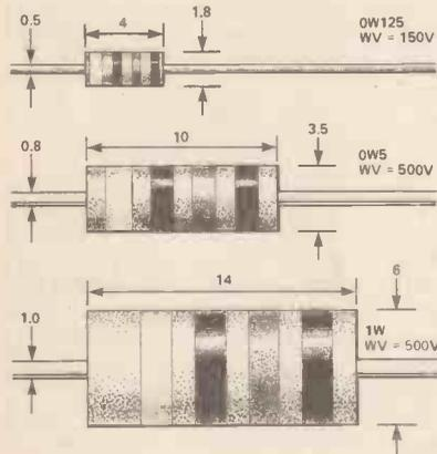
**Carbon Composition: Older type resistor, for general use where temperature coefficient and tolerance not critical; noise levels generally greater than 2uV/V. Carbon comp resistors are not usually available in values below 10R.**
