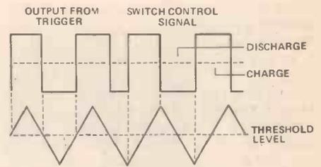
Figure 2. Generating a square wave from a triangular signal is quite easy. As shown in the block diagram (left), a trigger circuit is used to square the triangle (which is easier than squaring a circle) by switching rapidly between full positive and negative voltages whenever the triangle wave passes through a certain threshold voltage.
