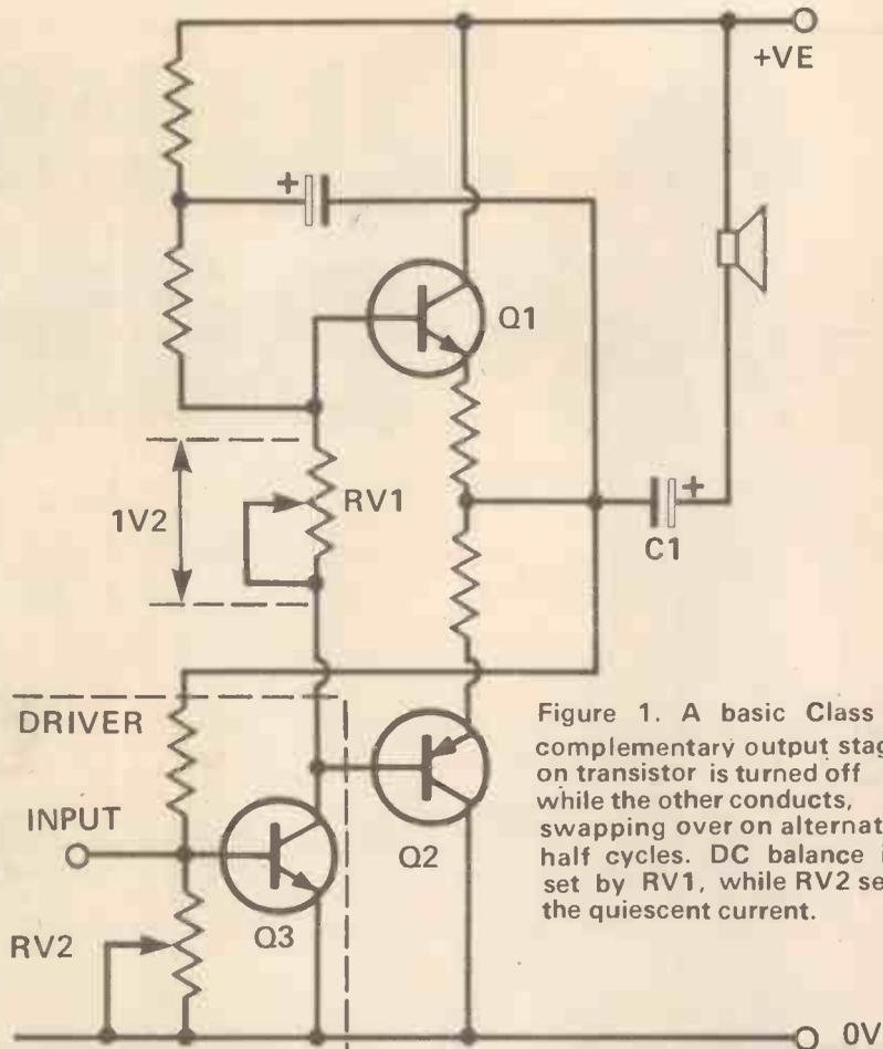
Figure 1. A basic Class B complementary output stage; on transistor is turned off while the other conducts, swapping over on alternate half cycles. DC balance is set by RV1, while RV2 sets the quiescent current.
