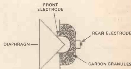
Figure 9. The principle of a carbon granule microphone used in a telephone handset: as the two electrodes move closer together the resistance between them decreases, reducing the voltage across them.
