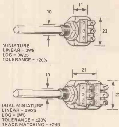
**Miniature or "Midget":** Carbon track potentiometers for general purpose. Dual (aka 'tandem' or 'ganged' pots) have closely matched tracks.
