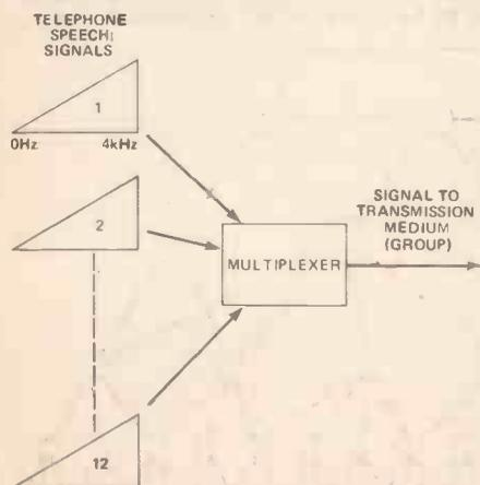
Figure 13. Twelve separate telephone speech signals multiplexed into a single group, for transmission over a single medium.
