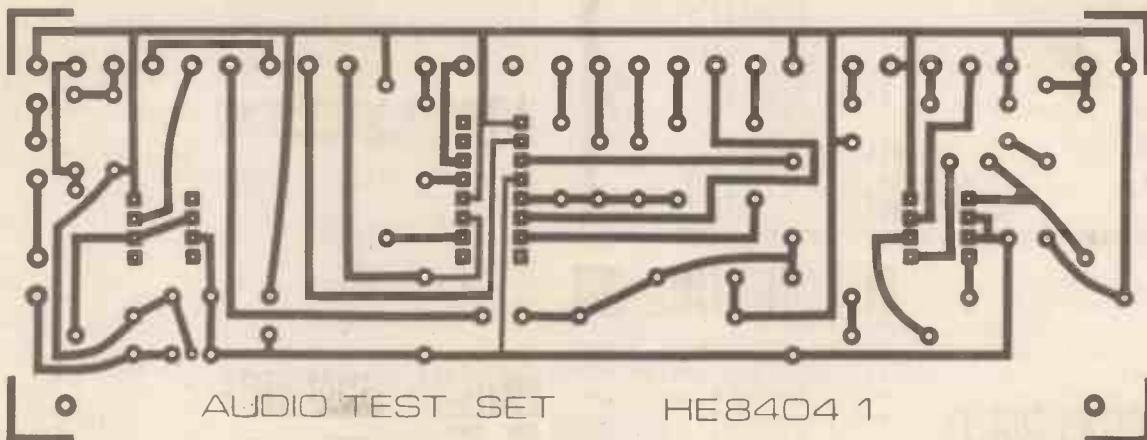
The PCB mask for the Analogue Test Set.
