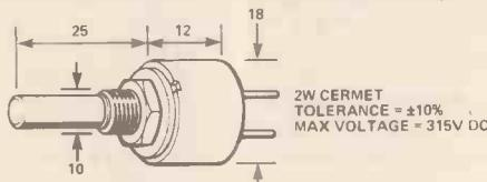
**Rotary Cermet: The cermet track provides good electrical and temperature stability, and linearity.**
