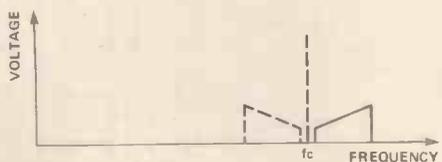
Figure 21. The spectrum of a single sideband AM signal, obtained by filtering out the carrier signal and lower sideband (shown in broken lines), leaving only the required upper sideband.
