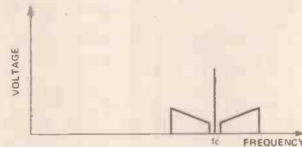
Figure 18. The possible spectrum of an AM telecommunications signal, generated by the system in figure 15, above.
