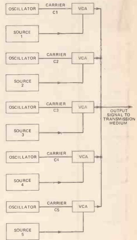
Figure 19. Five AM signals, frequency division multiplexed onto a single transmission medium.
