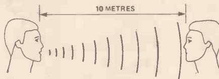
Figure 7. If the bandwidth of the air (transmission medium) is wide enough, the noise level low enough, and the attenuation low enough, the listener (receiver) will hear the speaker (source).
