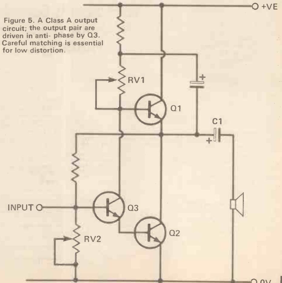
Figure 5. A Class A output circuit; the output pair are driven in anti-phase by Q3. Careful matching is essential for low distortion.
