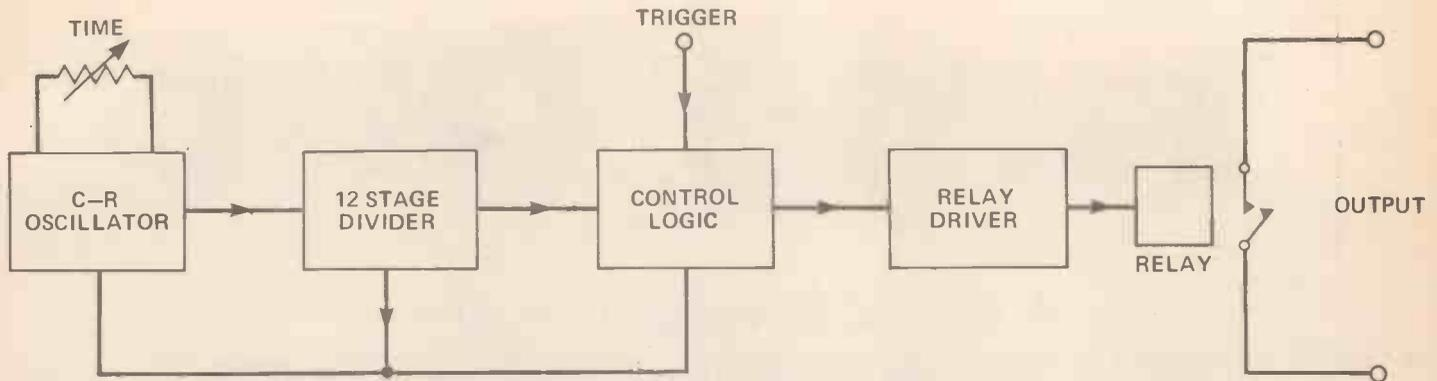
Figure 2. The block diagram shows the internal blocks of IC2, a ZN1034E, on which the Timer is based.
