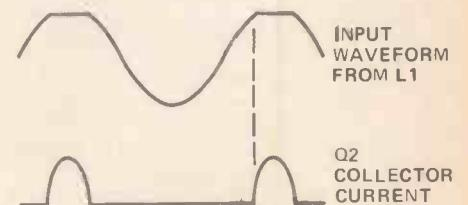
Figure 3. Waveforms for the operation of Q2 in class C.
