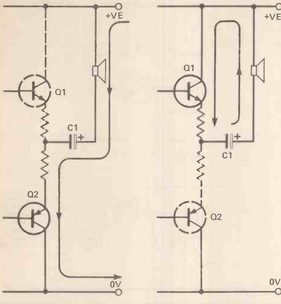
Figure 2 (left). When Q2 conducts (Q1 cut off), C1 charges through the loudspeaker and Q2.
