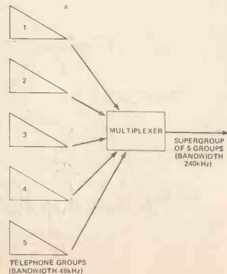
Firstly, as the bandwidth of a twisted-pair cable is quite low (about 0Hz to 5kHz) many thousands of such cables would be needed for the many thousands of links between telephone exchanges. Figure 11 gives some idea of the organisation of the UK telephone system and the approximate number of exchanges. If all these transmission paths were to be made using twisted pair cables then an almighty number and quantity of cables would be required.
