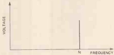
Figure 17. The spectrum of a carrier of frequency  $f_c$ .
