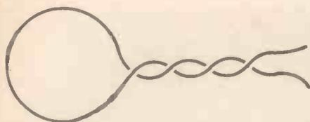
Figure 4. The coupling link should be wound quite loosely and cut to length without placing tension on the link (1½ — 2in).
