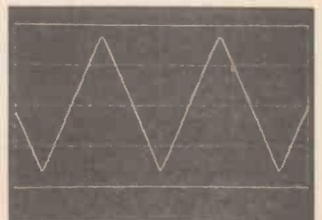
waveform. The sinewave signal is obtained by connecting a resistor (R6) between pins 13 and 14 of IC1.
