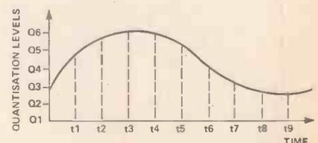
Figure 25. Digitising an analogue linear signal by sampling it and taking the value of the quantisation level which the signal is nearest to at each sampling (see overleaf).
