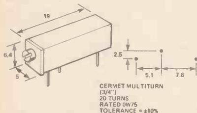
**Cermet Multiturn Presets: Essential for precision adjustment. A large range of single-turn cermet trimmers are also available, eg square, vertical, horizontal and round.**
