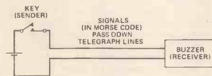
Figure 1. A simple telegraph system, illustrating the principle of communication: a sender (the key); a receiver (the buzzer) and an agreed code (Morse code).
