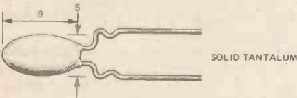
**Tantalum Electrolytic:** Preferred for accuracy in eg timing, filter circuits. They have very low leakage currents and good stability, but cannot withstand reverse voltages.
