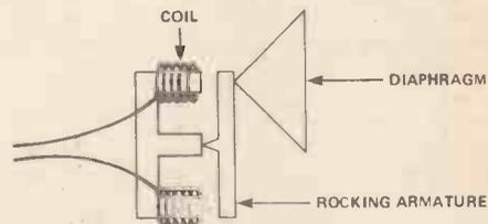
Figure 10. A telephone-type earphone. The input electrical signal from the microphone, which corresponds to the speech, causes a magnetic field around the coils. This attracts and repels the rocking armature, which therefore moves as the signal varies. The consequent movement of the diaphragm creates sound waves.
