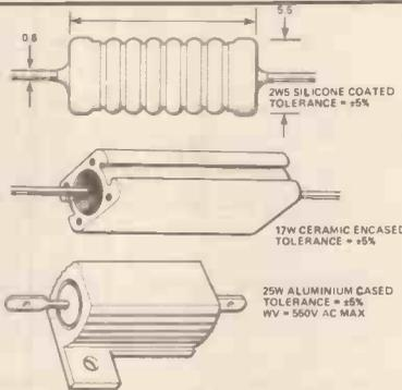
**Wire wound: Silicone coated types (top) suitable for general use up to 10W rating. Ceramic encased (middle) types are useful where high insulation resistance is needed (eg mains circuits); also supplied at 4W, 7W and 11W ratings. Aluminium-clad resistors (bottom) will rarely be used by the home constructor!**
