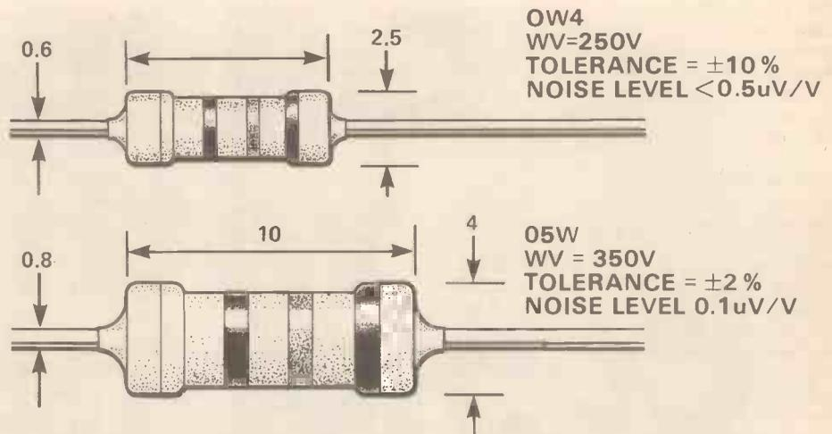
**Metal Film:** General purpose high stability types with low temperature coefficient. Five-band colour code gives three significant figures, multiplier and tolerance.
