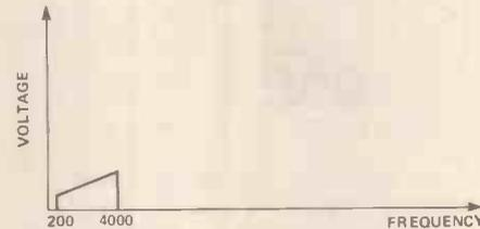
Figure 16. A typical spectrum of a telephone-style speech signal width bandwidth 200Hz to 4kHz.
