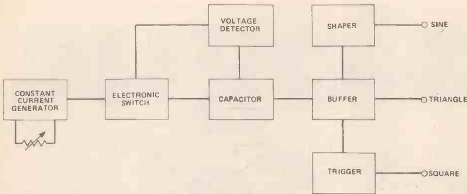
Figure 1. Block diagram of the function generator — all this on one chip!
