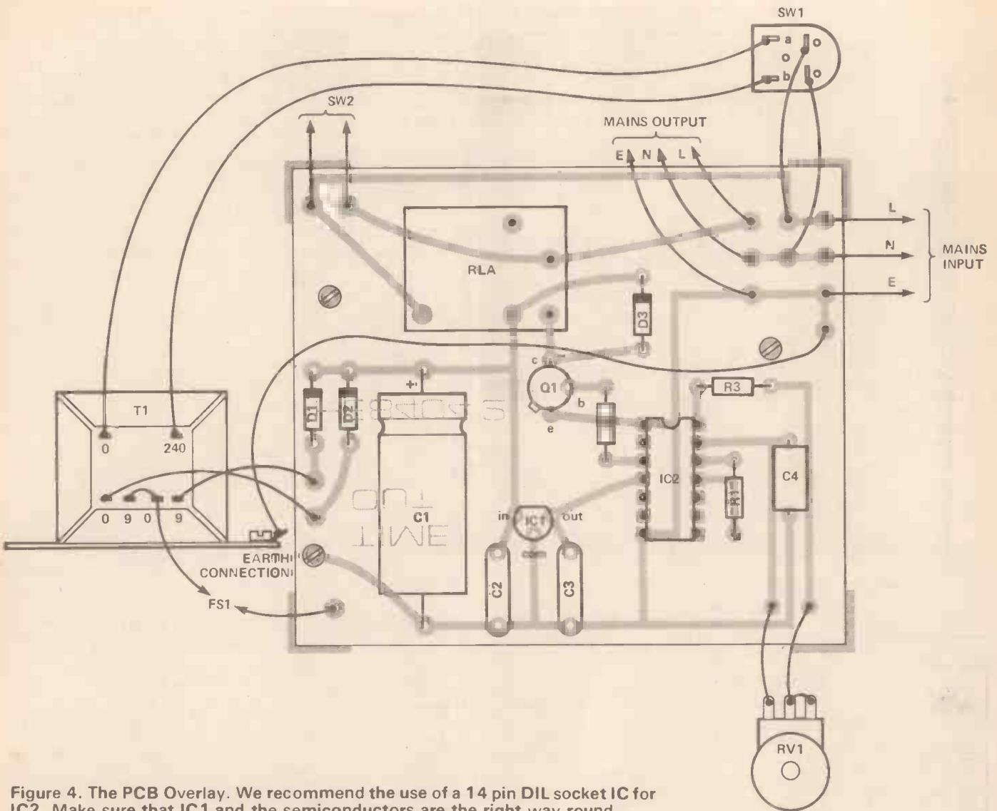
Figure 4. The PCB Overlay. We recommend the use of a 14 pin DIL socket IC for IC2. Make sure that IC1 and the semiconductors are the right way round.
