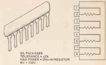
**SIL Package: Also available with 7 or 8 commoned resistors. As with DIL resistors, values are limited, and all resistors in the package are the same value.**
