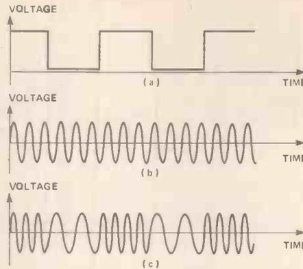
Figure 23. Signals within a typical FM telecommunications systems such as that of Figure 22: a) message signal (eg a squarewave); b) the carrier's centre frequency; c) the output signal to the transmission medium.
