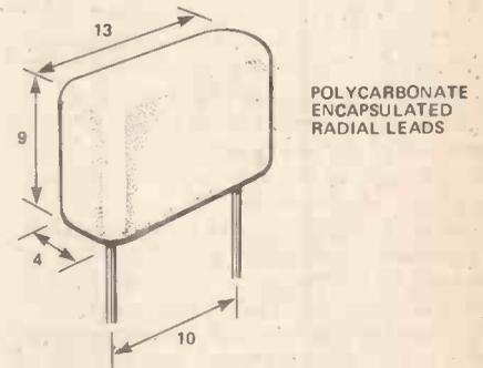
**Polycarbonate:** The material has better electrical characteristics than polyester and should be used, instead, in ore critical situations. A brass-encapsulated axial form is available for super-critical (eg high temperature) applications where price is of no concern!
