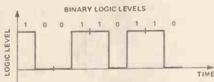
Figure 27. A pulse code modulated (PCM) signal corresponding to the first three sampled values of the linear analogue signal of Figure 26a.
