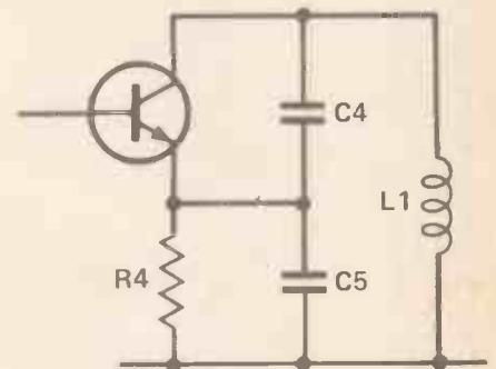
Figure 2. A diagrammatic layout of the oscillator stage.
