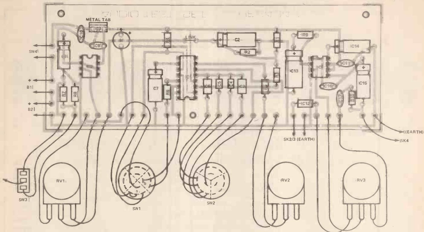
Figure 5. All components, with the exception of panel mounted controls, fit onto a single small printed circuit board (see page 64 for a full-sized foil pattern). Details of the connections from the PCB to the controls are also shown in the photographs below, and on the preceding page.
