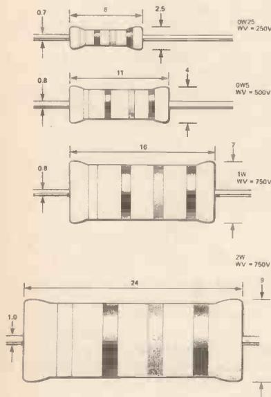
**Carbon Film:** The standard "1/4 watt 5% carbon" type, is has almost completely replaced older carbon composition resistors. Noise level is typically  $1.0\mu\text{V/V}$  for any value, which is adequate for most purposes.
