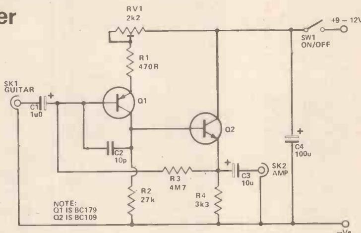
the required level, with maximum resistance of RV1 giving maximum feedback and minimum gain. Capacitor C2 rolls off the frequency response of Q1 at high frequencies outside the audio range, and this helps to avoid problems with instability and radio frequency breakthrough.
