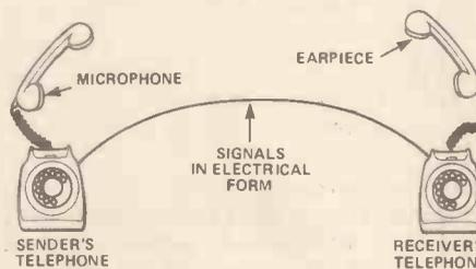
Figure 2. The telephone as a communications system.
