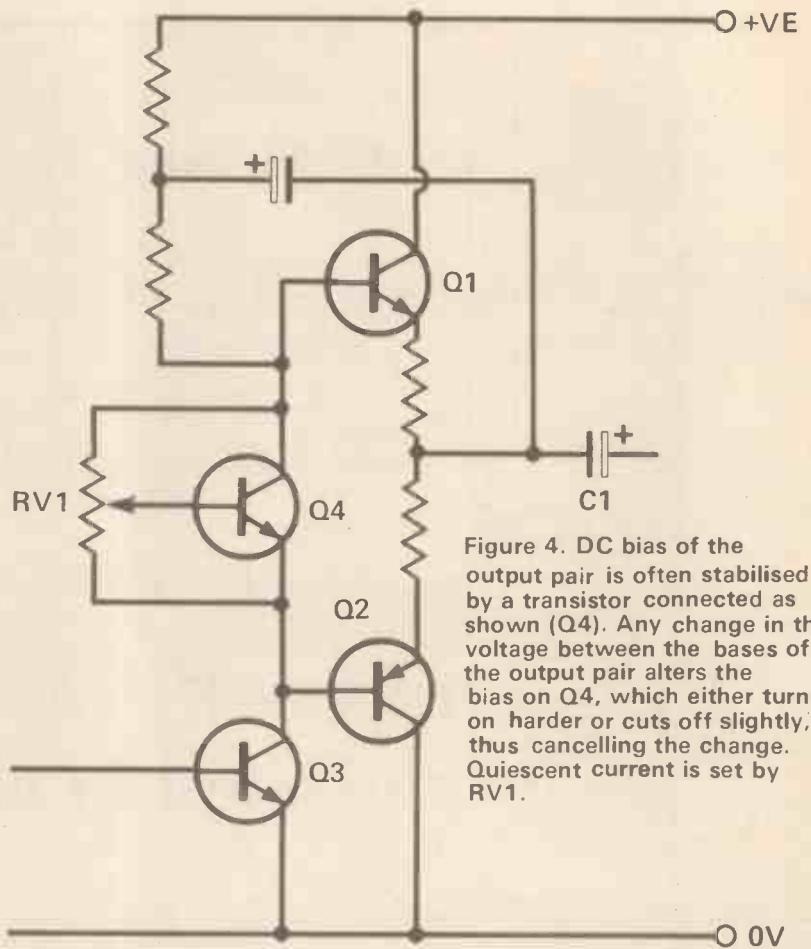
Figure 4. DC bias of the output pair is often stabilised by a transistor connected as shown (Q4). Any change in the voltage between the bases of the output pair alters the bias on Q4, which either turns on harder or cuts off slightly, thus cancelling the change. Quiescent current is set by RV1.
