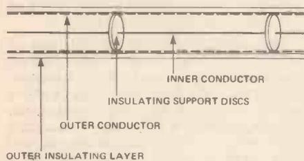
Figure 12. The construction of coaxial cable, with one conductor concentric with the other and insulated from it.
