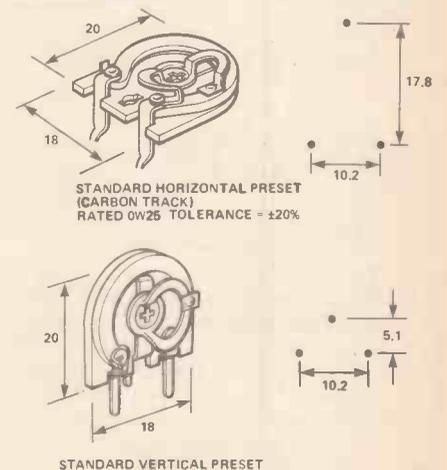
**Standard Horizontal Preset (top):** miniature types have pin spacings of 10.2 and 5.1mm in the same pattern.
