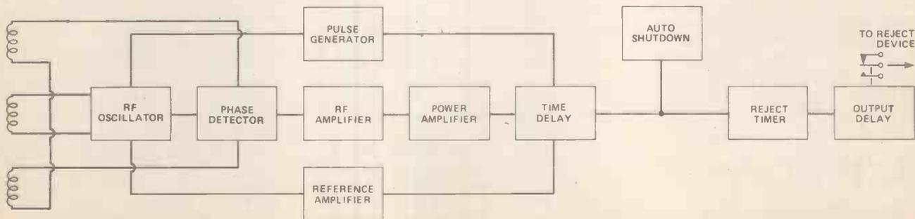
Figure 5. The Balanced Coil method, a simplified version of Induction Balance, favoured for "production line" detectors because it is very sensitive at speed.
