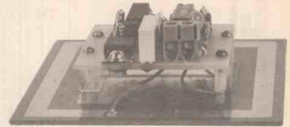
switches as used at the top and bottom of staircases. Don't forget to switch off your house lighting circuit at the mains first, and ensure that you get the neutral and live connectors the right way round! A glowing electrician's neon screwdriver can be used to locate the live side. The bulb must be of course be in circuit with the mains power on for this test.
