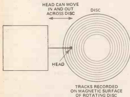
Figure 5. Principle of a magnetic disc memory system. Large capacity systems are possible with a fast access time compared to magnetic tape.
