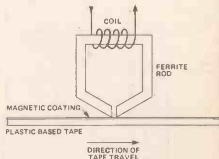
Figure 4. Principle of operation of a magnetic tape memory system. An electric current through the coil produces a magnetic field which is stored on the magnetic surface of the tape. On playback the stored information creates a current through the coil which can be amplified.
