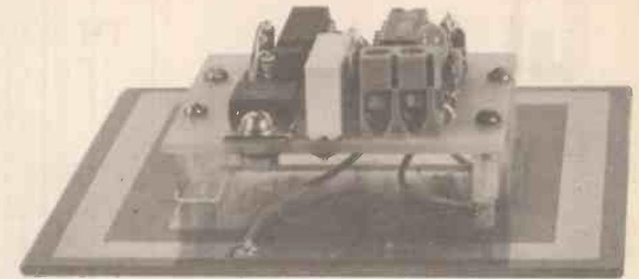
switches as used at the top and bottom of staircases. Don't forget to switch off your house lighting circuit at the mains first, and ensure that you get the neutral and live connectors the right way round! A glowing electrician's neon screwdriver can be used to locate the live side. The bulb must be of course be in circuit with the mains power on for this test.
