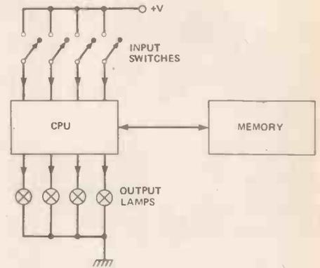
Figure 2. A simple computer system using four switches as input devices and four lamps as output devices.
