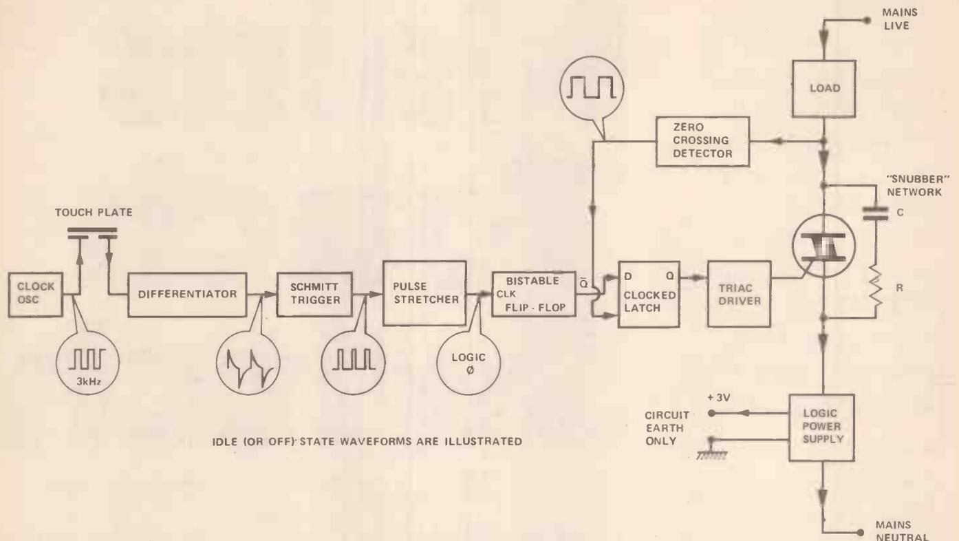
Figure 1. The complex block diagram of the mains touch switch.
