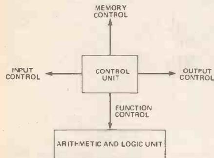
Figure 6. The main sections of a central processing unit (CPU).
