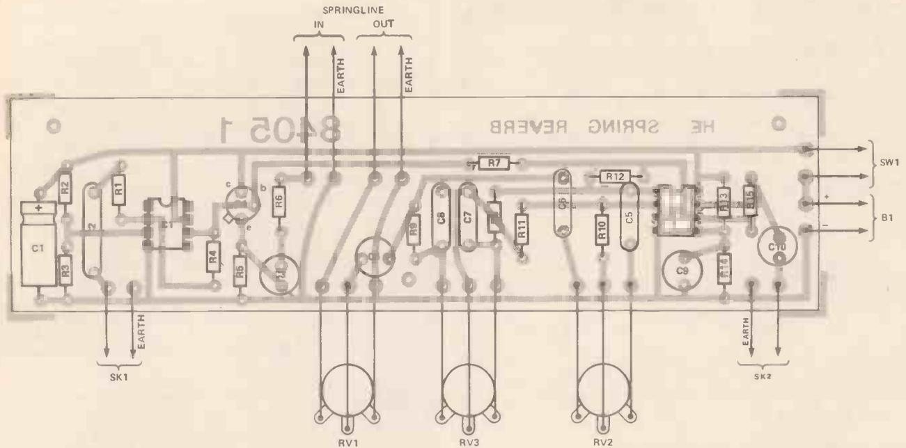
Figure 3. The PCB foil and overlay. The connections at bottom go to the controls, those at the top go to the small springline unit, which occupies more than half the case (see the picture on the previous page).
