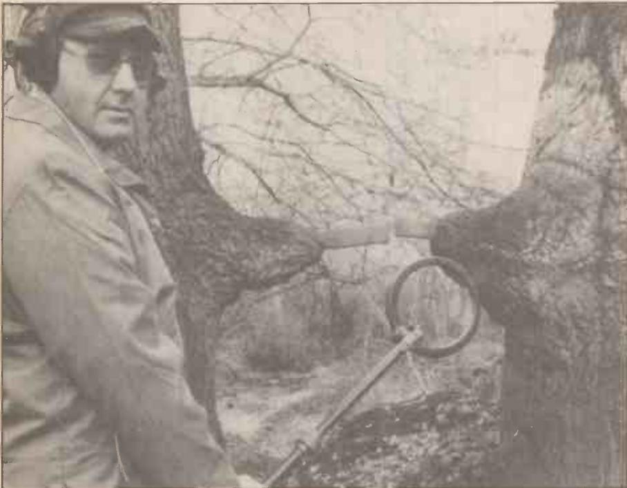
The Autopulse hand-probe is used to locate the exact position of a bracing bar before carrying out tree surgery.
