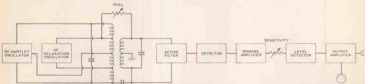
Figure 4. Induction Balance, the oldest and most sensitive method of detection, is now not much used because of its complexity.
