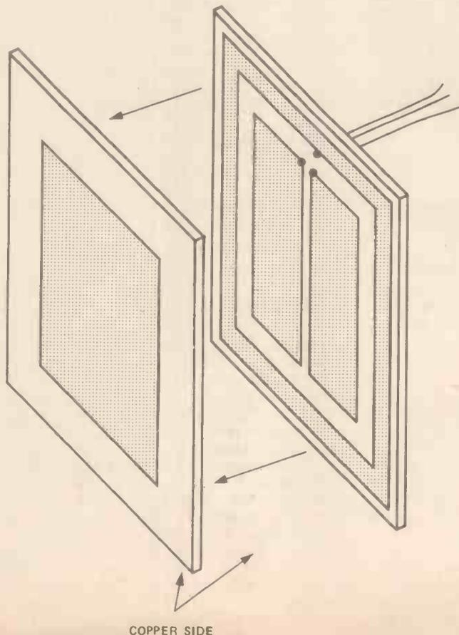
Figure 5. This diagram shows the construction of the Touch Switch from single, as opposed to double-sided PCB. Superglue or Araldite the two boards together as shown; drill small holes to let out the thin connecting wires to the other side of the board where it can be connected up to the circuit.
