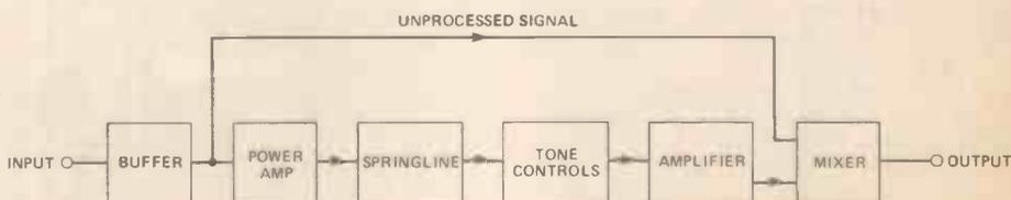
Figure 1. The block diagram showing the Springline in the complete system.
