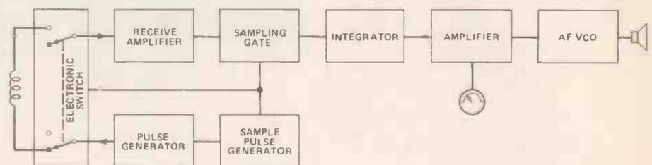
Figure 3. The block diagram of a pulse induction system. This method uses the ability of metal objects to absorb and reflect electromagnetic radiation as eddy currents which can be detected.
