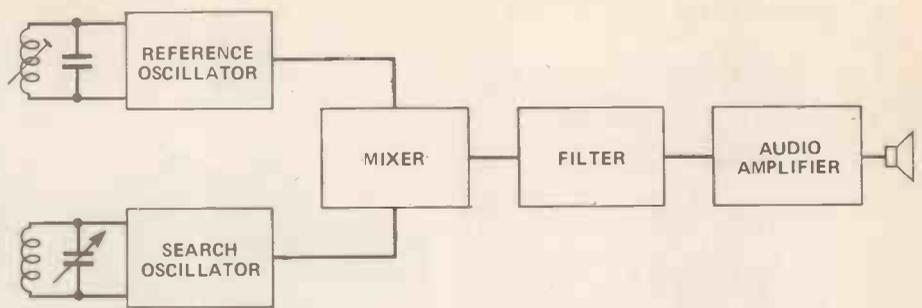
Figure 1. A block diagram for a Heterodyne Principle (BFO) detector, the simplest type for a home constructor to design.
