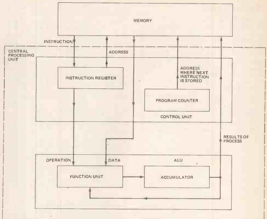
**Figure 8.** A block diagram of a whole central processing unit, complete with ALU, instruction register and memory.
