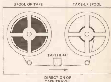
Figure 3. A magnetic memory system. Such an auxiliary memory has a large capacity but a slow access time.
