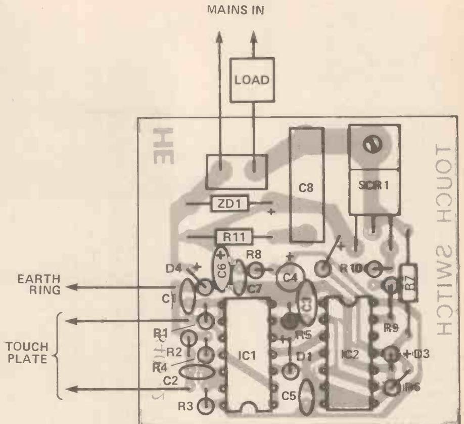
Figure 4. The component layout. There are many polarity components, so component orientation should be double-checked before connection.
