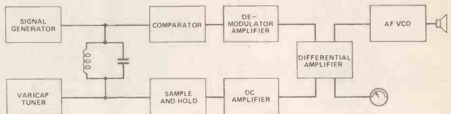
Figure 2. The Off Resonance Discrimination system. Very selective, this method is favoured by "treasure hunters".
