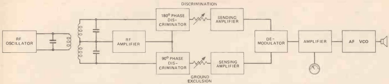
Figure 6. A block diagram for the Transmit-Receive Radio Technique, popular for its simplicity and ability to discriminate between worthless and valuable metals.
