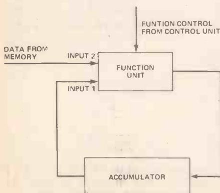
Figure 7. Inside an arithmetic and logic unit (ALU). The accumulator is a single-number store, or register.
