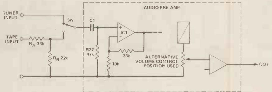
**Figure 6.** One possible application of the control amp: using the alternative volume control position, for recording say from a VCR and radio tuner at the same time.
