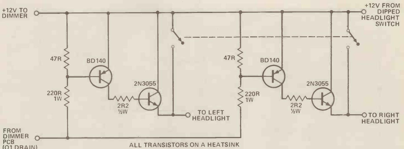
Figure 2. An experimenter's circuit for those wishing to try other applications for the circuit, including possible headlight dimming.
