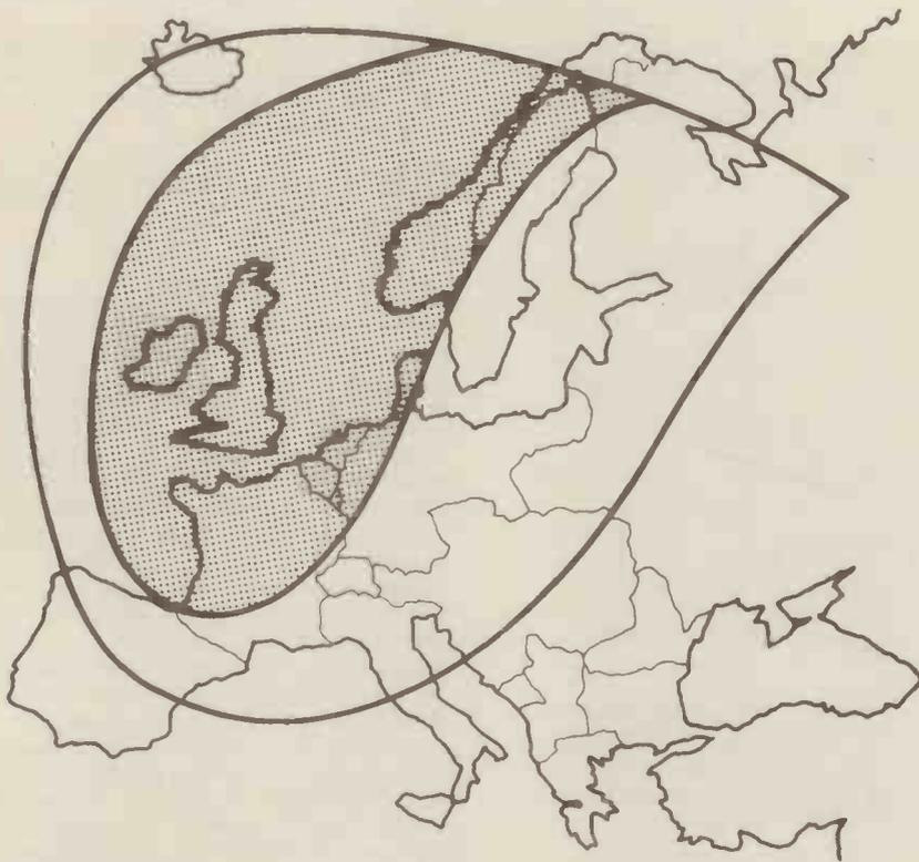
Figure 13. Footprint of the Direct Broadcast Satellite Service, which will be launched as a new television system.
