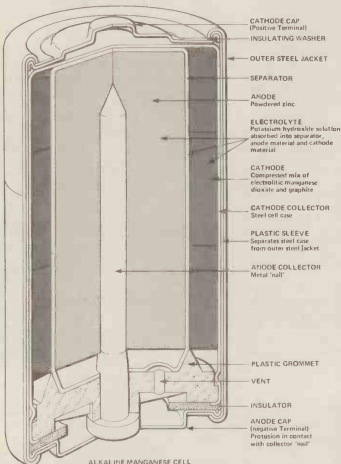
container is used which, unlike the zinc container of the zinc carbon cell, does not take part in the chemical process of producing current, so does not tend to perforate in use. It also provides a stronger and more leak-proof container. A metal central current collector — the nail — is in direct contact with the anode.
