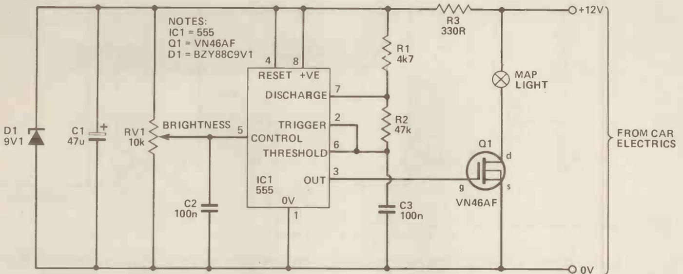
Figure 1. The circuit. The dimming is obtained by a rapid switching of the lamp, controlled by the 555 timer.
