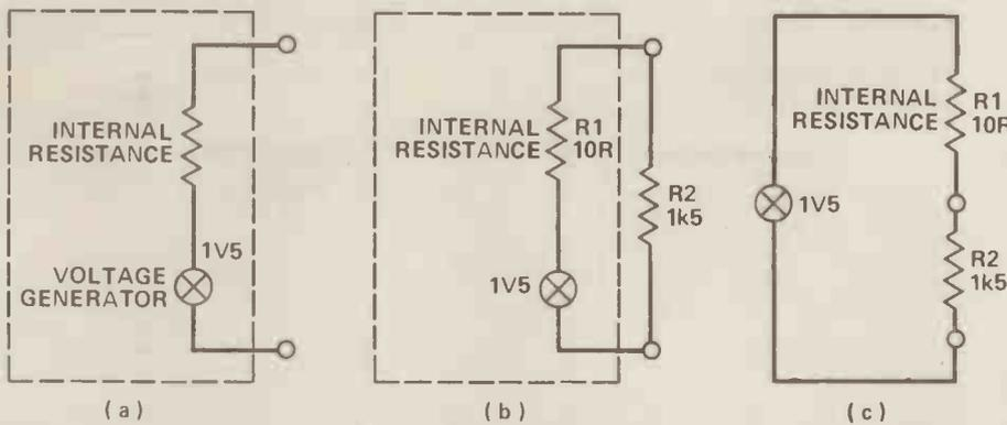
Figure 9a, b and c show the equivalent circuit (to Figure 8) of a 1V5 cell, showing internal resistance. For details see text.
