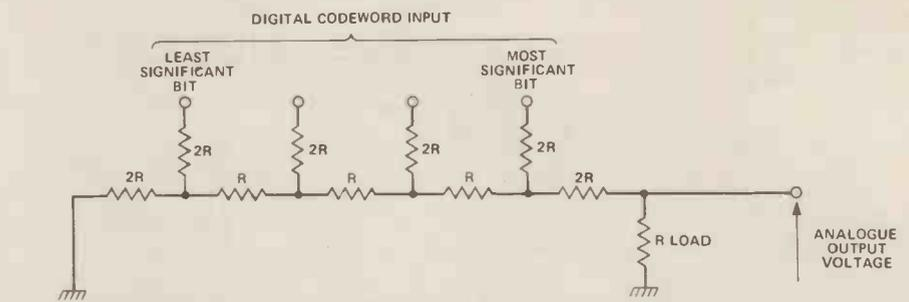
Figure 6. The R-2R resistor ladder type of DAC network.
