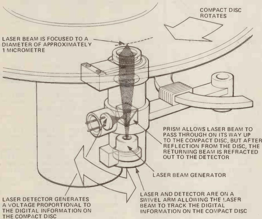
Figure 10. A low-power laser tracks the bottom surface of a digitally recorded compact disc.
