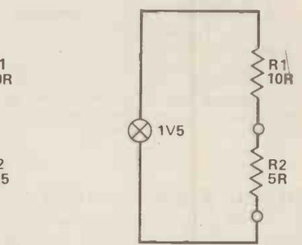
Figure 10. This shows how internal resistance affects operation in high current applications.
