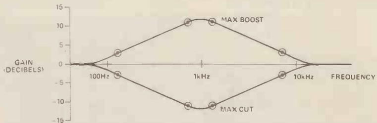
Figure 3. This diagram shows the boost and cut over the middle range of frequencies given by the middle tone control of the amplifier.
