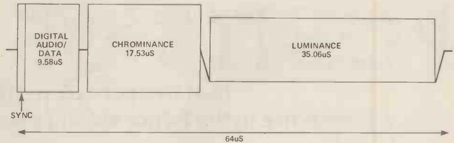
different method of transmission than the existing PAL colour system which we saw last month. DBS transmissions, in fact, are an ideal example of how digital and analogue concepts can be combined within a communications system. We shall look at DBS transmissions in detail.
