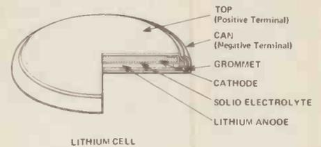
**Figure 14.** The construction of a lithium button cell.
