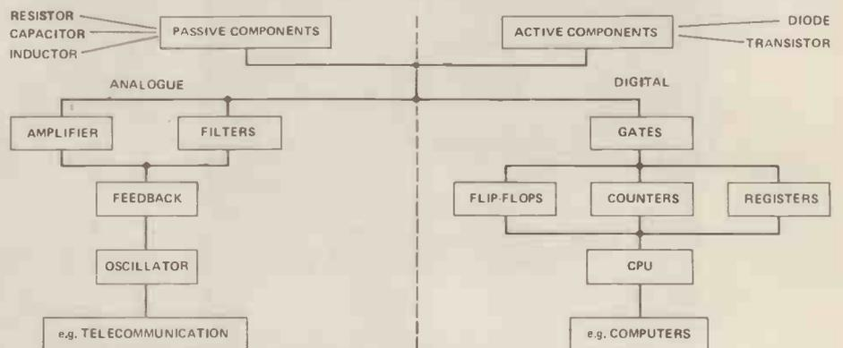
Figure 1. A 'family tree' of topics in electronics, all of which have been covered in past instalments of *All About Electronics*.
