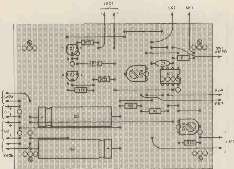
Figure 2. The PCB layout. If the CA 3140 is used, an IC socket is recommended. Note that resistors 2 to 7 are mounted on SW1 — see Figure 3.
