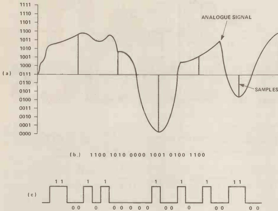
Figure 3. Pulse code modulations on an analogue signal, showing sampling and analogue-to-digital conversion.
