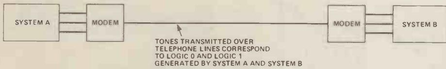
Figure 9. The use of a modem at each end of a telephone line allows digital systems to communicate in an analogue fashion.
