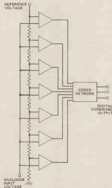
Figure 8. The parallel, or flash ADC which uses  $2^n - 1$  comparators.
