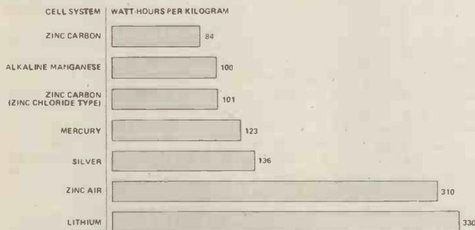
**Figure 15.** A graph showing a comparison of the capacities of various cell types with regard to their weight.
