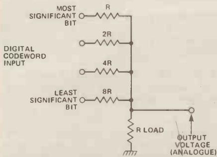
Figure 5. A binary weighted resistor network. This forms the basis of one of the simplest types of DAC.
