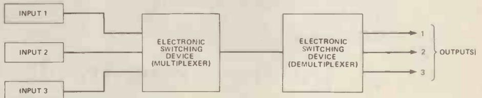
Figure 2. The principle of Time Division Multiplexing.
