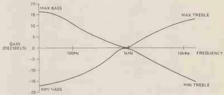
Figure 4. This diagram shows the boost and cut available over the bass and treble frequencies by the conventional Baxandall bass/treble tone controls.
