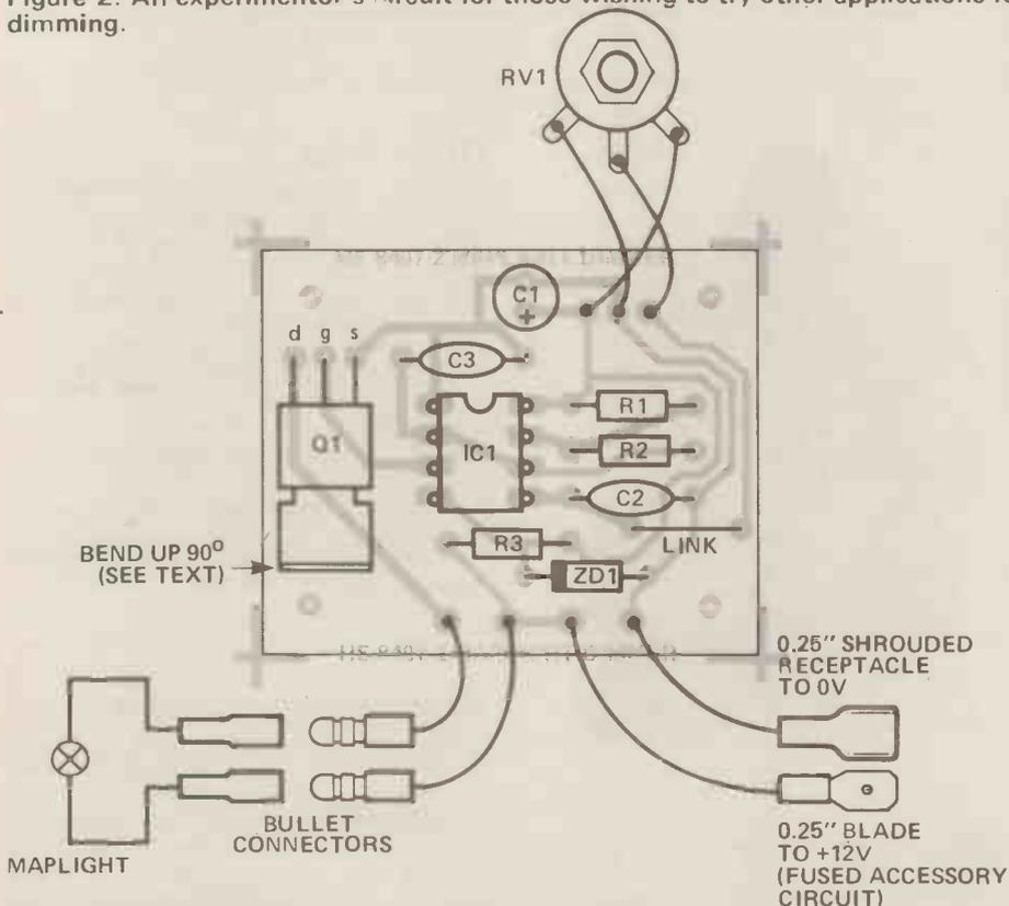
Figure 3. The PCB layout. Apart from the normal anti-static precautions, the only point to note is the careful bending-up of the heatsink tab on Q1.
