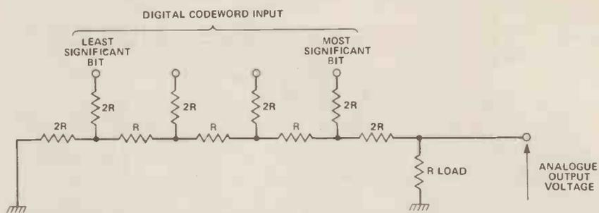
Figure 6. The R-2R resistor ladder type of DAC network.
