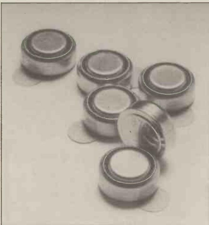
Zinc air cells (see previous page). Batteries tend to decay if they are stored for a long time without use. Zinc air cells are sealed until use, which gives them very long storage time. The seal is broken by pulling the tabs shown in the picture.
