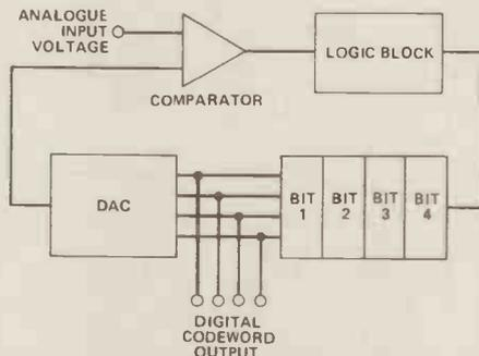
Figure 7. The successive approximation type of ADC.
