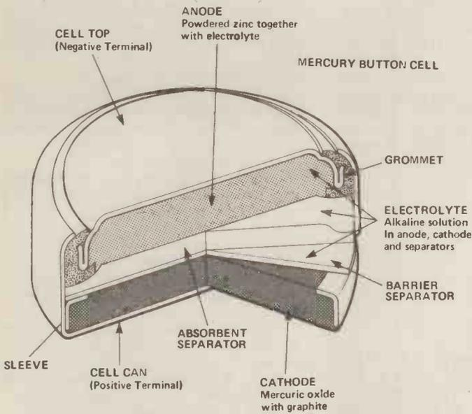
**Figure 13.** The construction of a mercury button cell. The silver button cell, and the zinc cell, are of similar construction.
