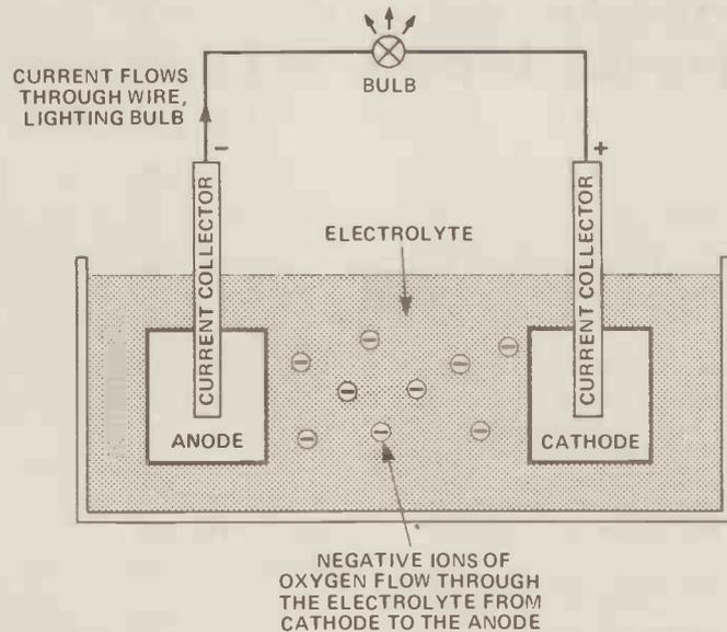
Figure 8. A basic cell in operation, in this case used to illuminate an electric light bulb.
