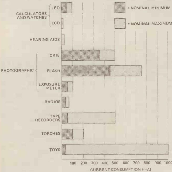
Figure 18. This graph shows the current consumption of some typical battery-powered devices. Typically, the more heat that is generated (as in the photographic flash) and the more moving parts the device has (as in the drive mechanism of a cine or tape recorder) the more expensive it is to run.
