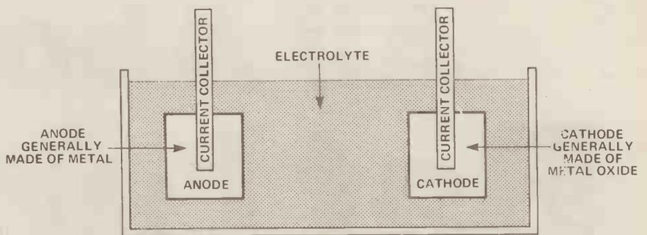
Figure 7. A basic cell, showing anode, cathode, and electrolyte.
