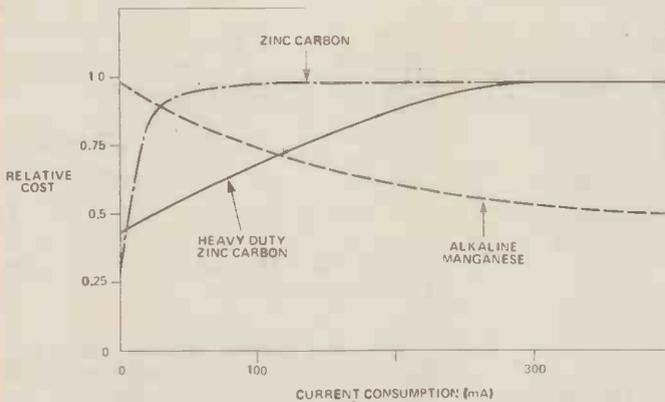
Figure 17. An interesting graph showing the relative costs of alkaline manganese, zinc carbon and heavy duty zinc carbon cells as a function of their current consumption.
