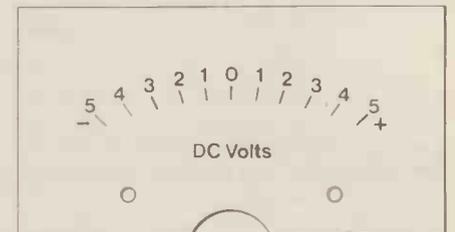
Figure 4. Cut out, or photocopy, this meter scale if you cannot obtain a suitable centre-zero meter.
