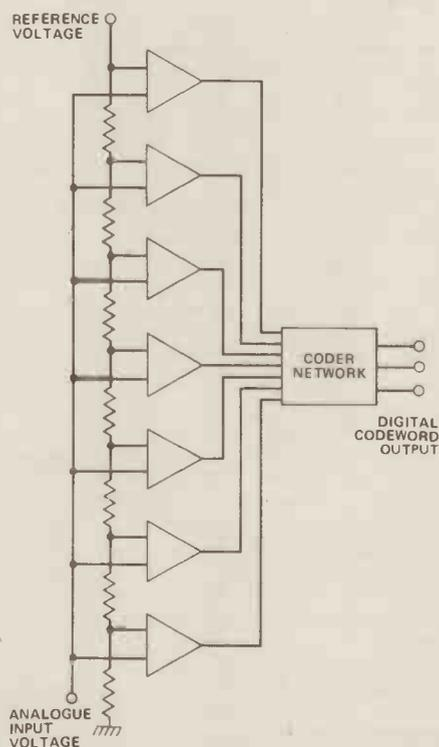
Figure 8. The parallel, or flash ADC which uses  $2^n - 1$  comparators.
