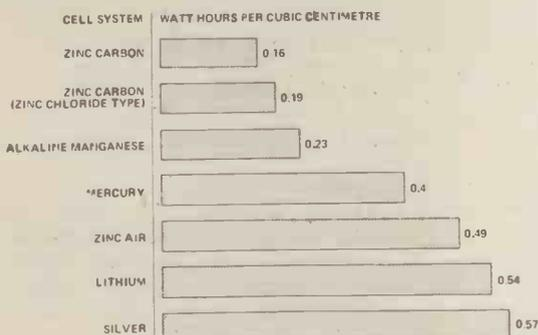
**Figure 16.** A graph showing a comparison of the capacities of various cell types with regard to their volume.
