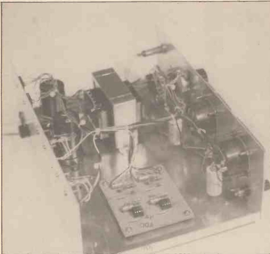
Our arrangements include the Dual PSU — two 'live' views. Because of the large number of small components and trailing wires, it's important to pay a lot of attention to insulating components where necessary (as described in the text) and clipping up the wires neatly to avoid a rat's nest.
