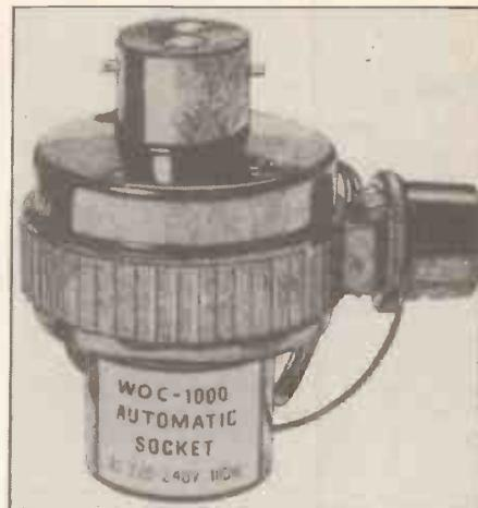
The socket fits into the existing light socket, and the bulb then plugs into a bulb fitting on the attachment. The unit is weatherproofed (indeed, it would possibly be more useful as an outdoor light than for indoor, for various reasons) and is fitted with a Cd-S Photocell. CSR recommend that only bulbs up to 60W are used, presumably because the bulb's own illumination will interfere with the photocell if the light is too strong.
