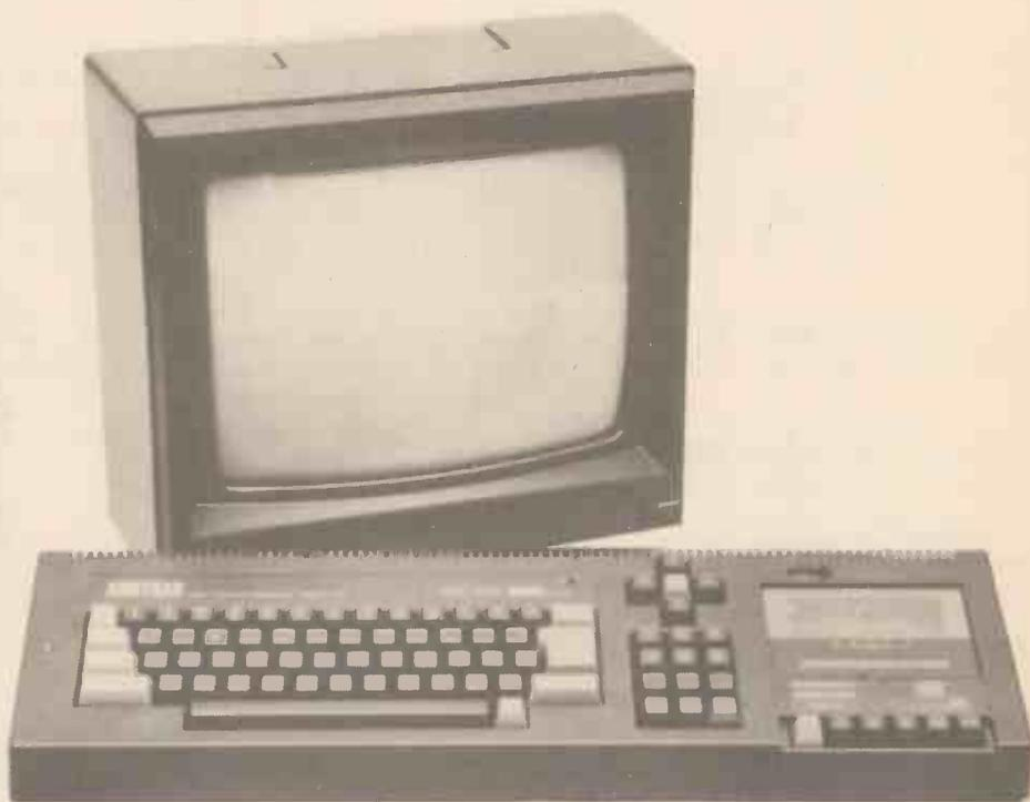
The Amstrad CPC464 comes complete with an integral data recorder, and a choice of monitors. The two are not available separately.
