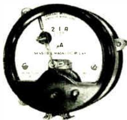
The Model S 124 is of the permanent magnet moving coil type and can be supplied to operate on currents as low as 2 mic A. d.c. High contact pressure is ensured by magnetic attraction between the contacts; these will "hold-on" until reset manually or by remote electrical control. Front-of-panel and flush mounting relays are available.
