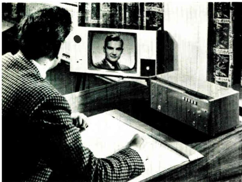
*The shape of things to come? This Pye video telephone was demonstrated at a recent exhibition in London. Up to ten extensions can be used with the system; signals are routed through a fully automatic exchange which can be equipped to carry up to five simultaneous audio, visual conversations with normal telephone privacy.*
