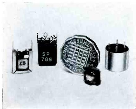
by the Joint Service Radio Components Standardisation Committee. General construction of these transformers and chokes, the result of many years of research into the design of miniature components, is in accordance with DEF 5214.
