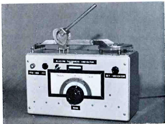
Figure 14. Capacitance bridge
