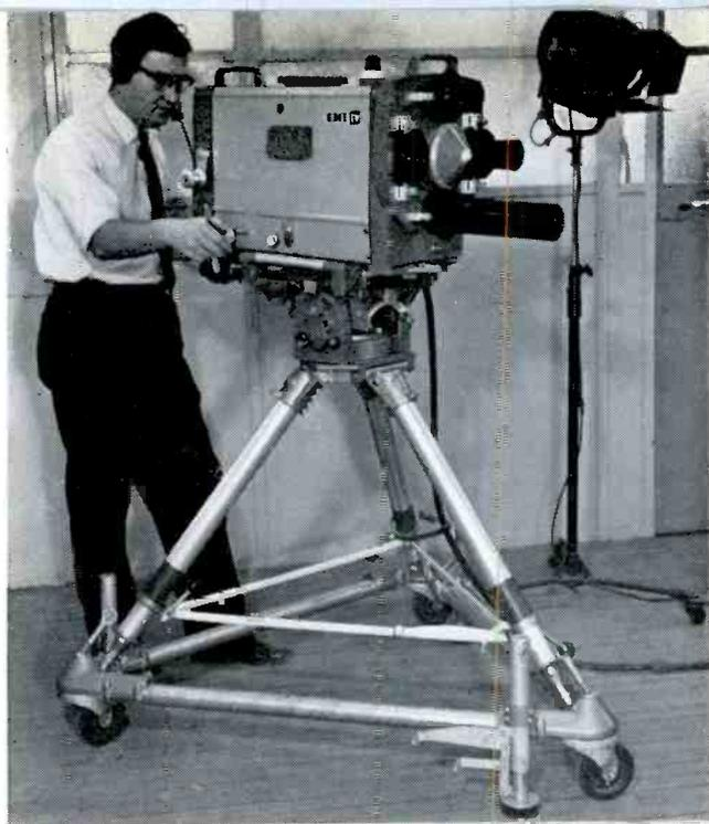
BRITAIN sends an amazing new camera, the EMI Type 206 channel, to Washington. Here is the big new  $4\frac{1}{2}$ -in image-orthicon channel being lined up at the EMI Electronics laboratory immediately prior to being flown over to Washington for all the technical world to see.
