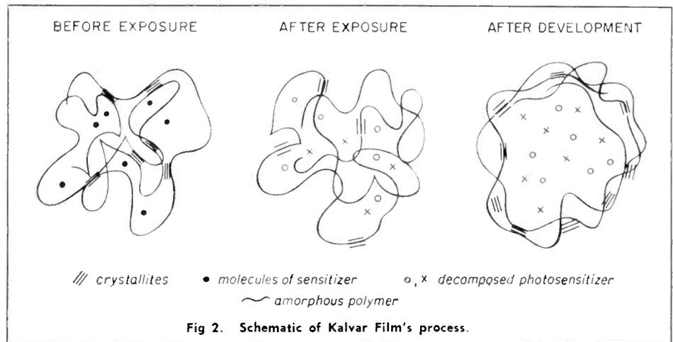
Fig 2. Schematic of Kalvar Film's process.
