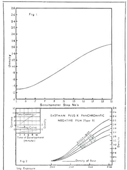
Fig 1. Standard negative characteristic curve.
