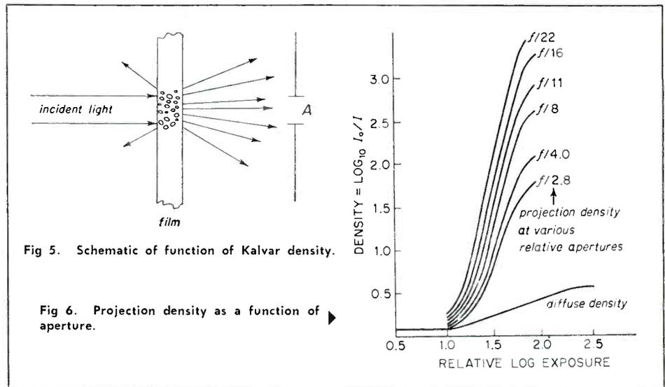
Fig 5. Schematic of function of Kalvar density.
