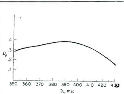
Fig 3. Spectral response of Kalvar film.
