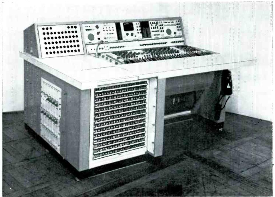
■ Three new solid-state television sound mixers with plug-in modular units are announced by EMI Electronics Ltd (see photo above).
