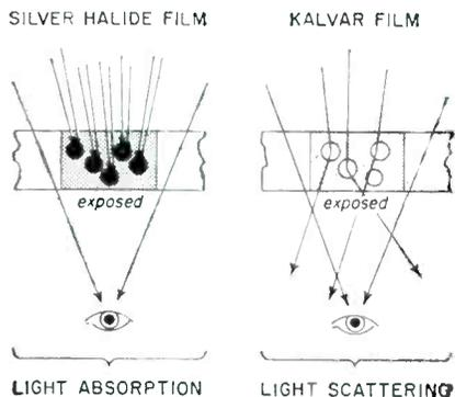
Fig 1. Comparison of the two systems of photography.
