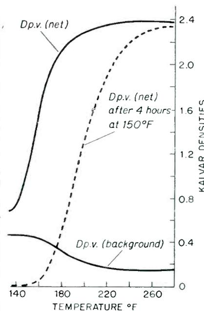
Fig 4. Kalvar film densities with constant exposure and development time, varying development temperature. Dpv = density projection visual.
