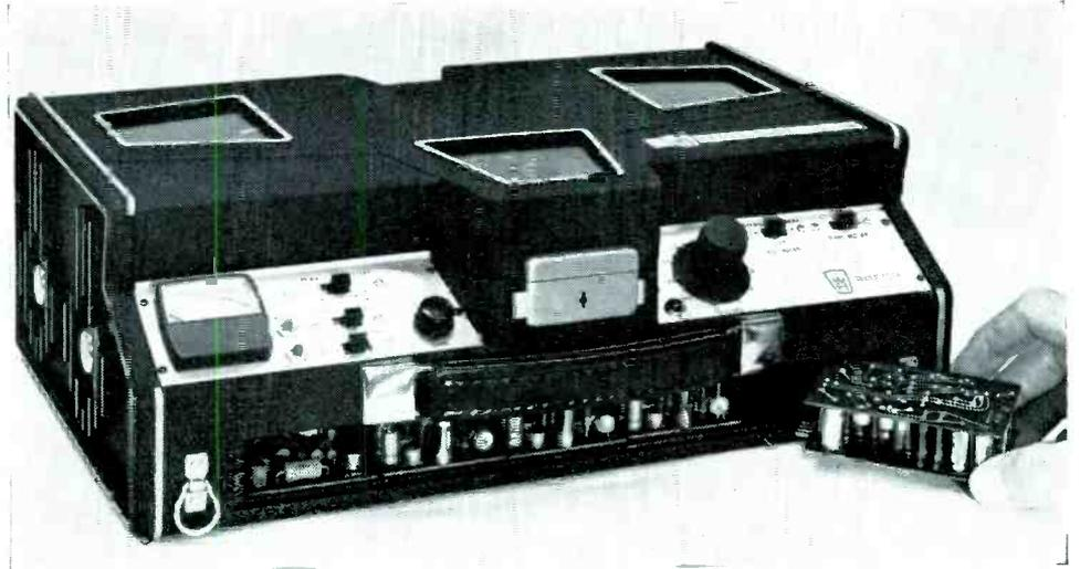
Plug-in modules are interchangeable between microphone pre-amplifier, record amplifier and playback pre-amplifier. Bias oscillator and one spare module complete amplifier section.
