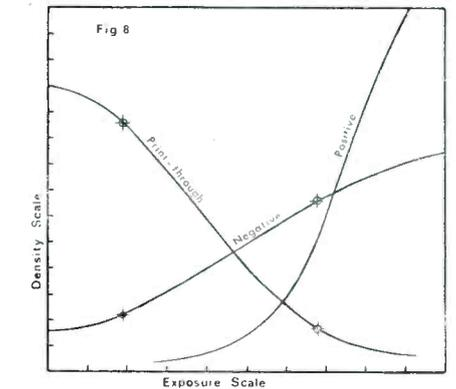
monly employed in the motion picture industry. This curve might be adopted for purposes of illustration as the standard positive characteristic. Here again, the positive processing conditions must be adjusted to conform with the standard characteristic.
