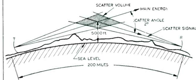
the tangent to the earth's surface at the site. Where nearby obstacles make a positive elevation unavoidable, the angle must be kept to a minimum as a slight elevation of two or three radians entails an additional loss of several decibels.
