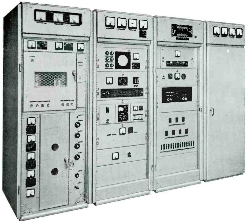
*The 10 kW vision transmitter type B 7102 is designed for use with the B 6551 2 or 5 kW sound transmitters*
