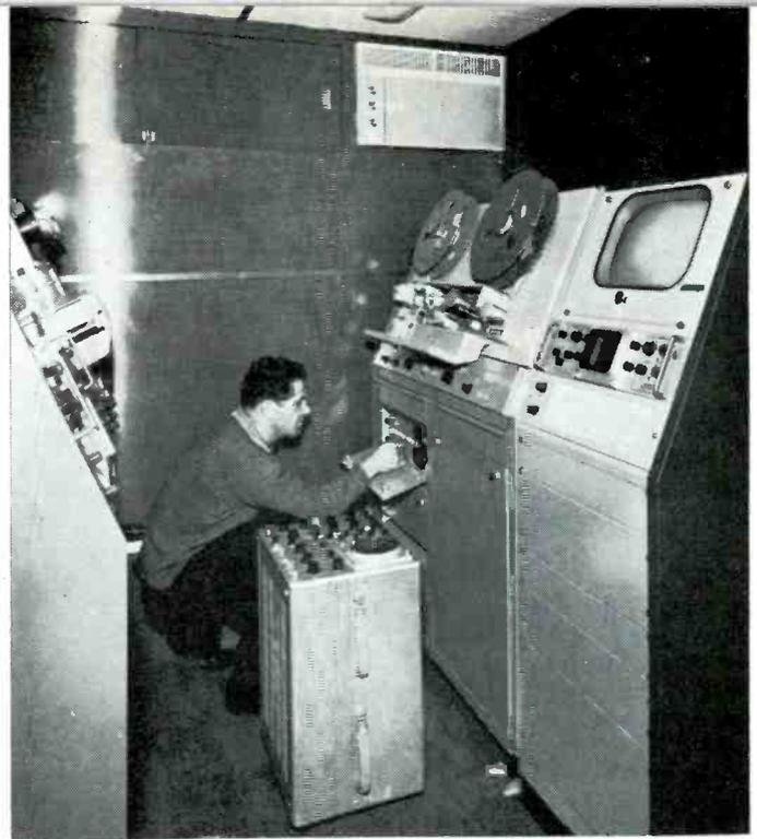
Interior view of recording room showing one of the two Ampex fully transistorised audio video tape recording units operated by Intertel (VTR Services) Ltd and mounted in a Luton body on a Ford D 800 chassis.
