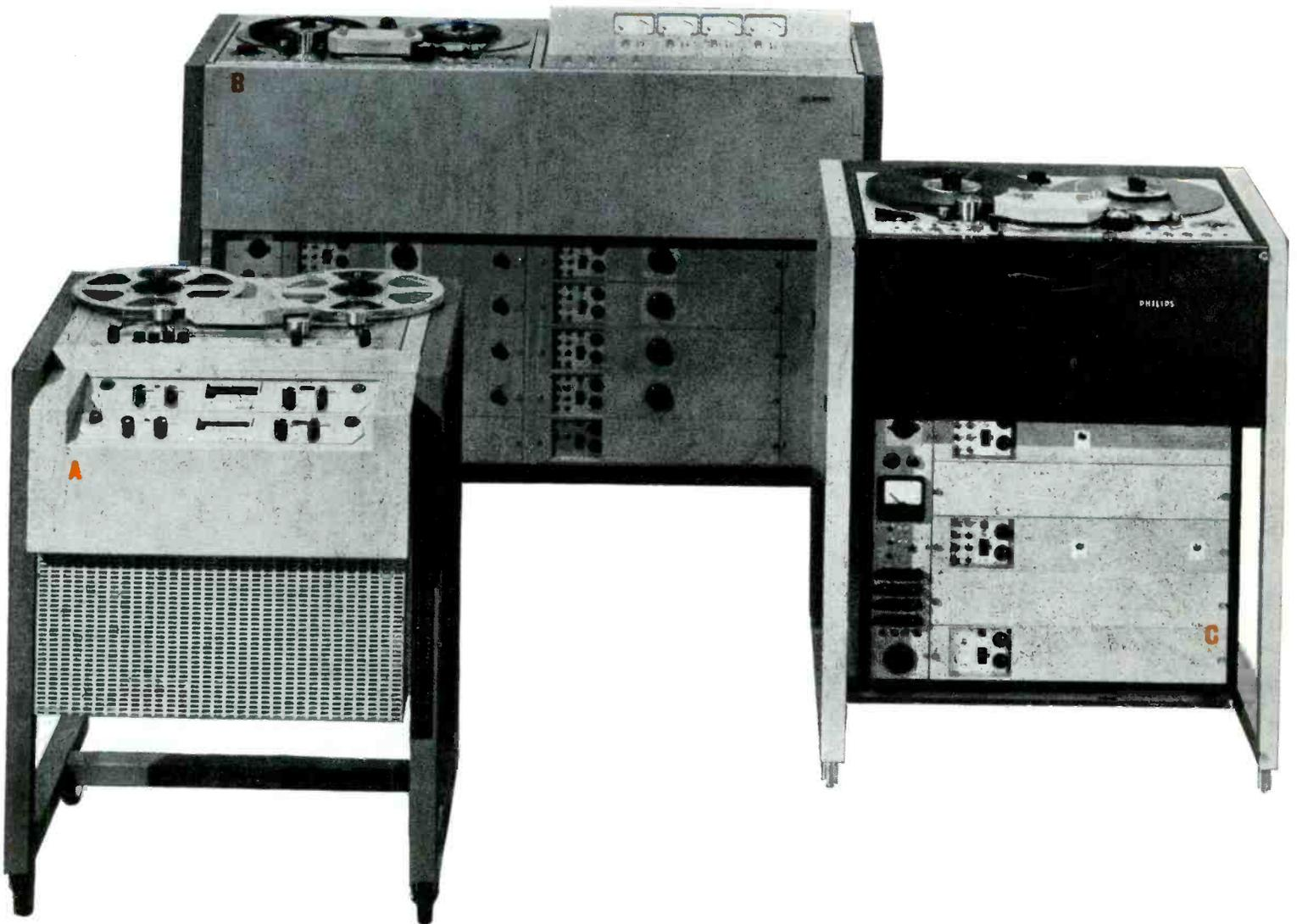
A new range comprises three types of recorder, available for 50 c/s operation, and with CCIR or NARTB equalisation.
