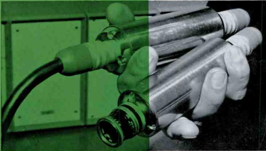
The half-inch vidicon, detailed at the London Symposium by Mr. A. C. Dawe, BSc (Eng) ACGI, makes it possible to produce an ultra-miniature camera such as this, which is only 4½ inches in length, weighs well under 2 lbs., and can be switched from 405 to 525 or 625 by pressing a button!. See page 606.
