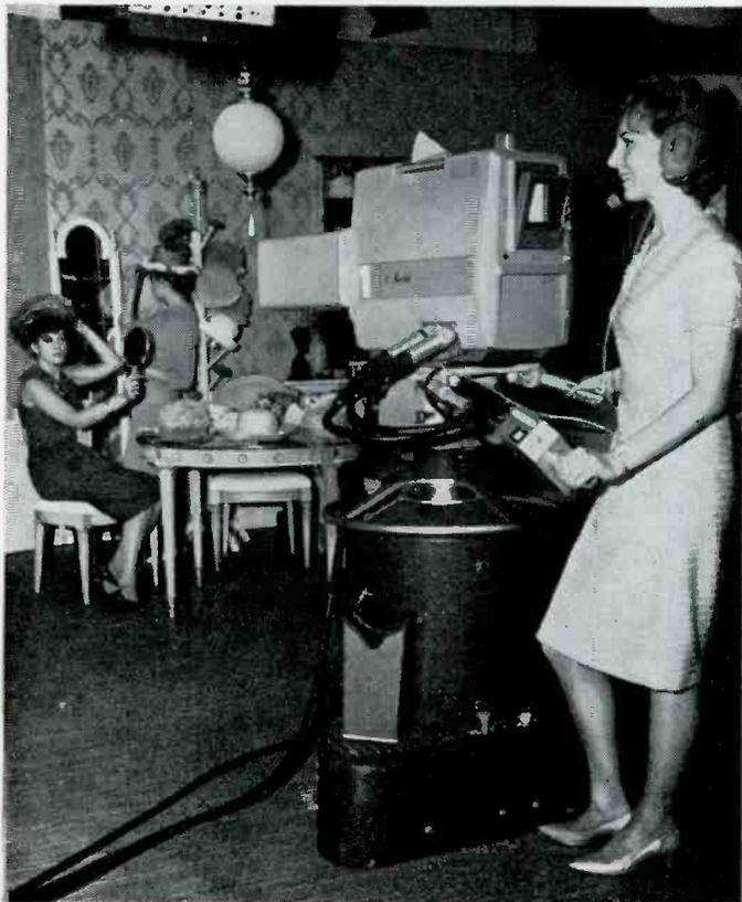
NORELCO's latest colour camera, complete with shot-box for remotely-controlled lens. In this exclusive tape interview, four leading colour experts talk of the future of systems using tubes as in the Norelco.
