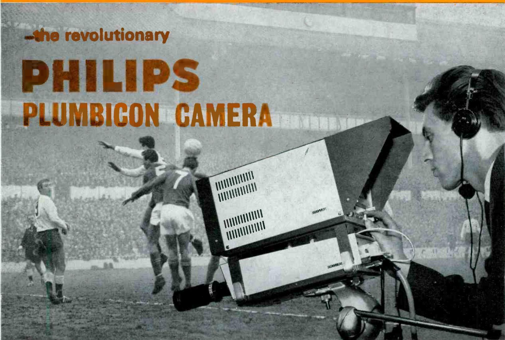
The Plumbicon Camera offers the picture quality of an image orthicon, combined with the compactness, the ease of control, and the low cost of a vidicon.
