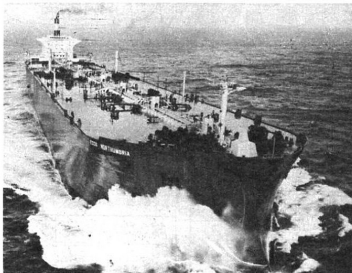
Above: the 'Esso Northumbria', a 250,262-ton tanker, is 1,143 feet long with a beam of 170 feet.
