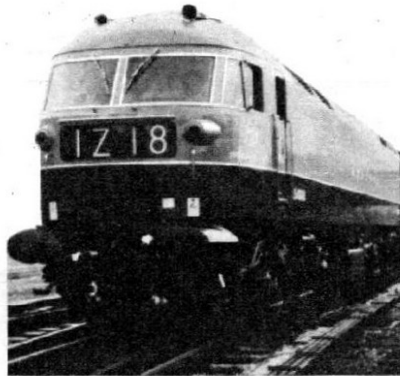
The Hawker Siddeley 'Kestrel' with a 4,000 hp engine, is the world's most powerful diesel electric locomotive.
