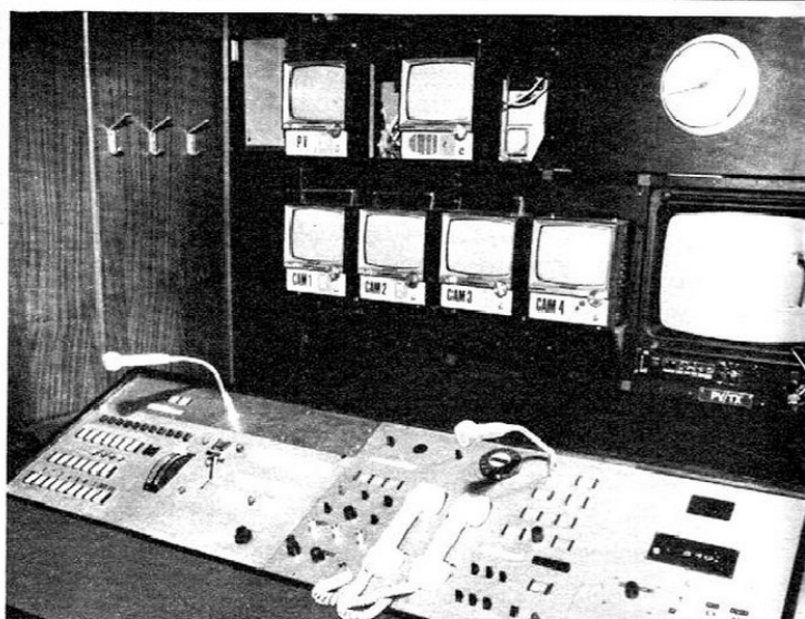
The production control desk inside Southern Television's mobile control room
