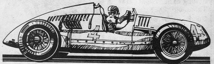
The massive Auto Unions (below) and Mercedes-Benz of the 1930s had real problems coping with the Monaco circuit and the factories had to produce special cars with shortened wheelbases to make them competitive.
