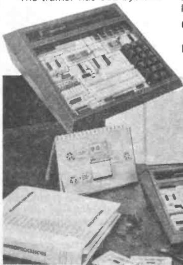
random access memory, 8 buffered LED's for display of breadboard logic states, 8 SPST DIL-switches for binary input and a breadboard for prototyping memory and interface circuits.
