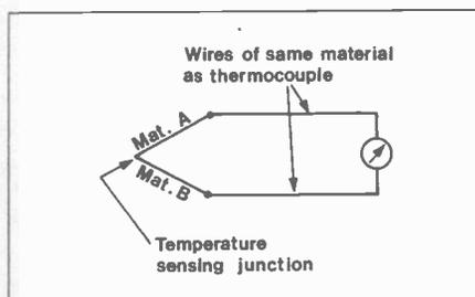
Figure 8. Thermocouple Circuit
