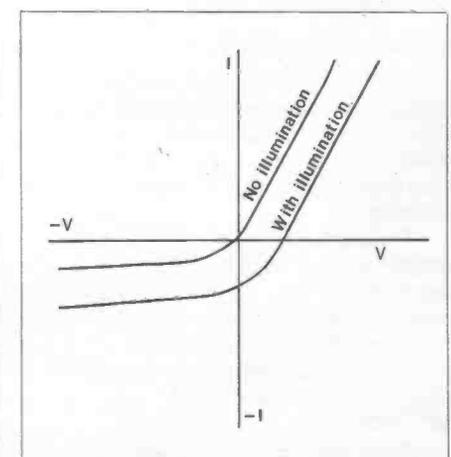
Figure 6. Photodiode Characteristic
