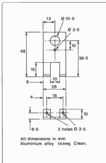
Figure 9. Tuner Bracket
