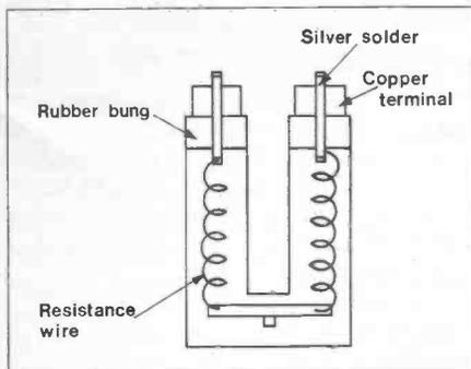
Figure 3. Standard Resistor
