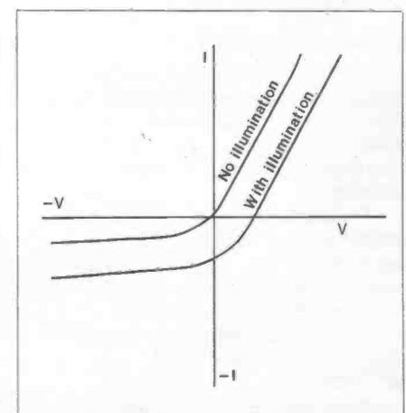
Figure 6. Photodiode Characteristic
