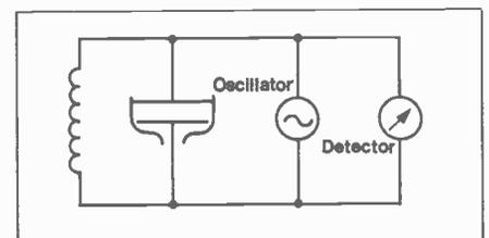
Figure 12. Capacitance Transducer
