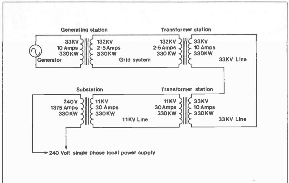
Figure 6. Power Supply from Generator to Local Supply.
