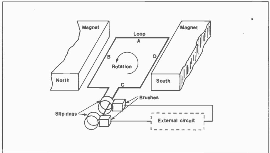
Figure 1. The Rotation of a Loop between two Magnetic Poles.
