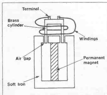
Figure 4. Hibbert Standard for Magnetic Flux
