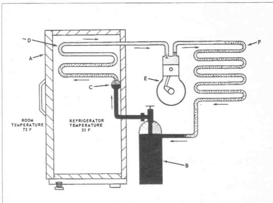
**Figure 1. An elementary mechanical refrigerator. A—Refrigerator. B—Liquid refrigerant receiver. C—Refrigerant control. D—Evaporator. E—Motor-driven compressor. F—Condenser. In this refrigerator, the refrigerant is not allowed to escape, but is recycled, as necessary, to get the desired temperature.**
