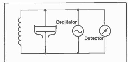
Figure 12. Capacitance Transducer
