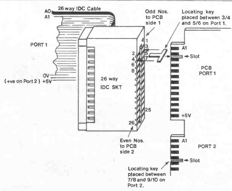
Figure 6. Connection to the 6 x 8-bit PCB
