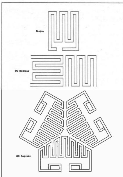
Figure 15. Foil Strain Gauges
