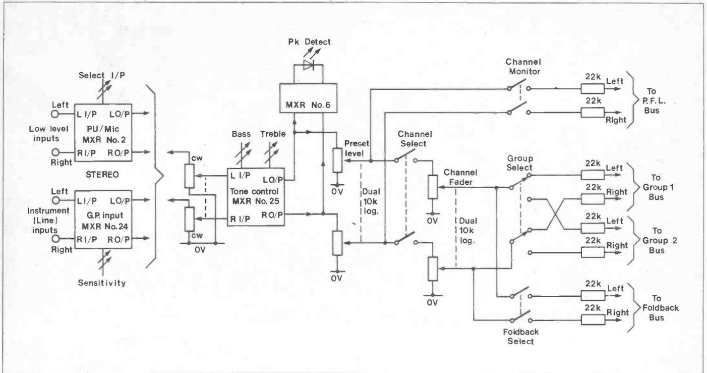
Figure 37. Typical Stereo System
