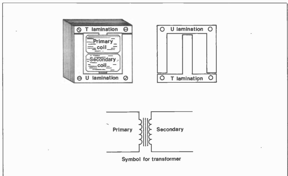
Figure 5. Transformer Laminations and Symbol.
