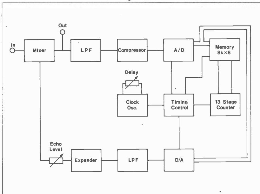
Figure 1. Digital Echo Block Schematic
