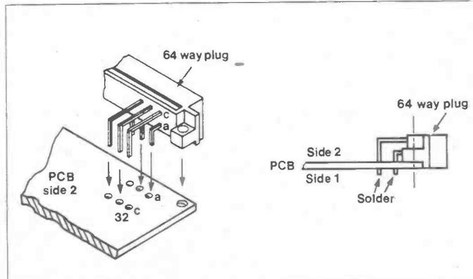
Figure 3. Fitting the 64-pin plug
