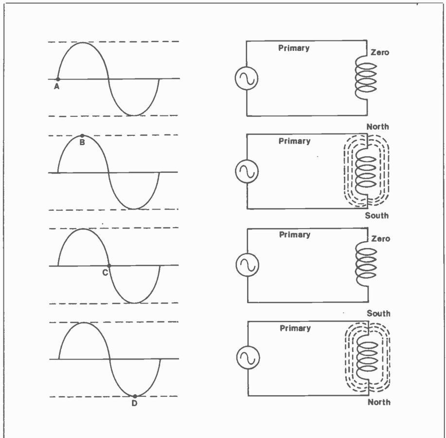
Figure 4. The Magnetic Field for one complete cycle.
