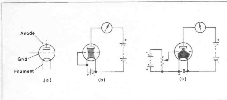
Figure 4. (a) The 'audion' or first triode valve.
