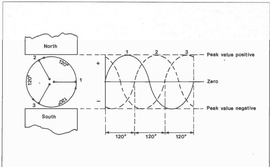
Figure 3. Three Phase Waveform.
