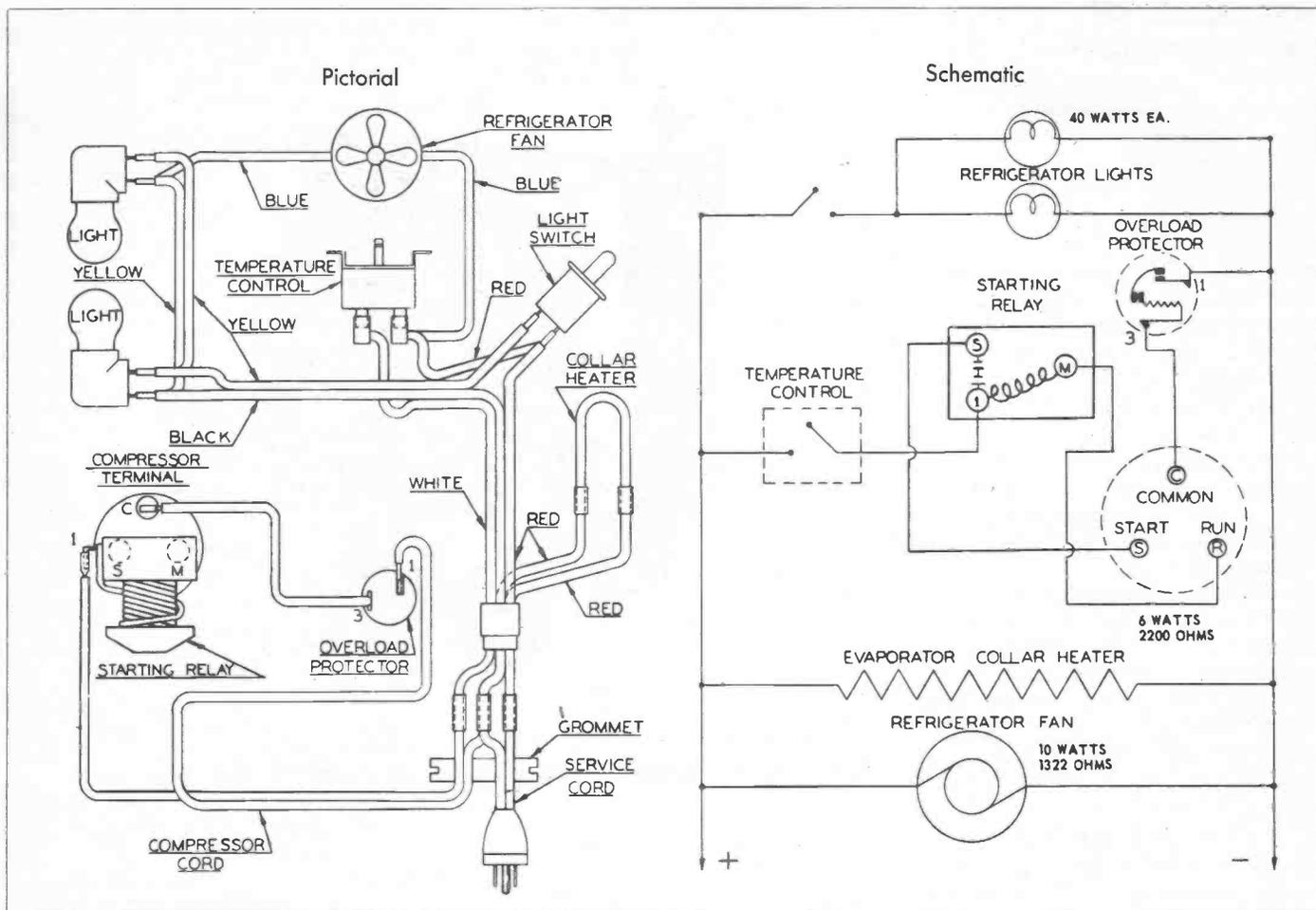
Figure 3. Typical wiring diagram of a refrigerating system.
