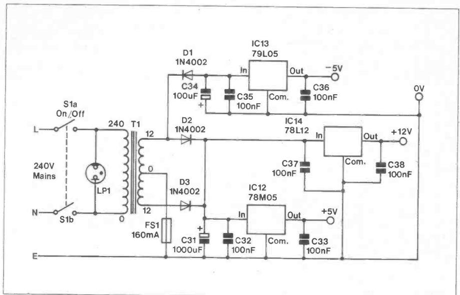
Figure 5. Power Supply Circuit
