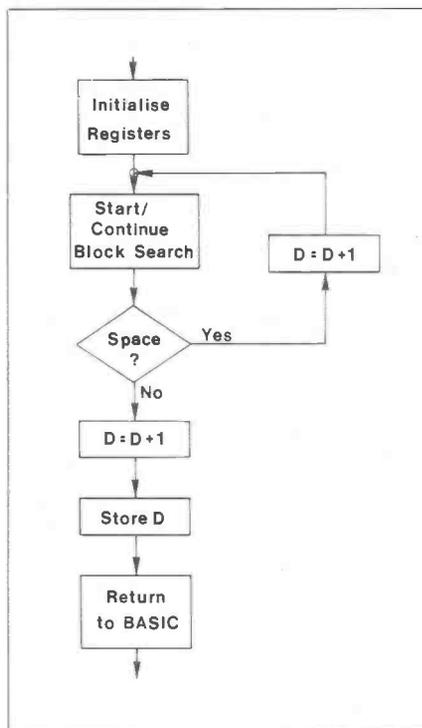
Figure 3. Flowchart for machine-code program.
