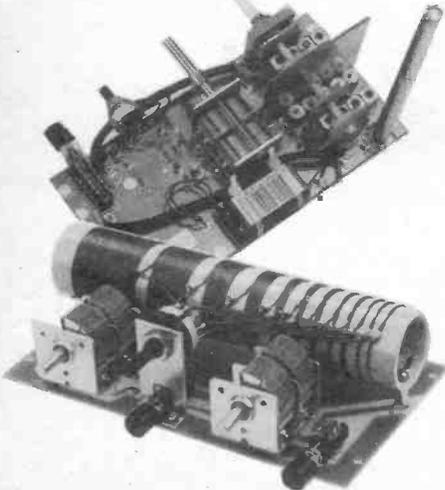
in telescopic aerial. The Aerial Tuning Unit provides for exact impedance matching of any antenna to the receiver, essential for getting the most out of any aerial and providing the best selectivity.
