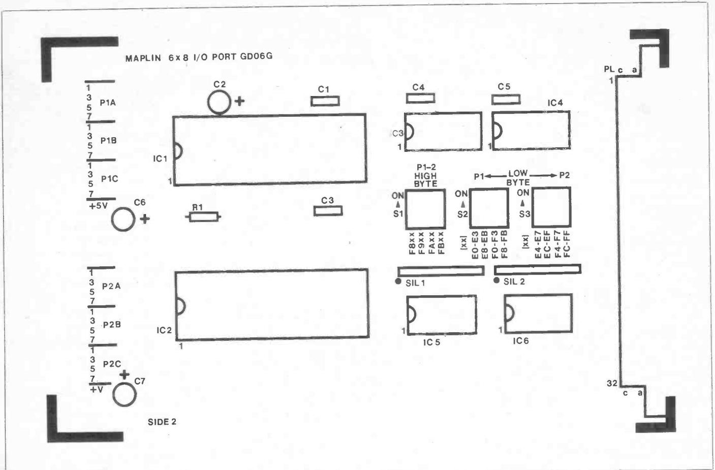
Figure 2. 6 x 8-bit Port PCB Overlay
