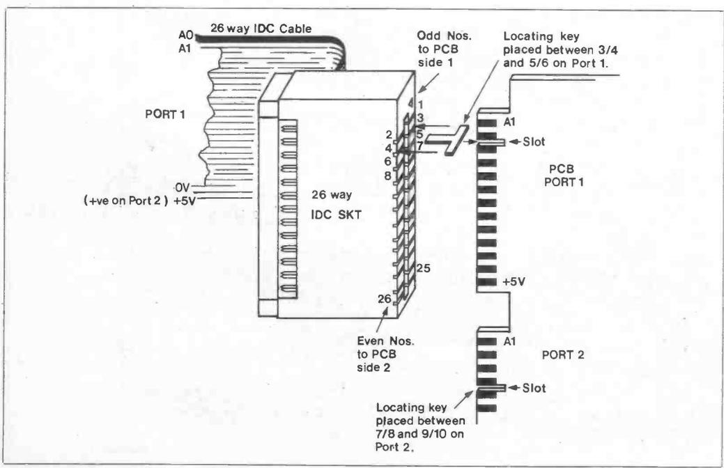
Figure 6. Connection to the 6 x 8-bit PCB
