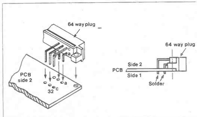
Figure 3. Fitting the 64-pin plug
