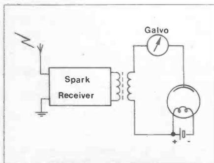
Figure 1. Fleming's arrangement for establishing the principle of the 'oscillation valve'.
