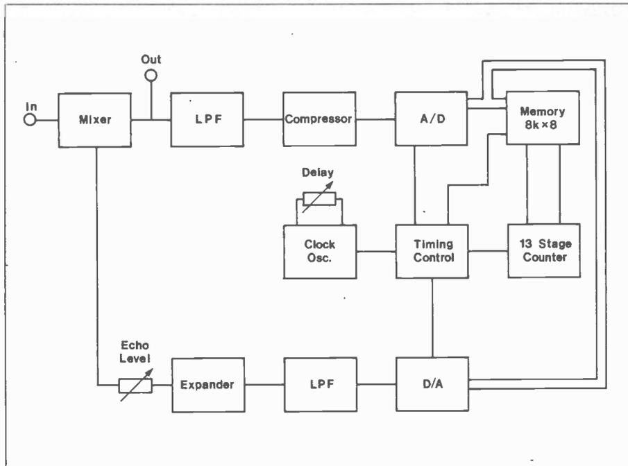
Figure 1. Digital Echo Block Schematic
