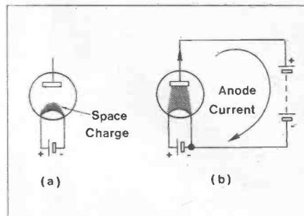
Figure 2. (a) Formation of space charge by heated filament. (b) Current flow when anode is positively charged.
