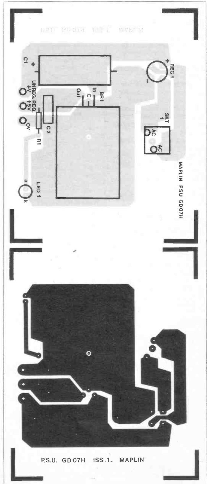
Figure 8. PSU PCB Track and Legend
