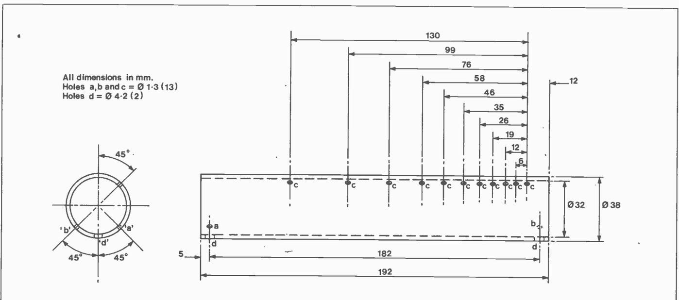
Figure 7. Coil Tube Drilling
