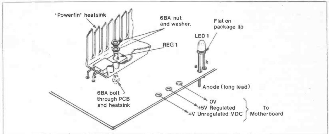
Figure 9. Fitting LED1 and REG1
