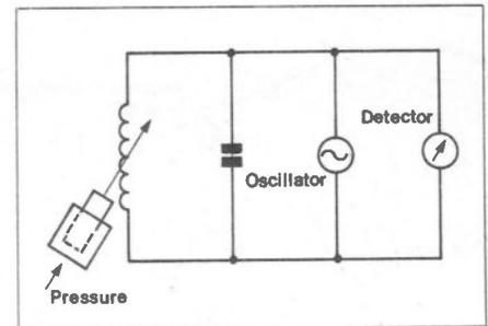
Figure 11. Physical Displacement changes the Frequency
