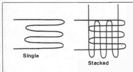
Figure 14. Wire Strain Gauges
