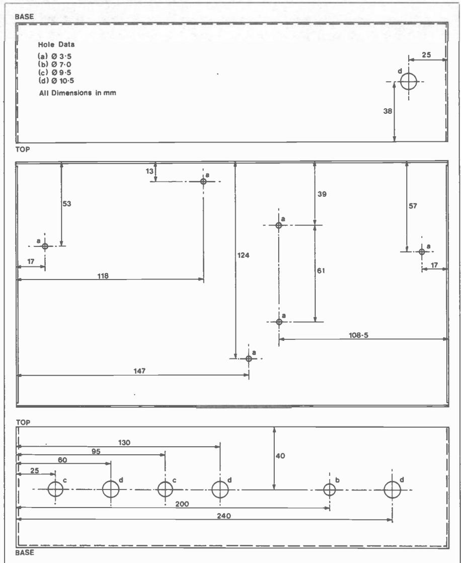
Figure 9. Box Drilling
