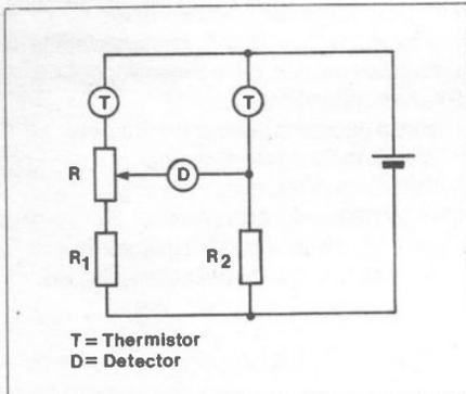
Figure 7. Thermistor Application in Air Flow Measurement
