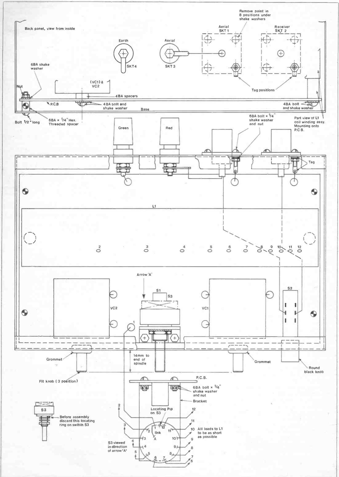
Figure 3. Wiring the Tuner
