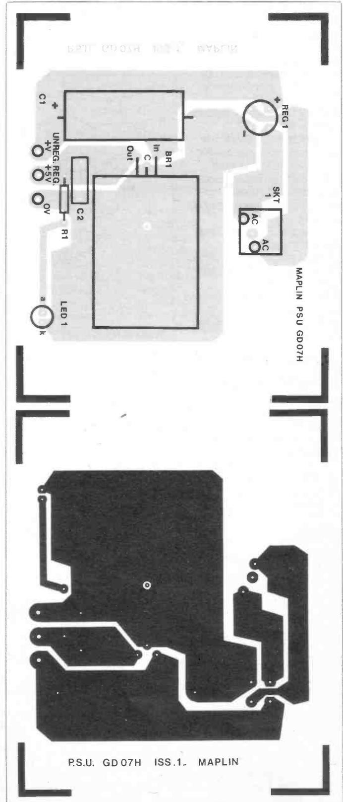
Figure 8. PSU PCB Track and Legend
