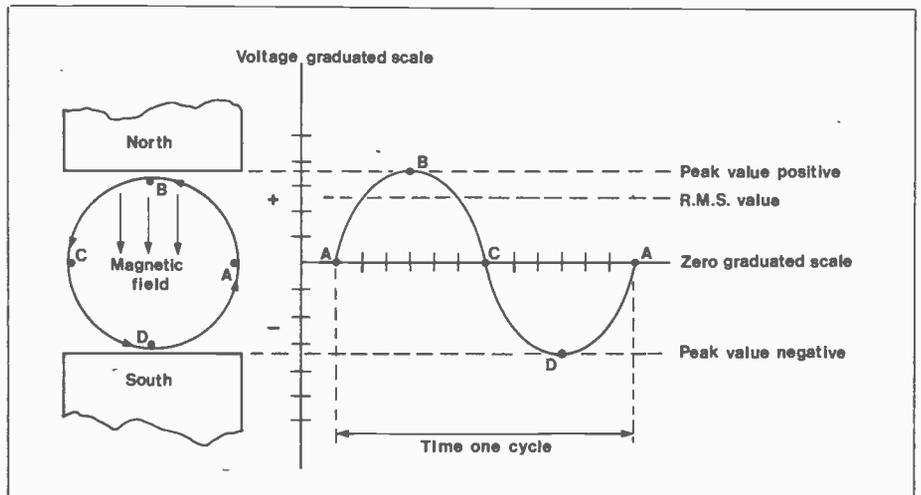
Figure 2. Single Phase Waveform.
