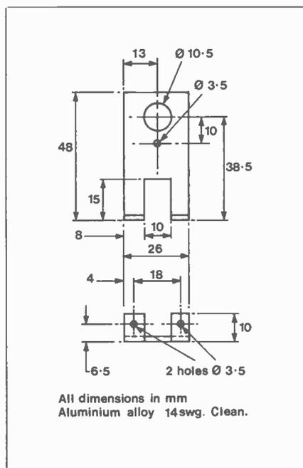
Figure 9. Tuner Bracket
