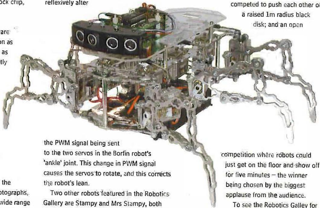
the PWM signal being sent to the two servos in the Borfin robot's 'ankle' joint. This change in PWM signal causes the servos to rotate, and this corrects the robot's lean.
