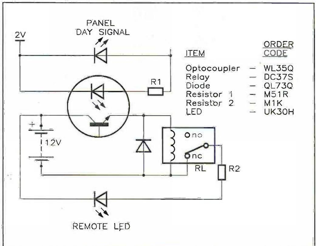
remote signalling using the 12V supply from the system standby lead acid battery.
