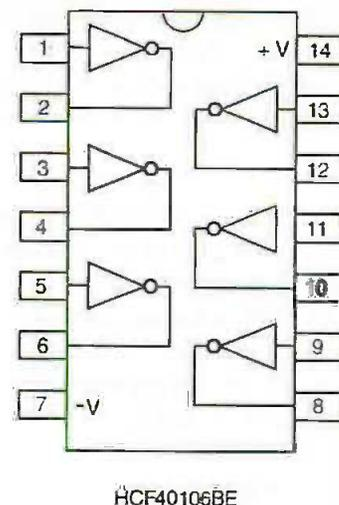
Figure 2. Semiconductor pin-outs
