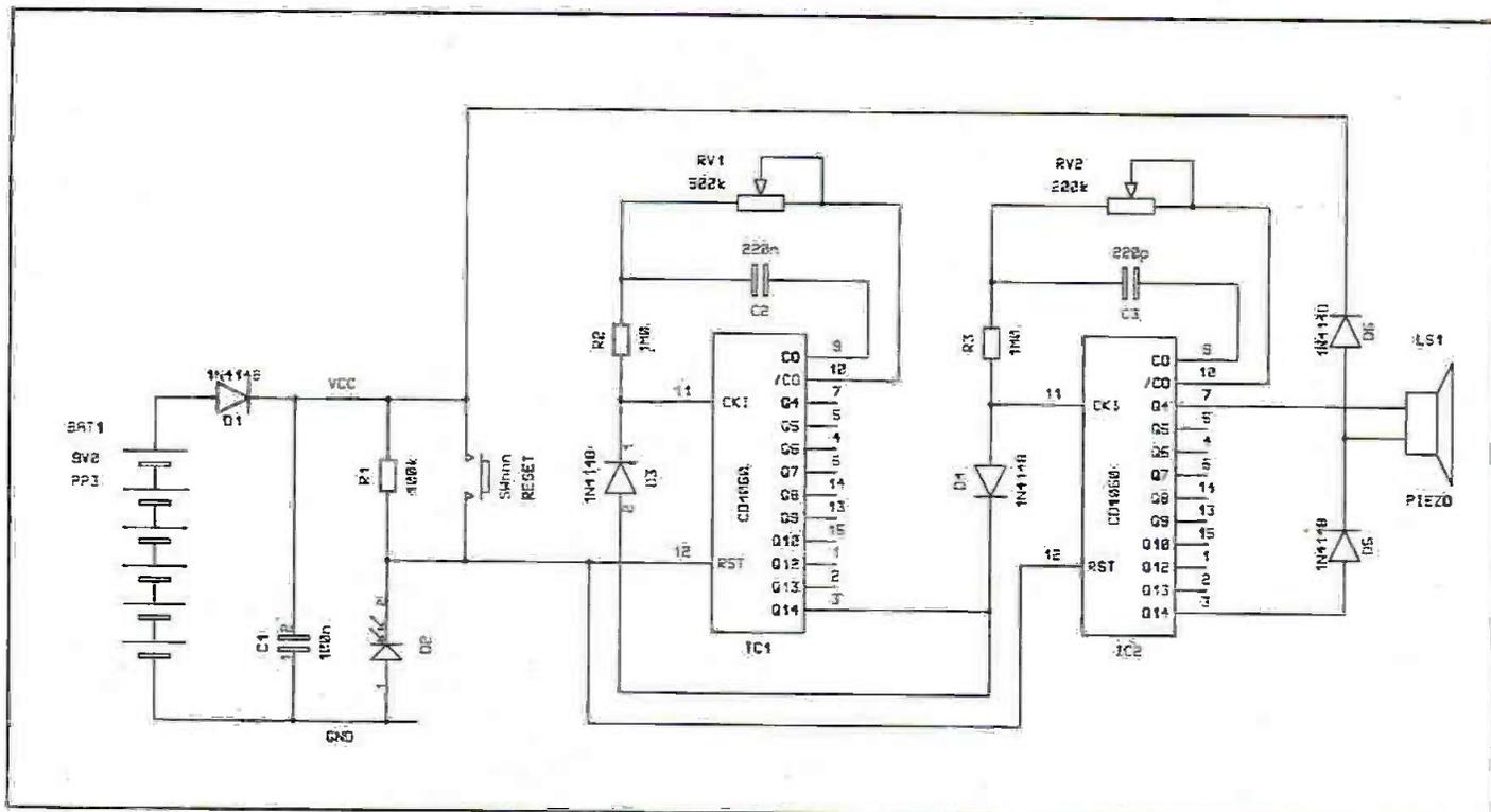
**THIS IS A DELAYED ACTION ALARM WITH A LEVEL-SENSITIVE TRIGGER CONDITION. IT WILL NOT SOUND UNTIL THE TRIGGER CONDITION HAS BEEN PRESENT FOR SOME TIME, AND WILL THEN ONLY CONTINUE TO SOUND WHILST THIS CONDITION IS HELD.**
