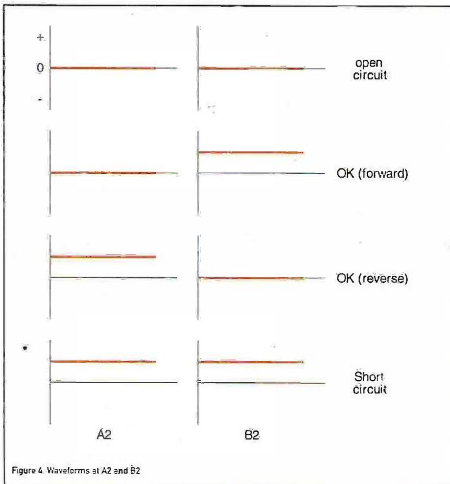
Figure 4. Waveforms at A2 and B2
