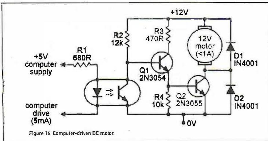
Figure 16. Computer-driven DC motor.
