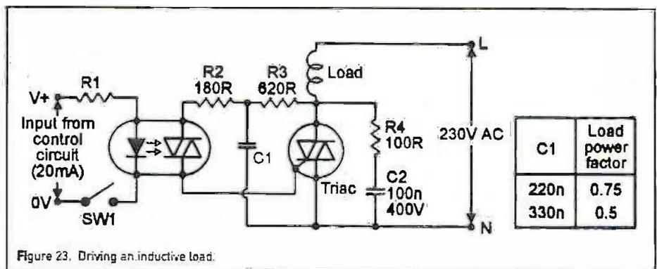
Figure 23. Driving an inductive load.
