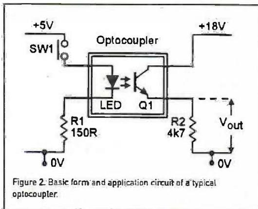
Figure 2. Basic form and application circuit of a typical optocoupler.
