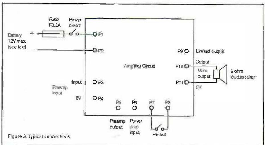
Figure 3. Typical connections
