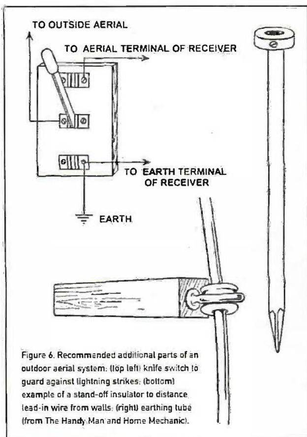
Figure 6. Recommended additional parts of an outdoor aerial system: (top left) knife switch to guard against lightning strikes; (bottom) example of a stand-off insulator to distance lead-in wire from walls; (right) earthing tube (from *The Handy Man and Home Mechanic*).
