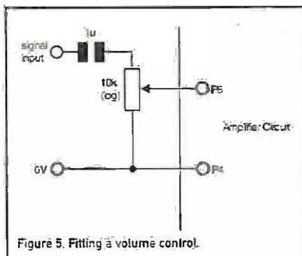
Figure 5. Fitting a volume control.
