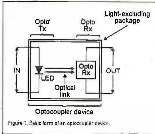
Figure 1. Basic form of an optocoupler device.
