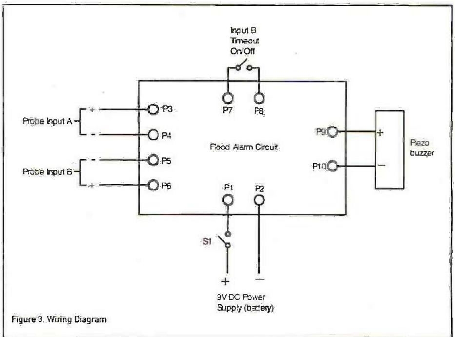
Figure 3. Wiring Diagram
