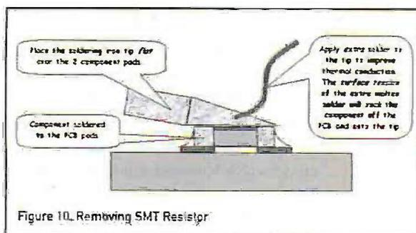
Figure 10. Removing SMT Resistor
