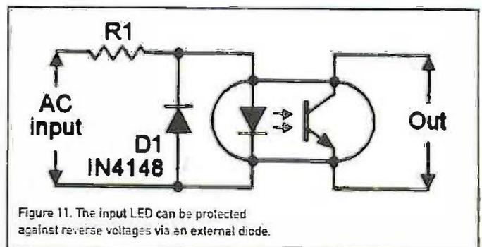
Figure 11. The input LED can be protected against reverse voltages via an external diode.
