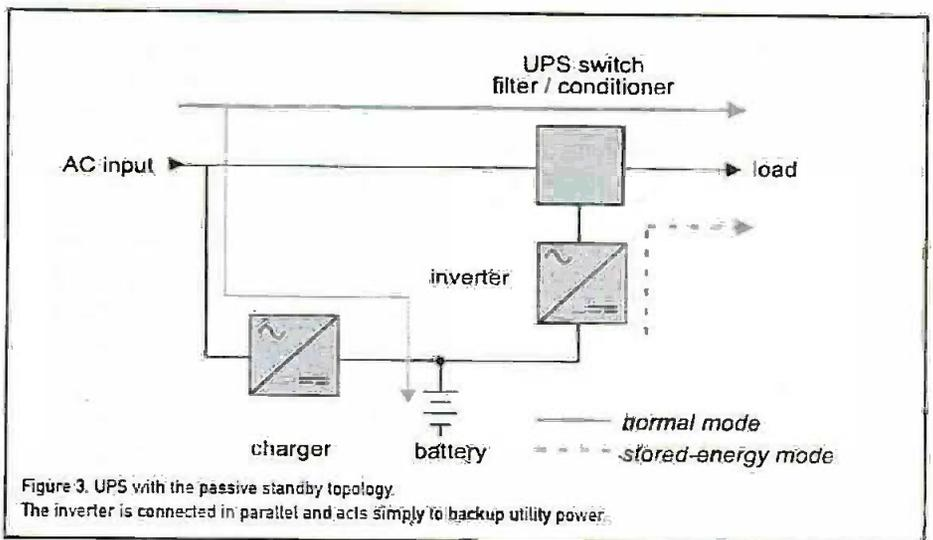
Figure 3. UPS with the passive standby topology. The inverter is connected in parallel and acts simply to backup utility power.
