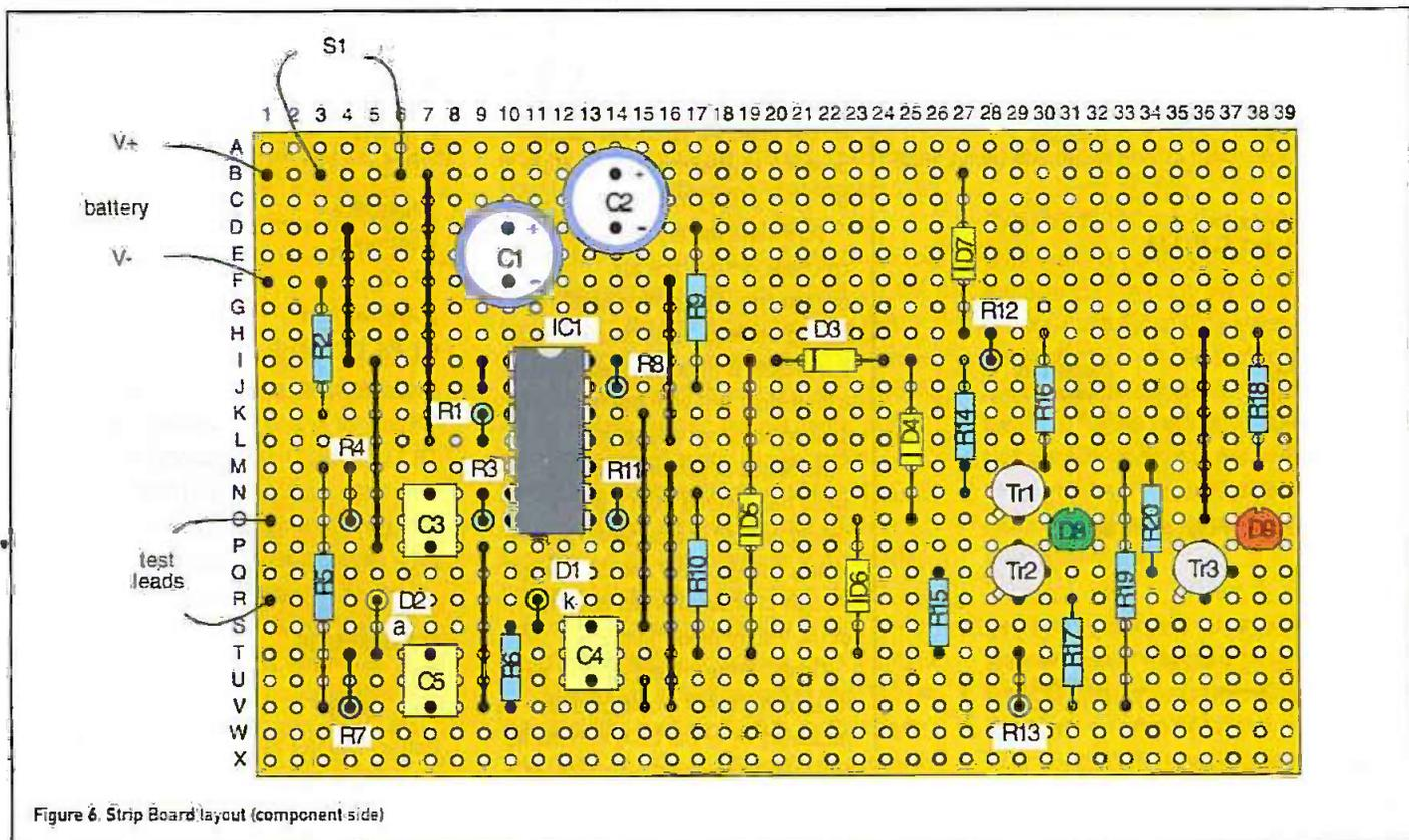
Figure 6. Strip Board layout (component side)
