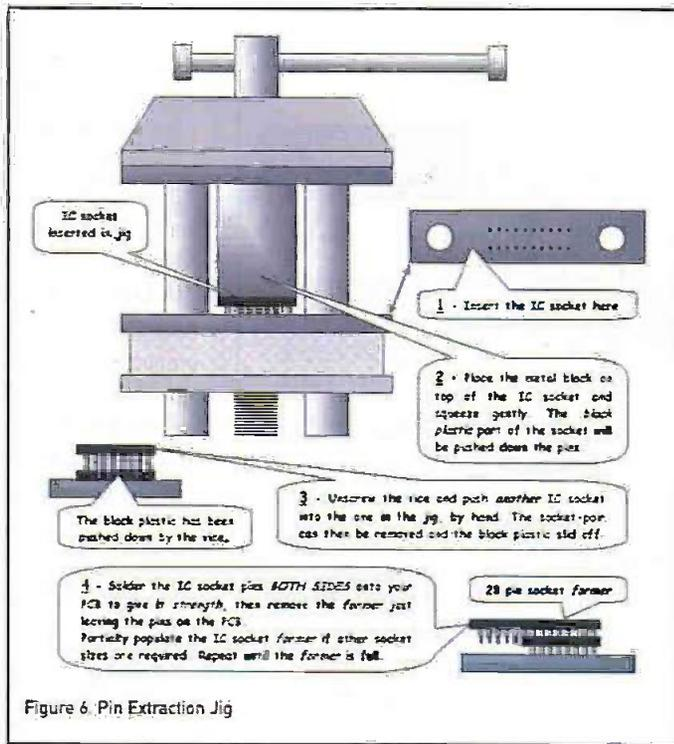
Figure 6. Pin Extraction Jig
