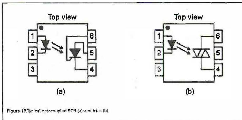
Figure 19. Typical optocoupled SCR (a) and triac (b).
