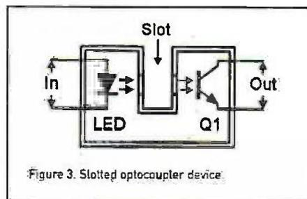
Figure 3. Slotted optocoupler device.
