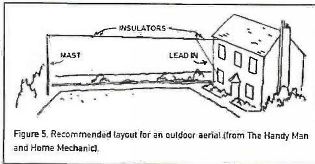
Figure 5. Recommended layout for an outdoor aerial (from *The Handy Man and Home Mechanic*).
