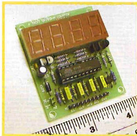
As an example of this great flexibility, this article presents two simple, low-cost, four-digit counter modules. One will count up or down and the other will count down in several user-defined ways from a preset value. The main difference between the modules is the software in the microcontroller.
