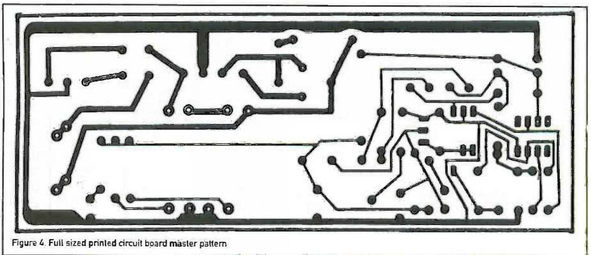
Figure 4. Full sized printed circuit board master pattern.
