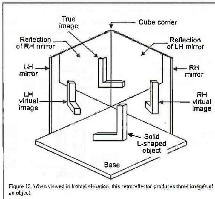
Figure 13. When viewed in frontal elevation, this retroreflector produces three images of an object.
