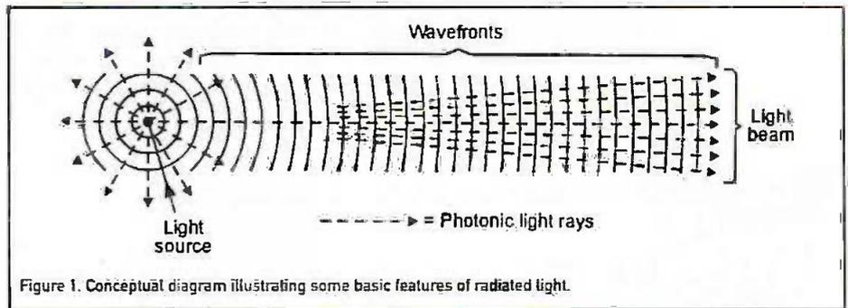
Figure 1. Conceptual diagram illustrating some basic features of radiated light.
