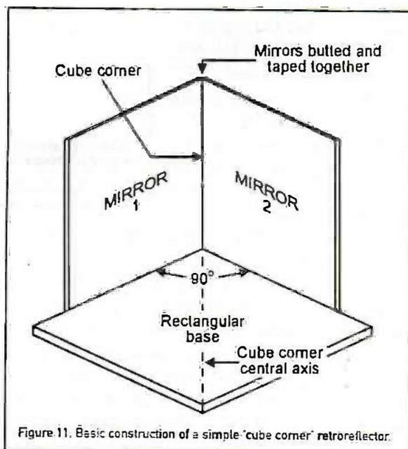
Figure 11. Basic construction of a simple 'cube corner' retroreflector.
