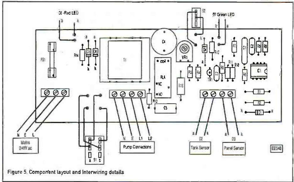
Figure 5. Component layout and interwiring details
