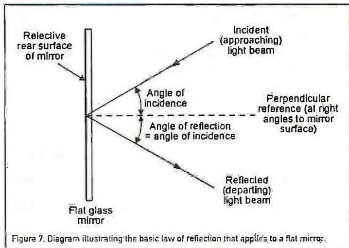
Figure 7. Diagram illustrating the basic law of reflection that applies to a flat mirror.
