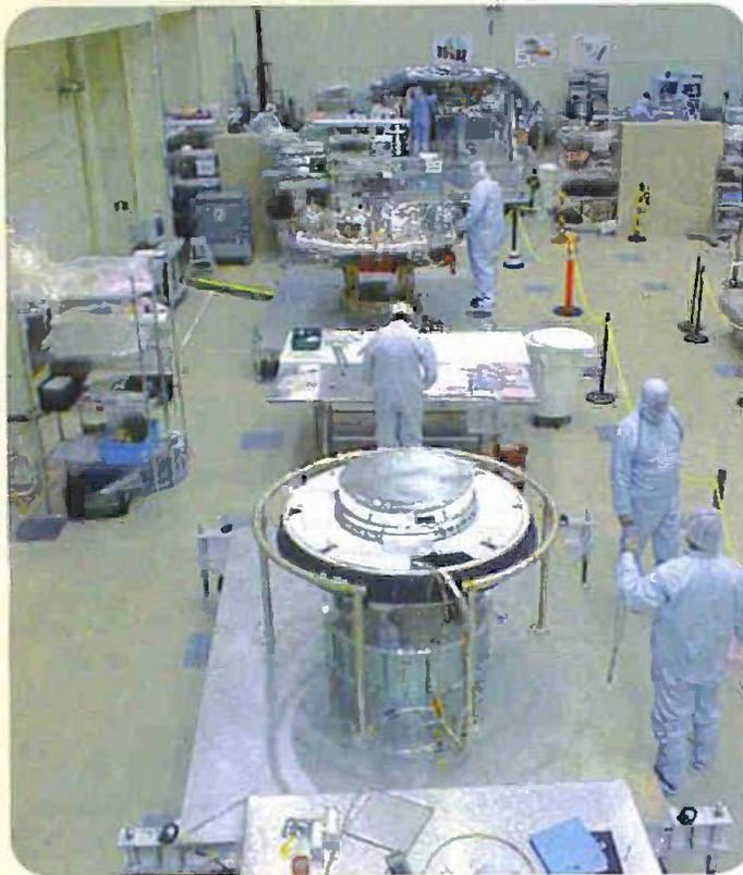
Above: LMA technicians install radiation shielding on the spacecraft
