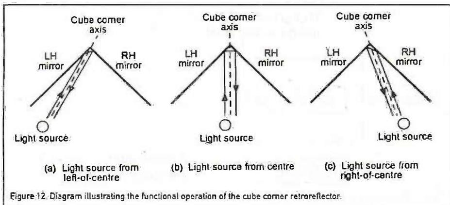
Figure 12. Diagram illustrating the functional operation of the cube corner retroreflector.
