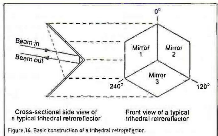
Figure 14. Basic construction of a trihedral retroreflector.
