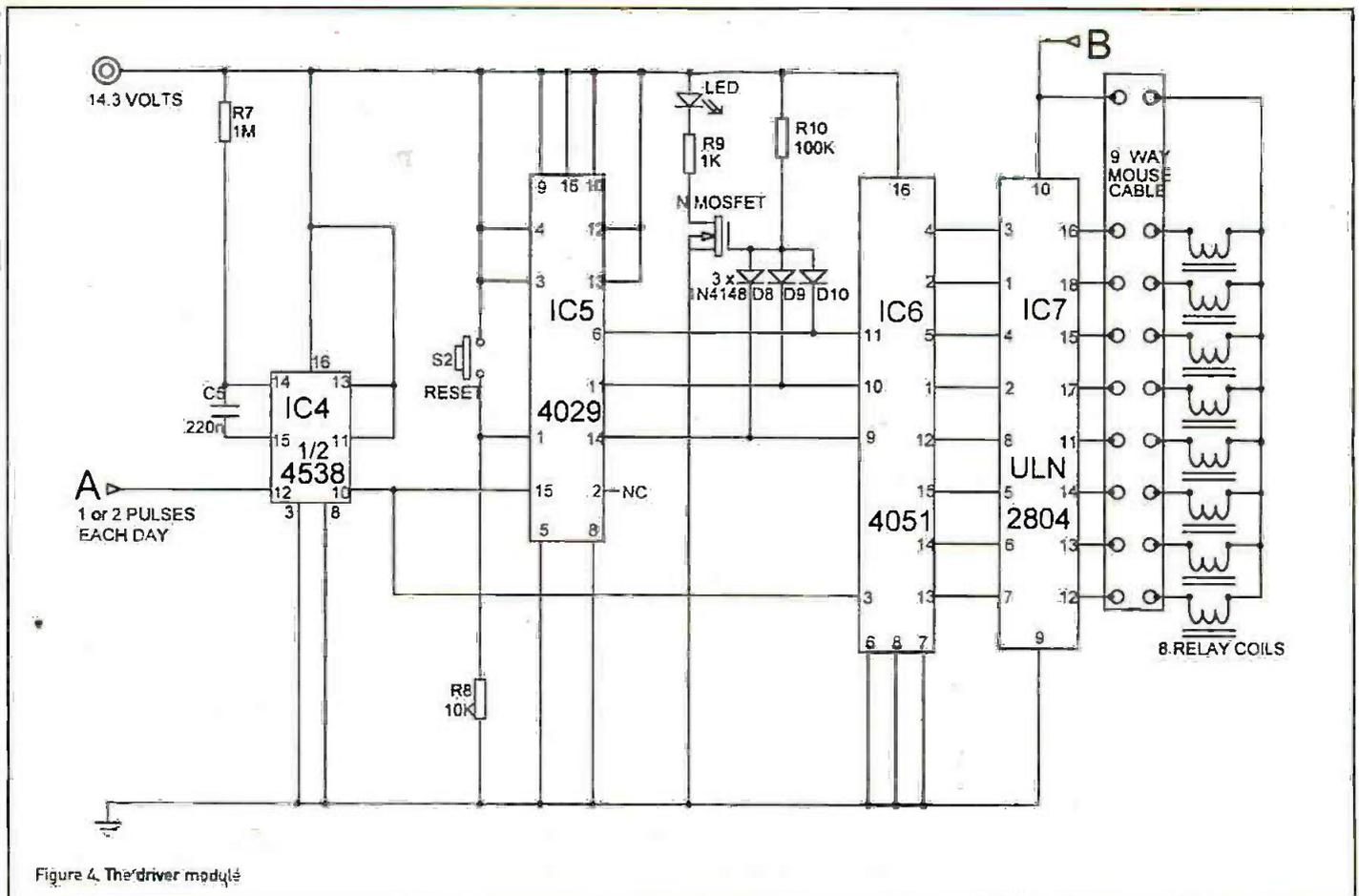
Figure 4. The driver module
