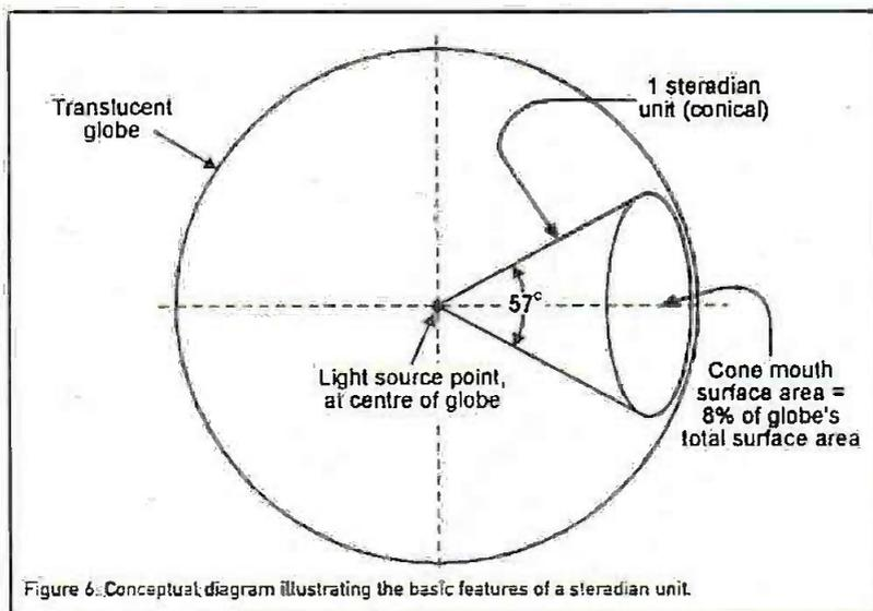
Figure 6. Conceptual diagram illustrating the basic features of a steradian unit.
