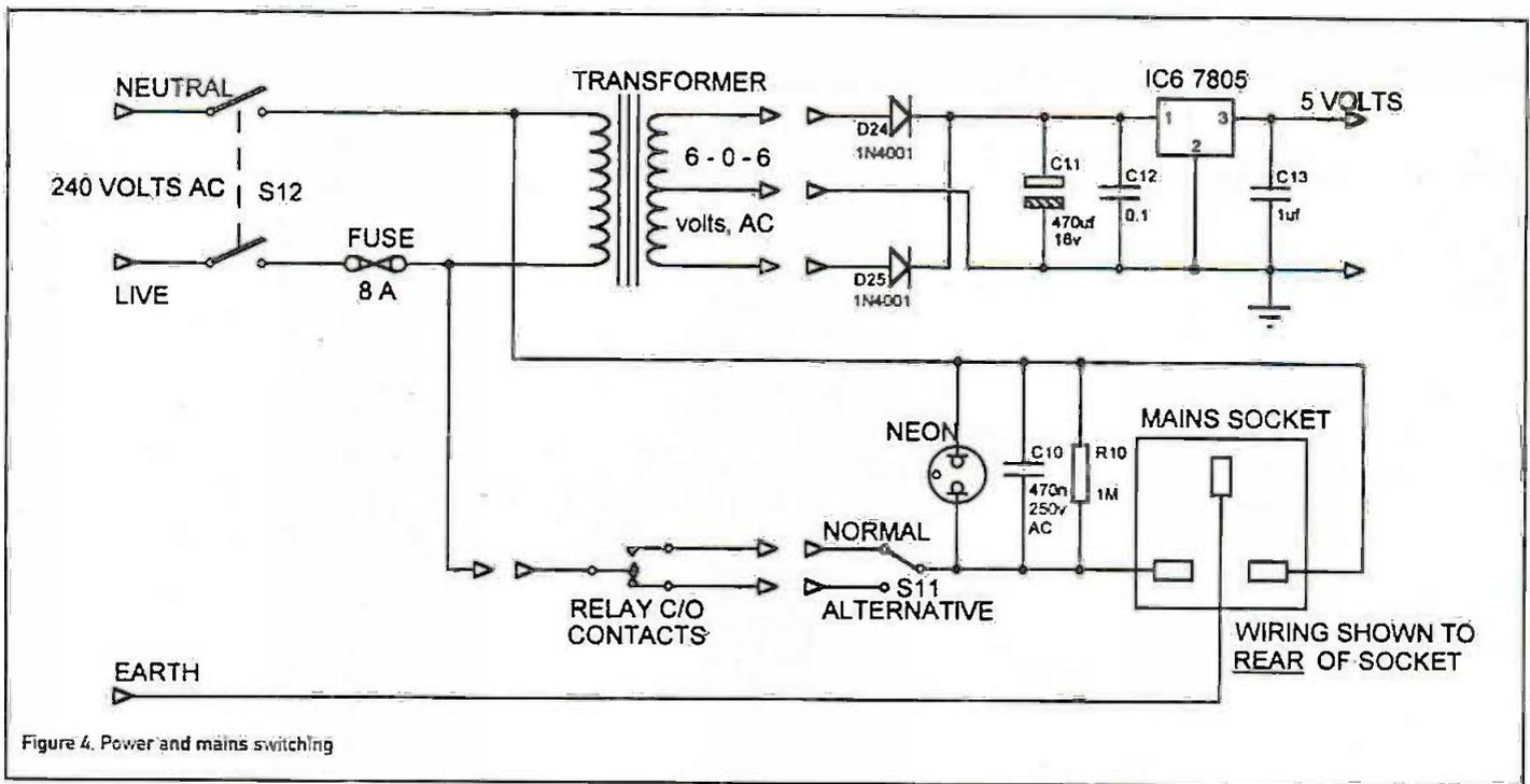
Figure 4. Power and mains switching
