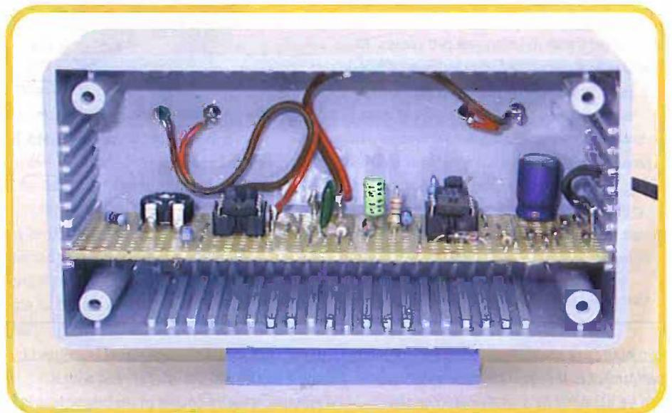
two diodes. During the periods when the input is providing the supply, one or other of the diodes will block the supply so that only an insignificant current flows through the two diodes. The output of IC1a is connected across the supply during these periods, but R1 prevents an excessive output current from flowing into IC1a's output stage.
