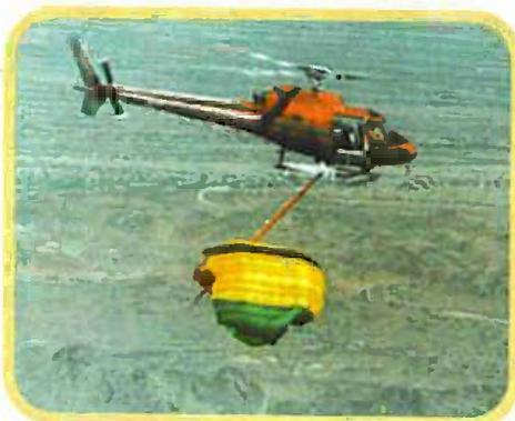
Above: Helicopter successfully snags capsule's parafoil (photo from preliminary test run)
