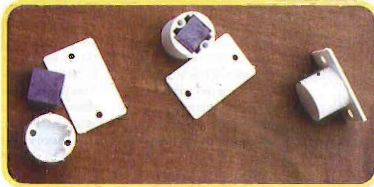
pieces can be screwed together using 1 inch, No. 4 wood-screws. No countersunk holes need be cut as Extrusion is soft enough to indent as each screw is tightened. But for the moment screws should not be driven home completely as the remainder of the assembly will require that the side sections of the box be taken apart again for further work.
