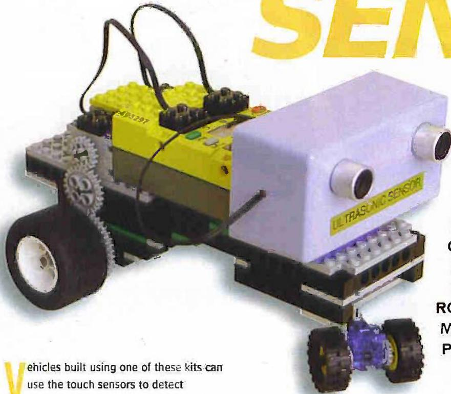
IN A PREVIOUS ARTICLE ROBERT PENFOLD DESCRIBED A SIMPLE ULTRASONIC REMOTE CONTROL UNIT FOR USE WITH ROBOTS CONSTRUCTED USING LEGO'S POPULAR MINDSTORMS CONSTRUCTION KITS. THE PROJECT FEATURED HERE IS ANOTHER ULTRASONIC DEVICE FOR USE WITH ROBOTS CONSTRUCTED USING A MINDSTORMS KIT, THIS UNIT IS A PROXIMITY SENSOR.
