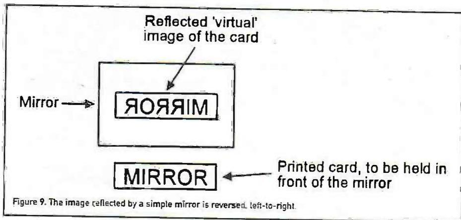
Figure 9. The image reflected by a simple mirror is reversed, left-to-right.
