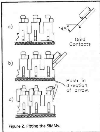
Figure 2. Fitting the SIMMs.
