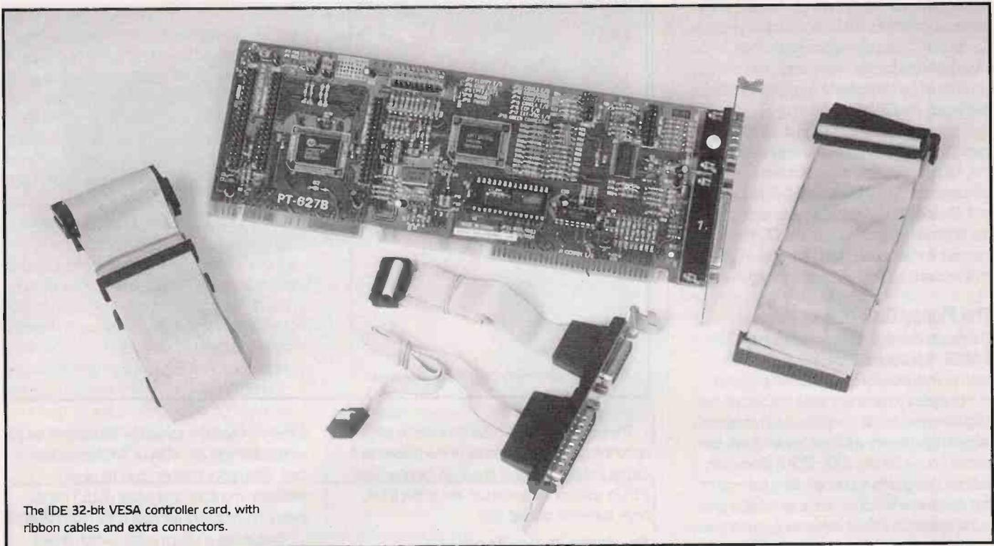
The IDE 32-bit VESA controller card, with ribbon cables and extra connectors.
