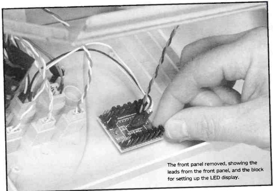
The front panel removed, showing the leads from the front panel, and the block for setting up the LED display.
