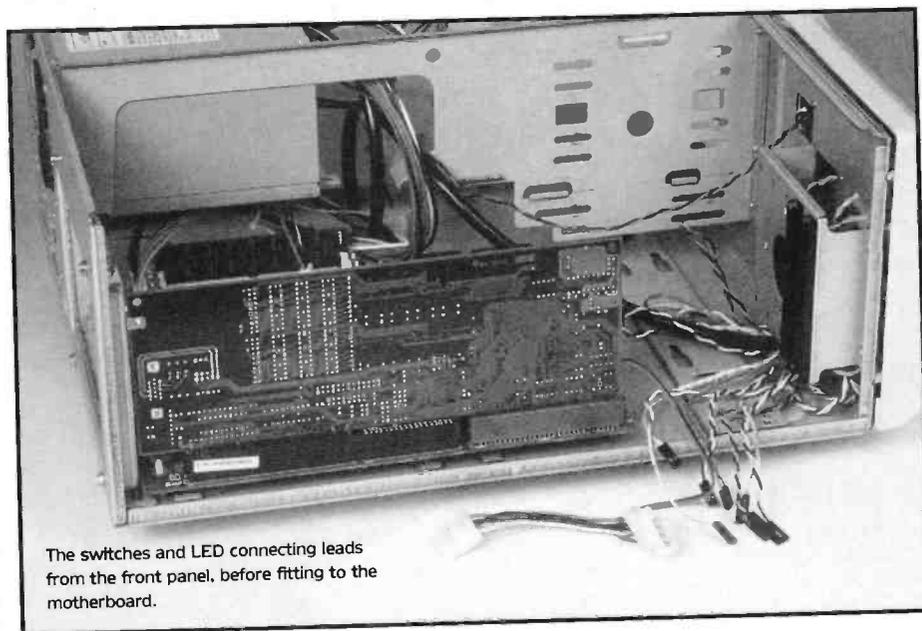
The switches and LED connecting leads from the front panel, before fitting to the motherboard.
