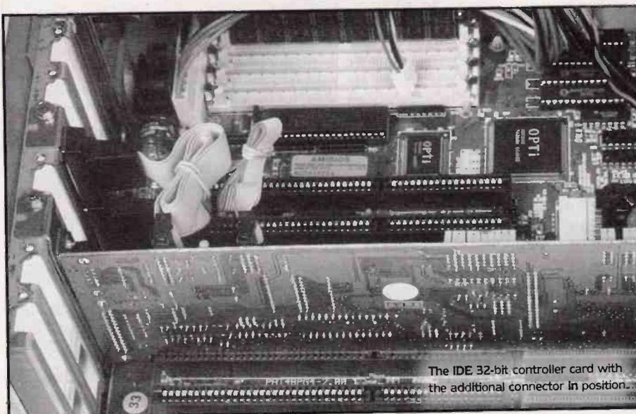
The IDE 32-bit controller card with the additional connector in position.
