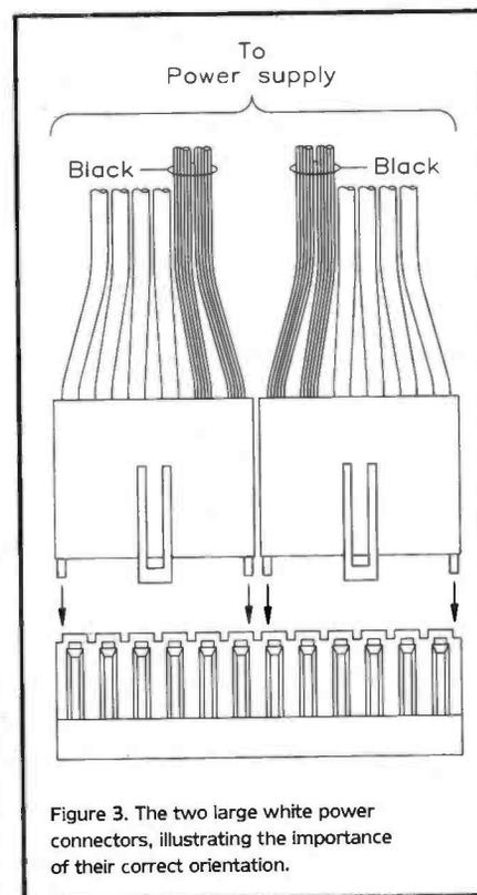
Figure 3. The two large white power connectors, illustrating the importance of their correct orientation.
