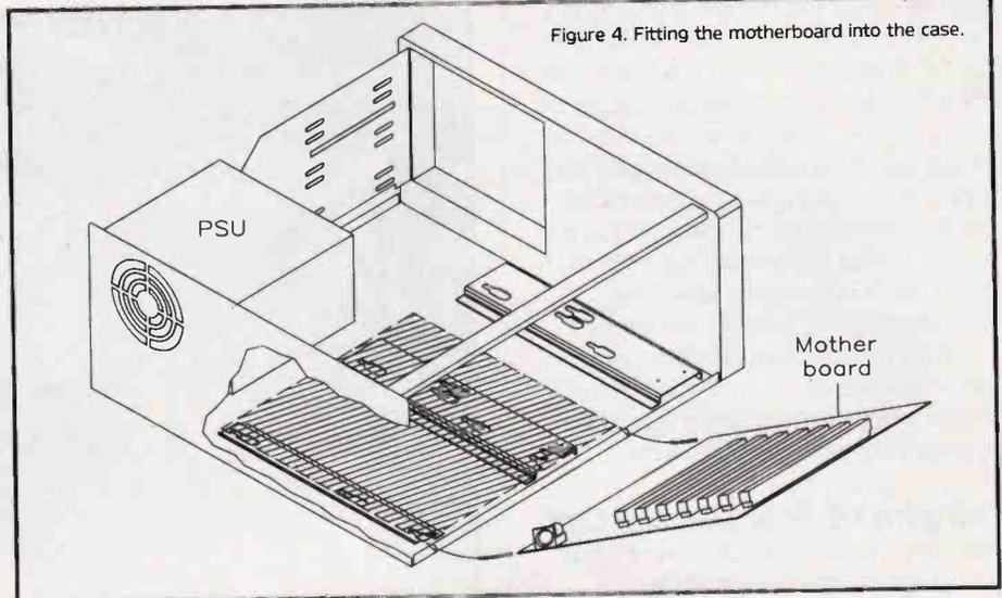
Figure 4. Fitting the motherboard into the case.
