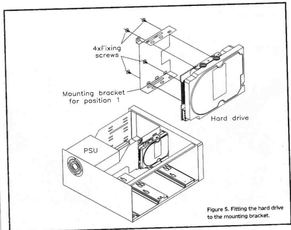
Figure 5. Fitting the hard drive to the mounting bracket.
