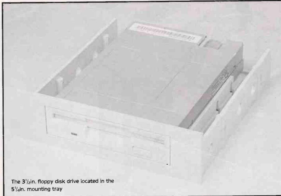
The 3 1/2 in. floppy disk drive located in the 5 1/4 in. mounting tray
