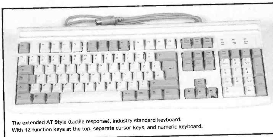
The extended AT Style (tactile response), industry standard keyboard. With 12 function keys at the top, separate cursor keys, and numeric keyboard.
