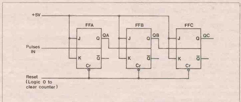
Figure 5. Scale-of-eight asynchronous (ripple-through) counter.
