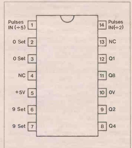
Figure 10. The 7490 decade counter chip.
