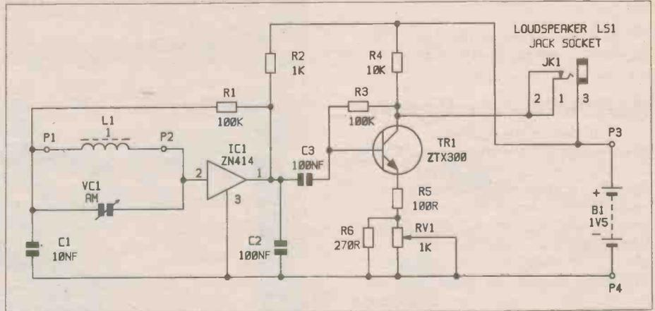
Figure 3. Earphone Radio circuit.
