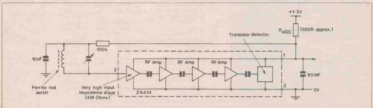
Figure 1. The ZN414 (within chain outline) in its most basic circuit configuration.
