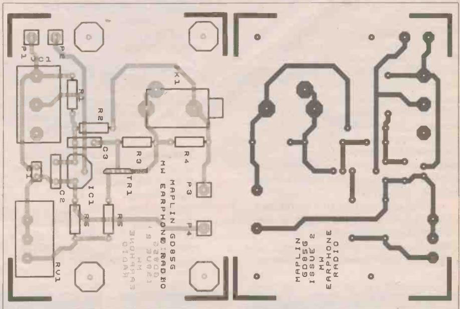
Figure 5. Track and overlay of PCB.
