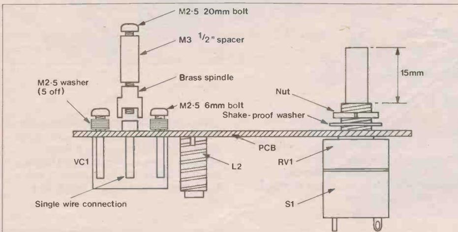
Figure 5. Spindle Preparation
