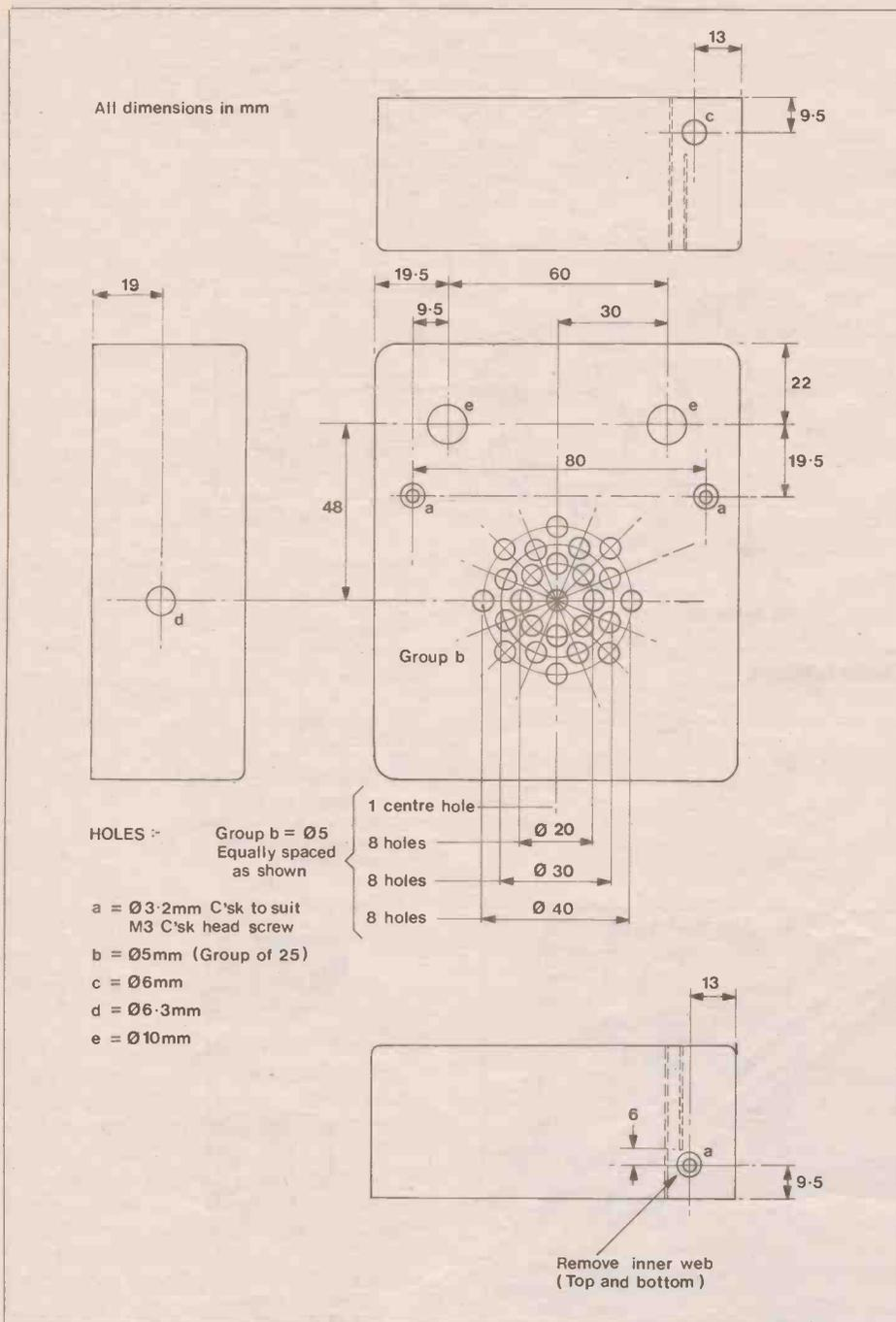
Figure 8. Box Drilling
