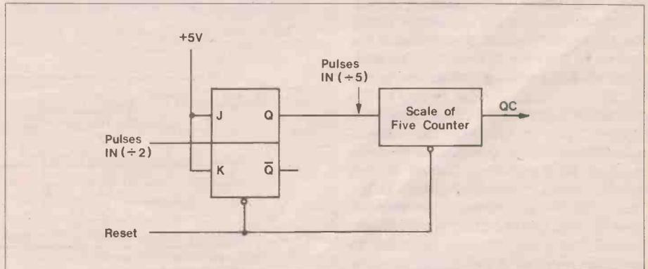
Figure 9. Decade counter constructed from basic divide-by-two stage and the circuit of Figure 8.
