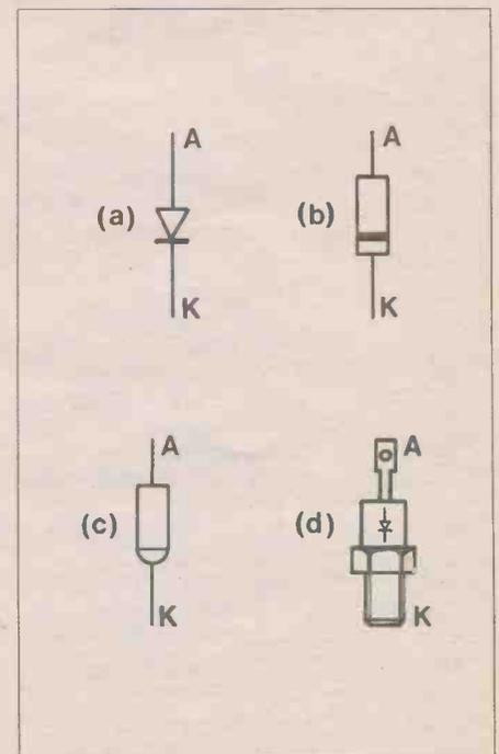
Figure 2. a) Diode symbol, b) 1 amp case, c) 3 amp case, d) Stud mounted, over 5 amp.
