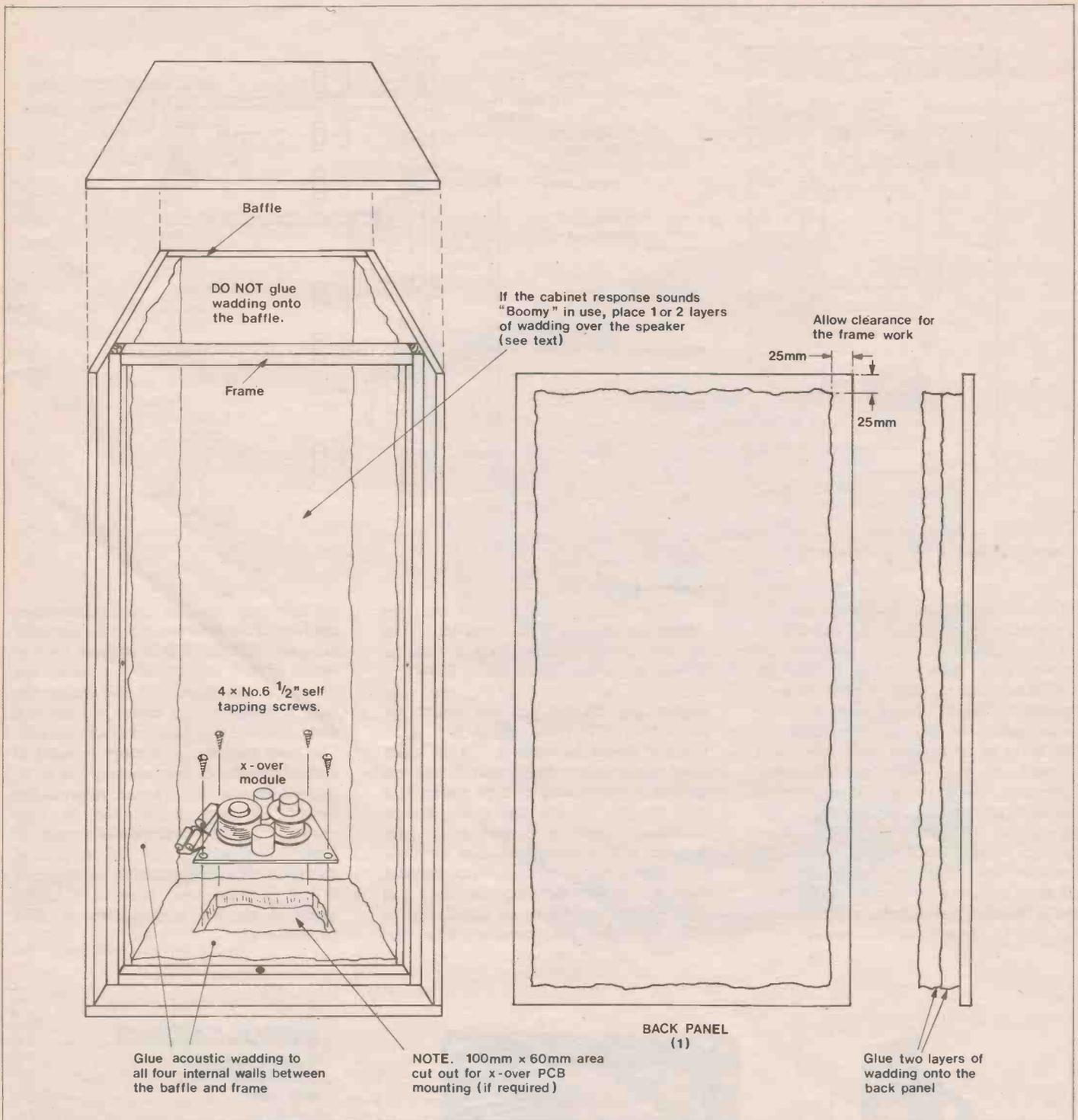
Figure 8. Fitting wadding and crossover unit.
