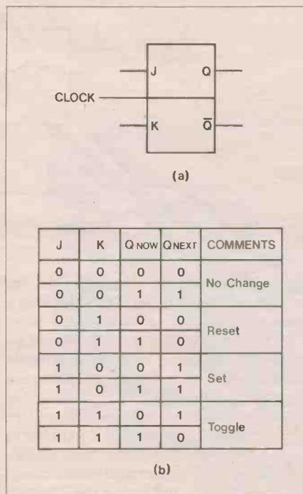
Figure 1. The JK Flip-flop, symbol (a) and truth table (b).
