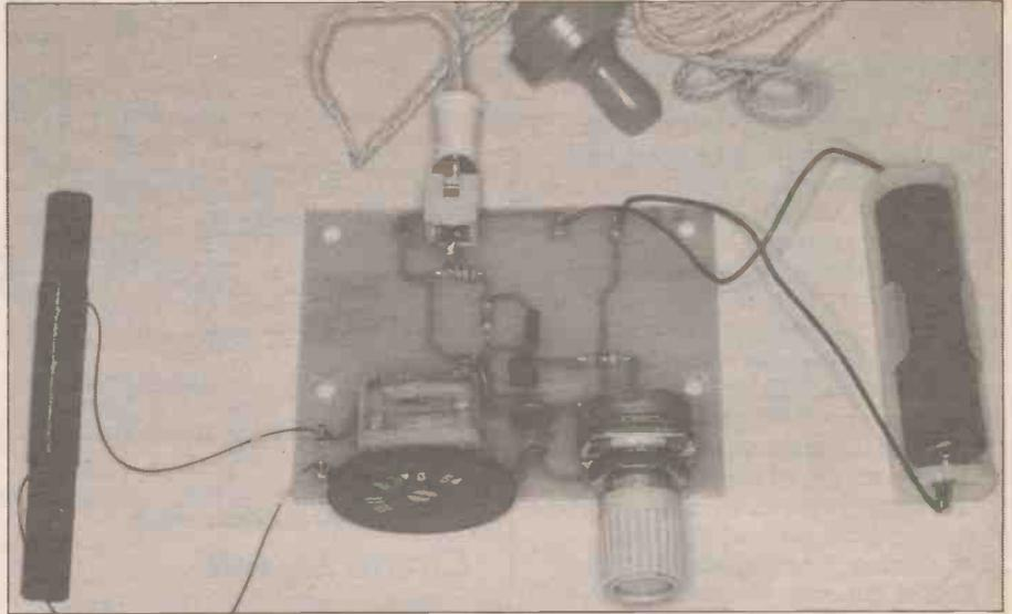
Photo 3. The fully assembled receiver, showing how simple it is!
