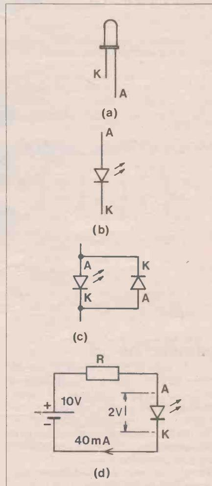
Figure 4. a) LED outline, b) symbol, c) Protected LED, d) Calculation for series resistor.
