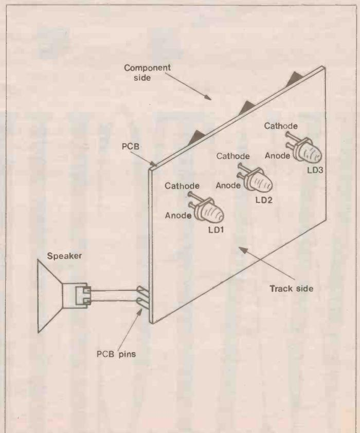
Figure 3. Mounting the LEDs.
