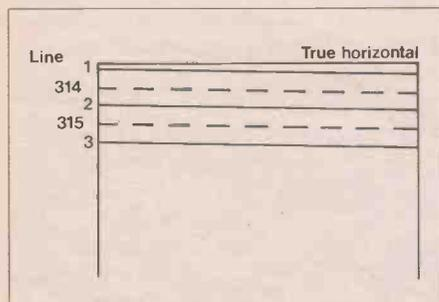
Figure 1. Principle of scanning: The first lines of two consecutive interlaced fields in a 625 line system.
