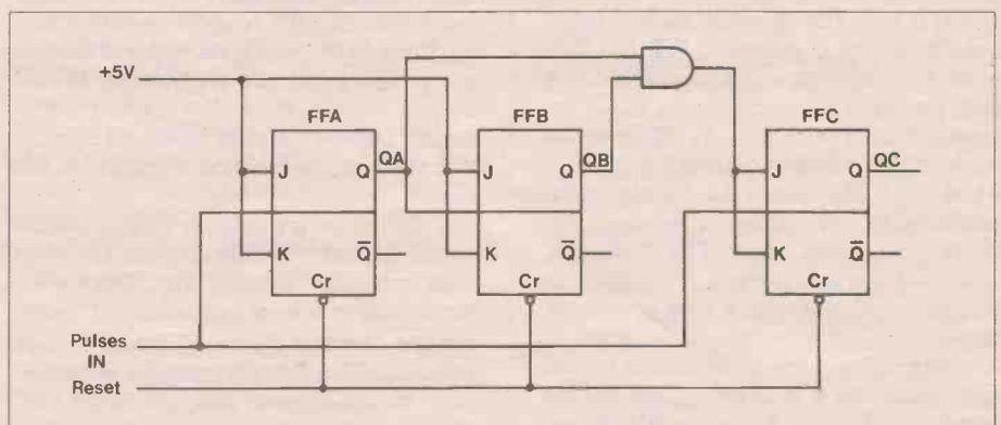
Figure 6. Scale-of-eight synchronous counter.
