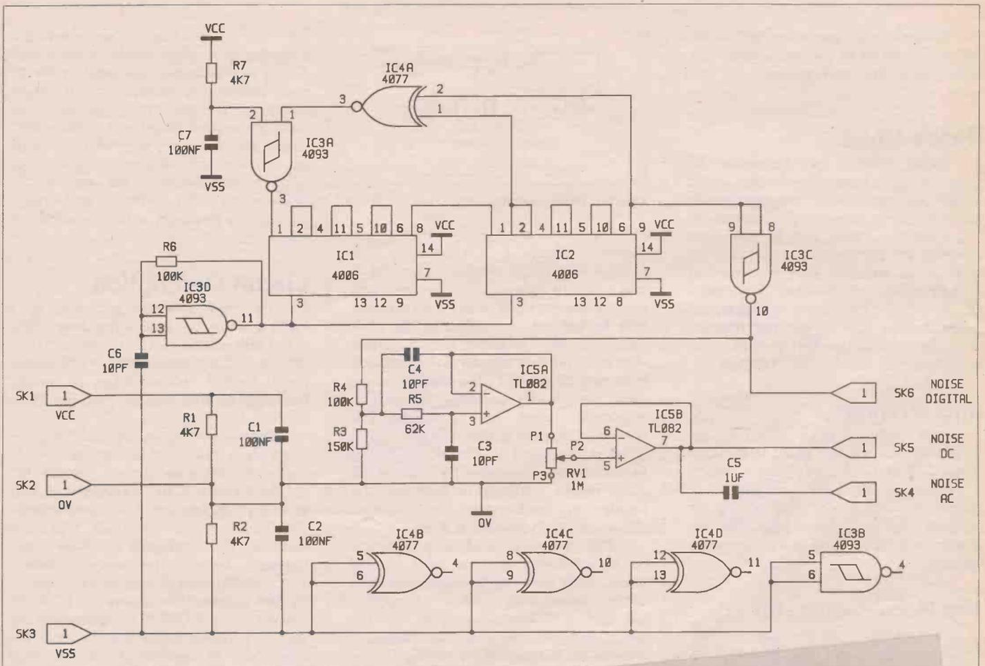
Figure 2. Noise generator circuit.
