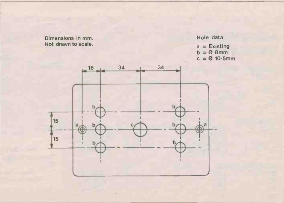
Figure 5. Case lid drilling details.
