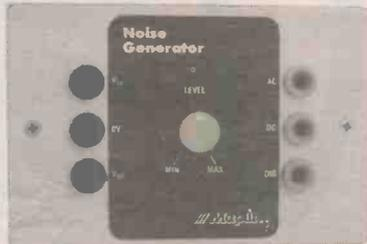
The main use of a Noise Generator is in testing equipment on the bench which will be used in noisy environments in the field. An in-depth discussion on the types of noise to be encountered is also given.
