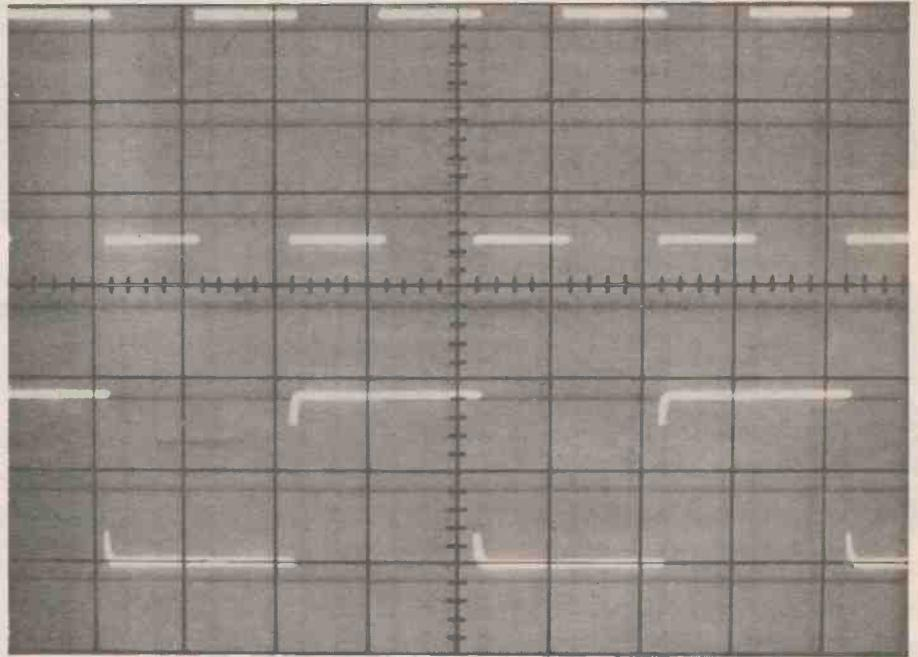
Photo 1. Oscilloscope traces for clock input (upper waveform) and Q output (lower waveform) of a JK flip-flop wired in the 'toggle' mode. Note that the Q output changes only when the input goes 'down', hence the divide-by-two action.
