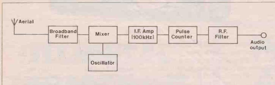
Figure 1. Block Diagram
