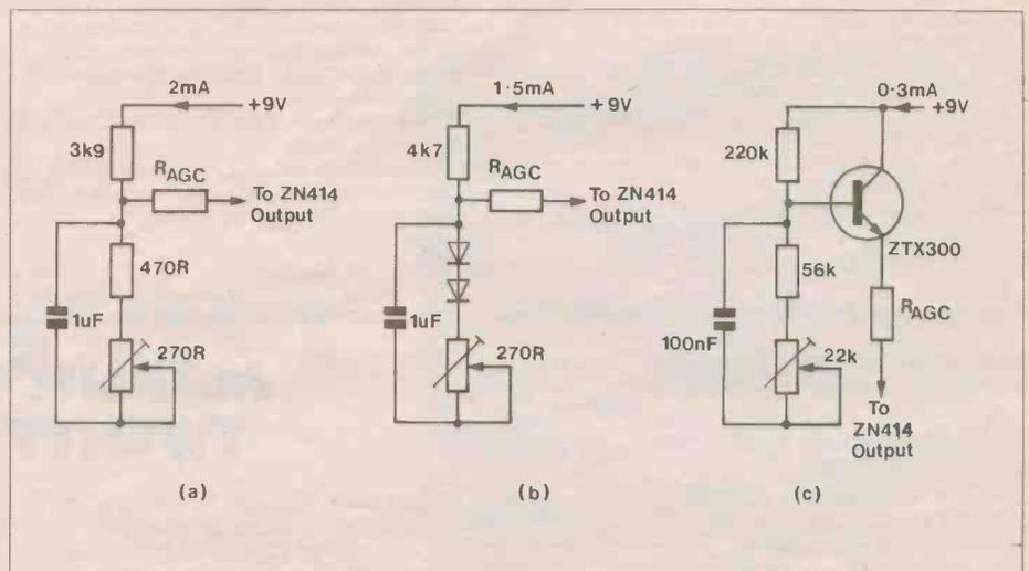
Figure 2. Drive circuits for the ZN414, (a) Resistor network, (b) Diode drive, (c) Transistor drive. In all cases the preset is a sensitivity control.
