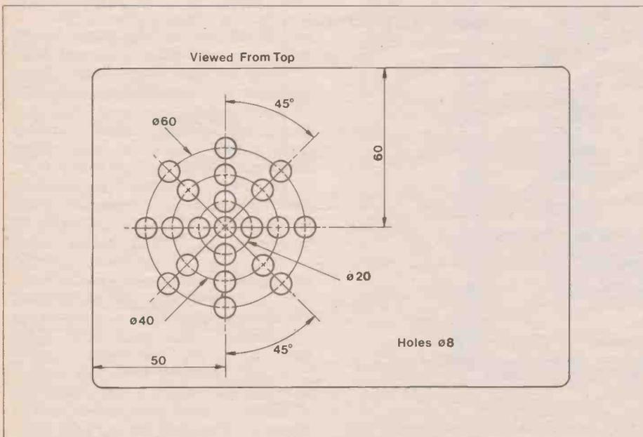
Figure 8. Box lid drilling
