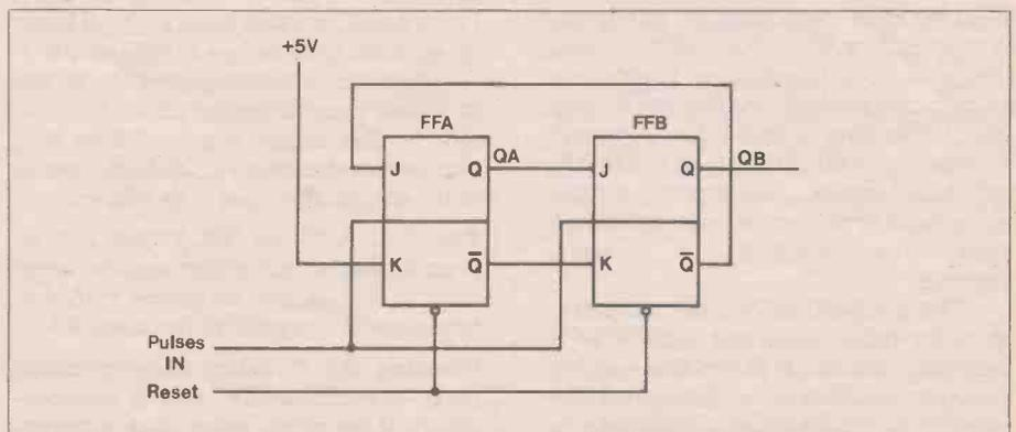
Figure 7. Scale-of-three feedback counter.
