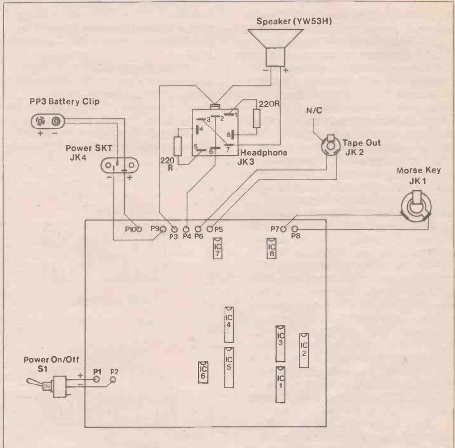
Figure 5. Wiring diagram
