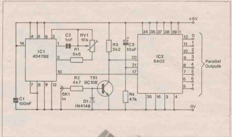
Serial/Parallel Converter Circuit
