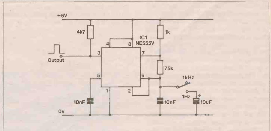
Figure 3. TTL 1Hz/1kHz oscillator.
