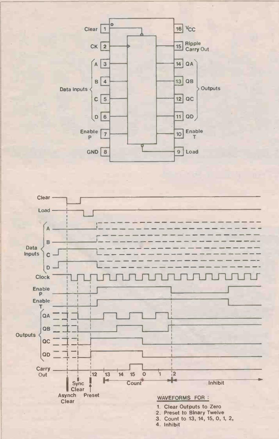
Figure 11. The SN74160-3 programmable counters.
