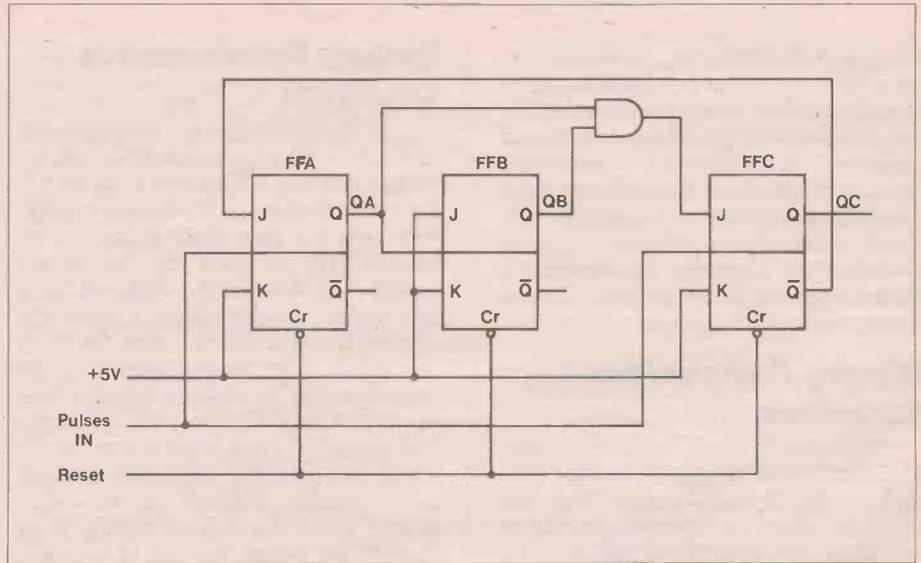
Figure 8. Scale-of-five feedback counter.
