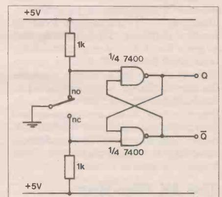
Figure 4. De-bounced switch with complementary outputs.
