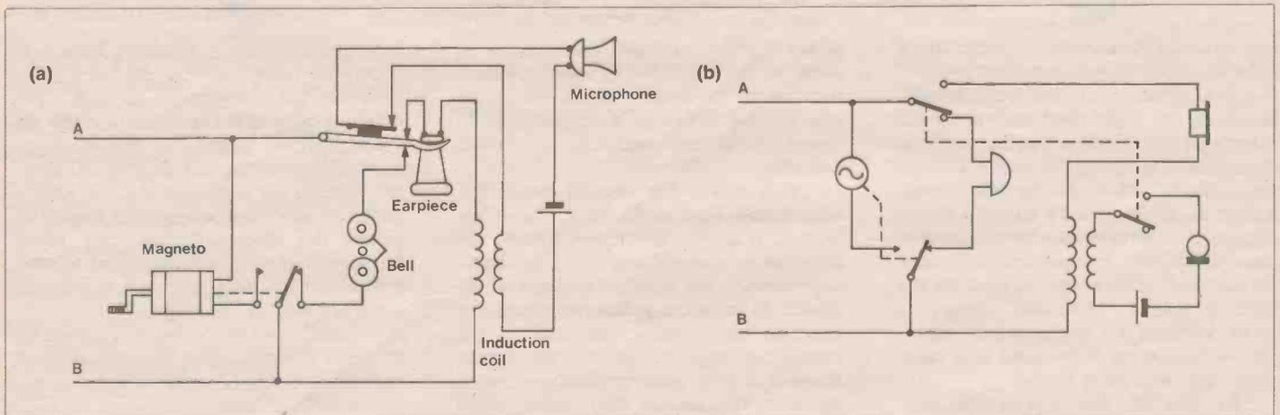
Figure 4. The Telephone No. 11 circuit (a) as it would have been drawn at the time, (b) redrawn with modern symbols.
