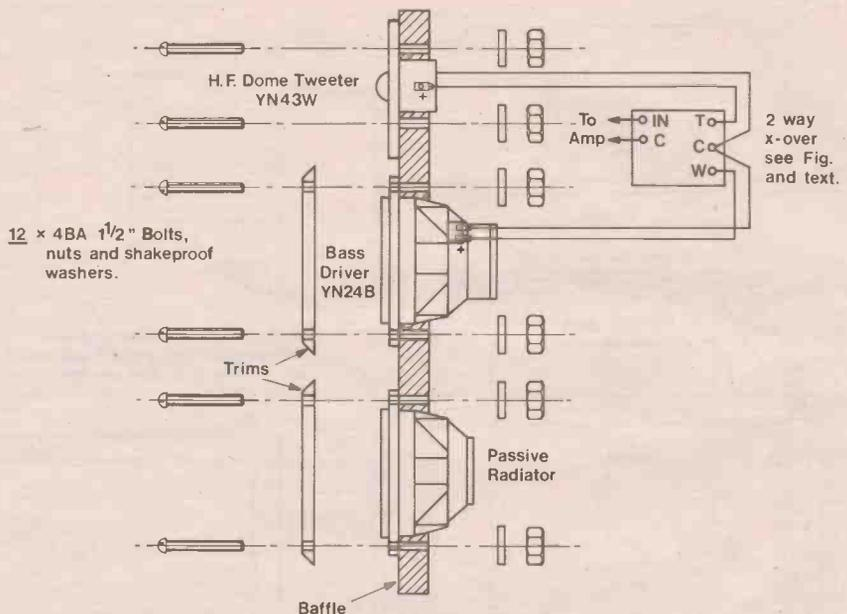
Figure 9. Installing the loudspeakers.
