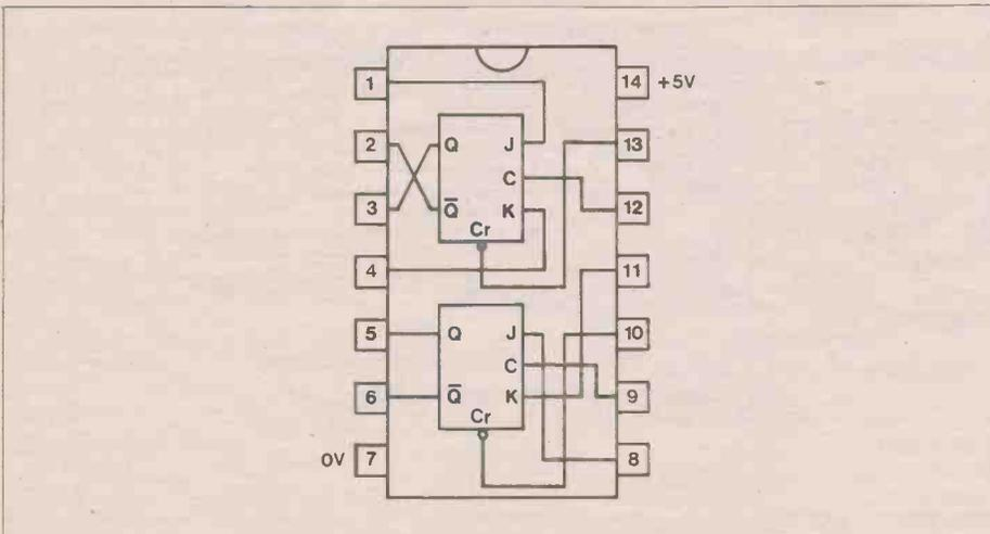
Figure 12. Pin-out for 74107 dual JK level-triggered flip-flops.
