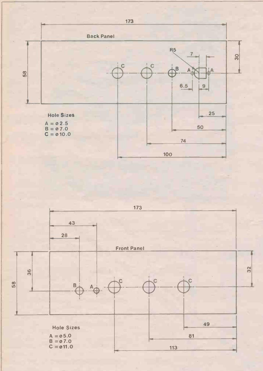
Figure 7. Front and back panel drilling
