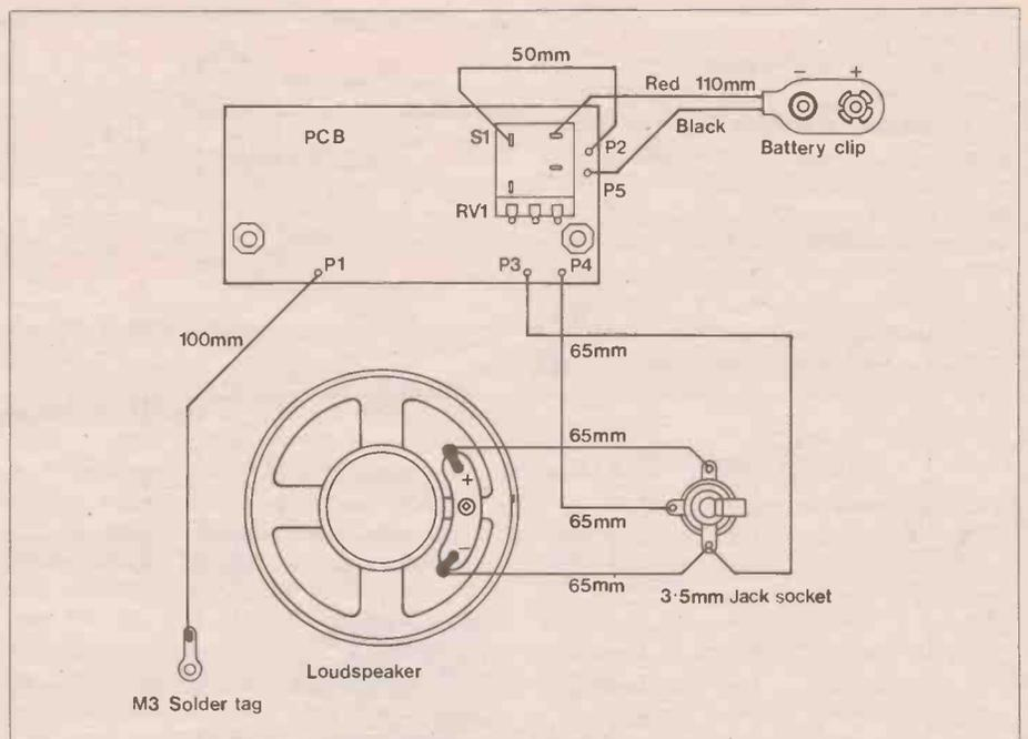
Figure 6. Wiring
