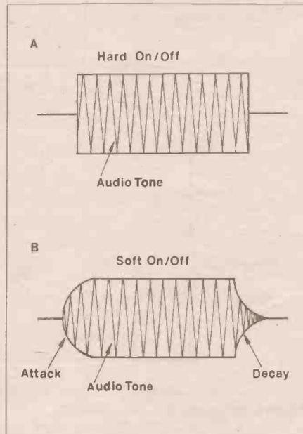
Figure 3. Morse signal envelope shaping
