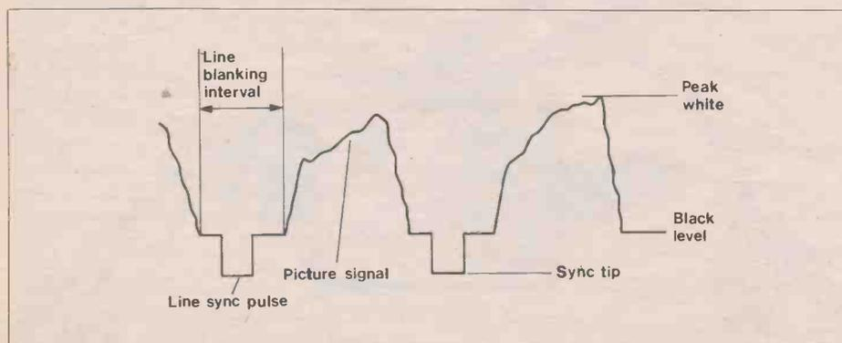
Figure 2. Video signal waveform showing line sync pulses and line blanking interval.
