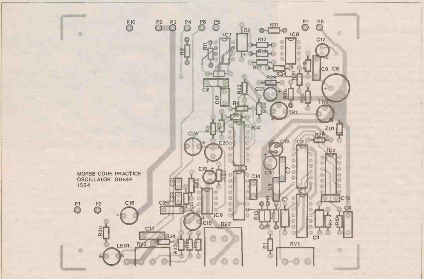
Figure 4. Track and layout of the PCB
