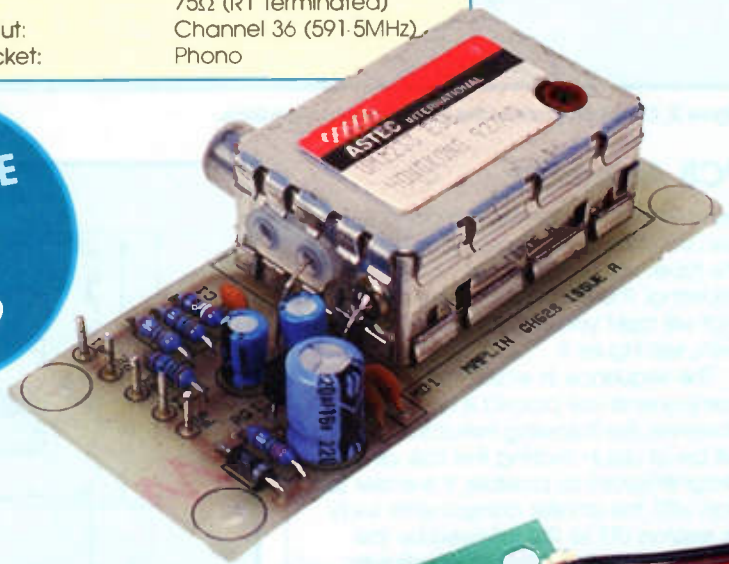
The assembled CCD Camera Modulator PCB.
