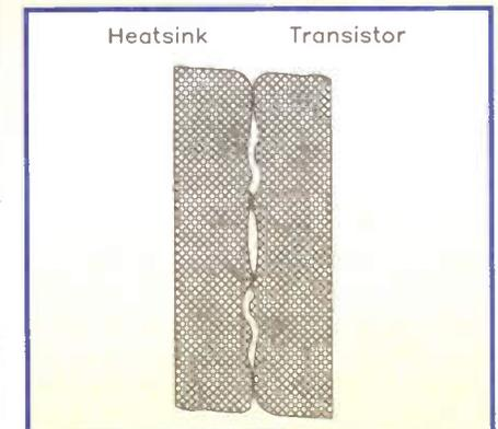
Figure 4. Typical microscopic appearance of the contact interface between a power device and a heatsink.
