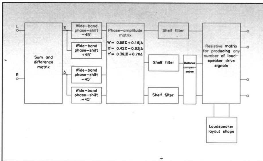
Figure 17b. Example of an Ambisonics decoder with 2-channel input.
