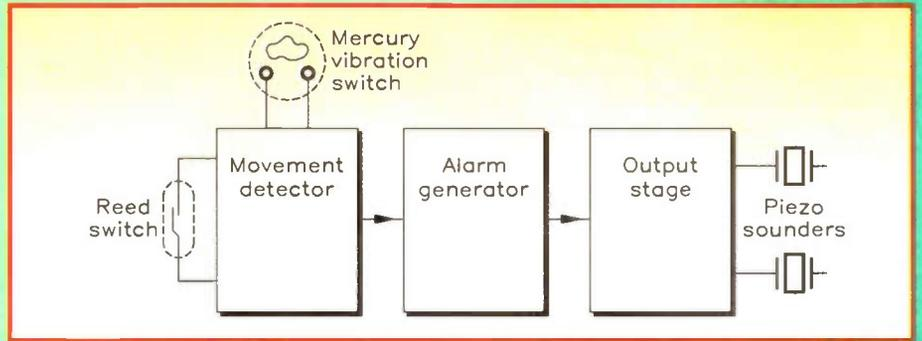
Figure 1. The ATD block diagram.
