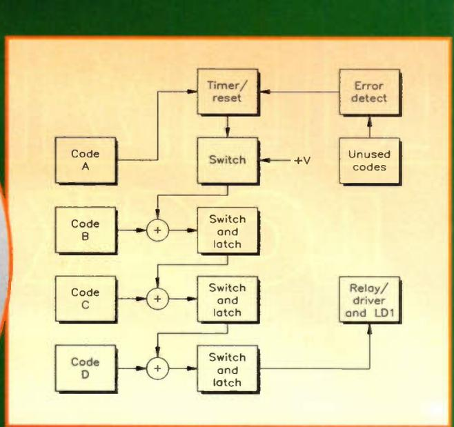
Figure 1. The block diagram of the Keycode Lock.
