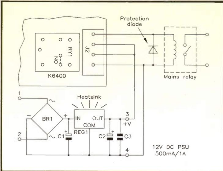
Figure 7. Mains relay and suitable DC PSU.
