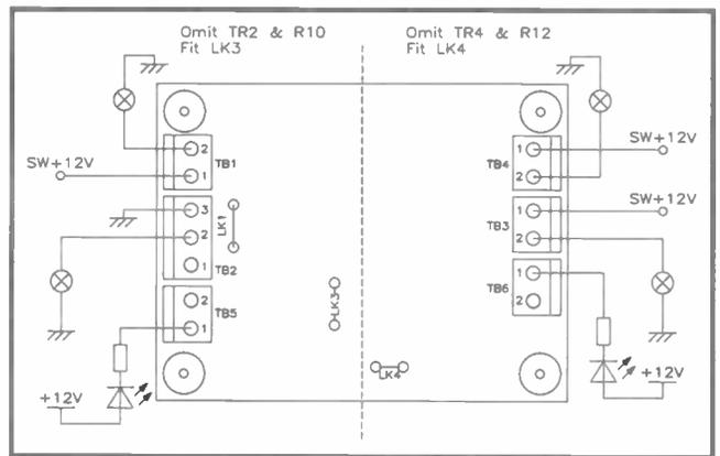
Figure 7b. Shared fault indicator LEDs for pairs of lamps.
