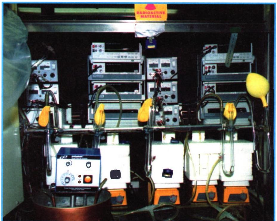
Bush and Eagleton's laboratory; electrolytic cells utilising Palladium on Silver substrate in Lithium Deuteride.
