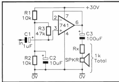
Figure 2. Low-power amplifier using a single-ended power supply.
