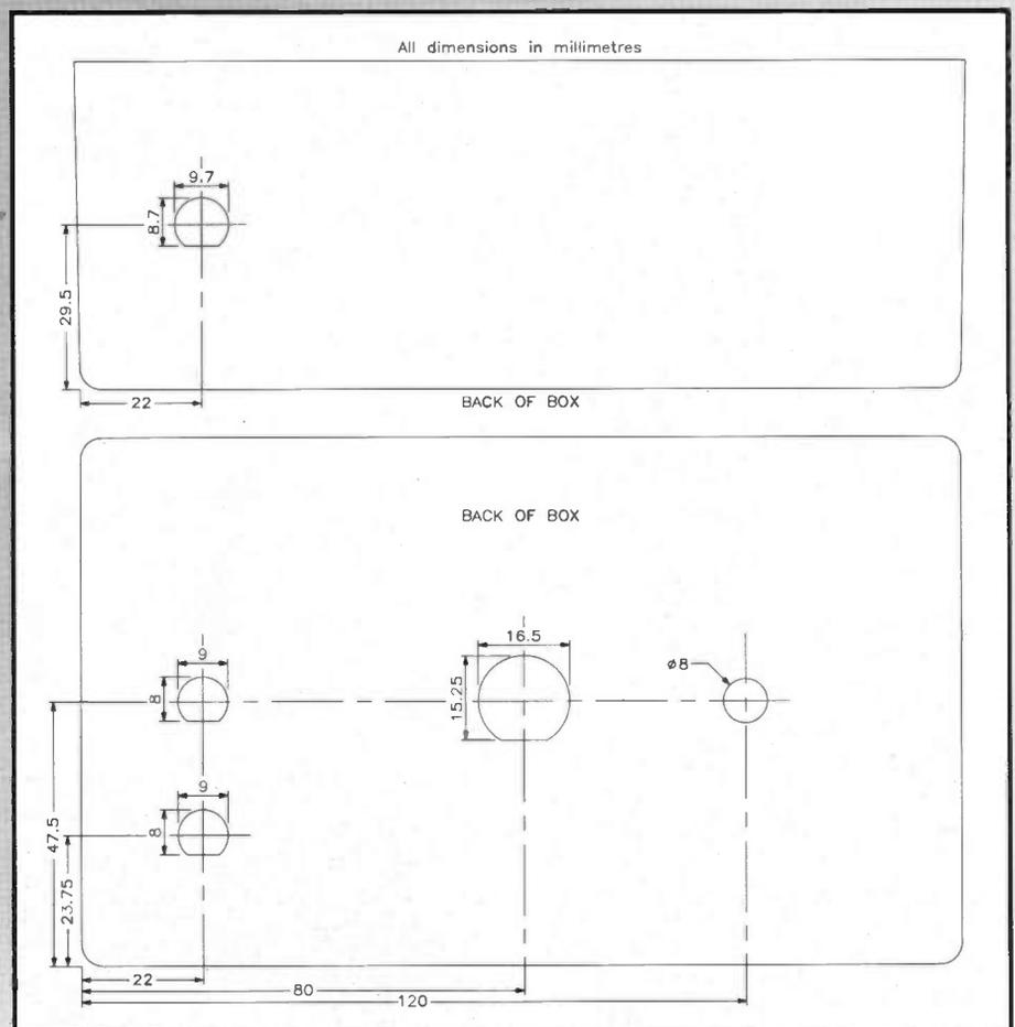
Figure 5a. Case drilling.
