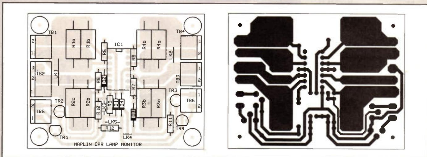
Figure 4. Car Lamp Monitor PCB legend and track.
