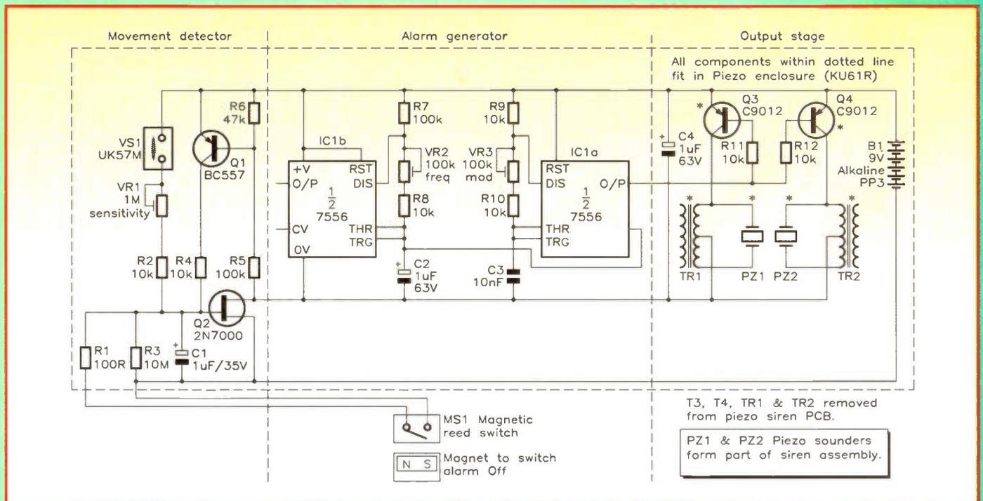
Figure 2. The ATD circuit diagram.
