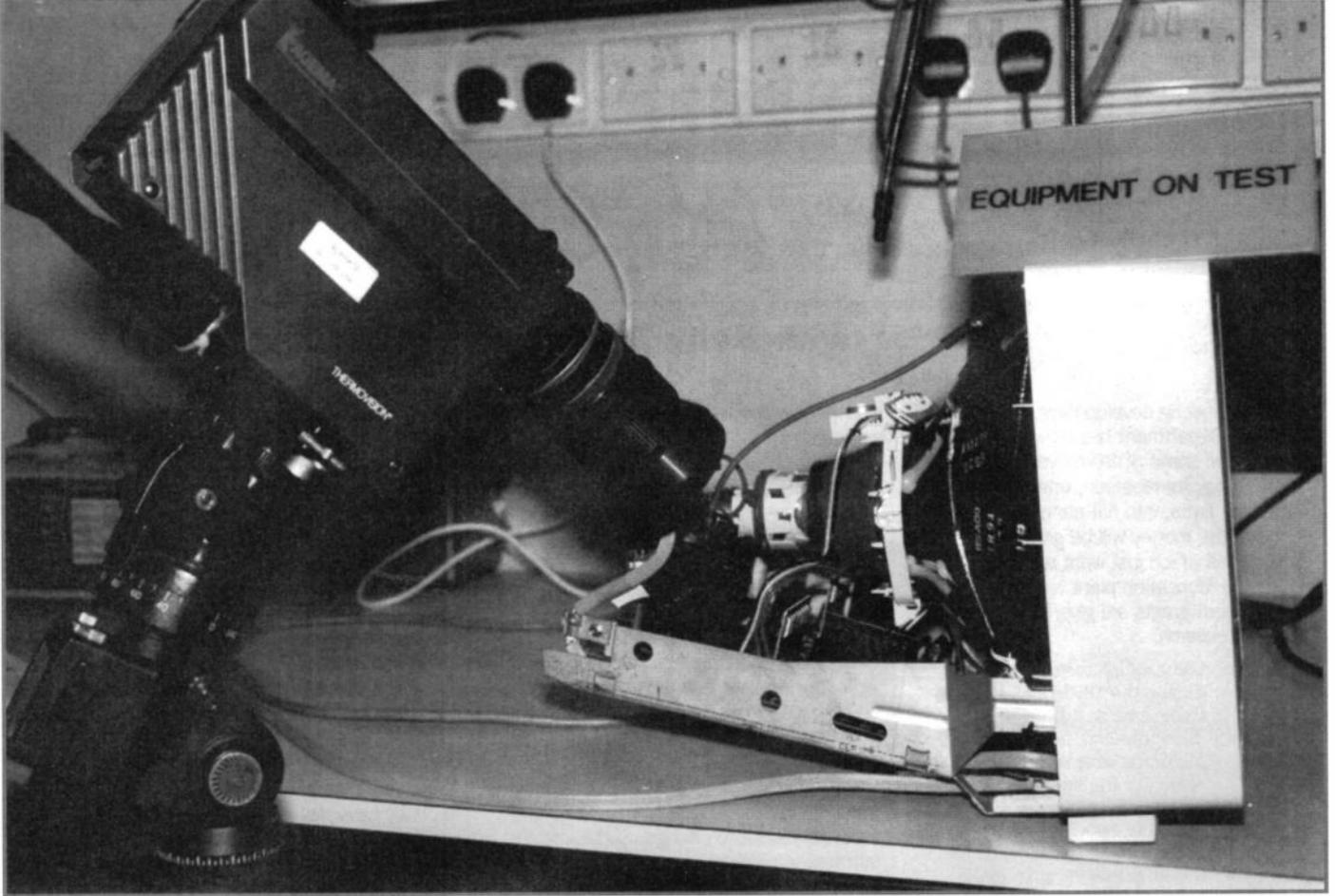
Photo 2. The test set-up for monitoring thermal images from the PCBs in a visual display unit, using the Thermovision 800 at IBM in Greenock.
