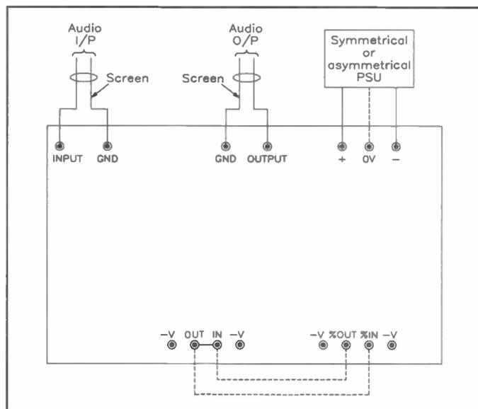
Figure 10. PCB connection diagram.
