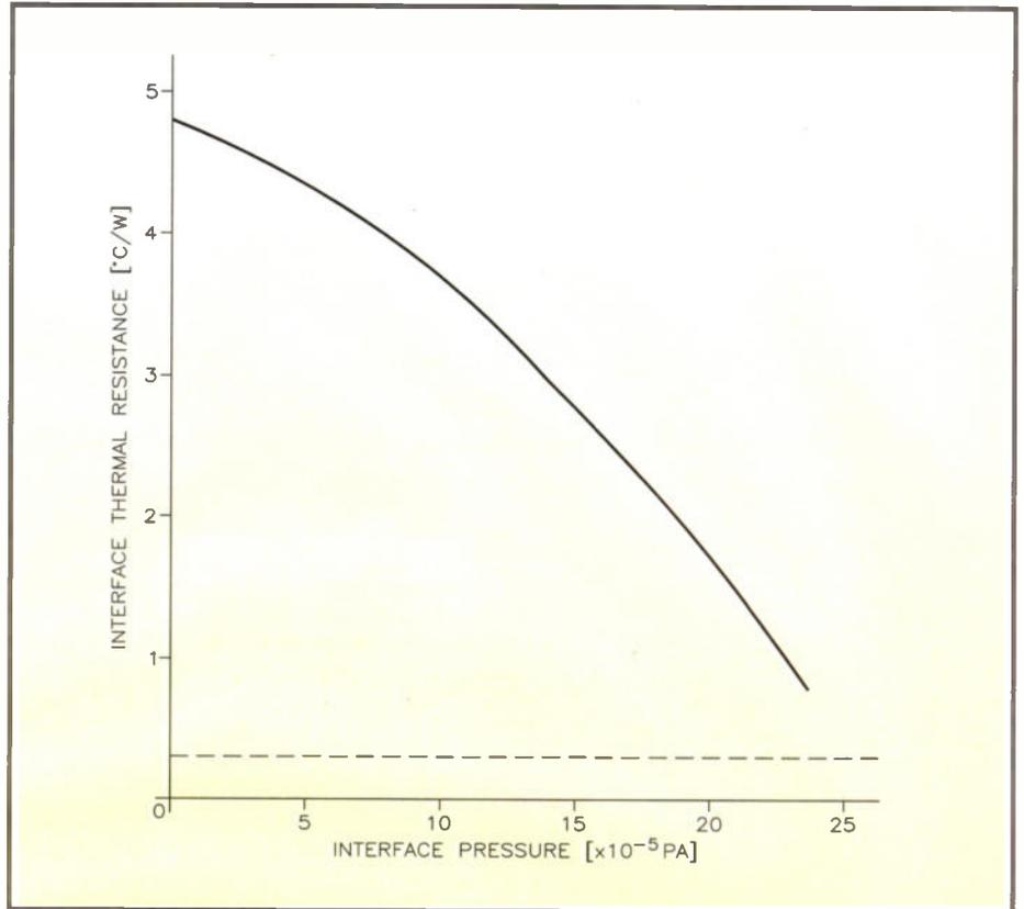
Figure 5. The effects of pressure and heat transfer grease on thermal resistance, when applied to the interface between a power device and heatsink.
