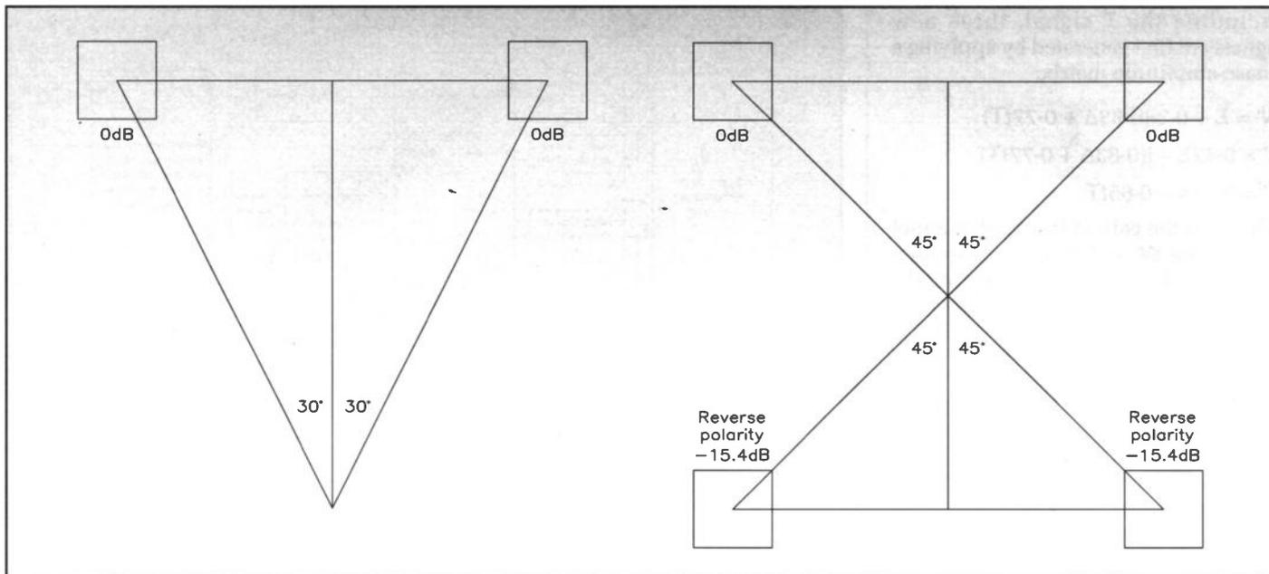
Figure 16. Optimum loudspeaker layouts for stereo and 2-channel Ambisonics.
