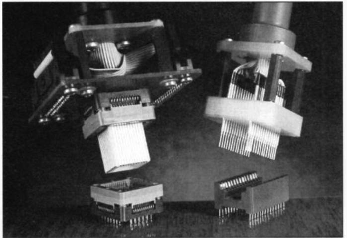
Now available from Peak is a range of test probe blocks for use with PLCC and DIP integrated-circuit sockets in burn-in and emulation applications.
