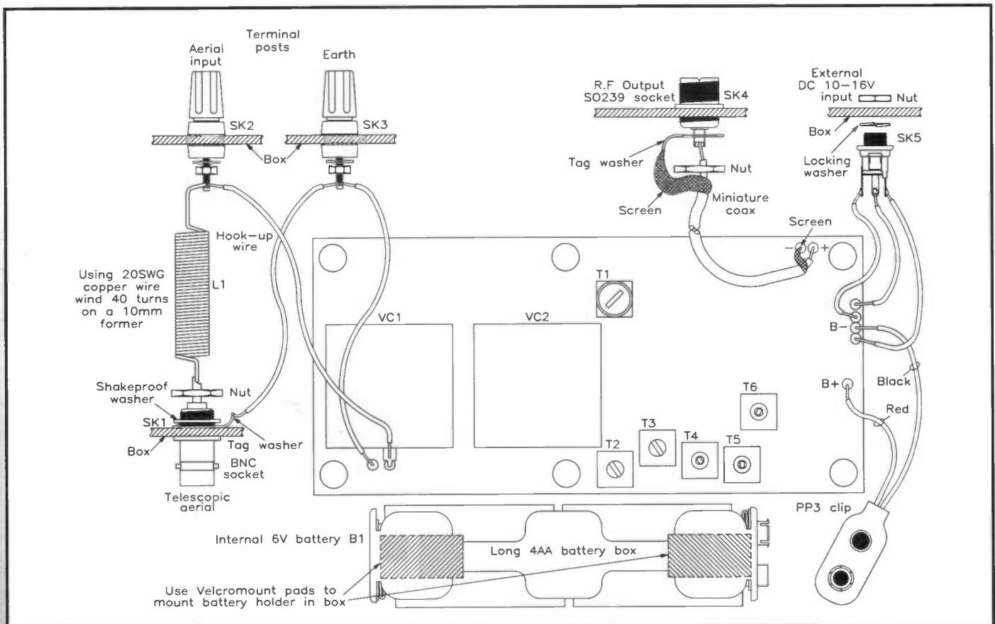
Figure 7. Wiring diagram of the Aerial Activator.
