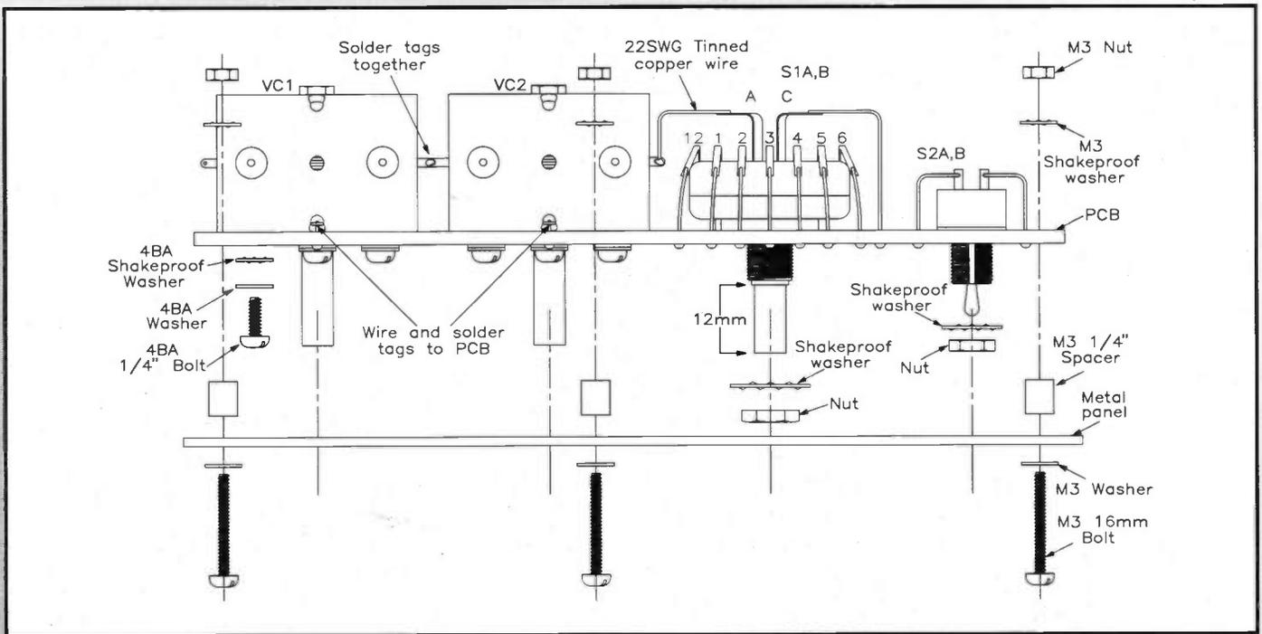
Figure 4. Variable capacitors and switches - mounting and wiring.
