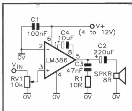
Figure 10. LM386 amplifier with AV = 200.
