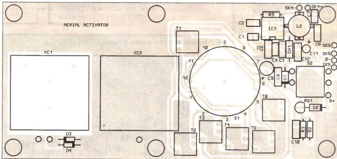
Figure 3. PCB legend and track (please note that this design employs a double-sided PCB with component side ground plane.,
