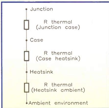
Figure 3. Electrical representation of a simple single power device thermal system.
