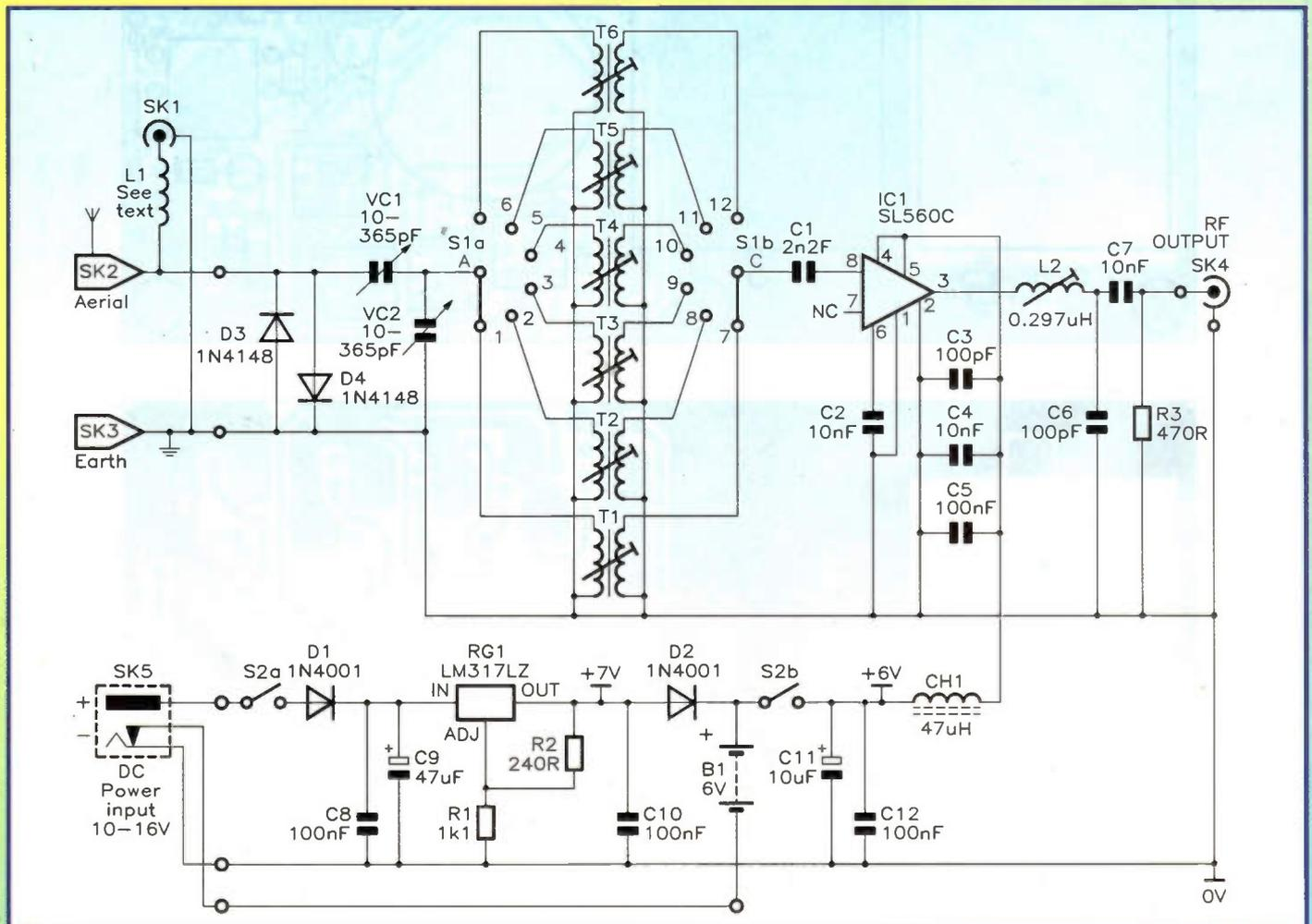
Figure 2. Circuit diagram of the Aerial Activator.
