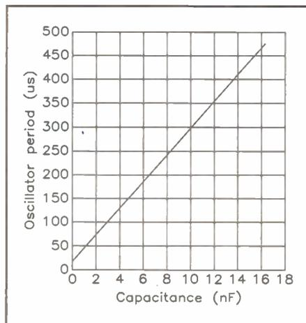
Figure 2(a). Internal oscillator period vs. capacitance value.
