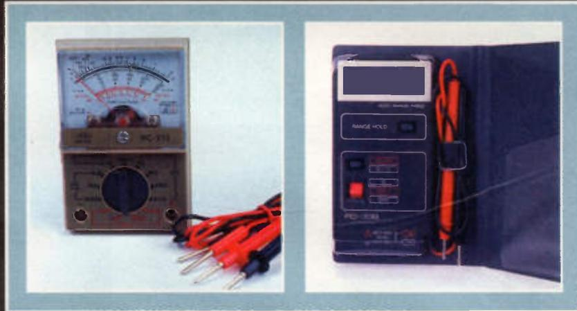
Above: A couple of inexpensive basic analogue and digital multimeters.
