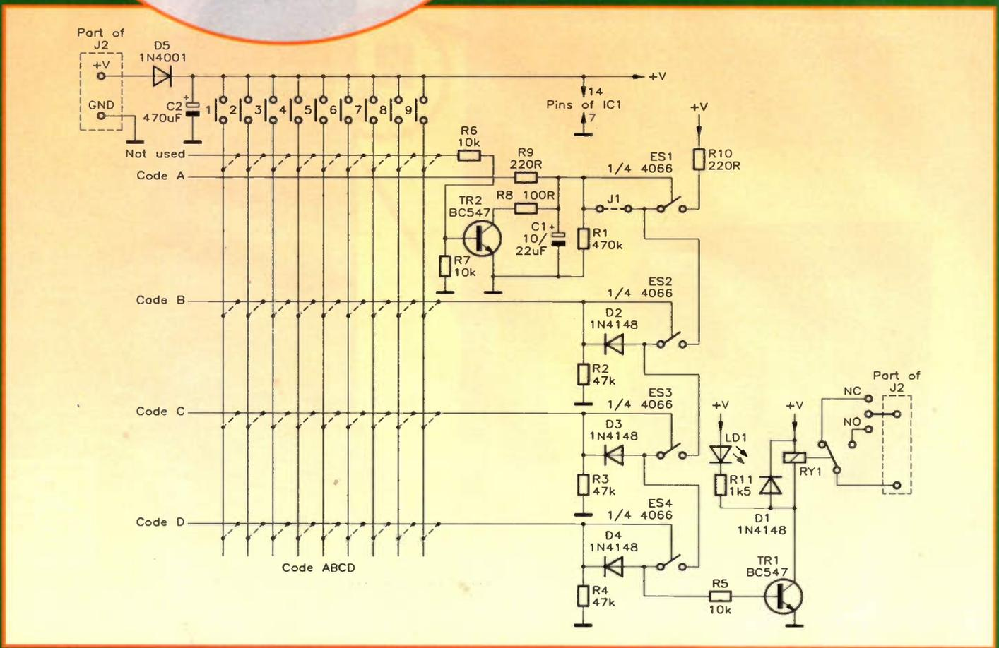
Figure 2. The circuit diagram of the Keycode Lock.
