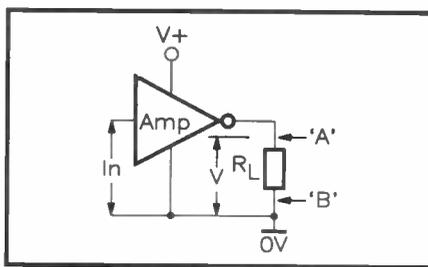
**Figure 6. An amplifier connected in the 'single ended output' mode gives a peak output of  $V^2 \div R$  watts.**
