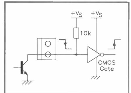
Figure 8. Interfacing the Car Lamp Monitor to CMOS logic.
