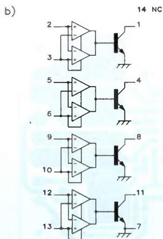
Figure 1. Block diagram/pinout of ULM2455A.
