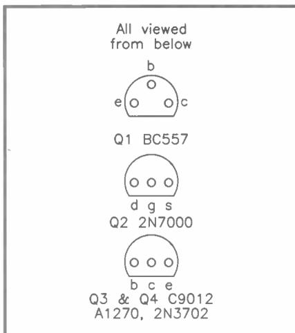
Figure 5. Transistor bases.
