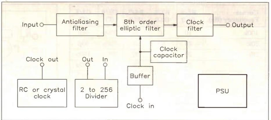
Figure 7. MAX293/297 block diagram.
