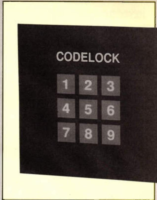
Photo 3. The membrane front panel.
