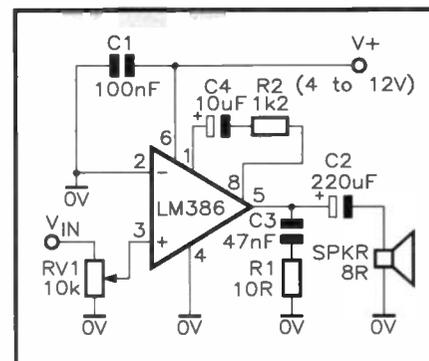
Figure 11. LM386 amplifier with AV = 50.
