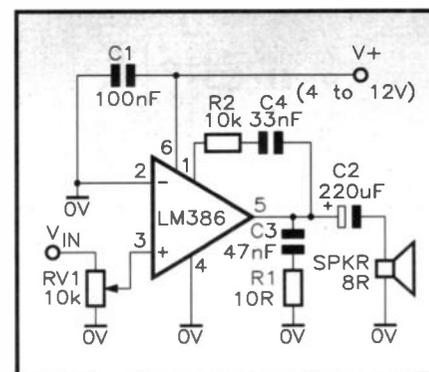
Figure 12. LM386 amplifier with 6dB of bass-boost at 85Hz.
