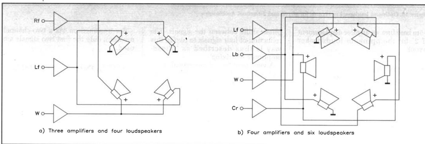
Figure 18. Arrangements of amplifiers and loudspeakers for Ambisonics.
