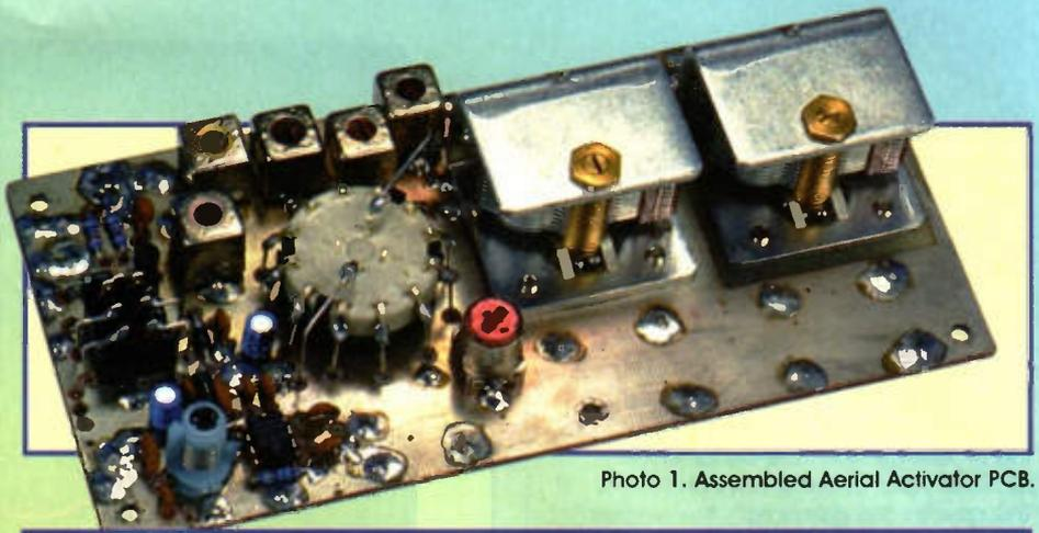
Photo 1. Assembled Aerial Activator PCB.
