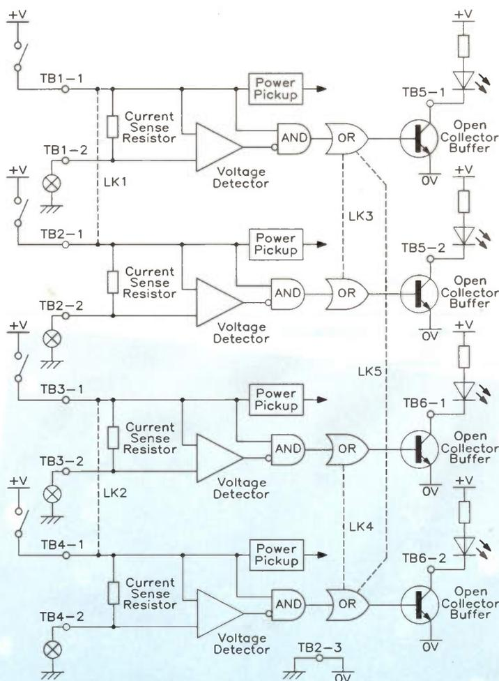
Figure 2. Block diagram of the Car Lamp Monitor.
