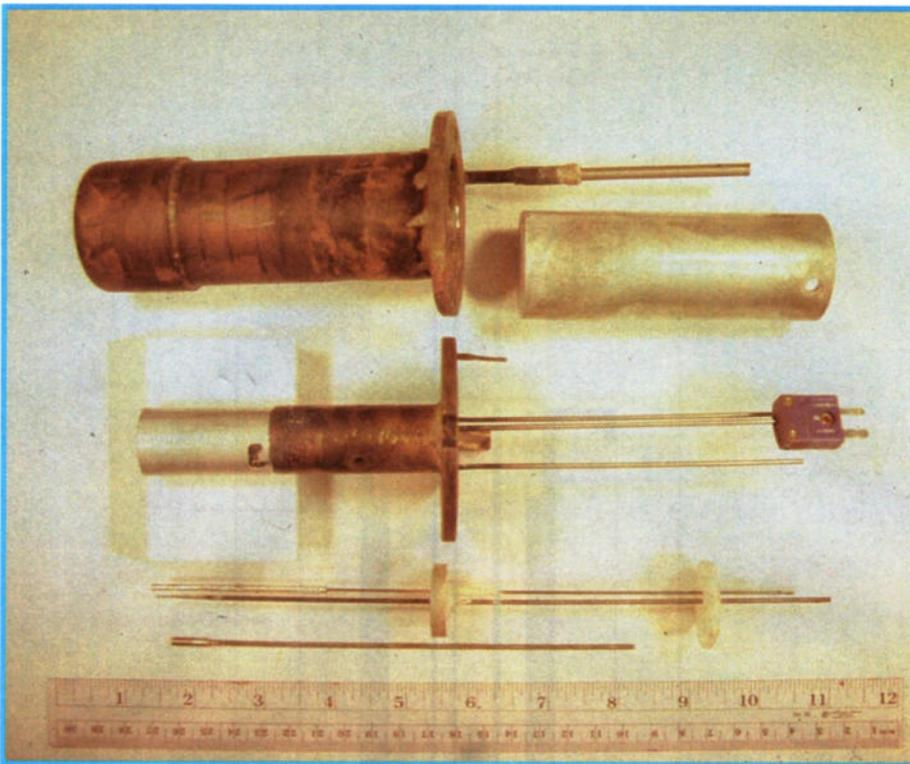
The cell used in a previous experiment using molten salt electrolyte. University of Hawaii at Manoa.
