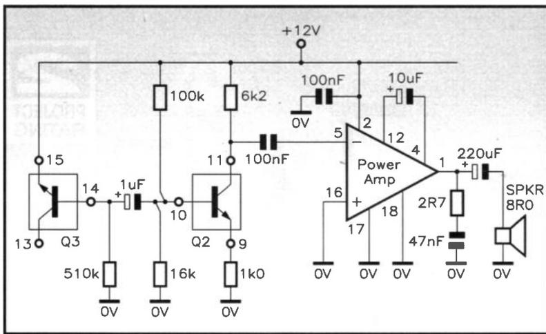
Figure 17. LM389 white-noise sound generator.
