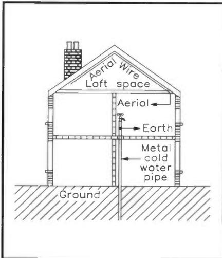
Figure 8c. Typical indoor loft aerial system.
