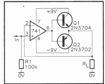
Figure 3. Basic 'boosted output current' unity-voltage-gain op amp circuit.
