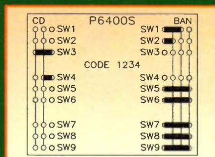
Figure 3. The wire links set up for code '1234'.
