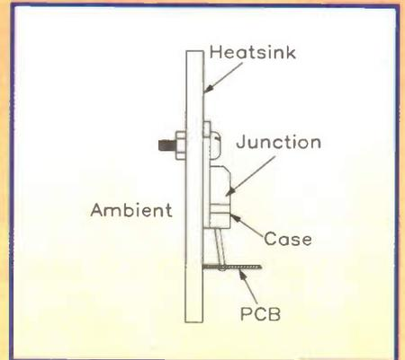
Figure 2. Heat transferring interfaces within a semiconductor system.
