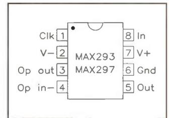
Figure 1(a). MAX293/297 pin connections.
