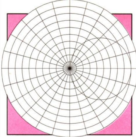
Figure 12a. Impossible half-lemniscate directional response required for correct capture of '4-channel stereo'.
