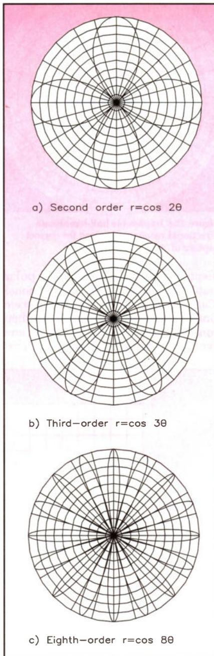
Figure 14. Higher-order spherical harmonics.
