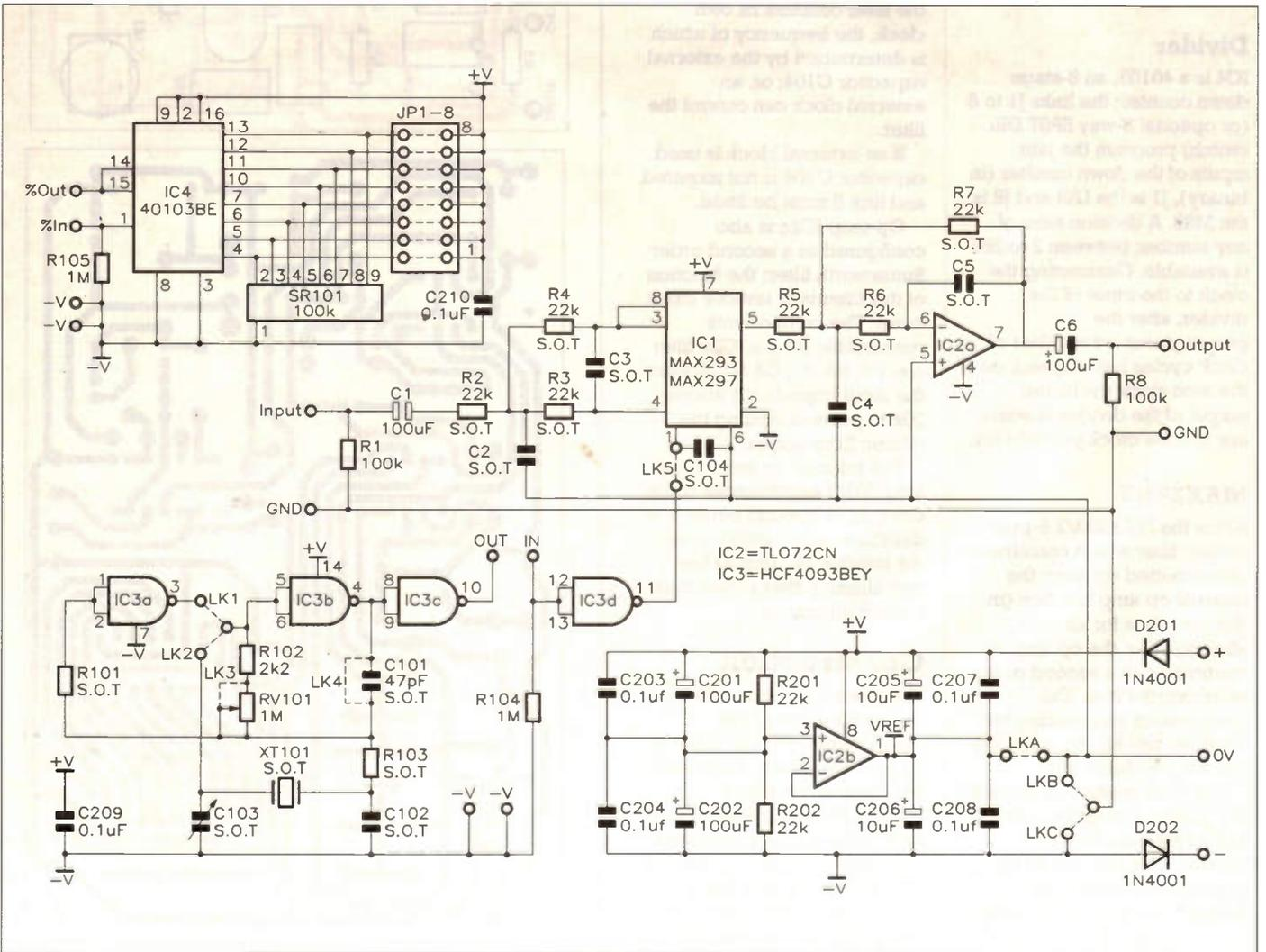
Figure 8. MAX293/297 circuit diagram.
