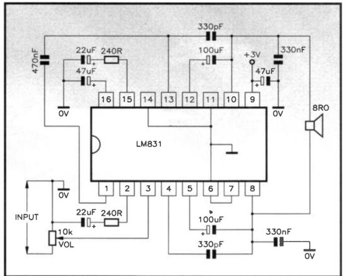
Figure 20. Bridge-connected LM831 amplifier.
