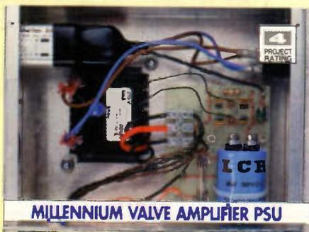
**MILLENNIUM VALVE AMPLIFIER PSU**
