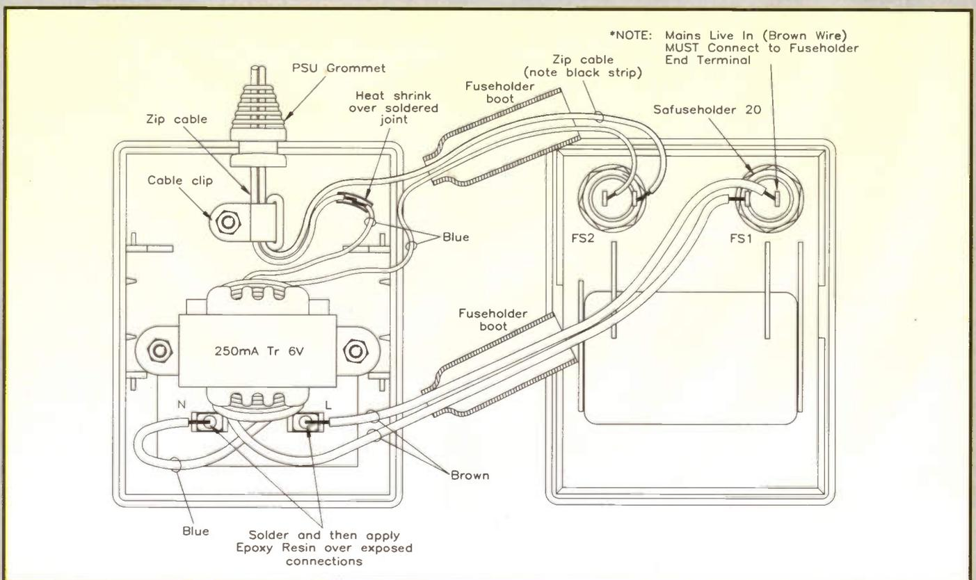
Figure 6c. PSU assembly details.
