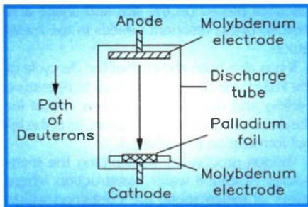
Figure 3. Glow discharge system of cold fusion. Excess powers of at least 300% have reported using this technique.
