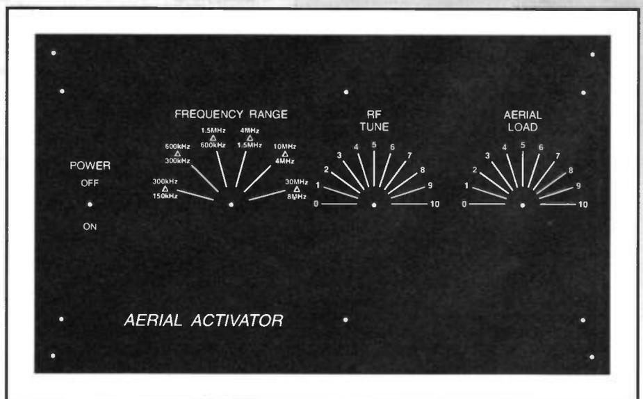
Figure 6. Front panel label (2/3 scale).
