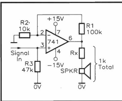
Figure 1. Low-power amplifier using dual power supplies
