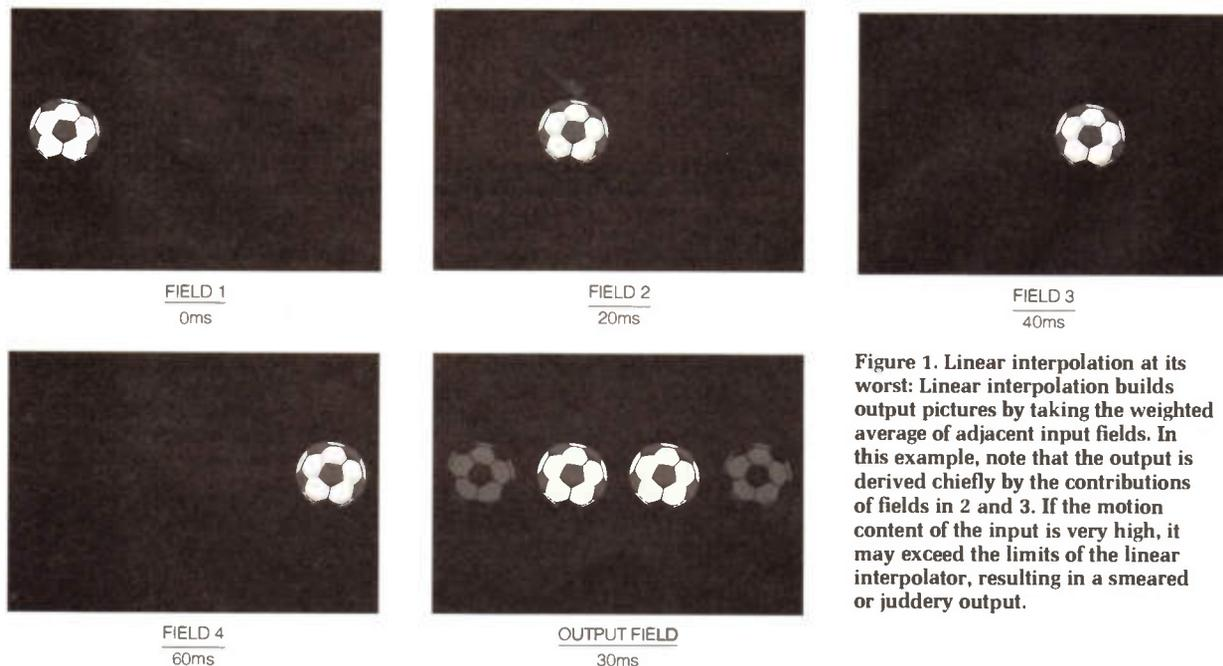
Figure 1. Linear interpolation at its worst: Linear interpolation builds output pictures by taking the weighted average of adjacent input fields. In this example, note that the output is derived chiefly by the contributions of fields in 2 and 3. If the motion content of the input is very high, it may exceed the limits of the linear interpolator, resulting in a smeared or juddery output.
