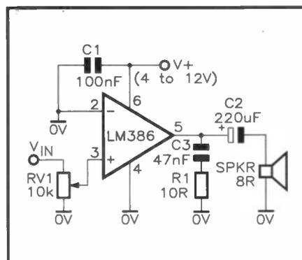
Figure 9. Minimum-parts LM386 amplifier with AV = 20.
