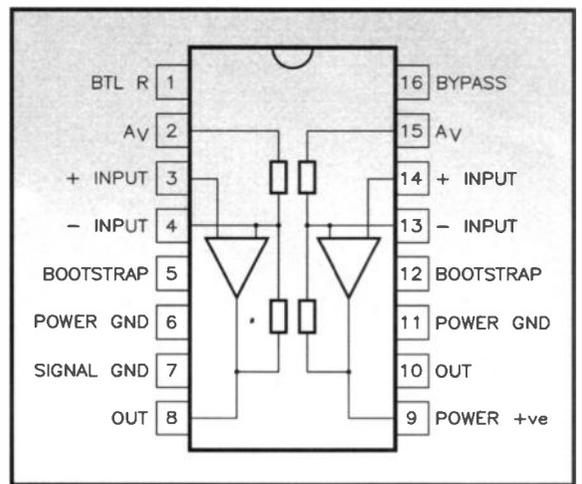
Figure 18. LM831 dual low-voltage audio power amplifier.
