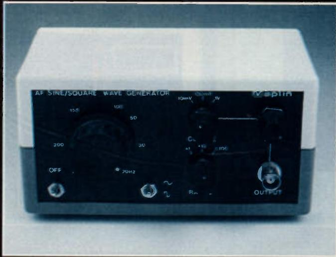
Above left: An audio frequency sine and square wave generator (LT25C), available as a kit, and just right to build.
