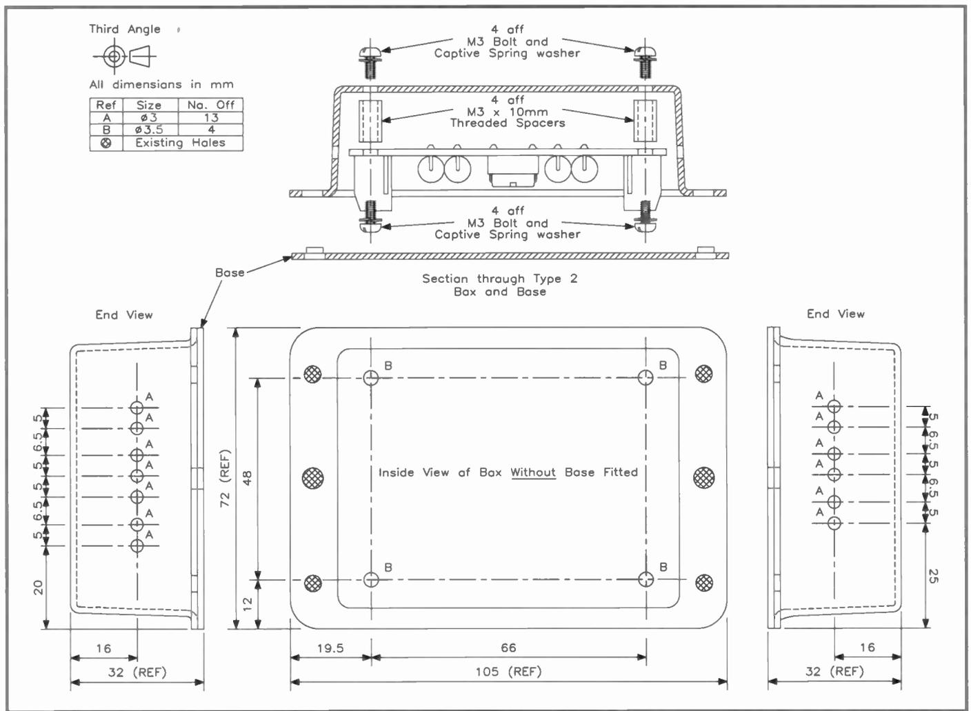
Figure 5. Car Lamp Monitor box drilling details and exploded assembly.
