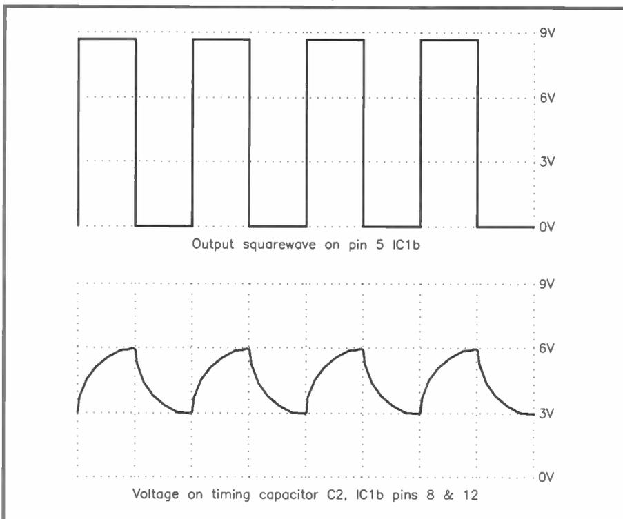
Figure 4. Modulation waveform.
