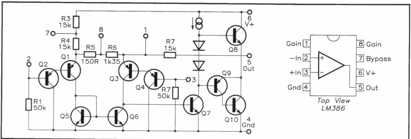
**Figure 8. Internal circuit and pin connections of the LM386 low-voltage audio power amplifier.**
