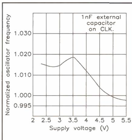
Figure 2(b). Internal oscillator frequency vs. supply voltage.
