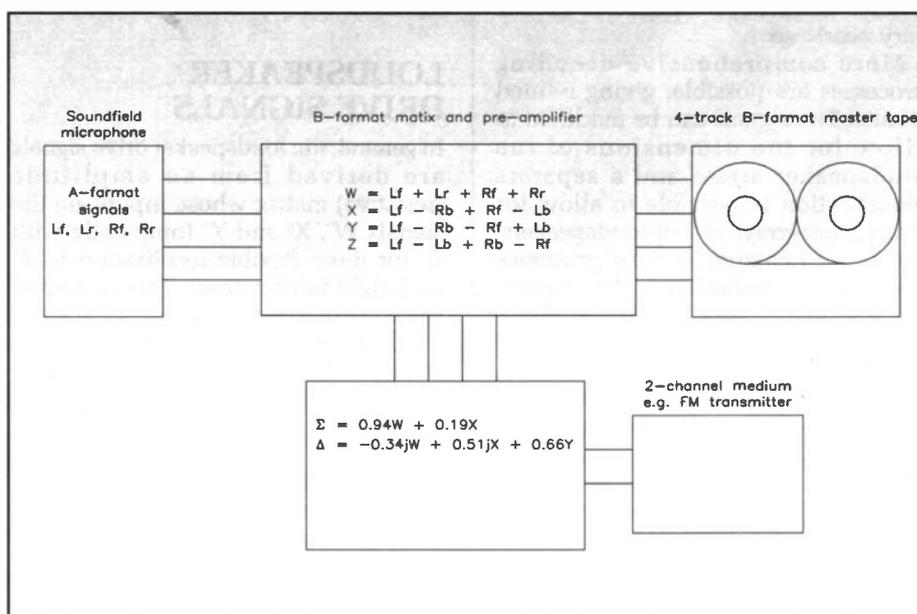
Figure 17a. Example of Ambisonics encoding.
