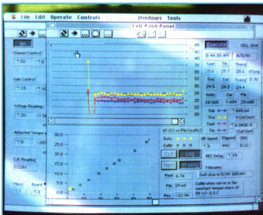
A close up of computer monitor showing the virtual instrument stored in computer memory and used for cell data acquisition and cell monitoring.
