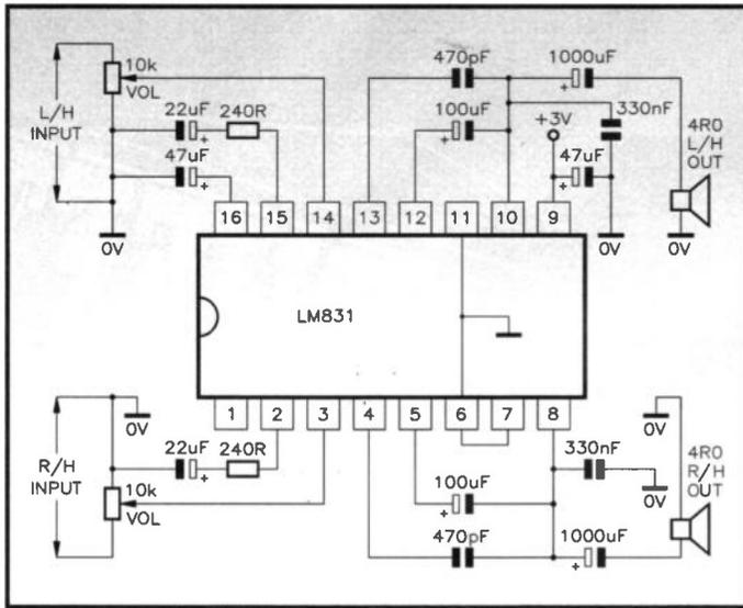
Figure 19. LM831 stereo amplifier.
