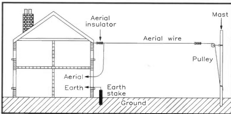
Figure 8a. Conventional end-fed, long wire aerial system.
