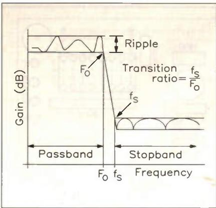
Figure 6. Typical filter response.
