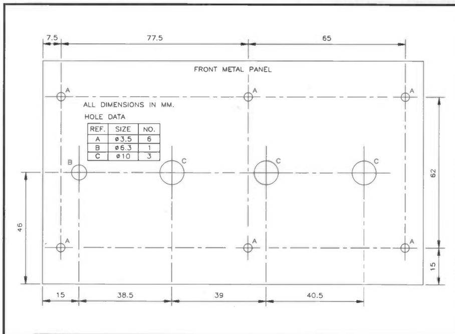
Figure 5b. Front panel drilling.
