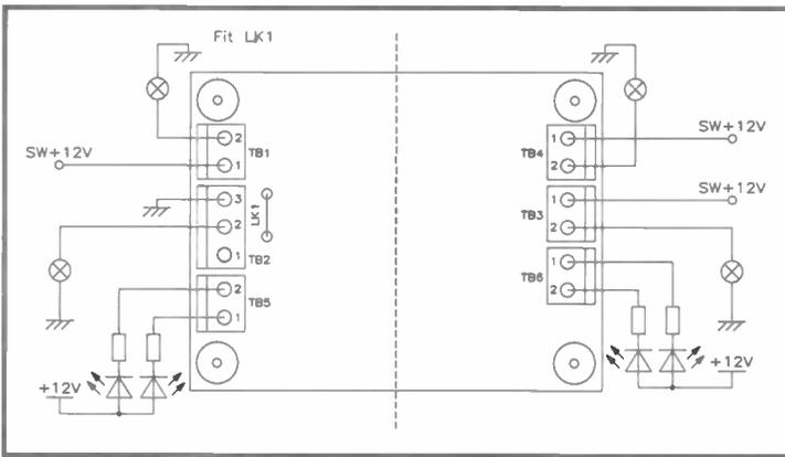
Figure 7a. Separate fault indicator LEDs for each lamp.
