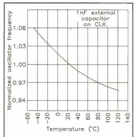
Figure 2(c). Internal oscillator frequency vs. temperature.
