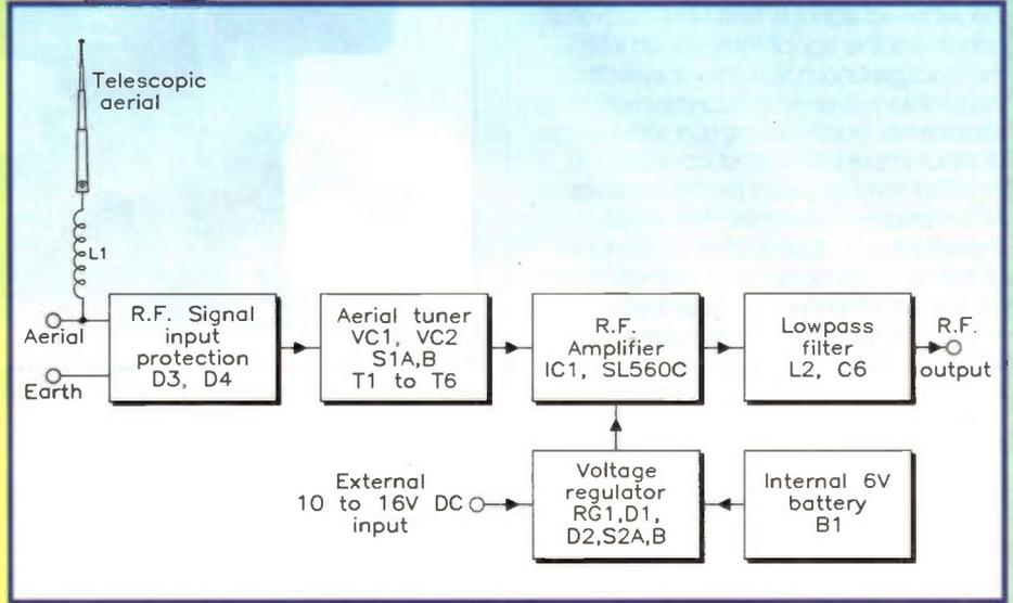
Figure 1. Block diagram of the Aerial Activator.
