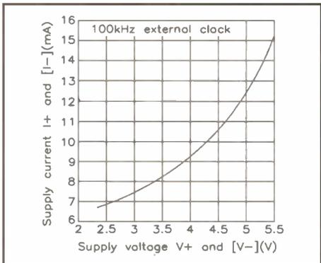
Figure 4. Supply current vs. supply voltage of the MAX293/297 ICs.
