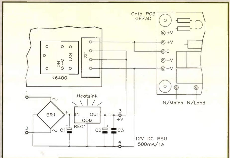
Figure 8. Zero crossing opto switch (LP55K).
