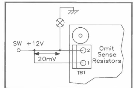
Figure 7d. Sensing voltage drop across wiring.
