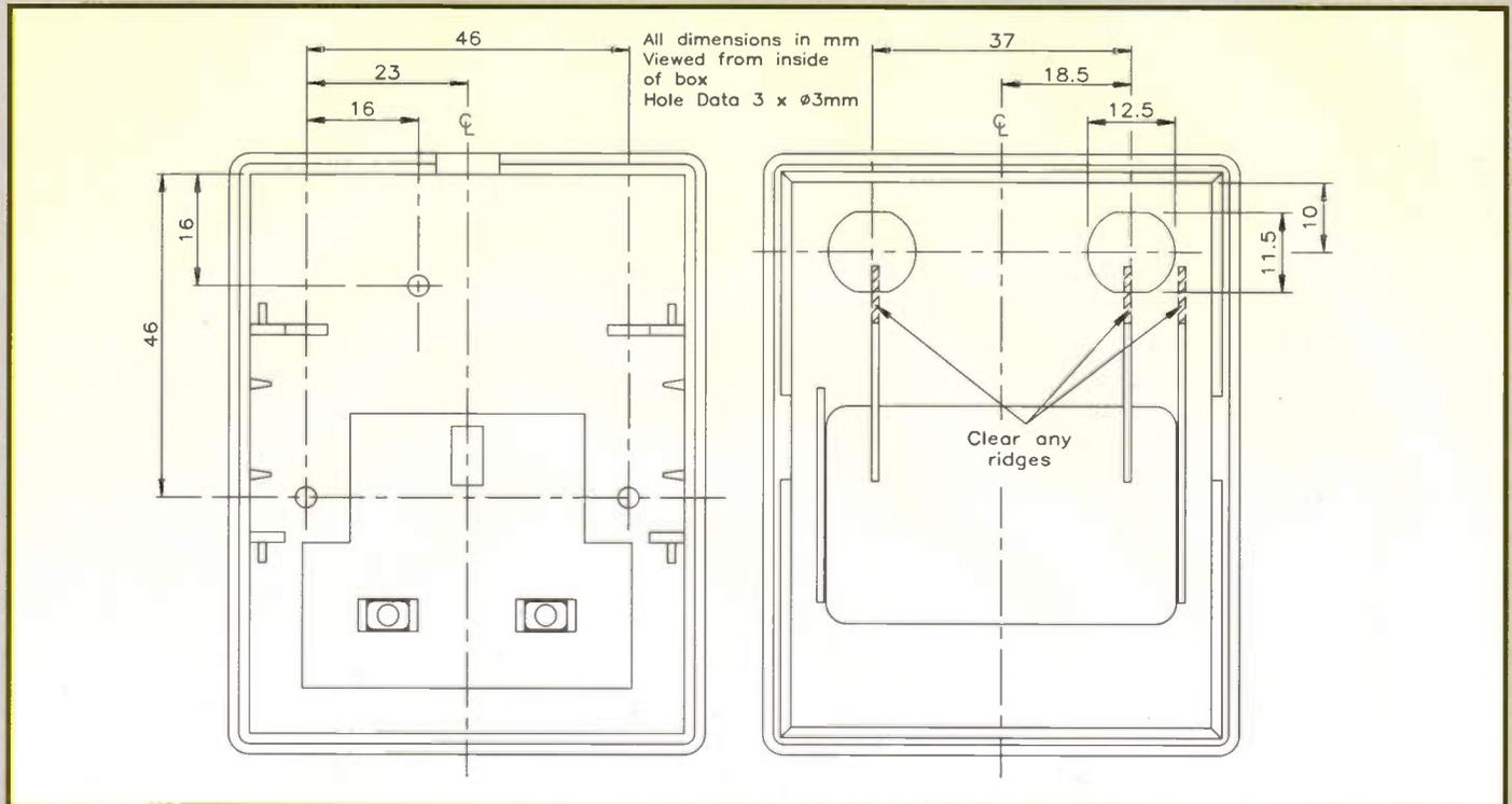
Figure 6b. PSU box drilling details.
