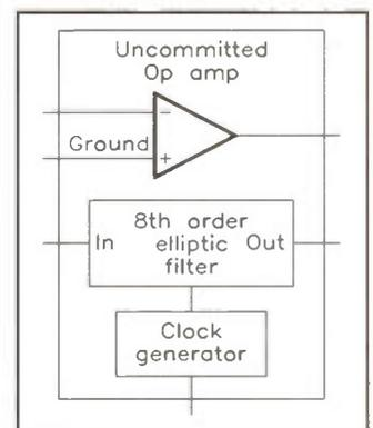
Figure 1(b). MAX293/297 internal diagram.
