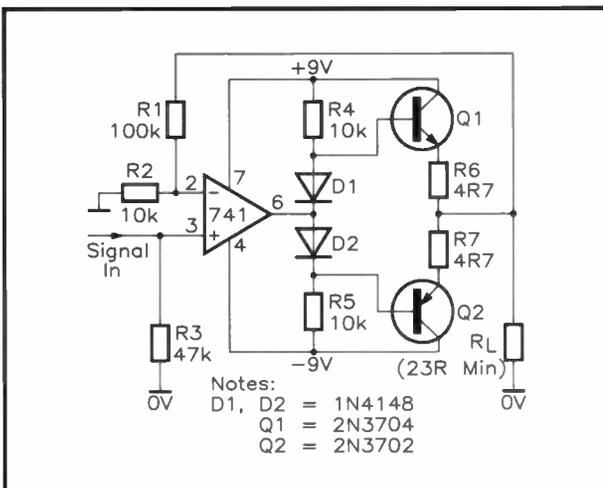
Figure 4. Op amp power amplifier using dual supplies
