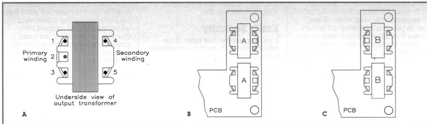
Figure 9. (a) Underside view of output transformer. (b) Type A orientation. (c) Type B orientation.
