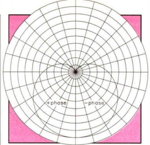
Figure 12b. Impossible directional response required for correct capture of rearward sound in a two-channel system.
