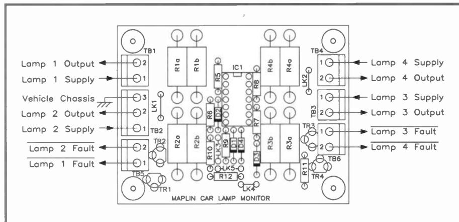
Figure 6. Car Lamp Monitor terminal functions.
