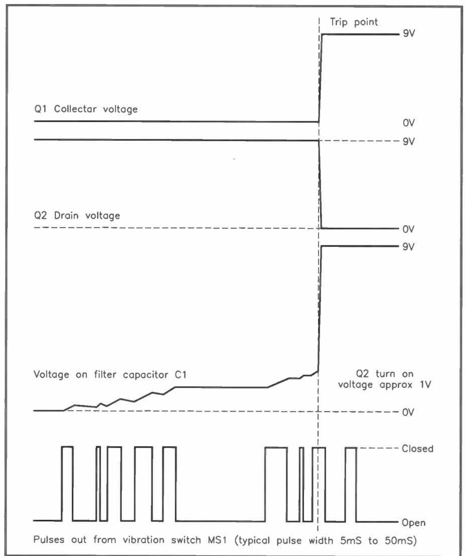
Figure 3. Movement detector, typical waveforms.
