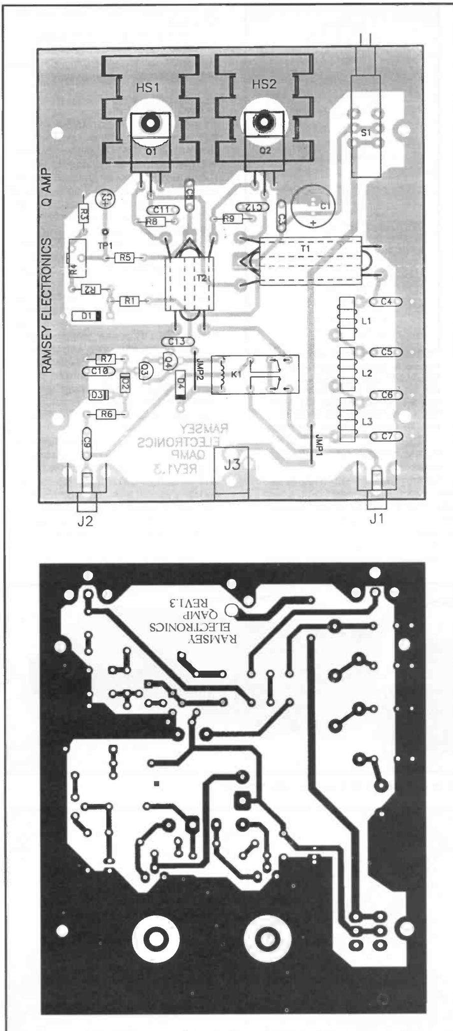
Figure 3. Legend and track of the 20 Metre 20W Linear Amplifier.
