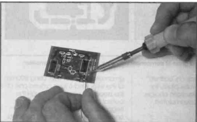
Photo 5c. Making the opposite joint of the component.
