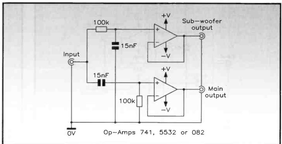
Figure 29a. Crossover for sub-woofer (100Hz).
