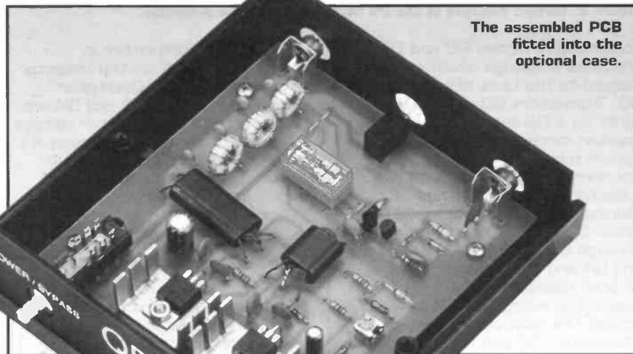
The assembled PCB fitted into the optional case.
