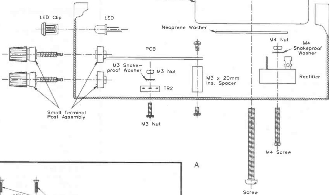
Figure 8a. PWM Drill Motor Speed Controller exploded assembly.
