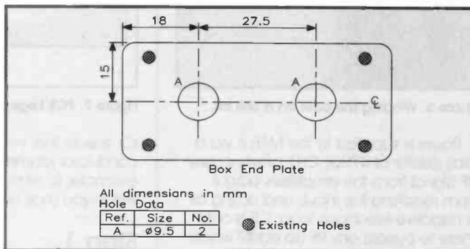
Figure 8. Box drilling of the VHF/UHF Pre-amplifier.
