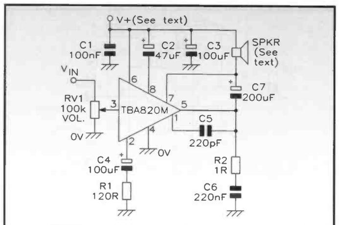
Figure 34. Alternative TBA820M application circuit.
