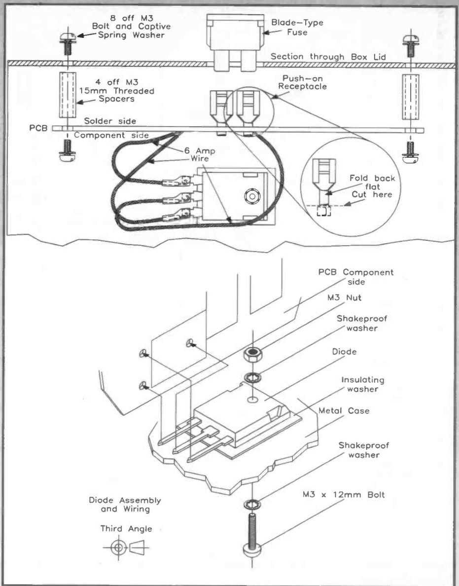
Figure 5. Exploded assembly diagram.
