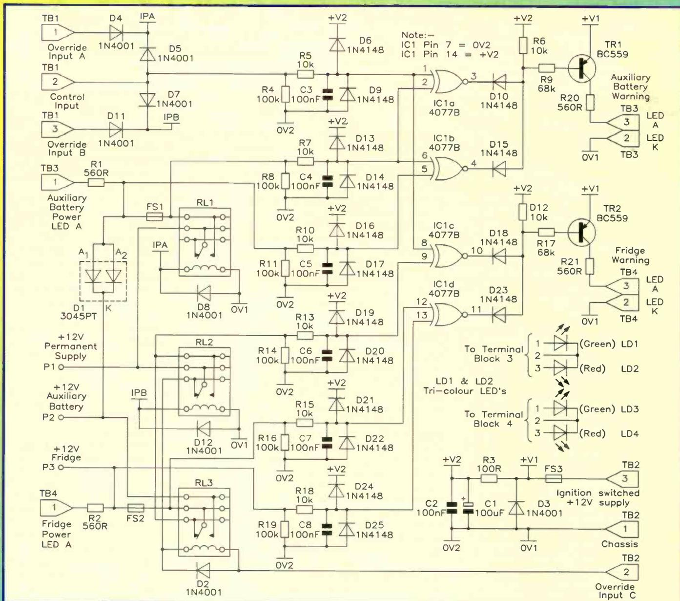
Figure 2. Circuit diagram of the Intelligent Split Charge Unit.
