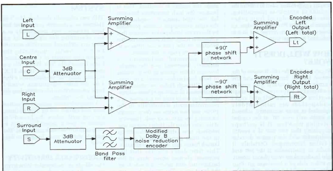
Figure 19. Dolby stereo encoder.
