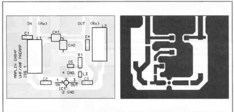
Figure 7. PCB Legend and ghost of component side track of the VHF/UHF Preamplifier.
