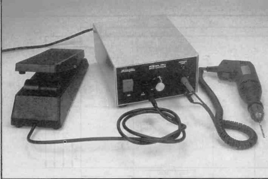
The Drill Speed Controller, optional foot controller and a typical PCB drill.
