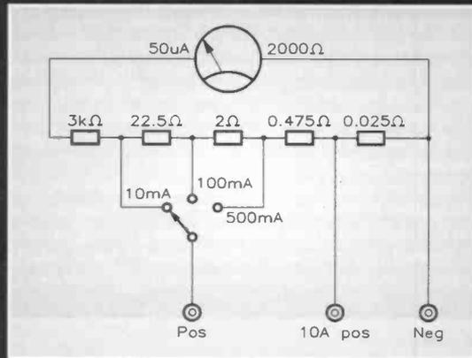
Left: Figure 4. 4-range DC current measuring circuit.
