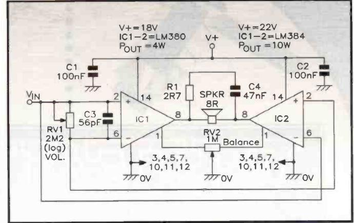
Figure 40. 4W or 10W bridge-configured amplifier.
