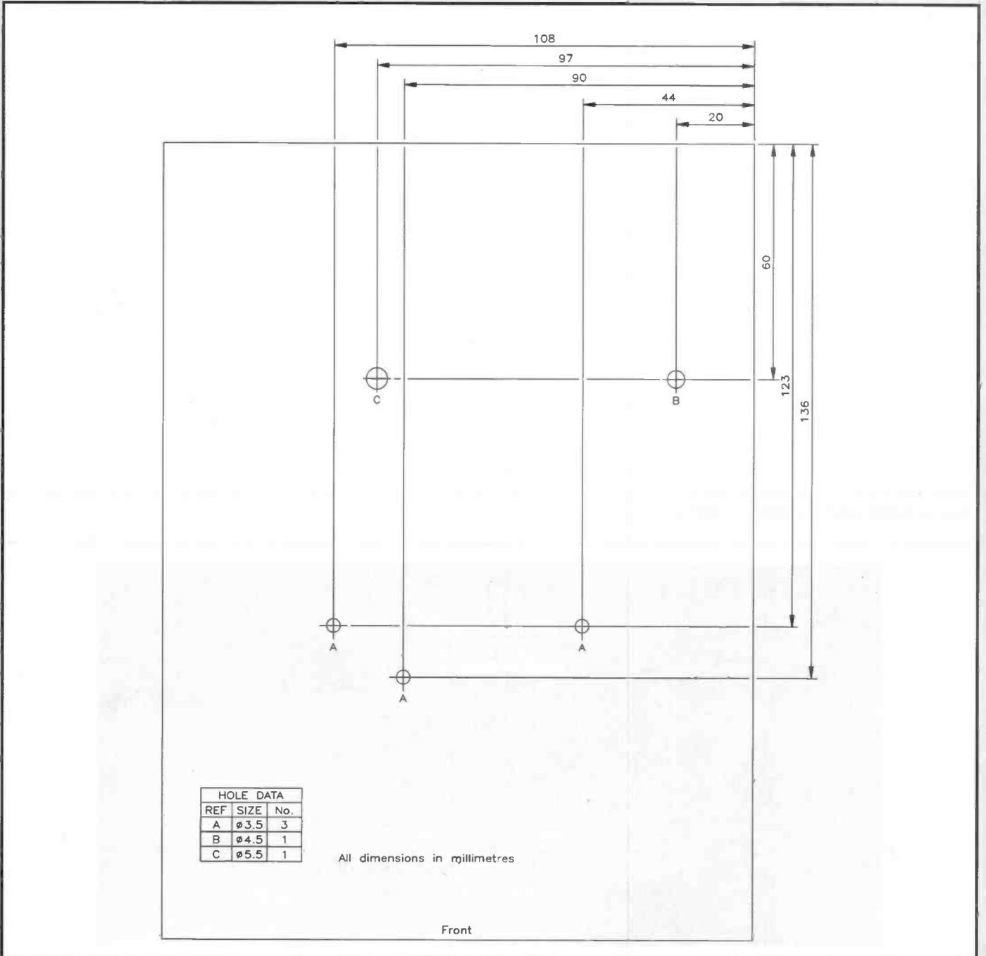
Figure 5b. Drilling details for the base of the box.
