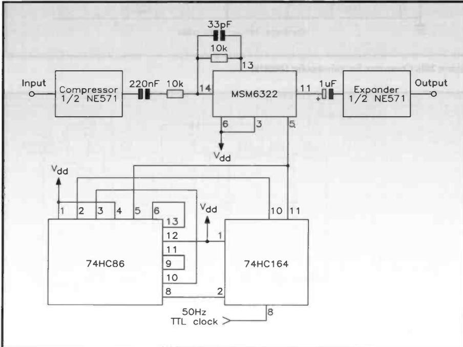
Figure 28. Basis of a pitch-shift decorrelator. The MSM6322 is used in a unity-gain mode at the 'line' input. For further information on this device, see the Data File in issue 44 of *Electronics* (XA44X). The multiple inversions in the 74HC86 are to prevent latch-up in the 'all-zeroes' condition.
