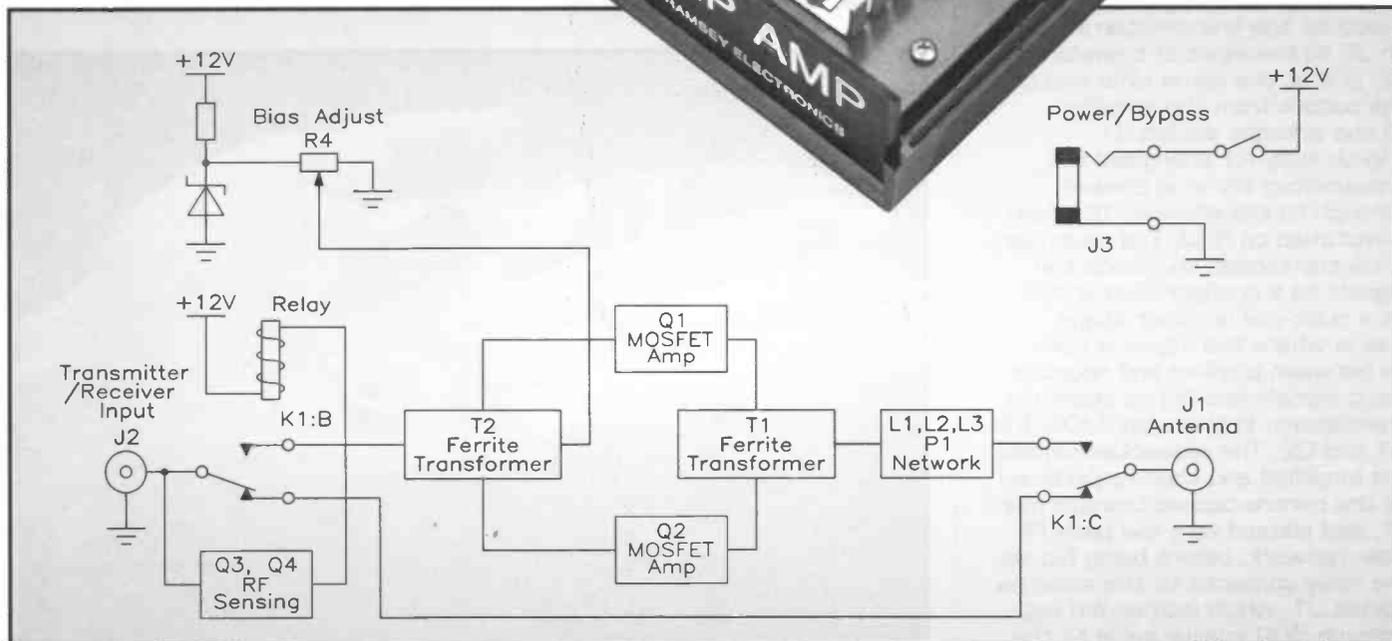
Figure 1. Block diagram of the 20 Metre 20W Linear Amplifier.
