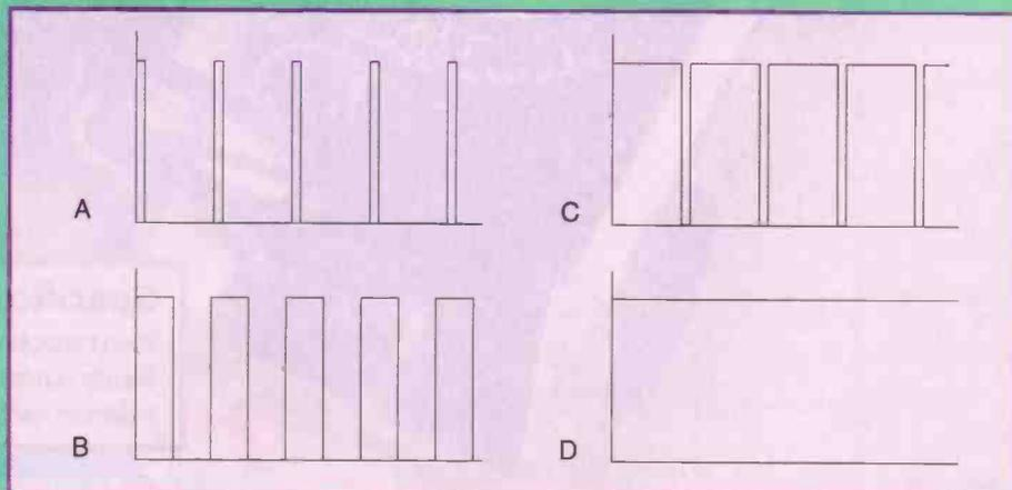
Figure 3. The PWM Drill Speed Controller Waveforms.
