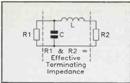
Figure 4. Low-pass input filter configuration of the VHF/UHF Preamplifier.
