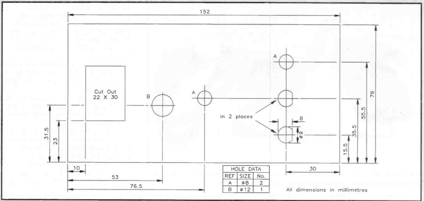
Figure 5a. Drilling details for the front of the box.
