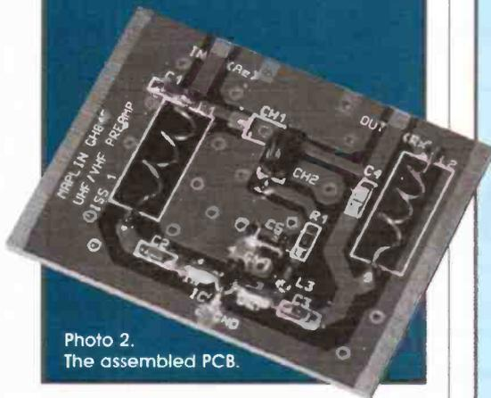
Photo 2. The assembled PCB.
