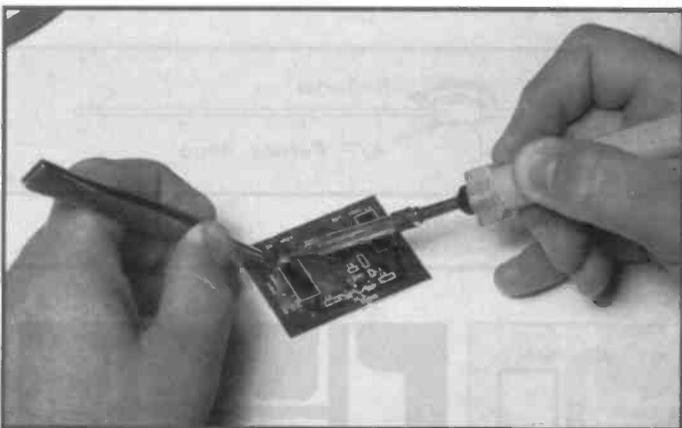
Photo 5b. Holding components in position with tweezers and reflowing the solder to wet the component.
