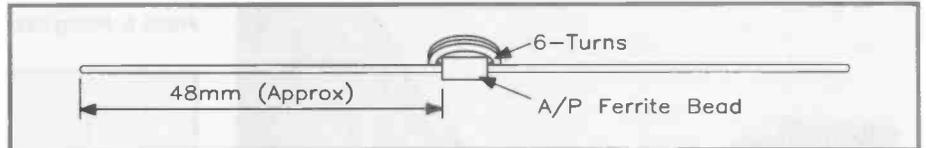
Figure 6. Making the chokes for the VHF/UHF Preamplifier.
