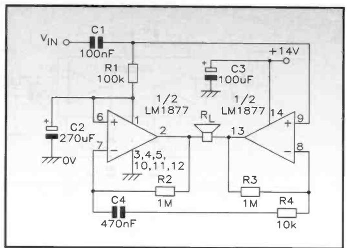
Figure 32. Bridge amplifier circuit using an LM1877 'dual' IC.
