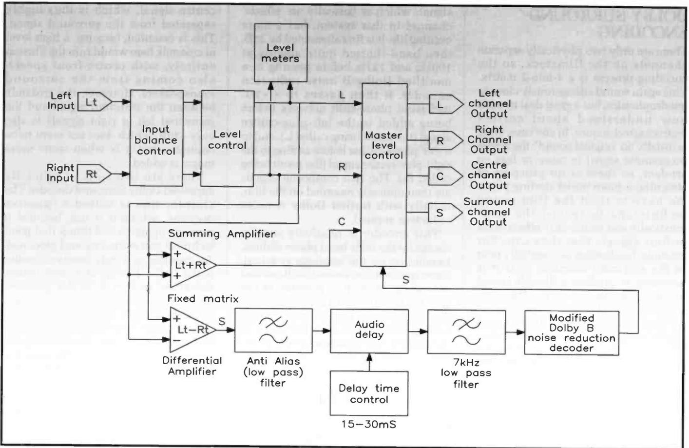
Figure 20. Dolby Surround 'passive' decoder. The level meters and level control are required so that the Dolby-B decoding is correctly applied; the Centre Channel is optional and the Fixed Matrix can be realised as an M-S matrix.
