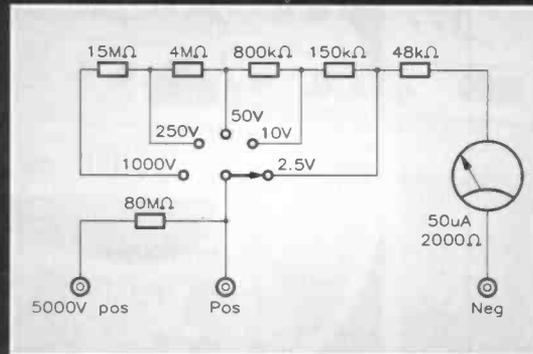
Left: Figure 3. 6-range DC voltmeter circuit, based around a  $50\mu\text{A}$  movement.
