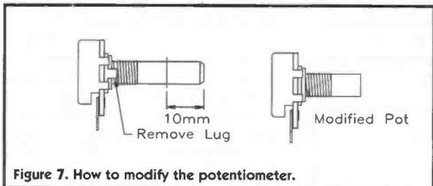
Figure 7. How to modify the potentiometer.
