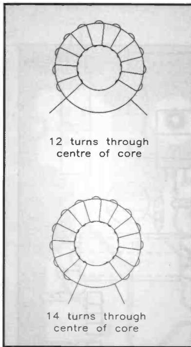
**Figure 5. Construction of the toroid RF coils L1 and L2. (a). L1 toroid RF coil showing the 12 turns through the core. (b). L2 toroid RF coil showing the 14 turns through the core.**
