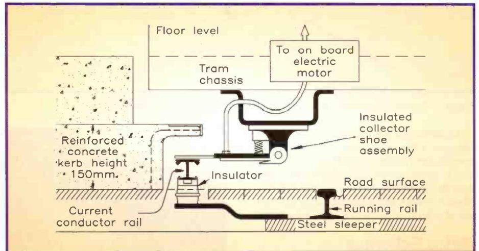
Figure 3. Track-side conductor for recharging the flywheel.
