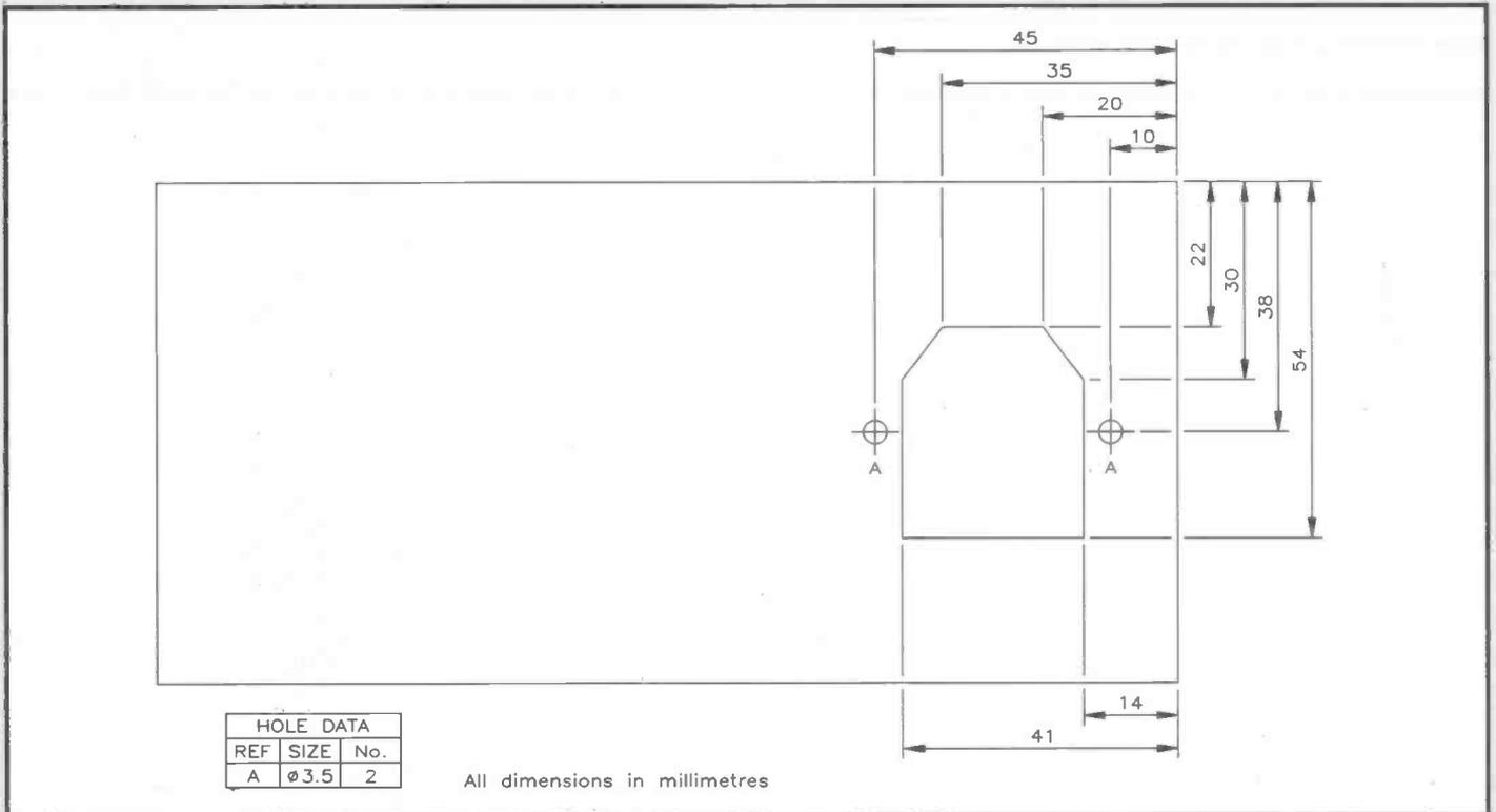
Figure 5c. Drilling details for the rear of the box.
