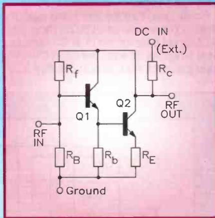
Figure 1. Internal circuit diagram of the MAR-6 chip.
