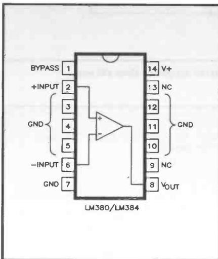
Figure 35. Outline and pin notations of the LM380 and LM384 ICs.
