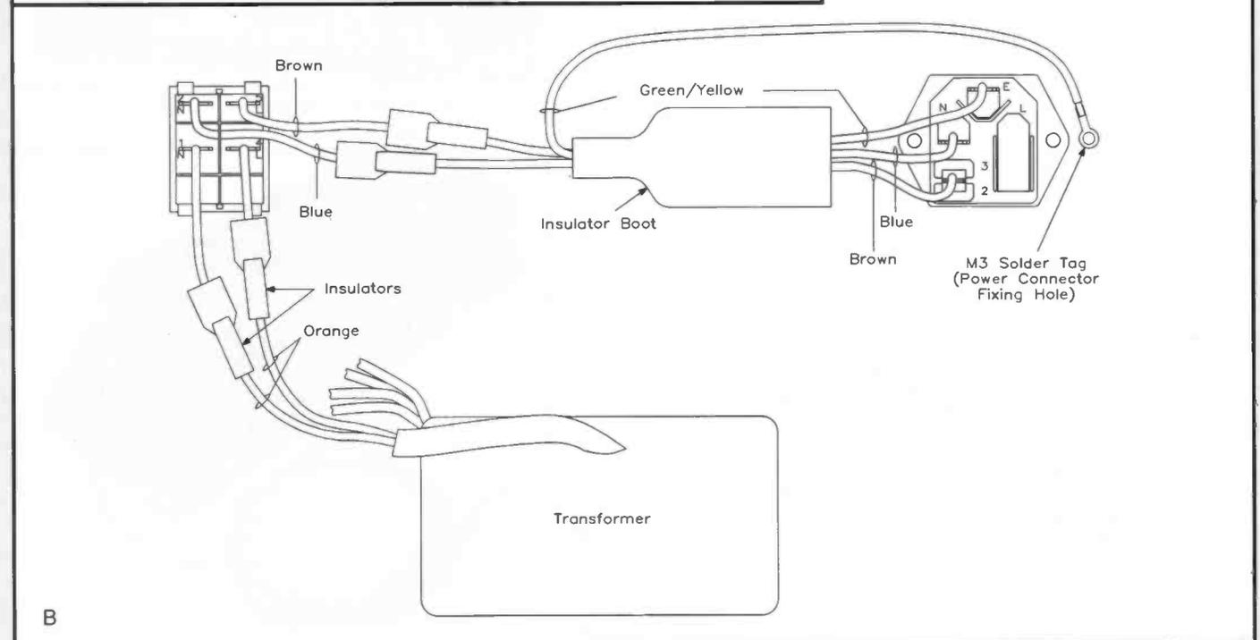
Figure 9. (a) Low-voltage and transformer primary wiring; (b) mains-voltage wiring.
