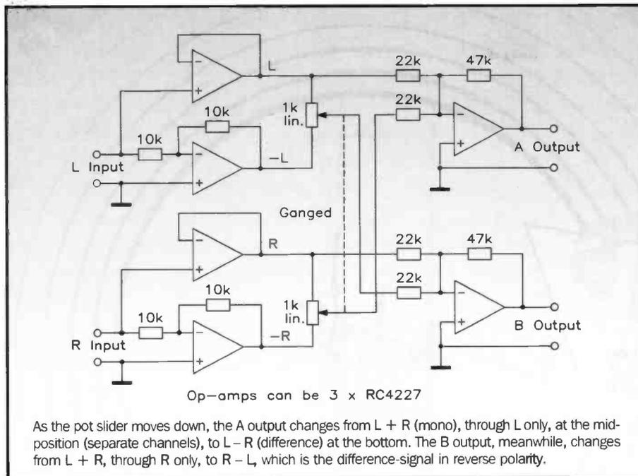
As the pot slider moves down, the A output changes from L + R (mono), through L only, at the mid-position (separate channels), to L - R (difference) at the bottom. The B output, meanwhile, changes from L + R, through R only, to R - L, which is the difference-signal in reverse polarity.
