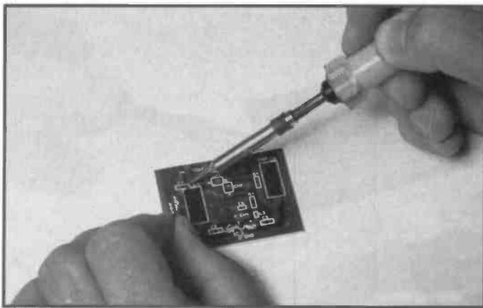
Photo 5a. Wetting one of the component pads with solder.
