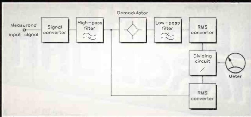
Figure 11. Intermodulation distortion measuring system.
