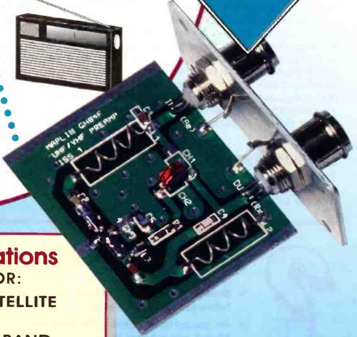
Right: The assembled VHF/UHF Preamplifier
