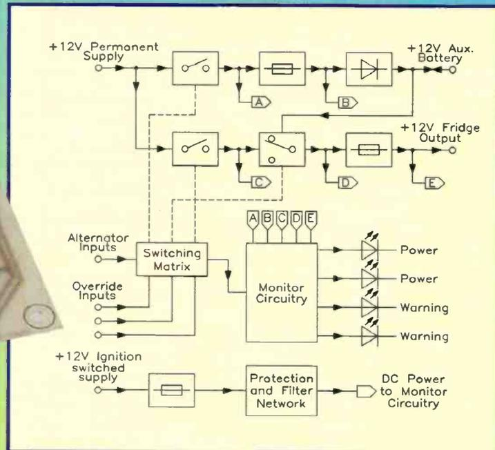
Figure 1. Block diagram of the Intelligent Split Charge Unit.
