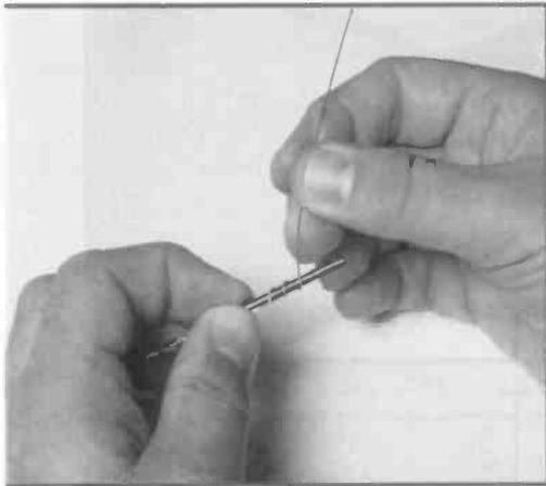
Photo 3. Winding the coils on a drill bit.
