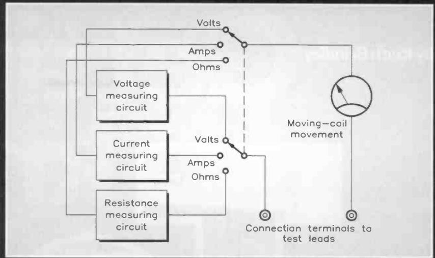
Above: Figure 2. Block diagram of a basic multimeter.
