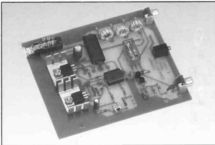
The assembled 20 Metre 20W Linear Amplifier PCB.
