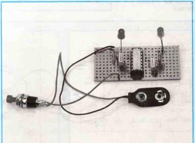
The assembled CMOS 4001/4011 chip tester.
