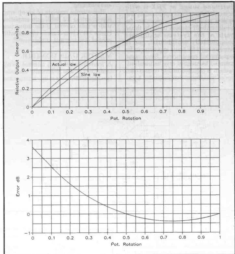
Figure 23b. Characteristics of the approximate sine-cosine potentiometer.
