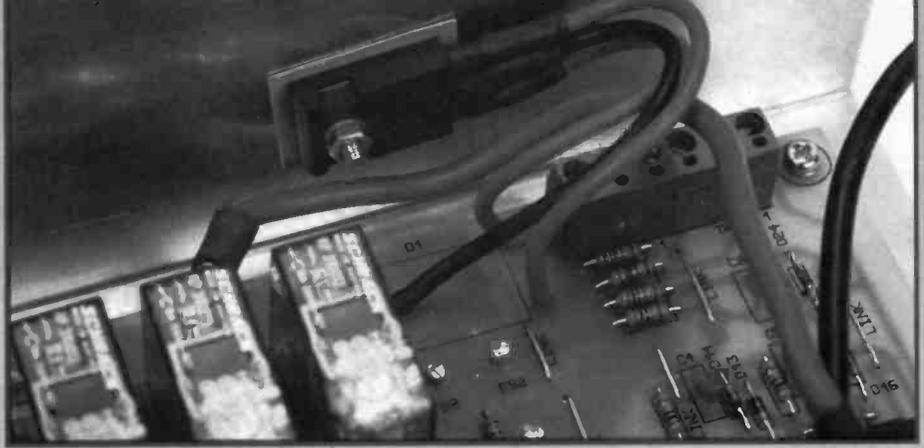
The complete Split Charge Unit ready for installation.
