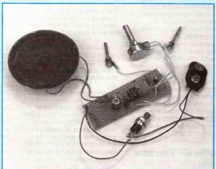
The assembled soil moisture tester.
