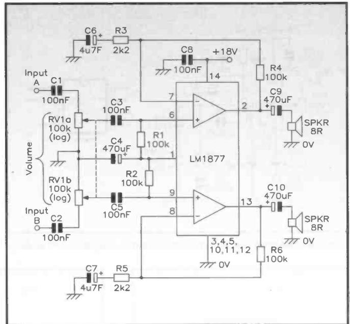
Figure 28. Non-inverting stereo amplifier gives 2W per channel output.
