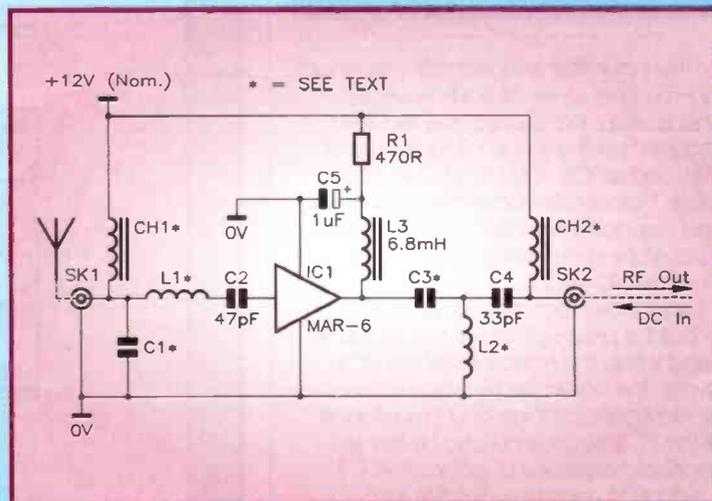
Figure 3. Circuit diagram of the VHF/UHF Preamplifier.
