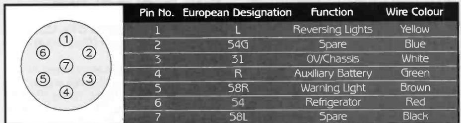
Figure 7. 12V supplementary connector pinout.
