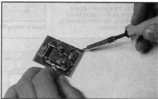
Photo 7. Fitting the finned copper wire inductors.
