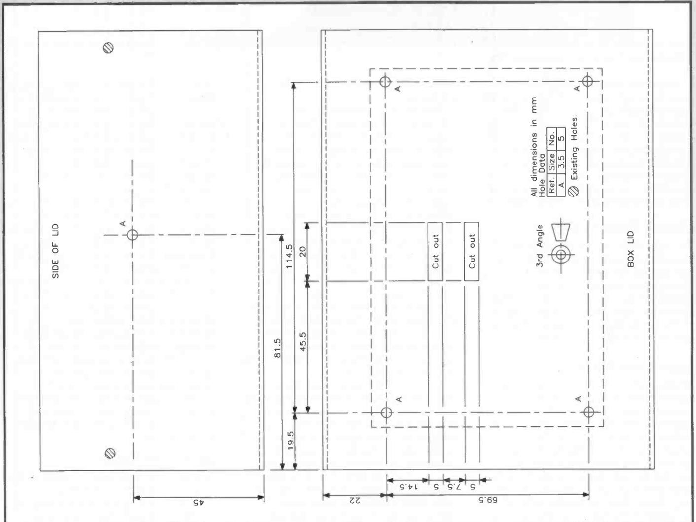
Figure 4. Drilling details of the suggested box.
