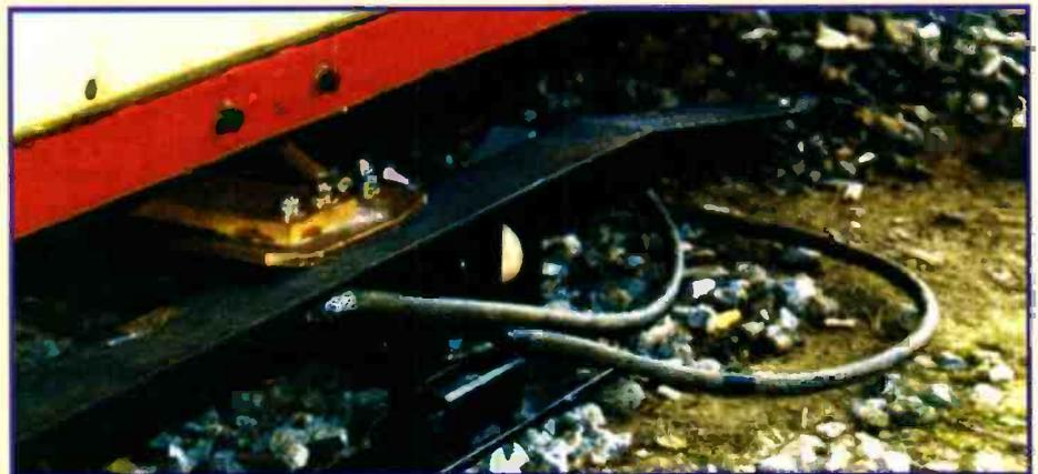
PPM Minitram contactor butts up to power source to recharge flywheel.
