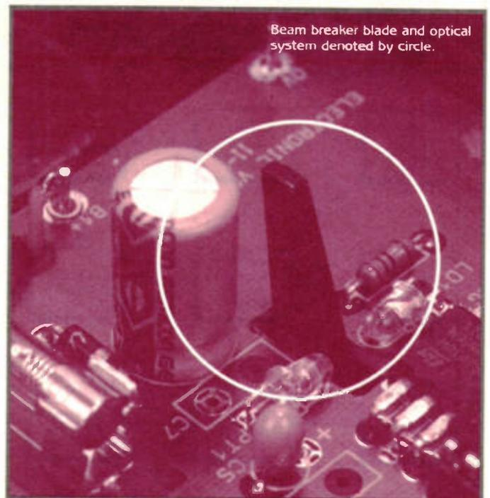
Beam breaker blade and optical system denoted by circle.
