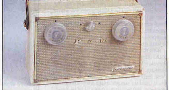
Photo 4. An early transistor portable radio – a Pam 720 made by Pye in 1956/7; the second transistorised set they produced, covering medium wave plus pre-set on long wave for receiving the Light Programme (Courtesy G. C. Arnold Partners).
