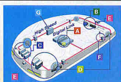
Photo 2. How Japanese in-car electronics manufacturer, Alpine, sees the future of integrated car electronics. Key: A = Mobile Media Computer, B = Interface Unit, C = Communication Unit, D = Audio/Visual Unit, E = Safety Unit, F = Sensor Unit, G = Security Unit.
