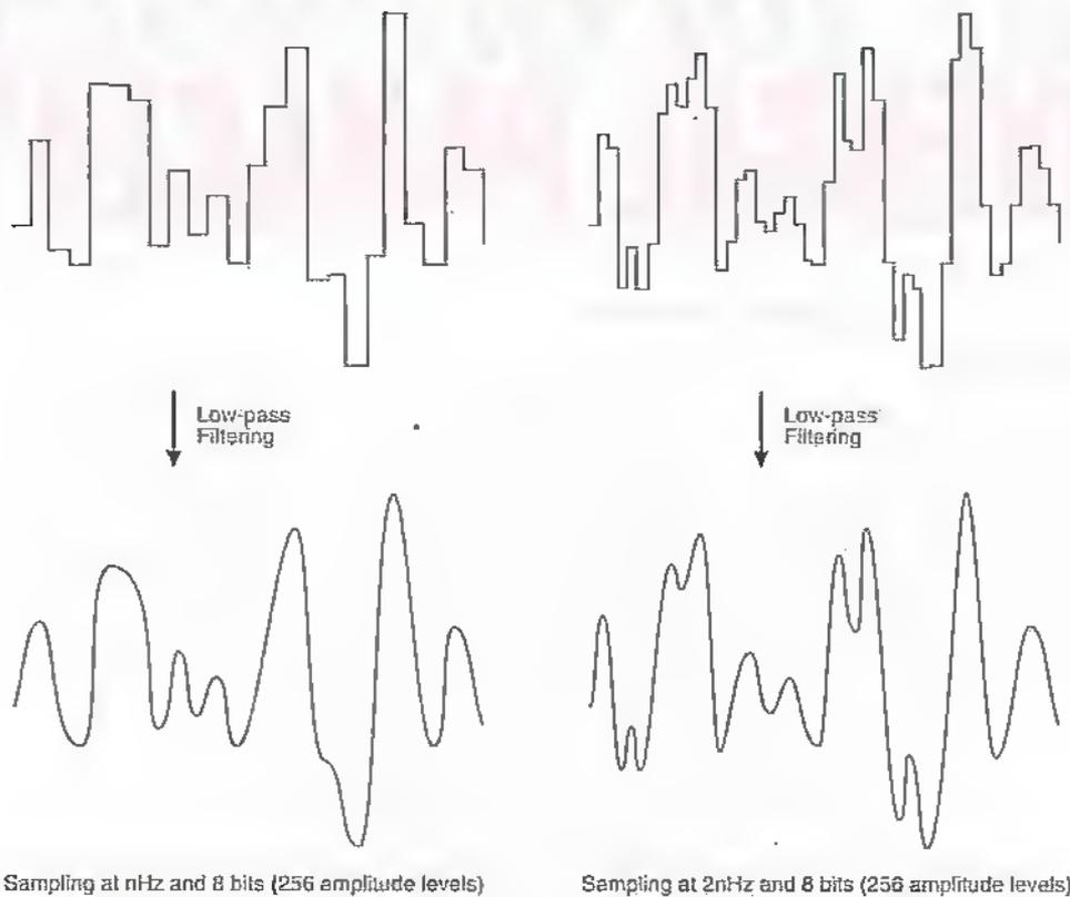
staircase waveform, so the signal then has to be filtered to remove the high frequency components in the steps and thereby generate a waveform similar to the analogue original. There are two factors which affect this sampling process – the frequency at which the sampling is carried out and the resolution to which each sample is measured and stored.
