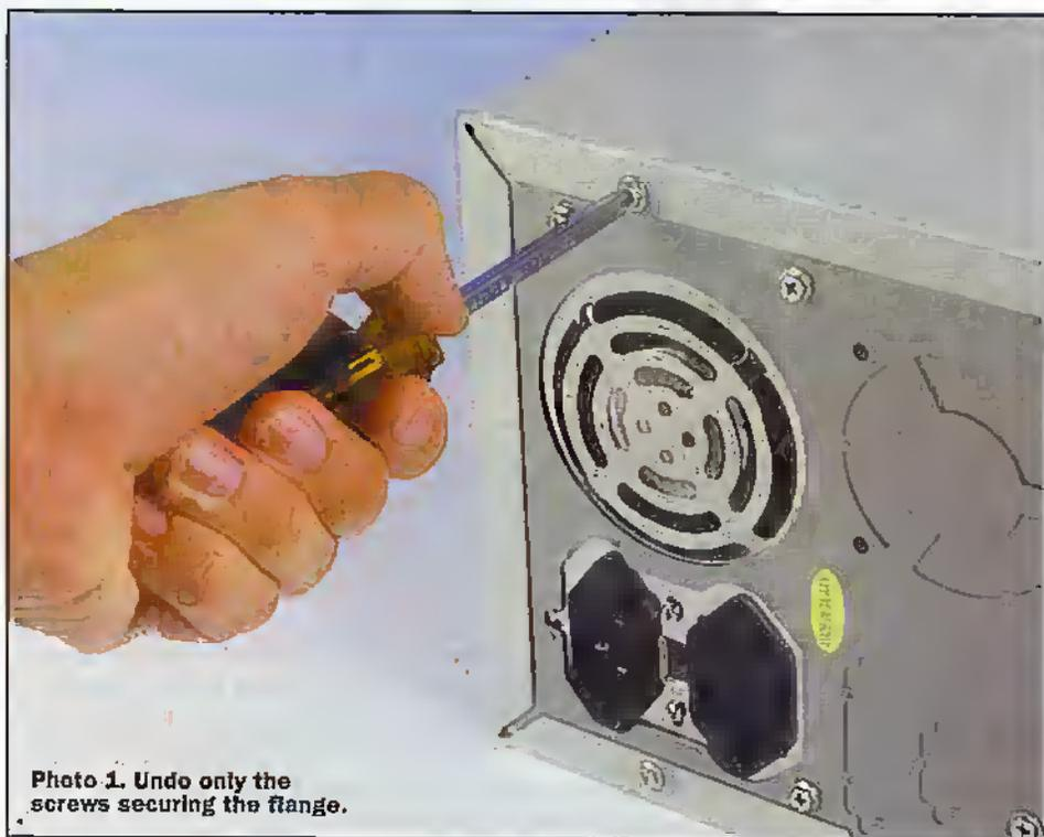
Photo 1. Undo only the screws securing the flange.
