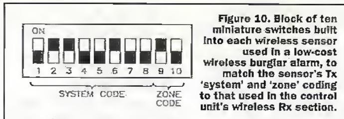
**Figure 10.** Block of ten miniature switches built into each wireless sensor used in a low-cost wireless burglar alarm, to match the sensor's Tx 'system' and 'zone' coding to that used in the control unit's wireless Rx section.
