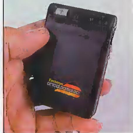
NV89X Optoelectronics Micro Frequency Counter.
