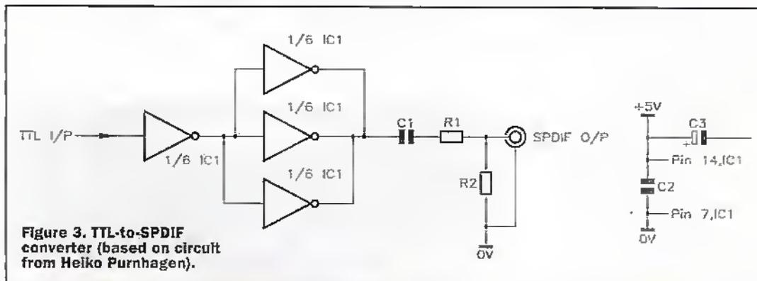
**Figure 3. TTL-to-SPDIF converter**
