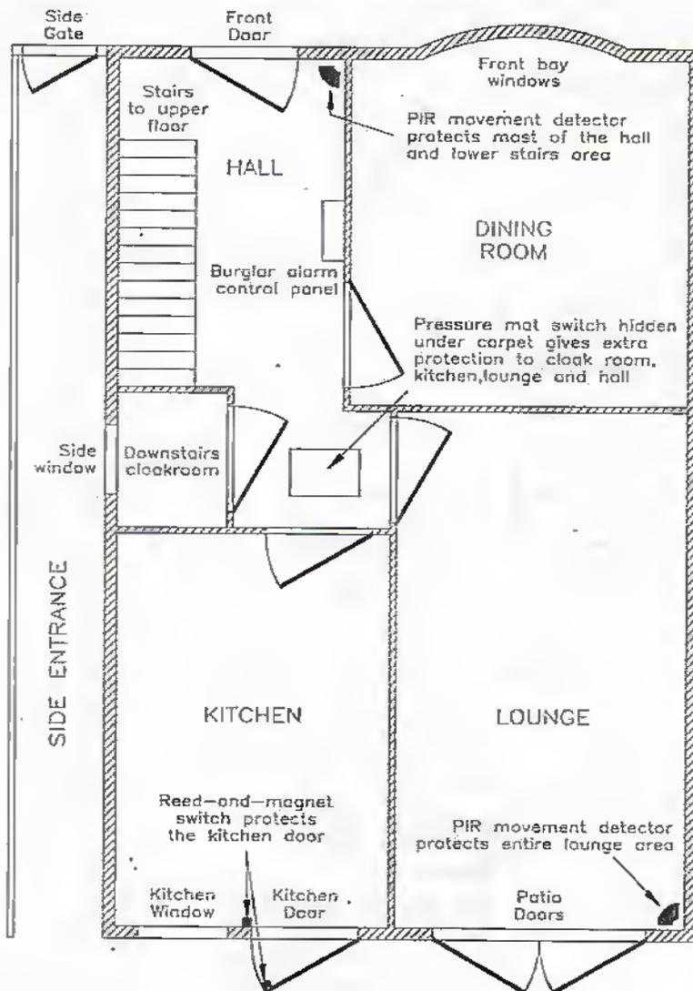
Figure 5. Ground floor plan of a semi-detached house, showing suitable positions for anti-burglary defences.
