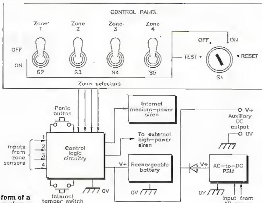
**Figure 7.** Typical basic form of a modern burglar alarm control unit and its control panel.
