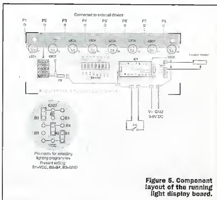
**Figure 5. Component layout of the running light display board.**
