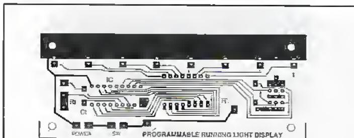
**Figure 4. PCB Board of the running light display board.**
