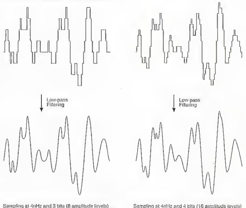
down this track, it has to be pointed out that our eyes and ears, even though they are analogue devices, have their limitations. So if the sampling rate and the sampling resolution of a digital signal are sufficiently high, the human senses won't notice the difference between this and the true analogue signal it represents. The trick, of course, is to choose a sufficiently high sampling rate and resolution to fool our eyes or ears, yet not to pick figures which are so high
