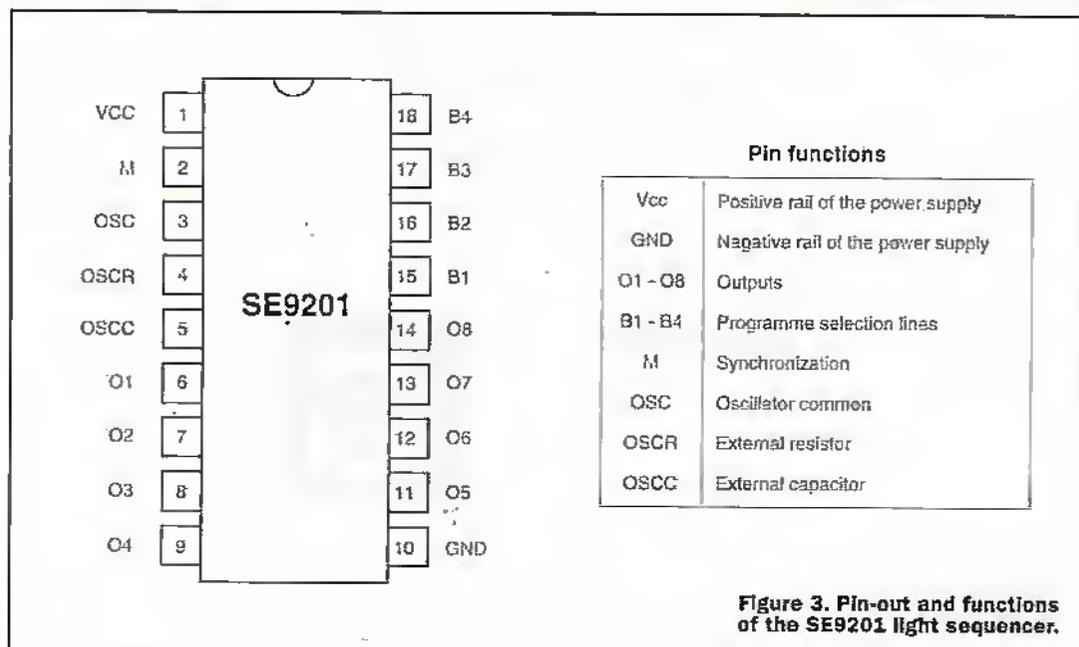
**Figure 3. Pin-out and functions of the SE9201 light sequencer.**
