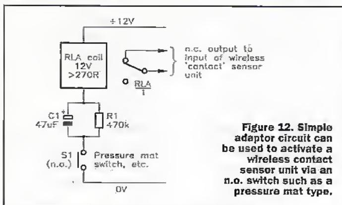
**Figure 12.** Simple adaptor circuit can be used to activate a wireless contact sensor unit via an n.o. switch such as a pressure mat type.
