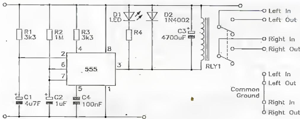
Figure 1. Circuit diagram of the loudspeaker control circuit
