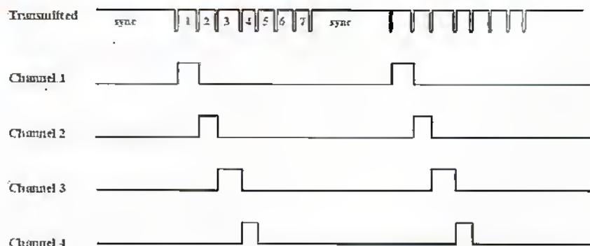
**Figure 1. Radio Control Data Transmission.**
