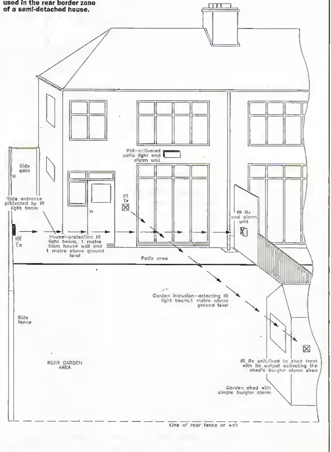
break into them before attacking the actual house. Thus, always fit your shed and garage with a simple battery-powered burglar alarm that activates a loud siren and a light strobe if not disabled (via a secret switch) within about 20 seconds of opening the shed/garage door.
