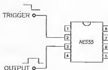
Figure 3. Trigger versus output timing cycles for NE555
