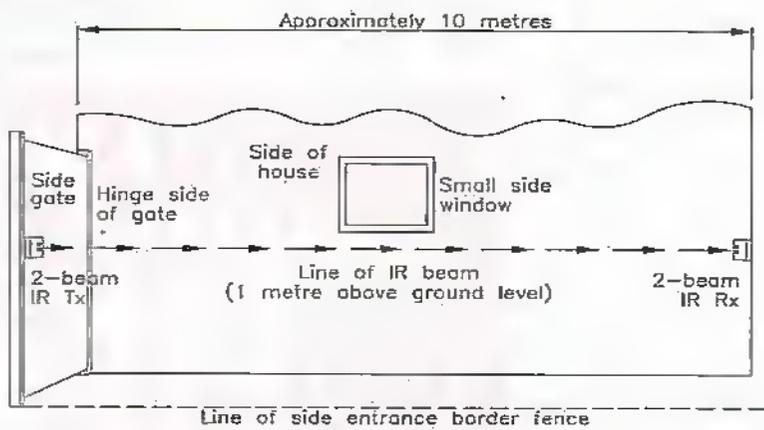
by a PIR alarm fitted with a 'corridor' type of lens, or by an IR dual 'light beam' alarm of the type described in Part 5 of this series; Figure 3 shows the basic arrangement of a suitable 2-beam IR light beam alarm system.
