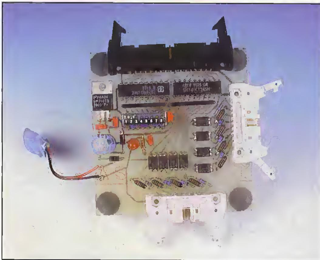
The light emitter and detector are physically spaced apart, usually by a few millimetres of plastic, which can provide electrical isolation up to several thousand volts. Because of these high ratings opto-isolators are used extensively in mains control systems, providing isolation between the "cold" low-voltage control circuits and the "hot" high-voltage mains switching circuits.
