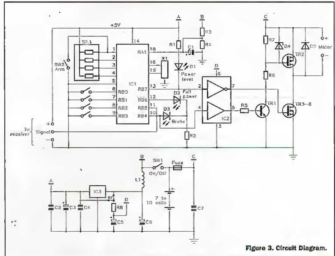
Figure 3. Circuit Diagram.
