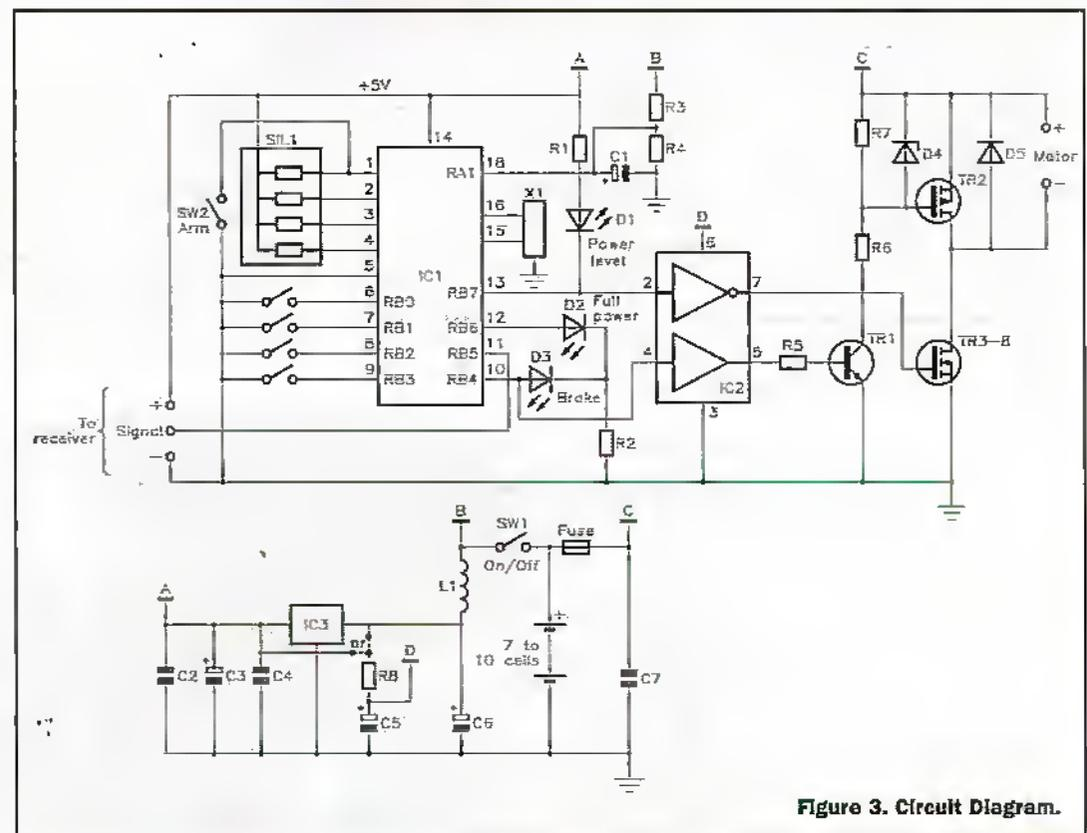
Figure 3. Circuit Diagram.
