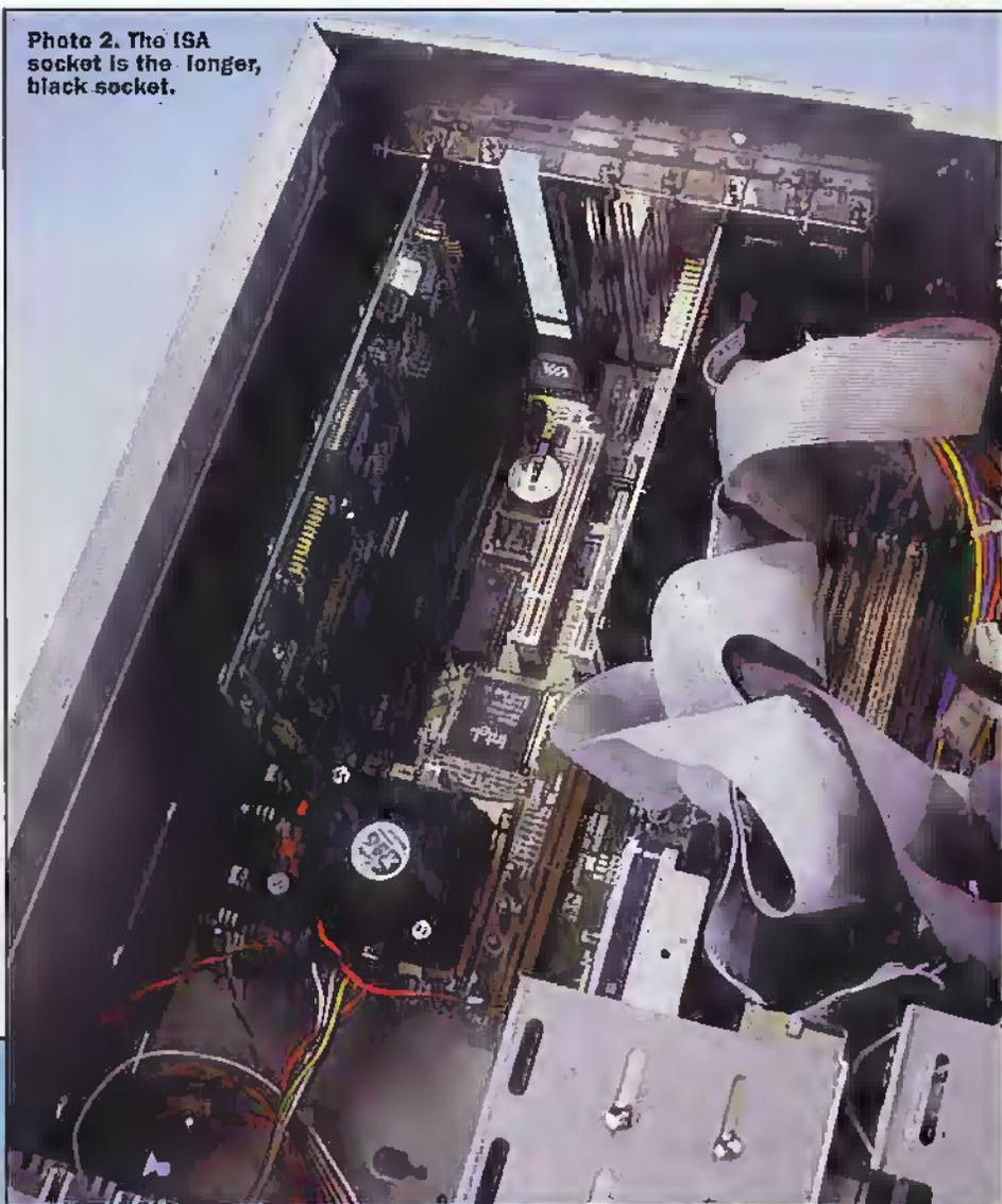
The PC's main board, called the motherboard because the smaller daughterboards plug into it, has a row of long expansion sockets at the back. You will see that some of these already have boards plugged into them. Your graphics card, sound card and possibly your I/O and disk drive controller cards all plug in here.
