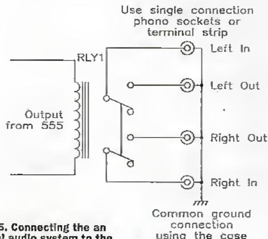
**Figure 5. Connecting the an external audio system to the loudspeaker control system**
