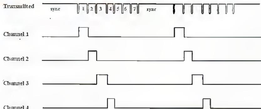
**Figure 1. Radio Control Data Transmission.**
