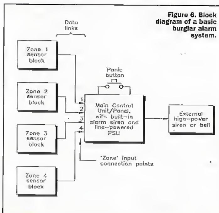
Figure 6. Block diagram of a basic burglar alarm system.
