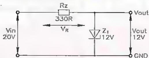
**Figure 4. Zener diode is used to bring external voltage within operating parameters of the NE555**
