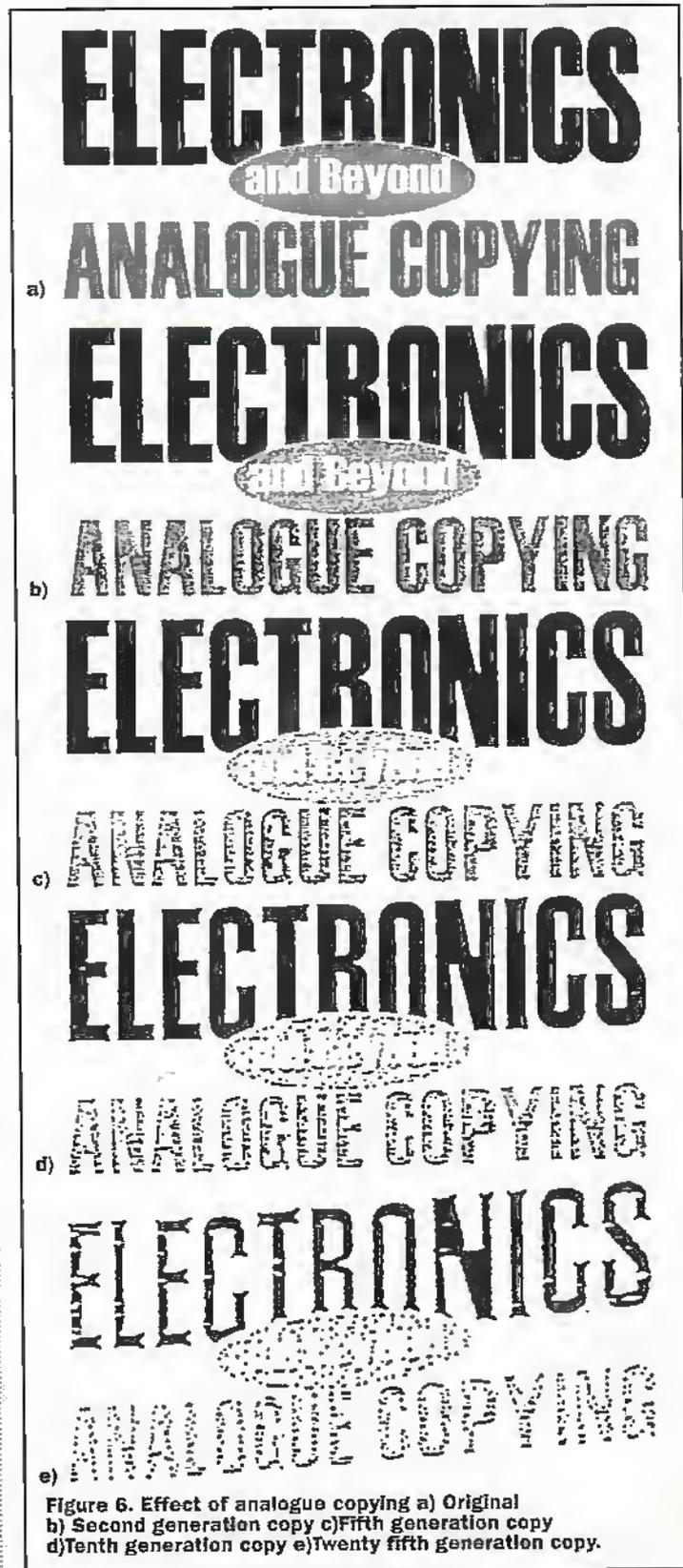
Figure 6. Effect of analogue copying a) Original b) Second generation copy c) Fifth generation copy d) Tenth generation copy e) Twenty fifth generation copy.
