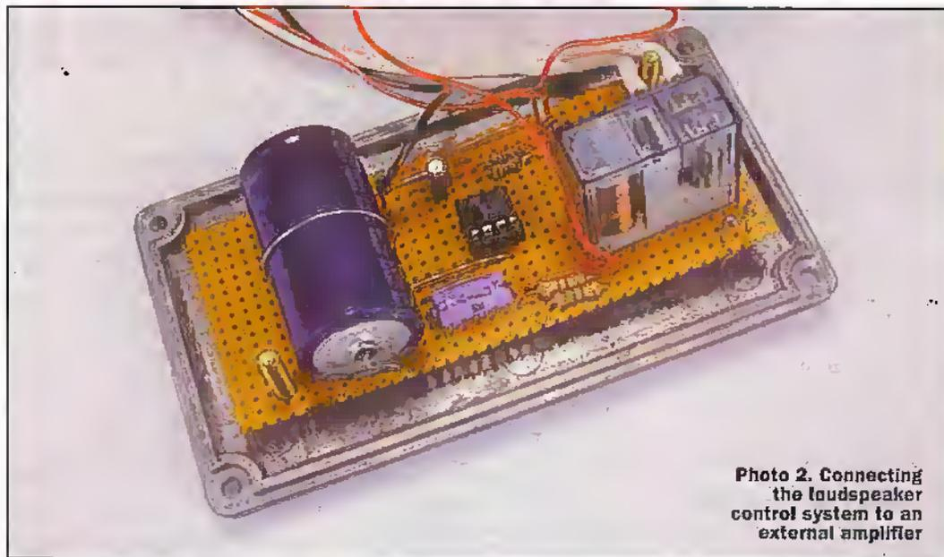
**Photo 2. Connecting the loudspeaker control system to an external amplifier**
