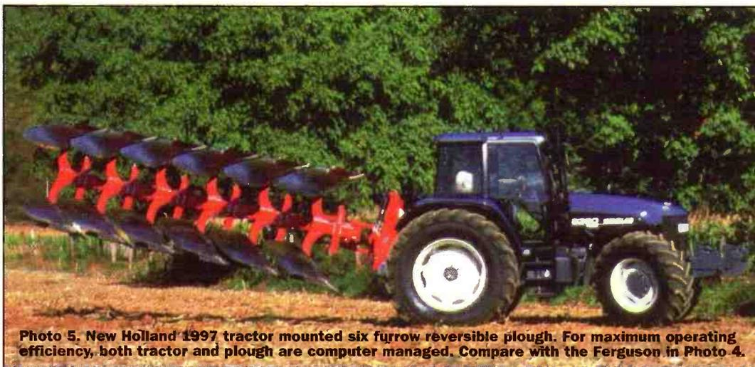
**Photo 5. New Holland 1997 tractor mounted six furrow reversible plough. For maximum operating efficiency, both tractor and plough are computer managed. Compare with the Ferguson in Photo 4.**
