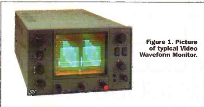
Figure 1. Picture of typical Video Waveform Monitor.
