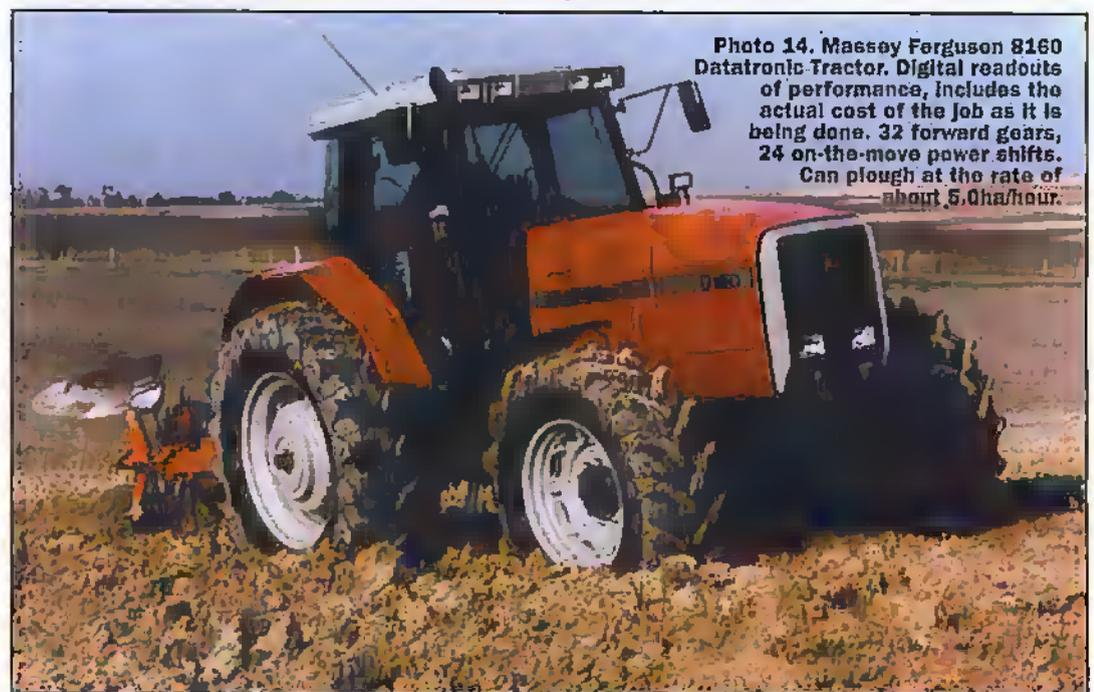
**Photo 14.** Massey Ferguson 8160 Datatronic Tractor. Digital readouts of performance, includes the actual cost of the job as it is being done. 32 forward gears, 24 on-the-move power shifts. Can plough at the rate of about 5.0ha/hour.
