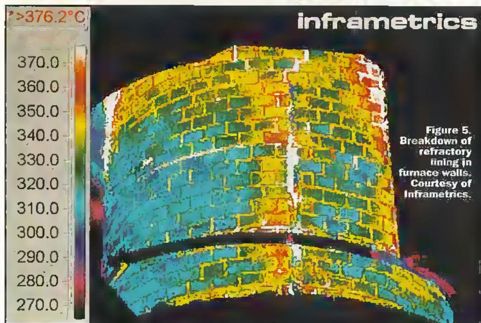
Figure 5. Breakdown of refractory lining in furnace walls. Courtesy of Inframetrics.
